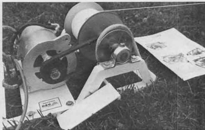
Pulleys are interchangeable between drum shaft and motor shaft to allow variable speed/torque. Comes with extra 2" and 3" pulleys.
