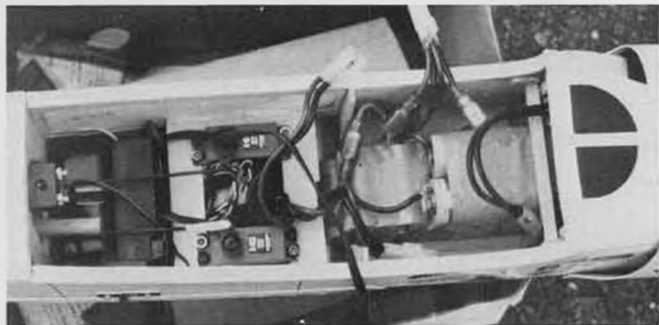
The Pilot Chipmunk holds everything you need right here: RX battery, receiver, aileron & elevator servos, power pack.
