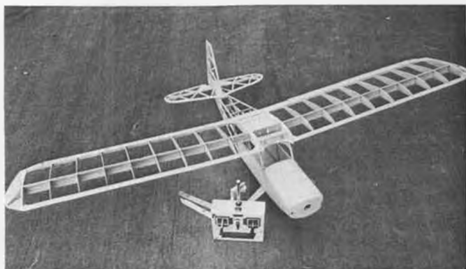
All framed-up and ready for covering, the Citabria looks a bit naked. Cover radio with thumb and you could be looking at F/F rubber job.
