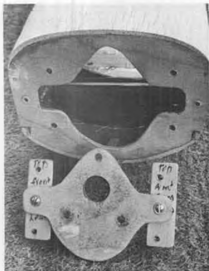
Shock-absorbing mount allows nose impact without damage to motor or gears. Unit is suspended by small springs. See text.
