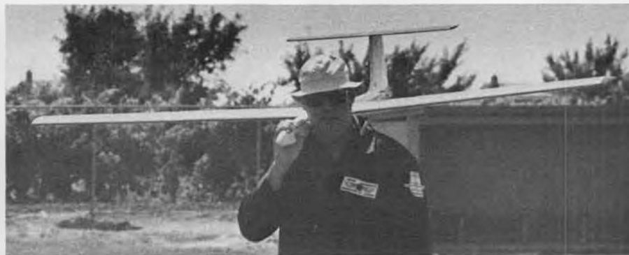
Fred China came from Canada to compete in this year's 2MWC. This is his second World Cup. The plane over his shoulders has: E-205 section, coupled rudder/ailerons, flaps, 17% stab area.
