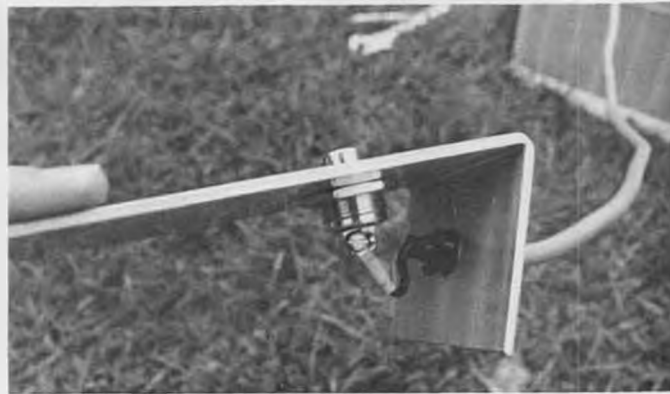
Pow'rtow winch pedal. Borg-Warner heavy duty starter switch is intended for use with solenoids. Had a few problems, however.
