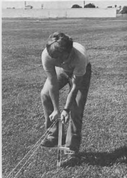
Turnaround is elevated. Bicycle hub is used as pulley. Insert in ground like a shovel, easy!
