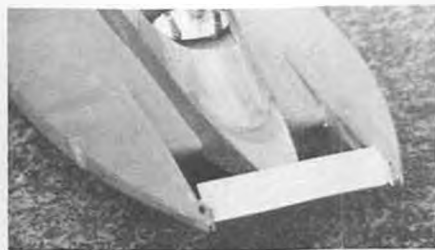
Bow wing keeps the boat down on the water while running into the wind. Try it!
