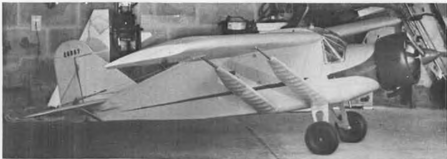
Roland Spicer's record setting Bellanca Skyrocket, built along with a sister ship in five months. Has a built-in nine gallon tank, although she took off with only 6-1/4 gallons. After the 454 mile flight, the Bellanca had a little over a gallon left. Roland has plans available.
