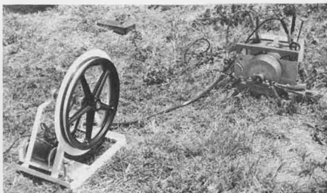
The Retriever may be used with other winches; it adds no noticeable drag to launch; high weeds need to be removed in front of Retriever.
