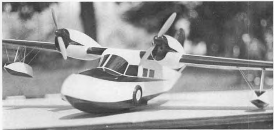
Jerry Holcomb's Grumman Widgeon model weighs only 32 ounces with a six-cell battery pack. All sheet construction is used. Astro 035s do the job of motivating with help from 5.25-4 props.
