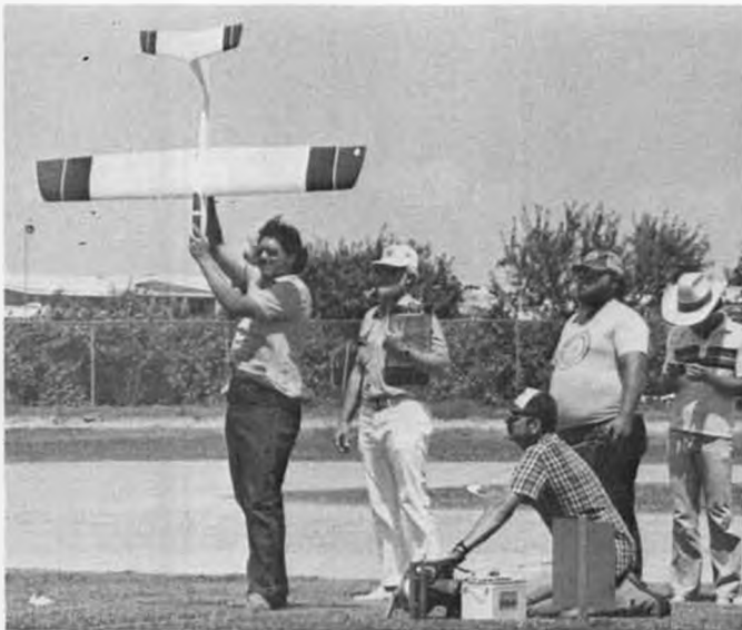
Robert Regalado IDs Marion Crowder's Interceptor prior to unlimited distance task. E-193 section with higher camber mod. F/A/C-R/E.
