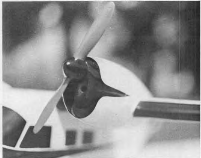
Jerry Holcomb molded these perfect fiberglass cowls for his electric Widgeon. Jerry also builds full-size aircraft.
