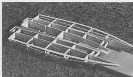
Hotshot IV framework features eggcrate construction. Use building fixture for straightness.
