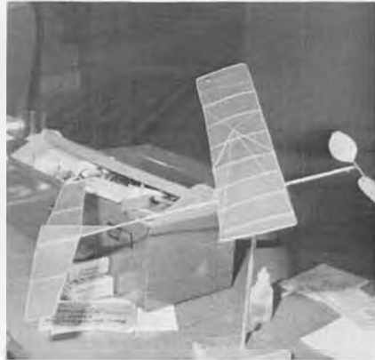
EZB rules say wood structure only. Richard Obarski complies fully with this model which uses fine balsa strips for "wires."
