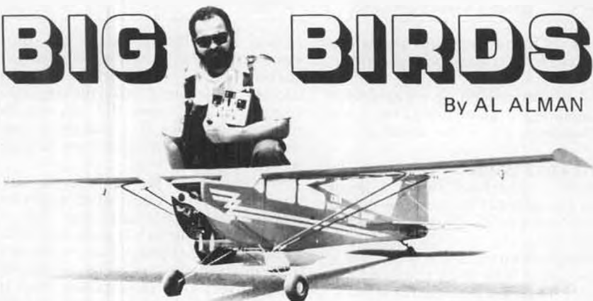
Roland Spicer's record setting Bellanca Skyrocket, built along with a sister ship in five months. Has a built-in nine gallon tank, although she took off with only 6-1/4 gallons. After the 454 mile flight, the Bellanca had a little over a gallon left. Roland has plans available.
