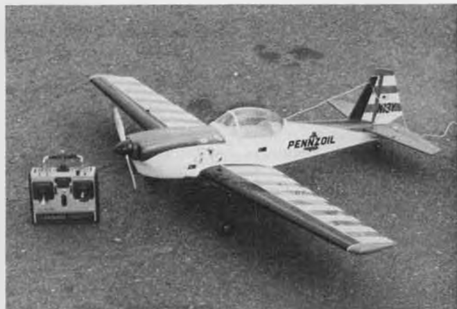
You can expect pattern performance from converted pattern planes when you use the Astro Cobalt 40 on 16, 1.2-amp Ni-Cd cells.
