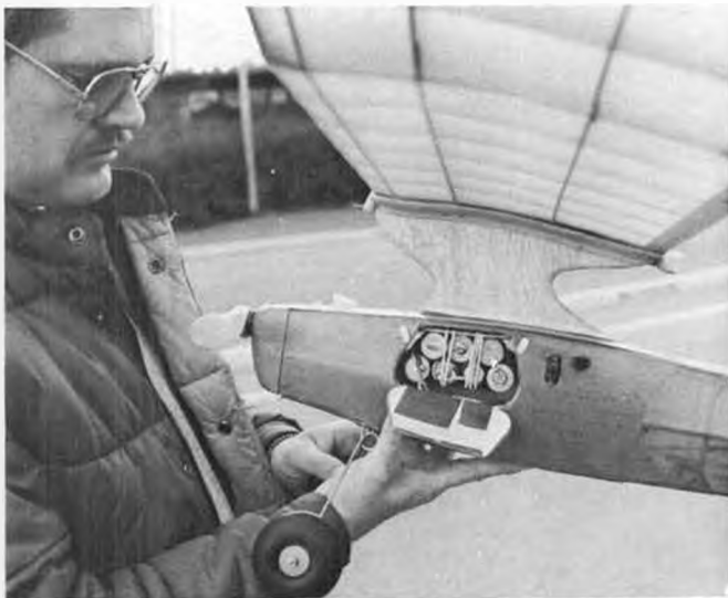
Leonard Bedford pops the cover from the side-mounted flight pack of his Leisure Playboy. Note 360-bend in LG: keeps LG from bending.
