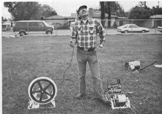
Admittedly posed shot of Howard Doering shows how you would operate Retriever hand switch and Pow'rtow foot brake in retrieve.
