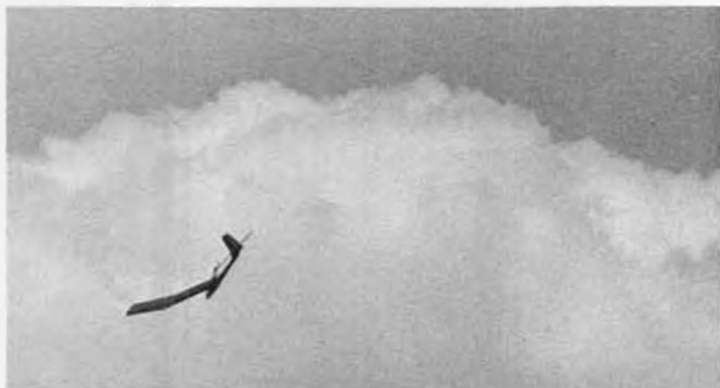
Winch victim. Thick winged aircraft had glue joint failure at joiner blade. Also, joiner ended abruptly, causing stress-riser.
