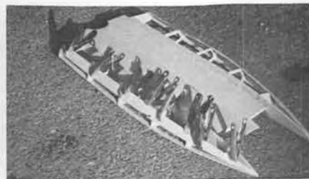
Clamps are useful to hold sponson sides in place while you work.
