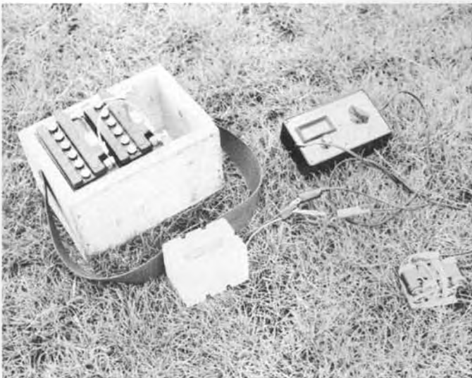
Leonard charges his flight packs from two motorcycle batteries which are kept in a wooden box to prevent acid spills. Leisure charger.
