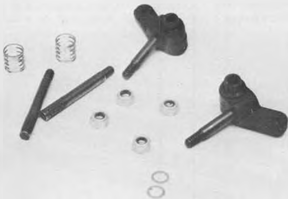
Delta's latest update kit for the Super Phaser. The Delta steering blocks feature improved wear characteristics. Threaded axles: 4-40.
