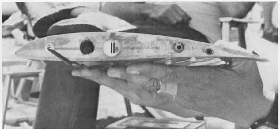
Brian Chan's Heavy Solution used a molded fiberglass skinned wing with E-214 section. Front hole is for aileron leads, next hole is ballast tube, double-blade steel joiners, pin, F torque tube.
