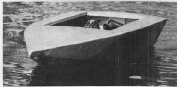
LEFT: A head-on shot of the Hurricane shows the deep V of the hull.
