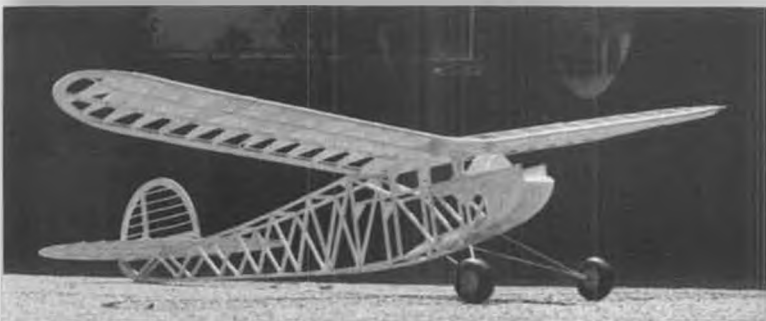
All framed up and ready for covering (well, almost!), the Powerhouse is a model builder's delight. Look at all them STICKS!
