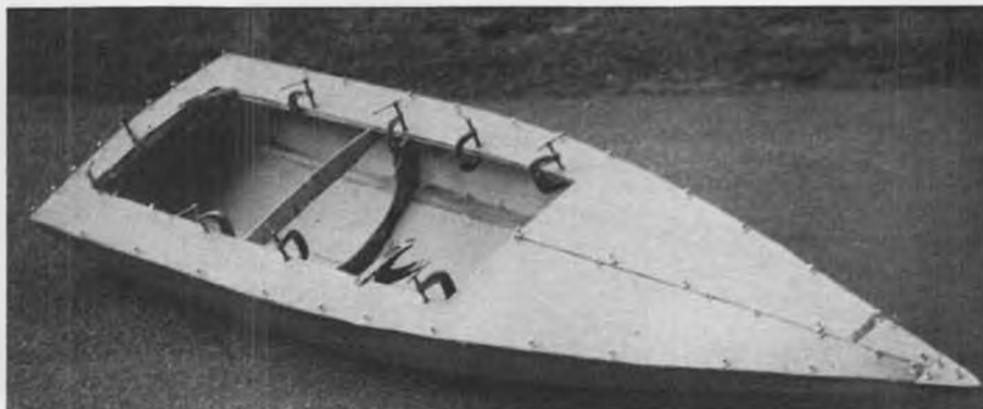
Nearing completion: map tacks and clamps hold deck sheeting in place while epoxy dries.
