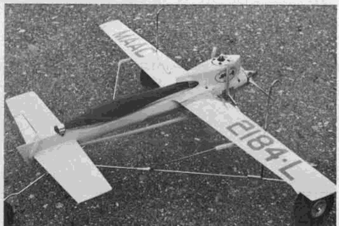
Chris Sackett sends this photo of his Class A Pink Lady (his own design). Features long fuselage & stab for stability, liftoff dolly.
