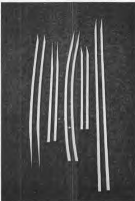
Preshaped fuselage sticks are cut from sheet stock. Grain is straight, pieces are curved.
