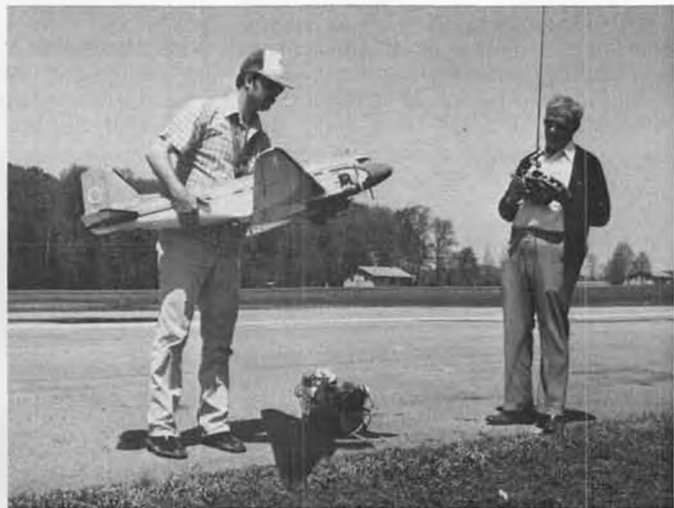
Bill Miller and helper demonstrate the 20-second cycling of the retracts in Bill's EAA DC-3 for the judges. Made from a Royal kit, the model weighs 11 lbs, has two OS .40s. Took 2nd in Sportsman D-2.
