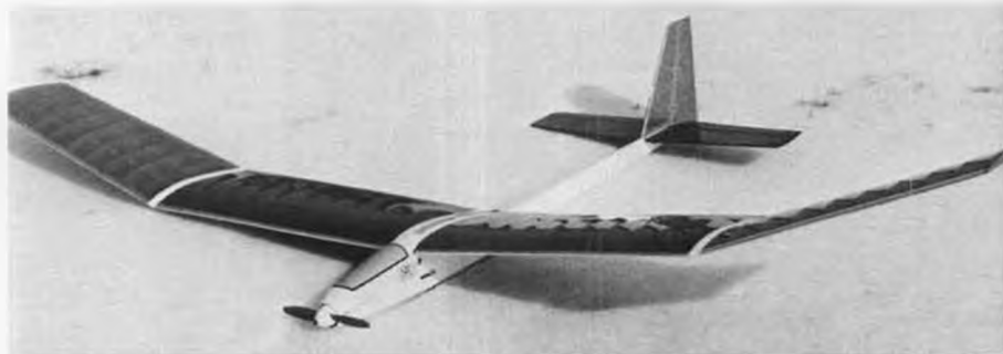
A close-up of Art's model. Note annular cooling scoop behind spinner cone. A prop stop device is used to save props and motor armatures. Art uses SR batteries.
