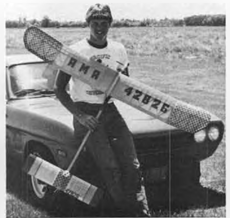
Author's son, Tom, poses with his FAI Class A model, the Zingo , designed by Tom Hutchinson and kitted by Campbell's Custom Kits. Rossi .15 on a Kraft mount. K&B finish over Japanese tissue (wing double-covered).
