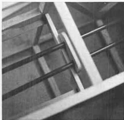
The plans do not show routing for pushrods as model was originally a F/F design.
