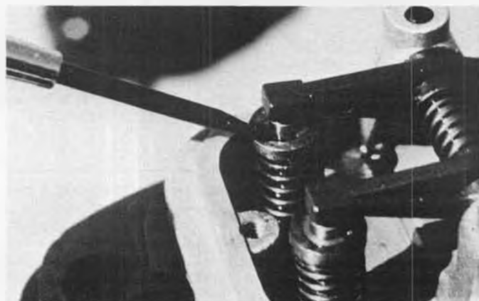
Photo 2. Beware of losing the valve stem keepers; they are held in place by spring pressure and can be dislodged if improperly handled. See text.
