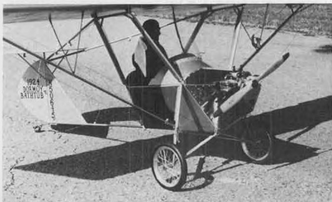
Although not entered or flown at the Mint Julep, this 1/3-scale Kimbrel Dormoy Bath tub from Model Builder plans was a real winner! Bill Brenchley, Marion, Illinois, powered this model with a Saito FA 80 four-cycle twin. Model weighs 13.5 lbs.
