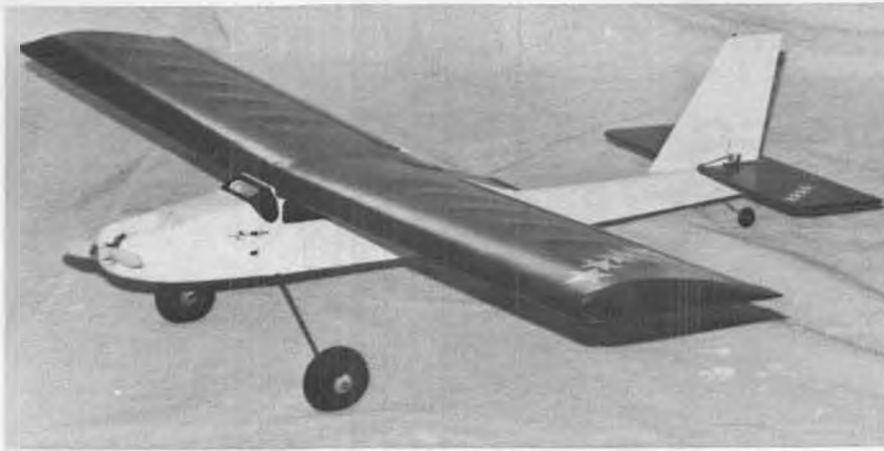
Northeast Aerodynamics Train-Air 20 converted to electric power by John Mountjoy.
