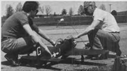
Hal Parenti and son, Gary, prepare Hal's Bearcat for flight. FAI model weighs 12 lbs, powered by Webra .61, silk & K&B covered.
