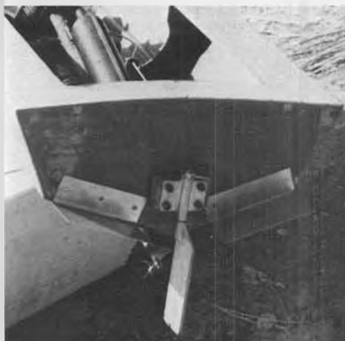
Here is a transom view of the model which shows rudder assembly and Octura X465 prop.
