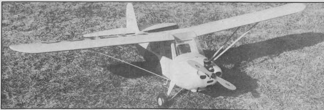
From the original construction article comes this photo of the Champion model. Engine doesn't have to be mounted vertically as shown.
