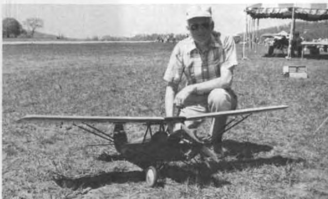
Don Brann poses with his "Silhouette Scale" Monoprep. Don finished sixth in his first scale contest, the Mint Julep, and proved that the AMA rules do work! (See text) An OS Max FS .60 four-cycle engine powers the eight-pound model.
