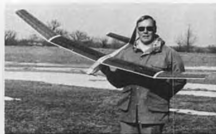
Noted Pylon racer, Art Arro, flies electrics year round to sharpen his flying skills. Model is a hybrid "Lady Electricus" design powered by an Astro Flight Super Ferrite 05 motor. 36 oz.
