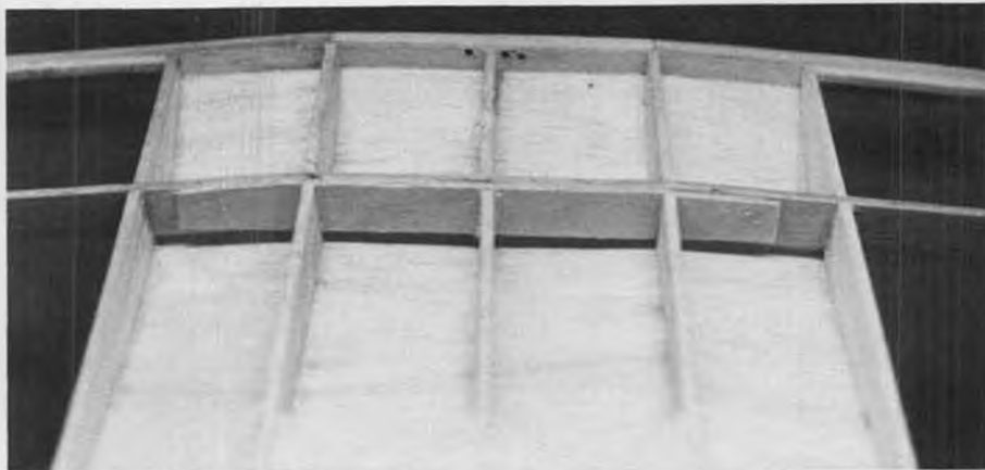
Five ribs have 1/16 of an inch of material removed from the upper surface to accommodate the 1/16 sheathing (top surface only). The 1/32 ply dihedral braces are clearly visible.
