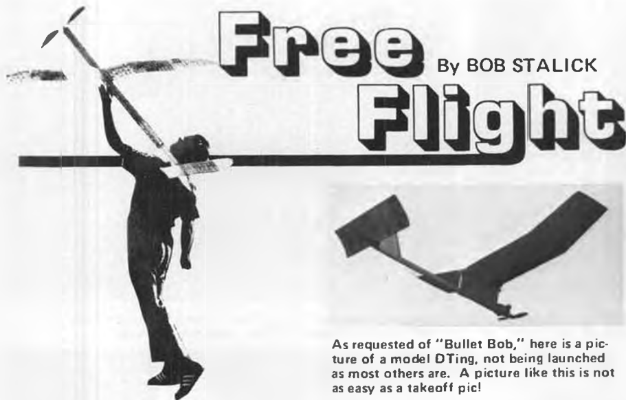
Author's son, Tom, poses with his FAI Class A model, the Zingo , designed by Tom Hutchinson and kitted by Campbell's Custom Kits. Rossi .15 on a Kraft mount. K&B finish over Japanese tissue (wing double-covered).
