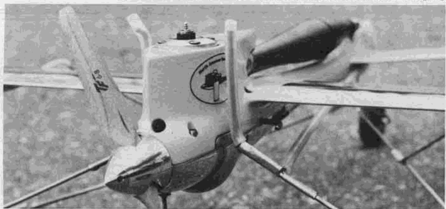
Chris Sackett's Class A Pink Lady viewed from the "business end." Power is by Super Tigre X-15, fed by suction uniflow tank. Quality workmanship is evident.
