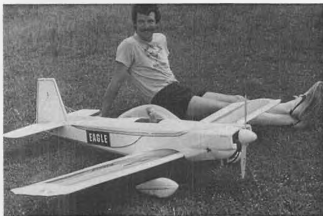
John Haskell, Shelby, North Carolina, reclines beside his nicely done Air Tech Eagle. The bird weighs 18 pounds with a modified Q-35. John likes the way an 18-8 prop works with the Q-35, and he likes the way Mickey Mouse and his Futaba 7-ch. pilot the model.
