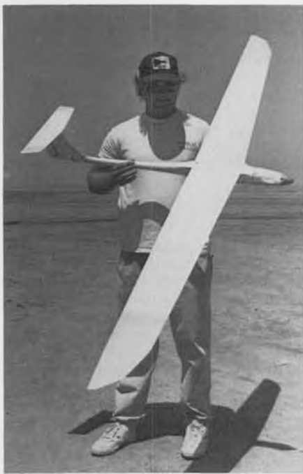
Astro 60 powered, 27-cell original by Jerry Bridgeman is a real hot rod. It was the lightest of the F3E models at the Astro Champs, has a very fast and very steep climb. Jerry also put on quite an aerobatics show with it after the contest.
