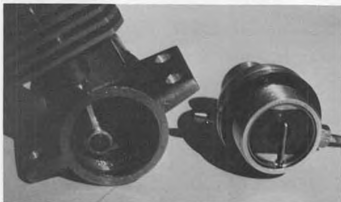
With the backplates removed, you can see that the engine on the left makes use of a reed intake valve similar to those used on small Cox engines, while the one on the right features the unique drum valve favored by East European speed enthusiasts. The drum (shown removed from the backplate) adds complexity and weight but allows large fuel/air openings that would seriously weaken a regular crankshaft.
