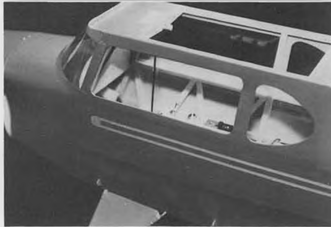
On the full-size Porterfield, the rear half of the left side window is openable; Bob left this part open for a cooling air exit and for access to the switches and charge plug.
