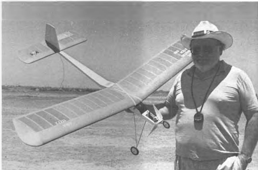
Gary Westland's Astro 15 powered Schmaedlg Flying Stick is an easy Old Timer to scratch build and a good flier to boot. Original was 84 inch span, but Gary scaled it down to 630 square inches.
