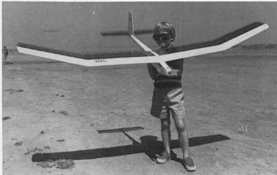
Fourth place in 7-Cell went to Jim Skinner and his red hot all-balsa original. Model uses an Astro 05 with a specially modified oversize gearbox.
