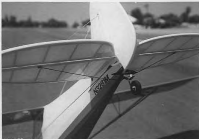
Wire bracing on the tail surfaces is scale and should not be omitted, as it adds immeasurable strength and rigidity.
