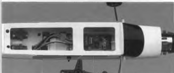
Hooked up with a pair of S133 micro servos, this system is perfect for electrics like our Hirobo/Futaba Professor.
