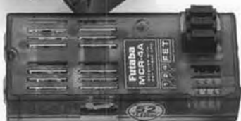
The MCR-4A four channel receiver/MOSFET speed control weighs just 1.5 oz. and can easily handle 280 to 540 size electric motors. 1.24" x 2.92" x 0.63"
