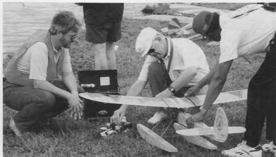
The "Higginsville Hornet," an original design by Bill Dickey, reflects his interest in Old Timers. Note that the floats are built-up stick construction with MonoKote covering. Power is a K&B .20 Sportster.
