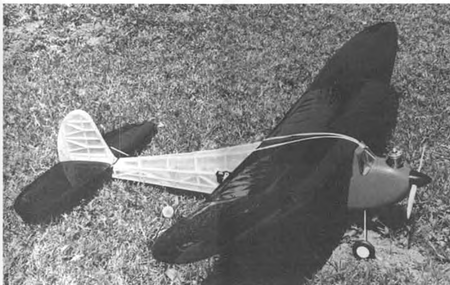
13. A real rarity is the Wigdor "Wasp," originally published in Aeromodeller . Col. Bowden influence is evident. This scaled-up copy uses an Enya four-stroke and was built by Albert Fisher of Australia.
