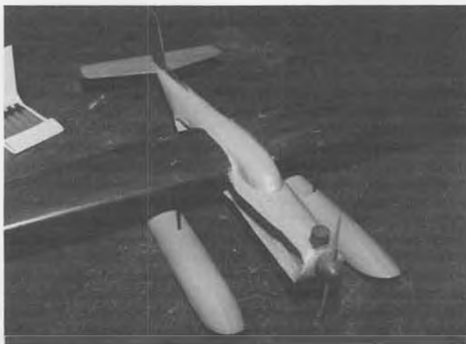
Our author's "Seatract," built back in 1975, was an experiment to determine the feasibility of twin retracting floats. The small scale model shown here, with the floats extended and retracted, was built first to develop the retract mechanism geometry. Discussion in text.
