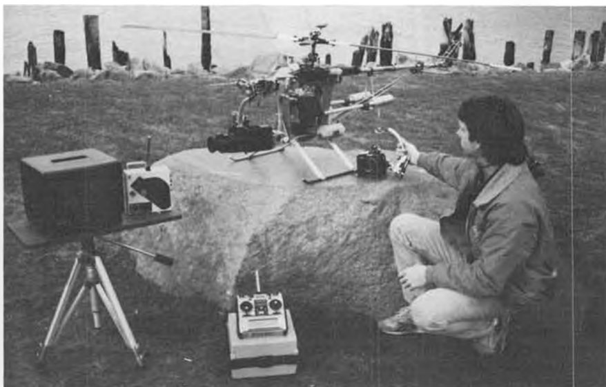
Eric Dustrude makes his living doing low-level aerial photography with this camera-carrying R/C chopper. It's a biggie with a 78-inch rotor diameter and Tartan Twin power.
