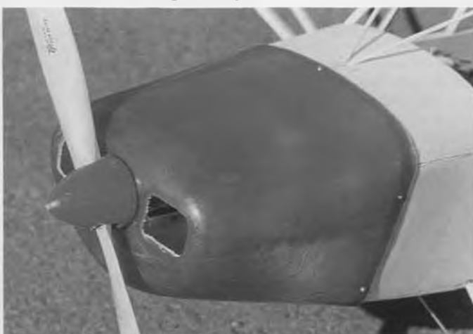
The Davey Systems kit includes parts for a built-up cowling, but our author chose to substitute a glass unit from Fiberglass Master (address in text).
