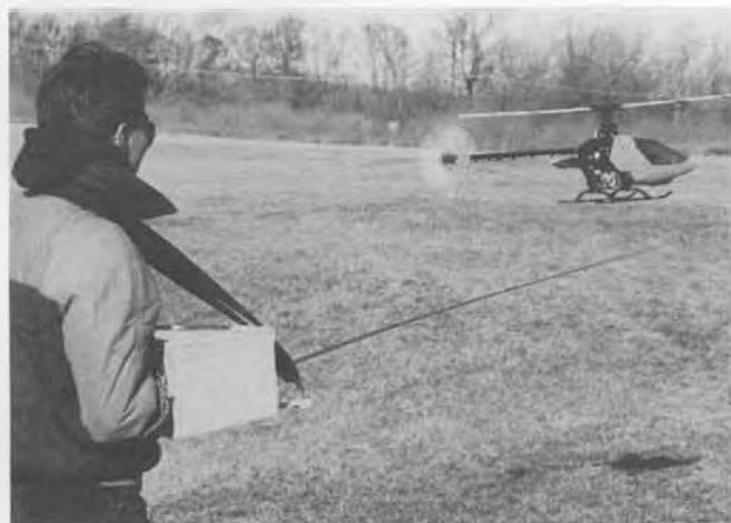
Here's a neat idea for chilly windy weather flying: a transmitter box made from thin plywood and supported by a neck strap. Use the photo as a guide to making your own, or buy one ready-made. Text has details.
