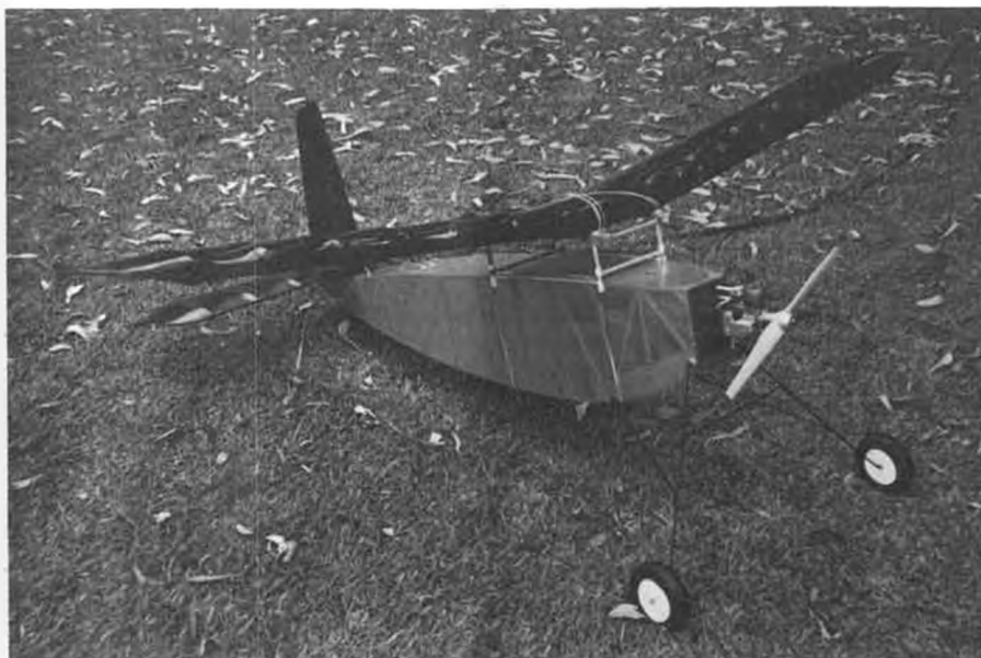
13. A real rarity is the Wigdor "Wasp," originally published in Aeromodeller . Col. Bowden influence is evident. This scaled-up copy uses an Enya four-stroke and was built by Albert Fisher of Australia.
