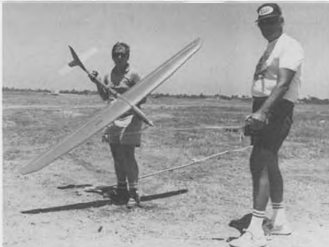
Steve Neu (left) and Keith Finkenbner flew identical "Drone" F3E electrics, based on a Freudenthaier fuselage. Astro 60 power.
