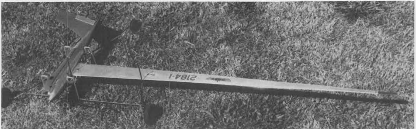
"Wildfire" is the name given to this wicked looking asymmetric FAI Speed model designed and built by Chris Sackett. He's got everything pared down to the bare minimum; ship has only half a wing, half a stab and half a prop!
