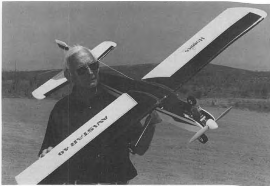
Left: Our columnist's flying buddy, Chuck Thompson, did the assembly work on the Avistar 40 for this month's review. The only notable recommendation offered is to add some striping or some other color trim to the bottom of the wing, as the all-white underside sometimes makes for marginal in-flight visibility.
