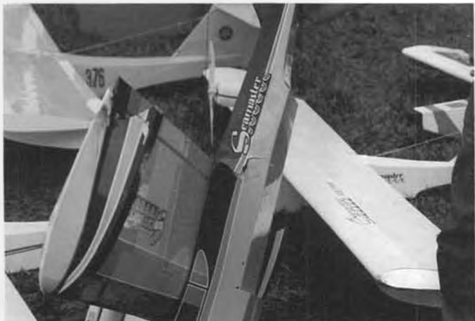
These two photos show the damage that resulted when two Seamasters, a 40 and 120, collided in flight. Both models landed safely and both were back in the air the next day, after a stop at the repair station and some attention from the Ackerman brothers.
