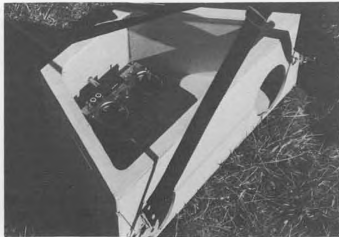
Here's a neat idea for chilly windy weather flying: a transmitter box made from thin plywood and supported by a neck strap. Use the photo as a guide to making your own, or buy one ready-made. Text has details.
