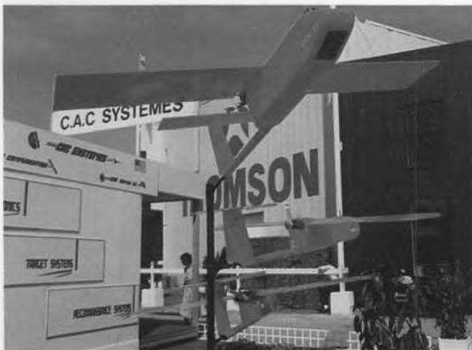
These “Aspic” R/C drones are produced by the French CAC company. Engines are 25-hp, two-cylinder, 275cc Limbachs, built in Germany.
