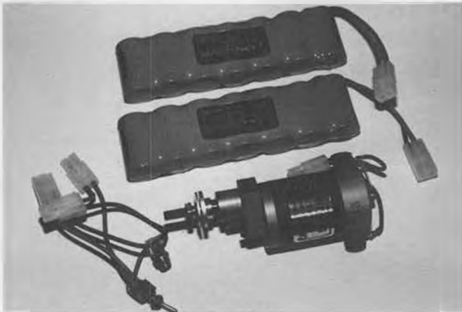
The complete Astro 25 Cobalt geared motor system. The wiring harness includes an on-off switch and charge connector, and couples the two 7-cell packs into a 14-cell flight battery.
