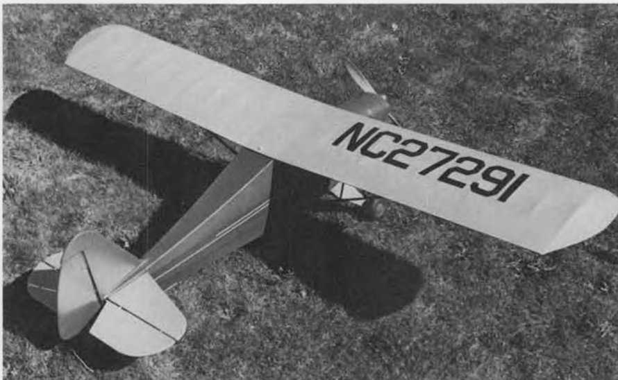
In this three-quarter rear view you can see the undercamber in the reworked prop, which started out as a 13x8 Top Flite Super M. This simple mod can yield a real boost in an electric's performance.
