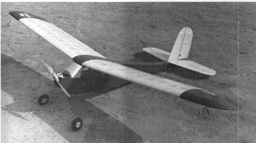
Above: Ray Westland's Turner Special didn't place in Unlimited O.T., but it sure was pretty in the air. Flew at the Champs with a geared Astro 15 Cobalt and fourteen 450 mAh cells, but has since been refitted with an Astro 25 and 800 mAh cells.
