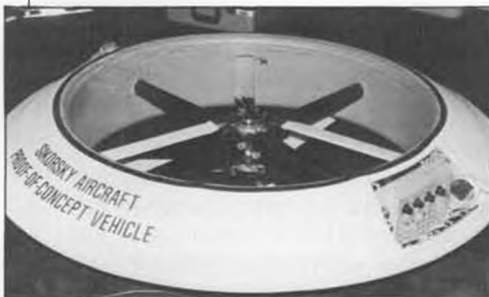
Sikorsky's proof-of-concept RC saucer. Uses two contra-rotating three-bladed main rotors to cancel the torque. The saucer is five-feet in diameter. Futaba radio used, and additional electronics shown in the clear window on the right.
