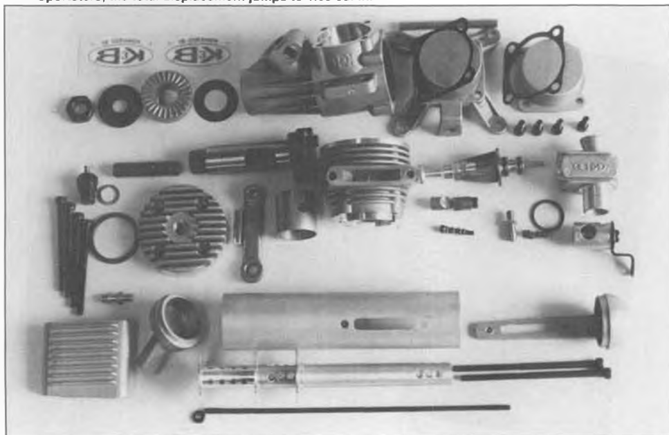
Parts breakdown of one of the K&B Sportster .20 engines used in the Mike radial. With the new .28 Sportsters, the total displacement jumps to 1.68 cu. in.
