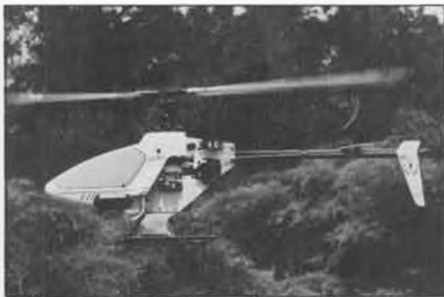
GMP's new 30-size Viper with metal Mini-Elite rotorhead. Available soon. It has forward facing engine, toothed belt-drive tail rotor, and interesting landing gear design.
