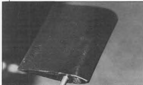
Miniature Aircraft's very new variable weighted paddle. The trailing edge portion is hollow, the leading edge has a hole where brass weights can be screwed into the paddles. Works quite well. Looks better than the original Japanese hollow paddles. The text has more details.
