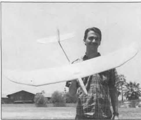
Competitive pod-and-boomer is the work of George Spitzer. The semi-elliptical wing planform and overall low parasitic drag made it do very well in the light lift at Riverside.
