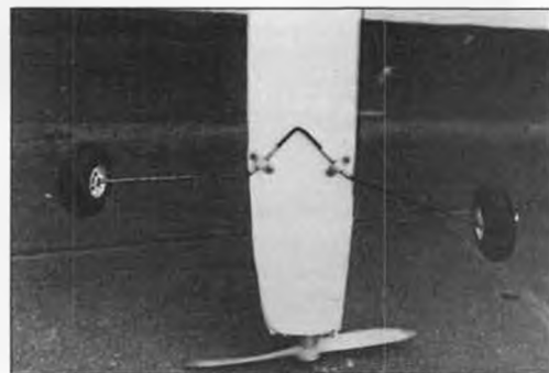
Mitch likes to mount his landing gears externally so as to avoid taking up valuable space inside the fuselage. The fuselage bottom is Lite Ply in this area.
