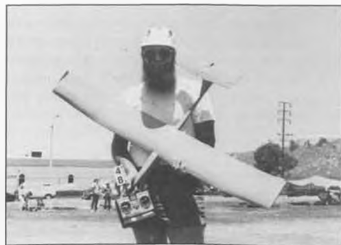
Rich Shelby took the Dick Odle "RO-8" plan and shot it at 75% to make a Class A model. Photo-reducing plans of two-meter ships has become a popular way to go in RCHLG.
