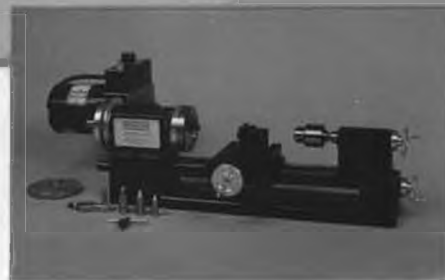
The Model 4000-A 3-inch lathe comes complete with everything you need to get started as a machinist. Included with the lathe is a faceplate, dog, collet set, 3-jaw chuck and a tailstock chuck and key.
