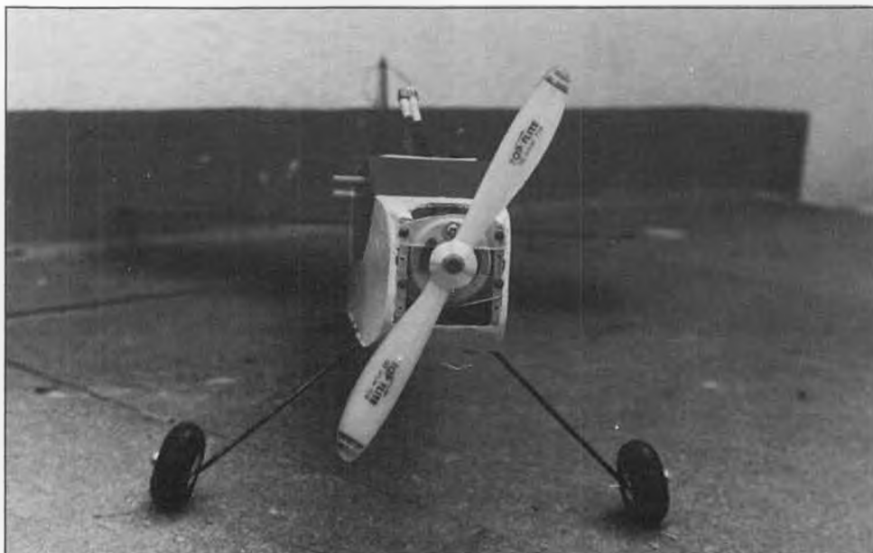
This head-on view of one of our columnist's model shows the type of motor mount he likes best. Not the prettiest, but what it lacks in esthetics it more than makes up in simplicity, light weight, ease of thrust adjustment, ample motor cooling... you get the idea.
