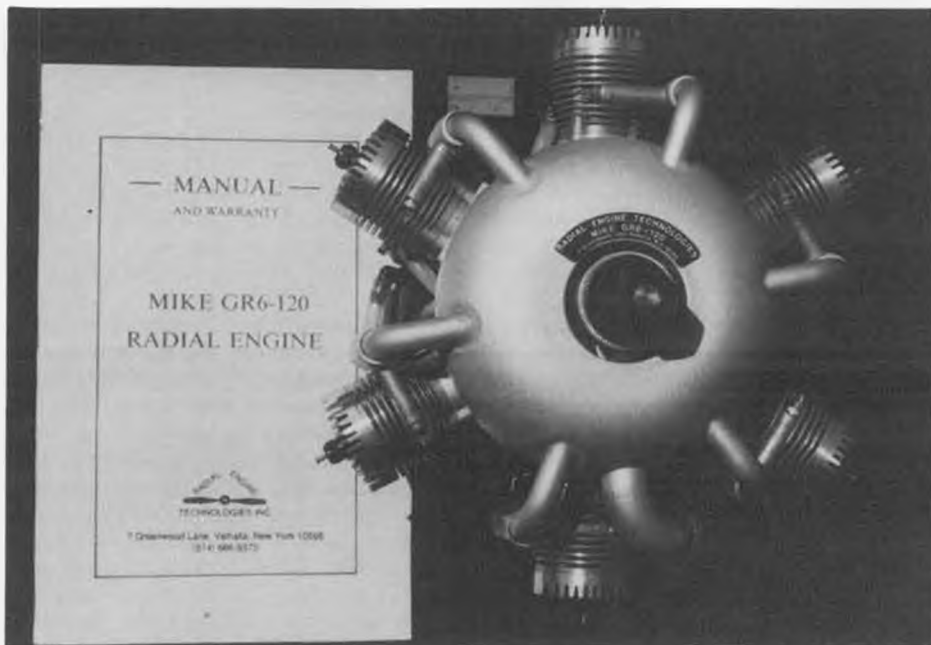
Looking for all the world like the old Curtiss Challenger, the Mike GR6-120 is probably the most successful two-stroke model radial engine ever produced. Turns an 18-inch prop at 8000 rpm and weighs under five pounds. (Below) The camera's flash almost stops the prop at a very reliable 1500 rpm idle with glow plug heat on. Stu strongly recommends the use of glow plug heat at anything below half throttle.
