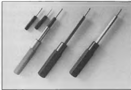
Century's tool-steel metric Allen wrenches. The one on the left has interchangeable size tips. These tips are guaranteed not to round or break. The ones on the right have fixed tips. Slightly over $10 a piece.
