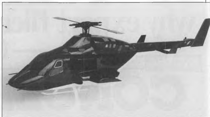
A pre-painted black Airwolf fuselage for all the 30-size helicopters. The bottom needs to be painted white by the builder. The fuselage is molded from a flexible material similar to Kyosho's Concept canopy and fuselage.
