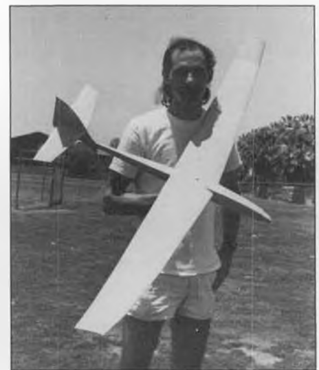
An unidentified modeler (a victim of our columnist's lost notes) with a really nice looking RCHLG. It sports a Jack Chambers airfoil similar to that on Dick Vader's "Skywalker," two polyhedral breaks per wing half, plus dihedral in the center section. Planes that look this right usually are right.
