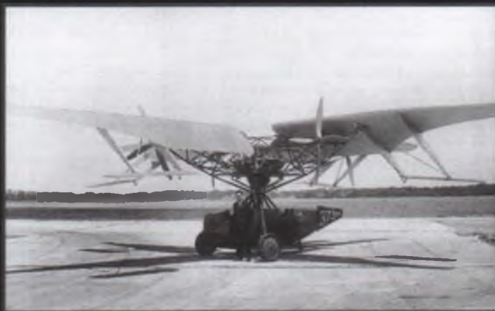
■ LEFT: Side view of Berliner's biplane. Rotary engine in the nose drove the two outboard rotors via shafts running through the lower wings. Note the highly undercambered airfoils used on both the top and bottom wings. ■ RIGHT: The 1929 Curtiss-Bleeker never got off the ground but serves as an example of a machine that needs no tail rotor or other torque compensation. The four-bladed rotor is spun by the thrust from four propellers driven by a radial engine mounted vertically in the center. Who will be the first to do an RC model?
