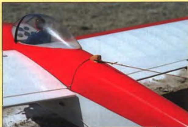
Here the big Ka-6C is being towed aloft. It's made from a molded fiberglass fuselage from France and scratch-built foam core wings. A full-size Ka-6CR (the "R" suffix indicates retractable gear) was present at the VSA meet to lend instant scale documentation!
