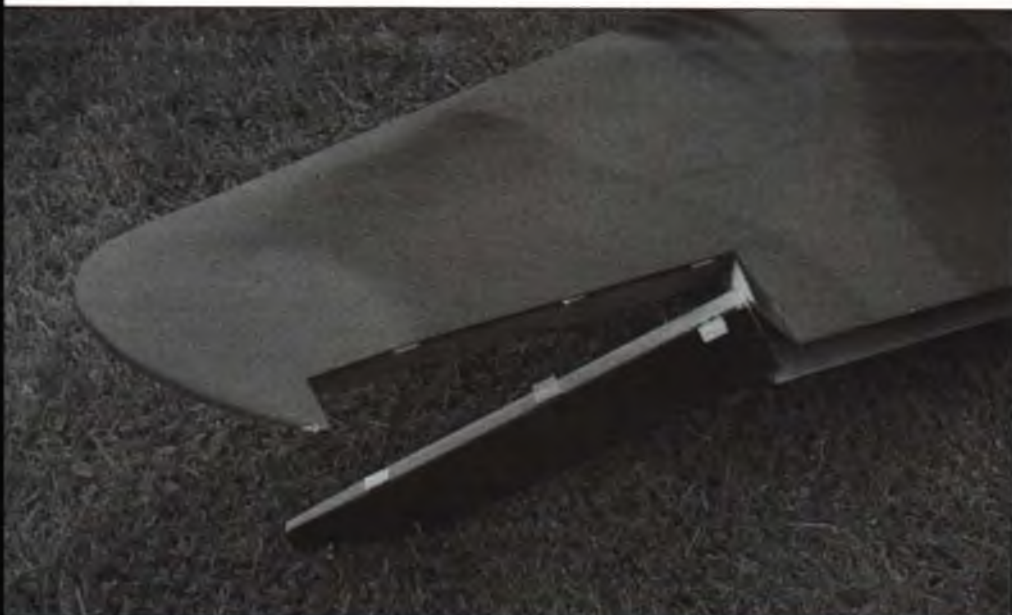
This is what can happen if you don't pin your flight control hinges. Hinges appear to have pulled out cleanly, taking almost no wood with them. Dave Grip exhibited great piloting skills getting his wounded P-40 back to Mother Earth.
