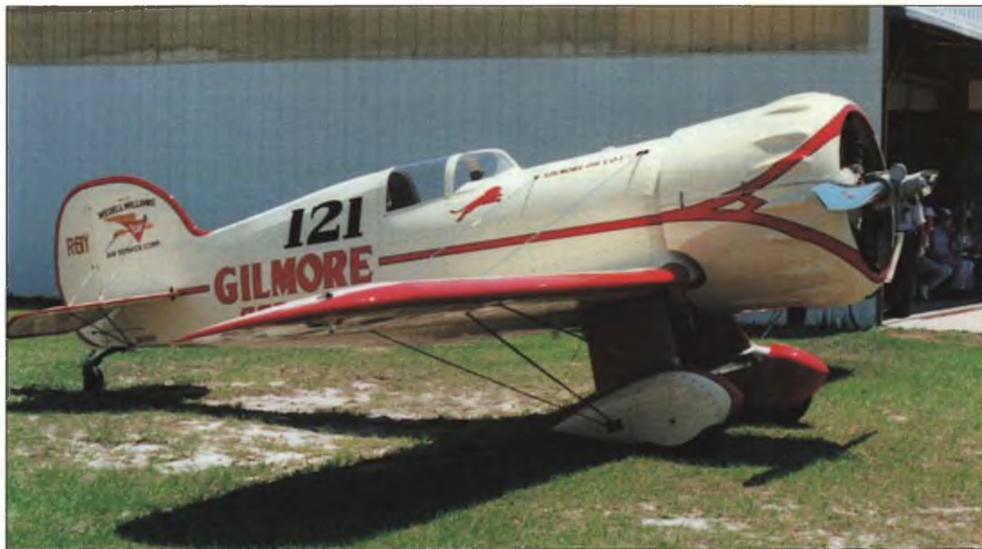
Jim Clenger's marvelous full-size reproduction of Roscoe Turner's Wedell-Williams racer features a slightly increased wingspan and increased airfoil thickness to provide more docile handling characteristics. Photo by Walt Grigg.
