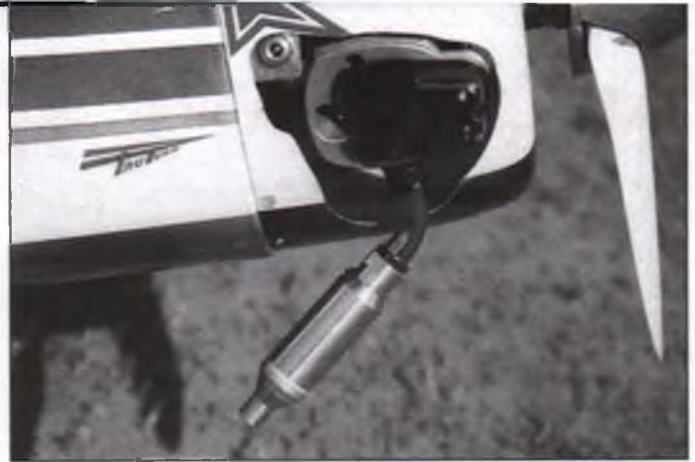
Muffler shown here is from an O.S. 1.20 Surpass and was custom installed on the YS 1.20 by Olaf Kitchin.
