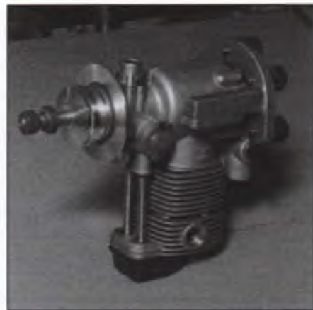
A YS 1.20 mounted to one of the new Super B/Mounts from CAN-AM Aero. Rick is using this mount in his new Python—see text. Photo by Bryan Boutrie.
