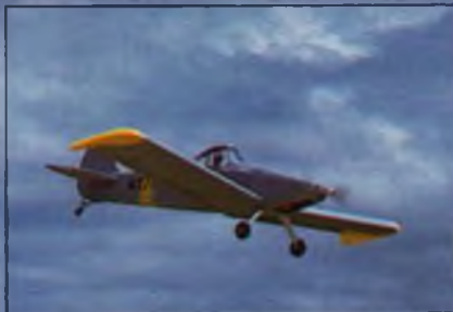
■ LEFT: Holcomb's Piper Pawnee in flight. Model is powered by a geared Astro 40 running on 21 cells, and features flaps that can be operated either independently or coupled with the elevator. ■ RIGHT: Our author was very impressed with the performance of Bernard Cawley's Ace Whiz40/Astro 40 combination. This airplane will be the subject of an electric conversion article in an upcoming issue of MB.
