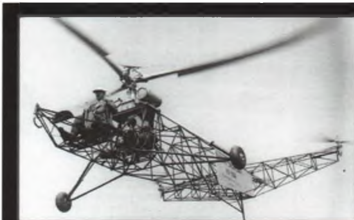
The great Igor Sikorsky at the controls of his VS-300, the first successful American helicopter, circa 1940. In this configuration the machine is fitted with two small vertical tail rotors in addition to the torque-compensating horizontal tail rotor; these three all rotors controlled the pitch, roll and yaw axes. The two additional tail rotors were eventually discarded.
