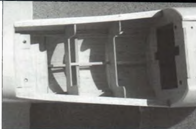
The huge interior of the fuselage will accept any radio installation. Note the neatness of the all-wood construction.
