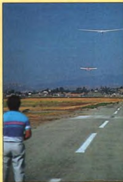
Here the big Ka-6C is being towed aloft. It's made from a molded fiberglass fuselage from France and scratch-built foam core wings. A full-size Ka-6CR (the "R" suffix indicates retractable gear) was present at the VSA meet to lend instant scale documentation!
