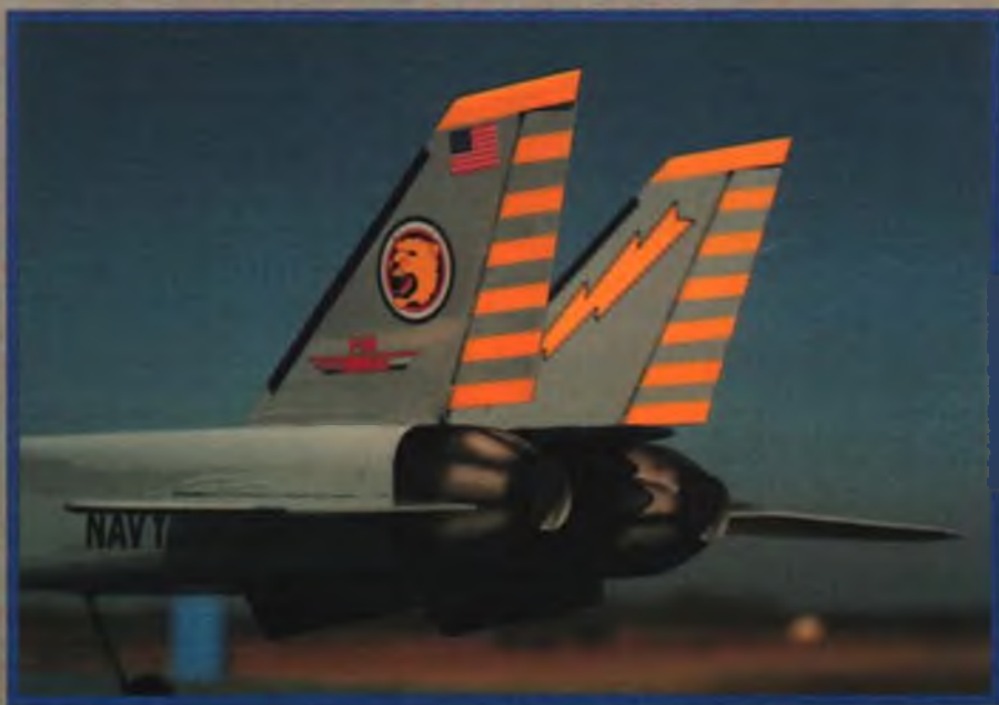
Molded ABS plastic exhaust nozzles were airbrushed with water-based acrylic paint and finished with clear enamel. Neat effect, huh?
