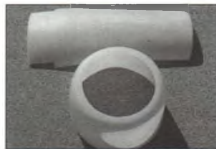
The Sukhoi's belly pan and cowl are non-gelcoated fiberglass and require painting; quality is excellent.
