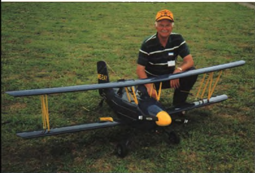
Don Belisle poses with his fine flying 2.5"-1' scale Grumman Turbo Ag-Cat. The scratch-built model is powered by a Zenoah G-38, weighs 22 pounds and spans 90 inches. Model Builder has plans for a radial-engine version of this same aircraft, drawn to the same scale; it's plan #12781, $24 plus $6 S&H.
