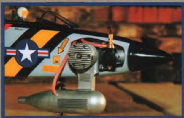
Close-up of the Irvine .61 ABC installation. Although at the bottom of the recommended engine size range, the author found it to be an excellent choice for the Tomcat—more than enough power to make the airplane perform as advertised. The extra-pointy spinner was designed by Great Planes specifically for this model.
