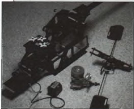
The Ninja composite sideframes took James three hours to assemble. The finished unit is stronger than the standard plastic frames and has higher torsional rigidity. The whole structure, including the servo tray, weighs only 15 ounces.
