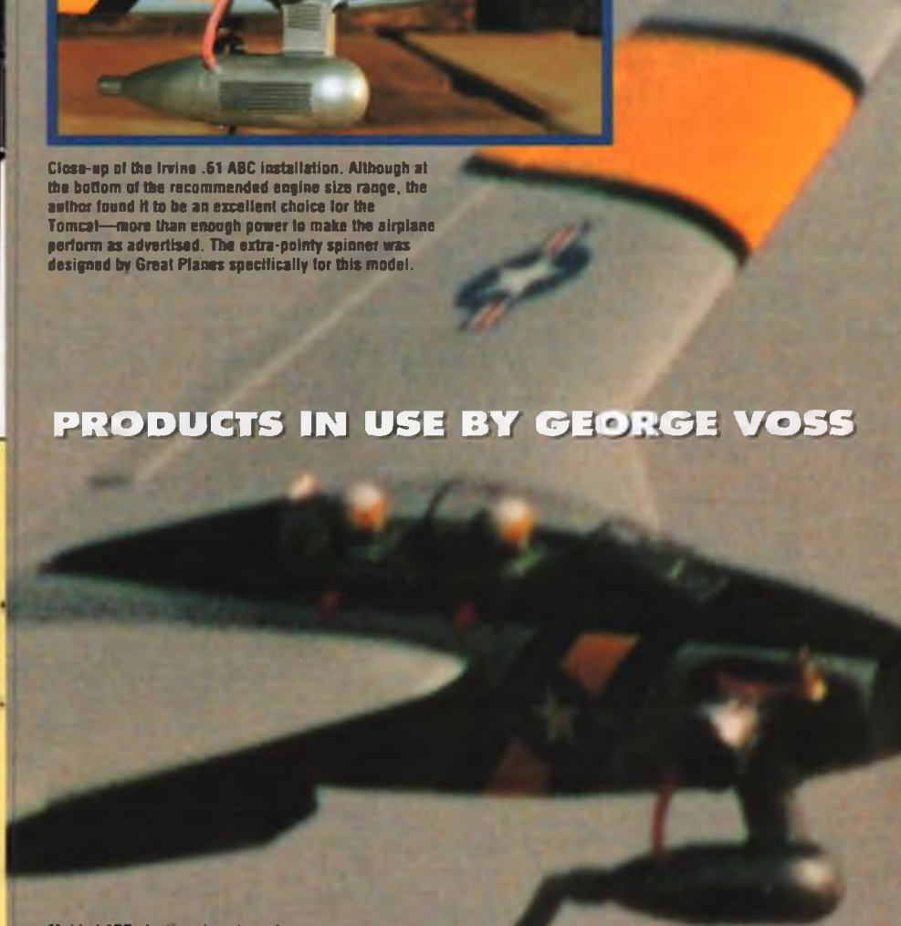
Molded ABS plastic exhaust nozzles were airbrushed with water-based acrylic paint and finished with clear enamel. Neat effect, huh?
