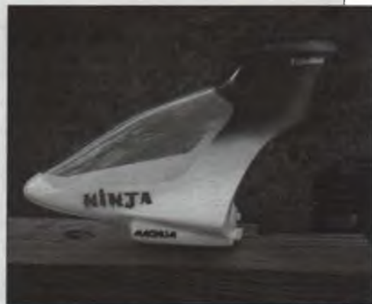
CHP's Ninja composite sideframe kit includes this sleek canopy (supplied unpainted). Note that the mast fairing extends higher than normal to smooth the airflow around the swashplate for reduced drag.
