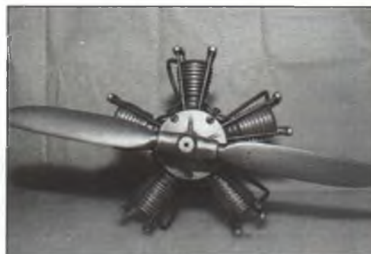
Nicely made 1930s vintage five-cylinder compressed-air engine by the late Levere "Cookie" Cook has a very realistic scale appearance. Photo by Remo Galeazzi.
