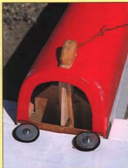
Close-up of the Stinger with the cockpit section removed reveals more details of the towing setup. Main post is cut from maple, and there are four beety hard balsa compression beams that attach to the top of the post just under the ABS turtledeck and tie in to the basic wood box fuselage farther aft. Towline is captured by a wire that protrudes vertically through a horizontal slot in the maple post; towline can be released in an emergency when a servo pulls the wire down and opens the slot.
