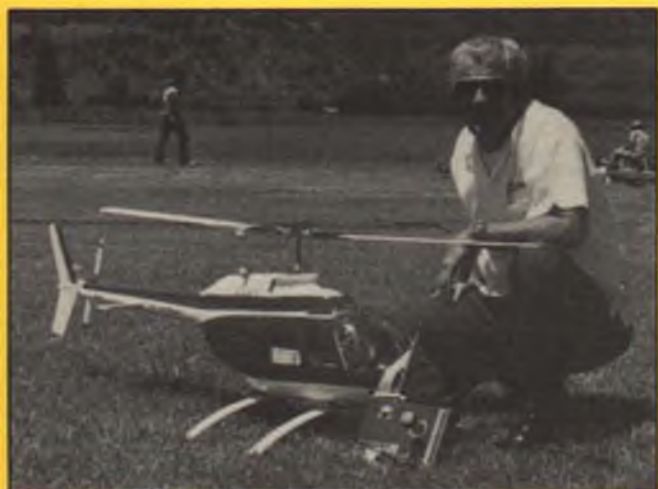
LEFT: Model Builder's first Chopper Chatter columnist, John Tucher, with his Kavan Jet Ranger, a popular model during the '70s. Introduced in 1973, the Jet Ranger was the first kit chopper to have collective pitch. RIGHT: Dieter Schluter's first heli kit was the Heli-Baby, a fixed-pitch machine for .60-size engines. Featured a Bell-Hiller rotor head design and a heli-drive tail rotor. It was on one of these models that MB columnist James Wang learned to fly in 1976.
