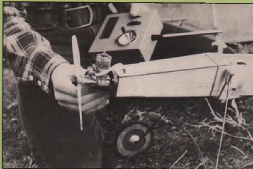
How's this for an easy-to-service engine installation? O.S. .10 is bolted to a Kraft-Hayes mount.
