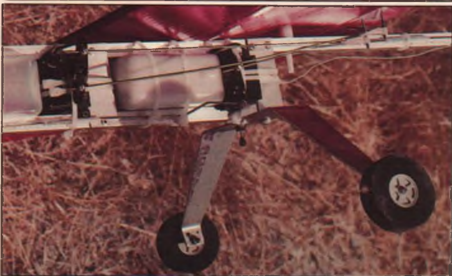
Right and left side views of the nose showing the simple engine and radio installation. The four standard-size servos are mounted out in the open, between the upper and lower fuselage members, and are held in place with tie-wraps. The receiver and radio battery are contained within the modified fuel tank strapped in place just under the wing leading edge.
