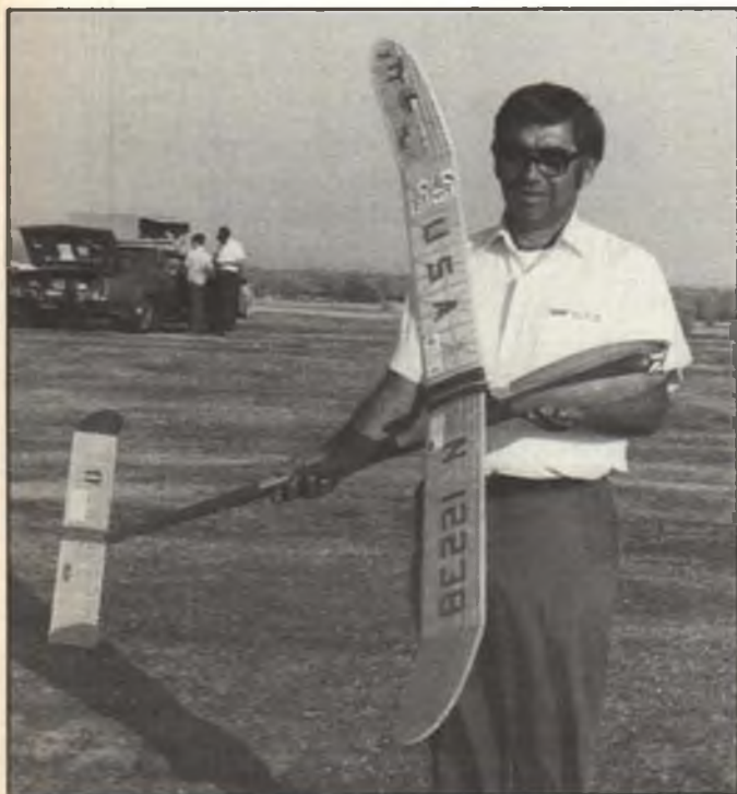
Legendary Wakefield flier Bob White with the seventh in his ongoing series of twin-fin, rolled tube fuselage, high-nylon models; this one placed 3rd at the 1971 World Champs in Finland and was published as a construction feature in the June 1972 Model Builder . Our columnist picked Bob's later No. 22 Wakefield, winner of the 1987 World Champs and very similar in appearance to the one pictured, as his top choice for the F1B category.
