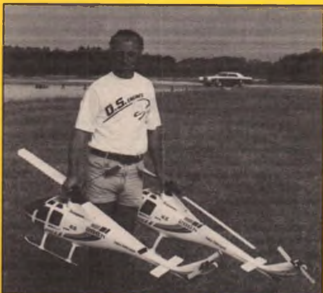
Mr. Ewald Helm of Germany with two of his own design Lockheed 286H scale models. Helm pioneered the leading axle main rotor head, and used semi-monocoque fuselages on his helicopters to keep weight down.
