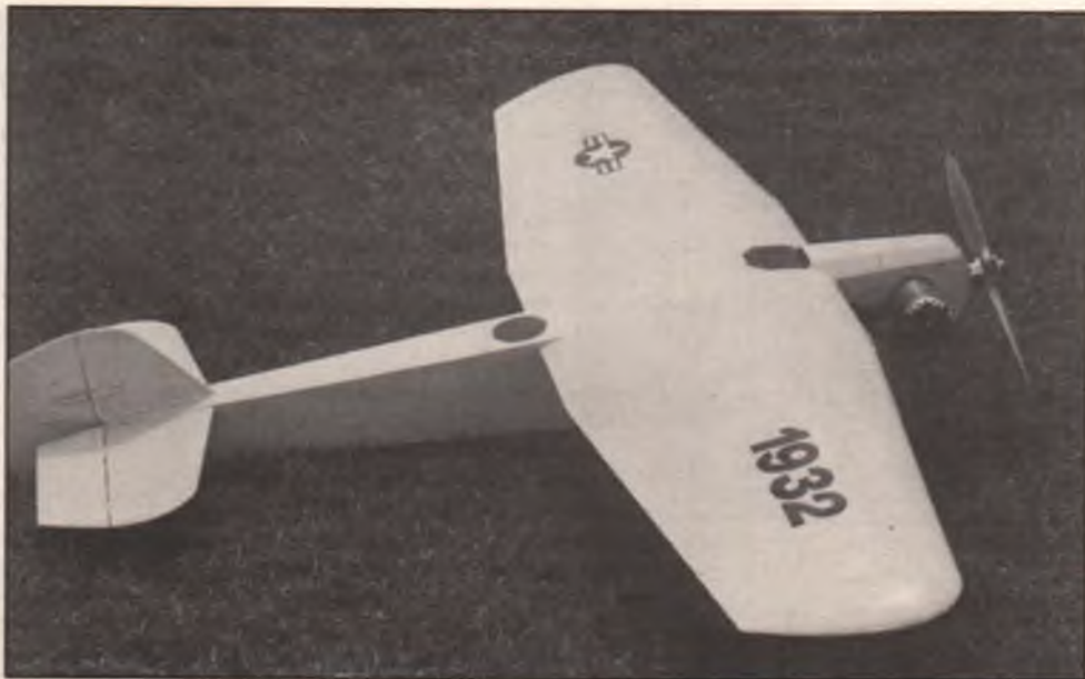
The Martin MO-1 has become by far the most popular carrier plane due to its capability for prop-hanging. This is Pete Mazur's Class II model.
