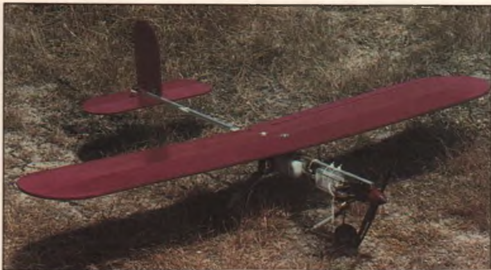
By far not the prettiest model on the market, but strong and easy to work on — perfect for beginners. Assembly is all done with bolts and nylon tie-wraps, no glue required. It took our author just four hours to get his model completely assembled and ready to fly, including radio and engine installation.
