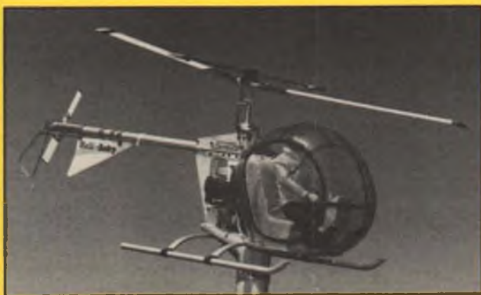
LEFT: Model Builder's first Chopper Chatter columnist, John Tucher, with his Kavan Jet Ranger, a popular model during the '70s. Introduced in 1973, the Jet Ranger was the first kit chopper to have collective pitch. RIGHT: Dieter Schluter's first heli kit was the Heli-Baby, a fixed-pitch machine for .60-size engines. Featured a Bell-Hiller rotor head design and a heli-drive tail rotor. It was on one of these models that MB columnist James Wang learned to fly in 1976.
