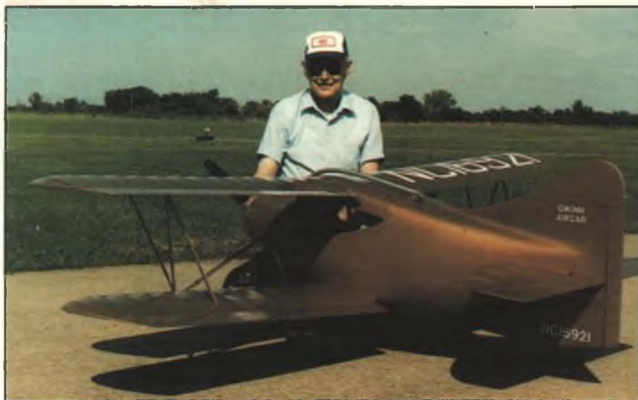
Master scale model designer Claude McCullough, of Iowa, behind his wonderfully crafted Gwinn Aircar Model II. The 32-pound 1/3-scale RC machine is powered by an O.S. 320 Pegasus four-stroke, four-cylinder engine.
