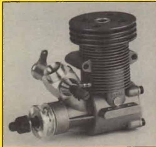
James finds the new Austrian-made Webra .33H puts out even more power than the Webra Red-head .32H. Features a Dykes ringed piston (easier to crank over than an ABC or AAC engine), Webra's well-liked TNII carb and a large heat-sink head.
