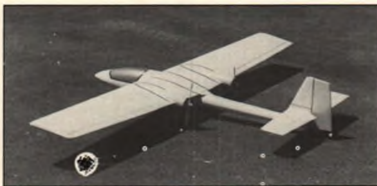
The Electro 225 looks as exotic today as when Astro first kitted it in the late '70s. Featured a fiberglass fuselage, built-up wood wing and tail, a single main wheel with wingtip skids, and two Astro 25s mounted as pushers on the wing.
