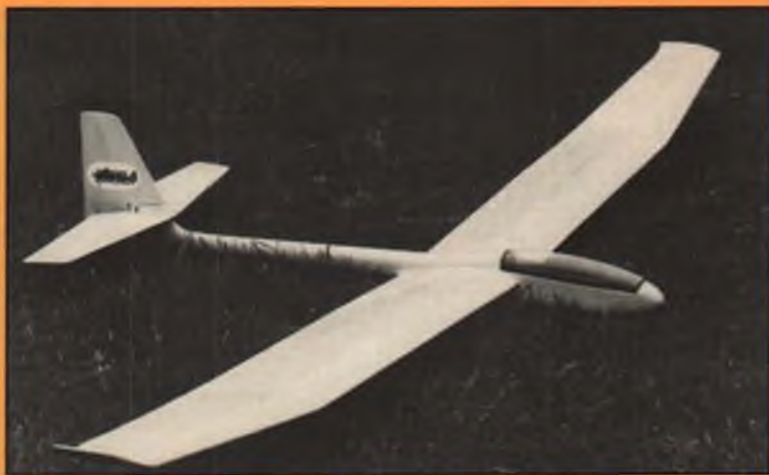
■ LEFT: Craft-Air was a major player in the RC sailplane market in the early '70s. The Drifter was a 72-inch glider designed to compete with the popular Pierce Aero and others in the same size bracket. Craft-Air's sailplanes were characterized by having the outer polyhedral break at 2/5 of a half-span from center. ■ RIGHT: Back in the mid-'70s the standard class ship to beat was the Airtronics Aquila. Early kits had a wood fuselage, later ones were glass. This particular example was built by former MB soaring columnist Taylor Collins for a product review article.
