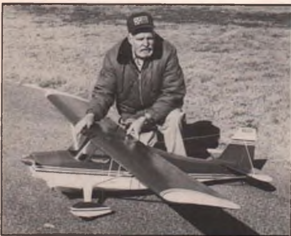
Another popular series of early Giant Scale kits was produced by Bud Nosen; the line included a 1/4-scale J-3 Cub, Citabria (pictured here with builder Dale Bossant, his first Big Bird), Aeronca Champ, Goro Sport biplane and several others. These were relative lightweights that came in at 9-10 pounds and flew well on .80 glow engines.
