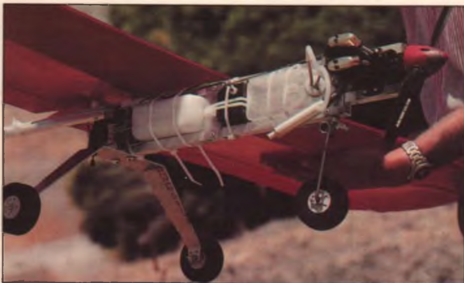
By far not the prettiest model on the market, but strong and easy to work on — perfect for beginners. Assembly is all done with bolts and nylon tie-wraps, no glue required. It took our author just four hours to get his model completely assembled and ready to fly, including radio and engine installation.
