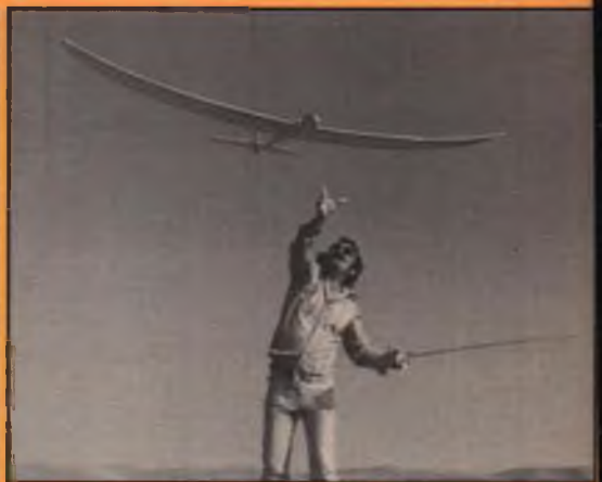
◼ LEFT: Bob Dodgson was a real pioneer of RC sailplane design and is still going strong today. The Dodgson Designe Todd, released in 1973, was one of the first sailplane kits with all-glass (Rapocore, actually), featured a molded fiberglass nose mated to a rolled balsa tailboom and could be built with either 78-1/2 or 100-1/2 inch wings. ◼ RIGHT: Hobie Alter's famous Hobie Hawk was introduced in 1974. Graceful elliptical dihedral and drooped nose made it stand out from all others. After Hobie stopped production, the Hawk design was purchased and produced by successive owners, including Bob Martin, Midwest and most lately, Ross Models.
