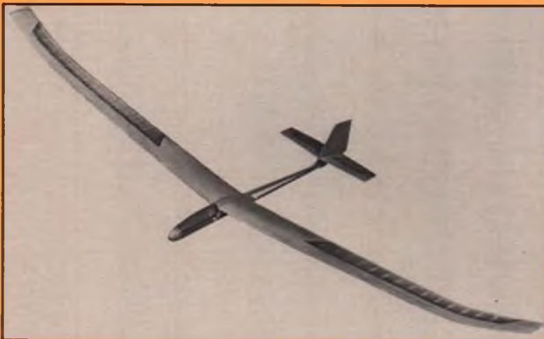
◼ JP Models had some high-performance sailplanes in the early to mid '70s, the largest of which was the 134-inch Javelin II pictured here. Came with a pre-painted rolled plywood fuselage with fiberglass nose and could be built with your choice of V-dihedral, polyhedral or elliptical tip dihedral.
