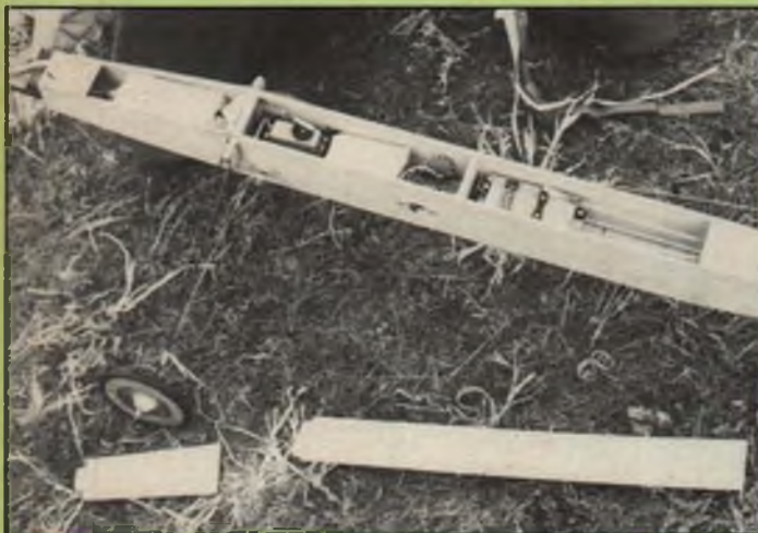
■ LEFT: Fuel tank and radio are likewise completely accessible. Photo shows the Kraft "brick" (remember those?) in one of the prototype Dragonflies. Any of today's inexpensive "standard" servos would be perfect for this ship. ■ RIGHT: Plans show a two-piece wing, joined in the center with music wire rods in brass tubes. Could just as easily be built in one piece if storage and transportation are not a problem.
