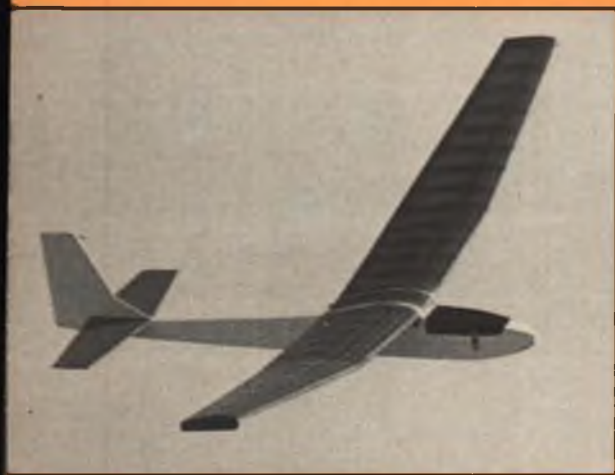
■ LEFT: Craft-Air was a major player in the RC sailplane market in the early '70s. The Drifter was a 72-inch glider designed to compete with the popular Pierce Aero and others in the same size bracket. Craft-Air's sailplanes were characterized by having the outer polyhedral break at 2/5 of a half-span from center. ■ RIGHT: Back in the mid-'70s the standard class ship to beat was the Airtronics Aquila. Early kits had a wood fuselage, later ones were glass. This particular example was built by former MB soaring columnist Taylor Collins for a product review article.
