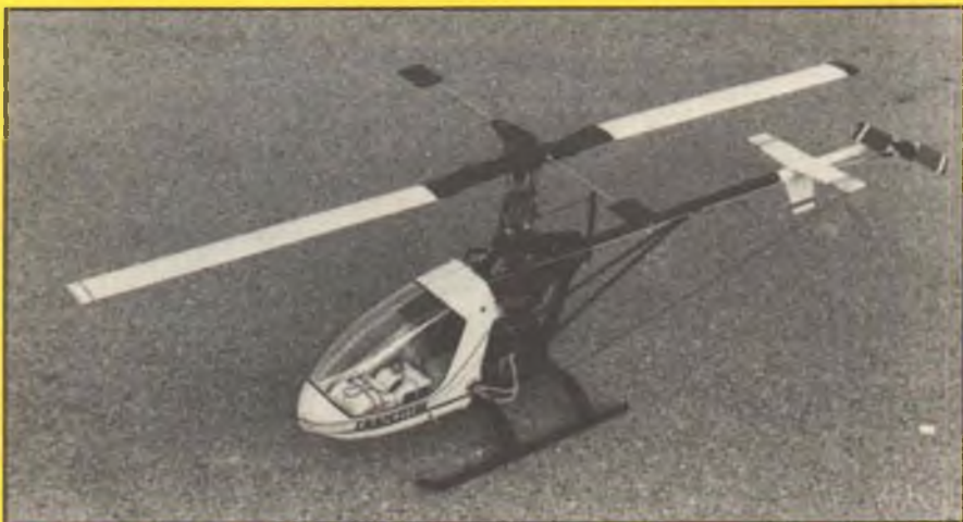
The .60-size GMP Competitor was the first of the really high-performance pod-and-boom aerobatic RC helis, winning almost every contest in the country during the early '80s.
