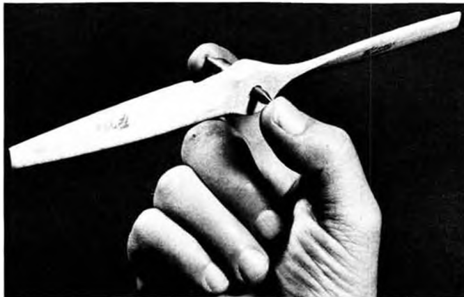
Don't squeeze da balancer! The less pressure, the more sensitive this prop balancer by Prather Products . . . also the less it will hurt!
