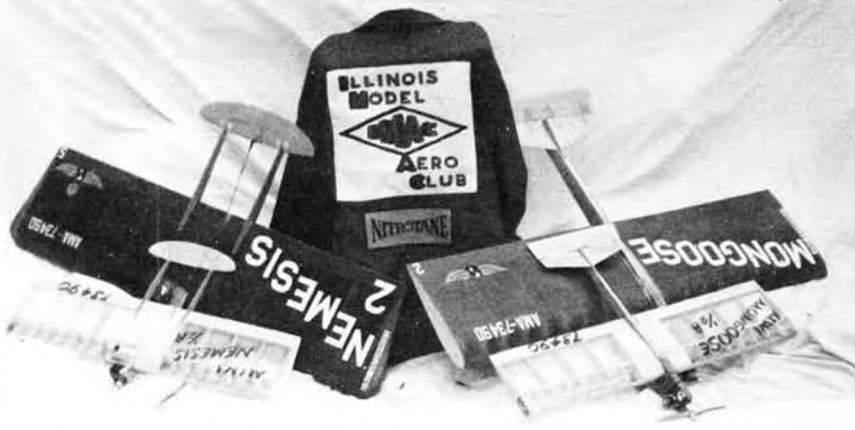
Steve Fauble goes for the 1/2A models in C/L. Here he has built 6/10 size versions of the Nemesis II and the Mongoose. Both fly very similar to the big ones.
