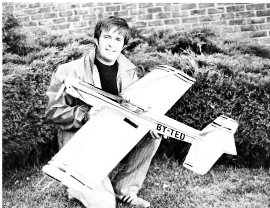
This Akrobat built by Ted Fancher . . . like it says on the fuselage! He's a member of the San Mateo .049'ers. Power is a Fox 35 with muffler. Weighs 51 ounces.
