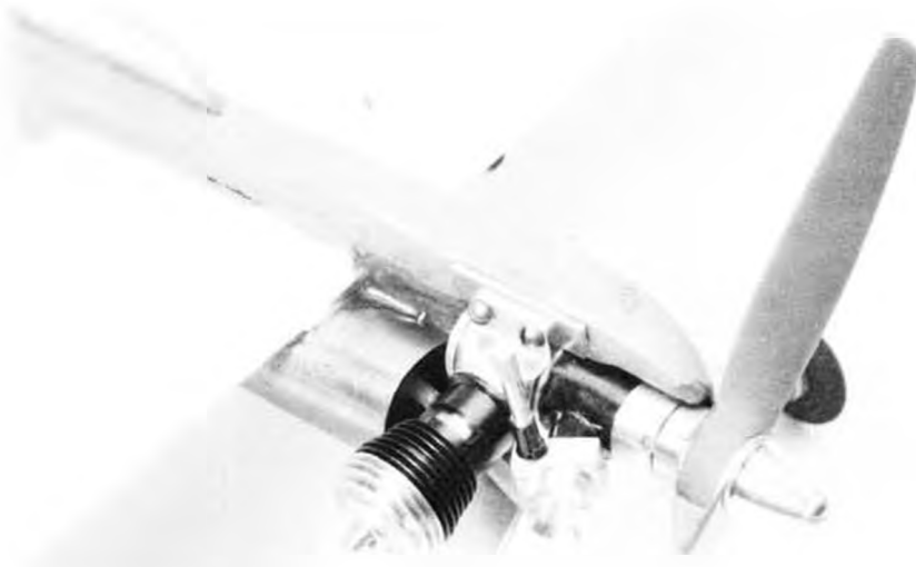
This 1/2A Proto (Profile) plane is equipped with pen bladder, Kirn-Kraft front needle valve and prop. The single blade prop (5.2" diameter) uses a one-piece brass counterweight.
