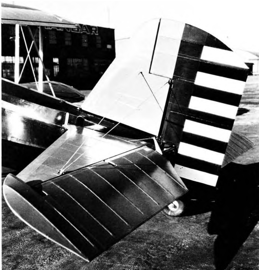
Tail surfaces of the O-38 and O-38A. The rudder chord on the B and C was 4 inches wider. The horizontal stabilizer was adjustable in flight from minus 3 to plus 4 degrees.
