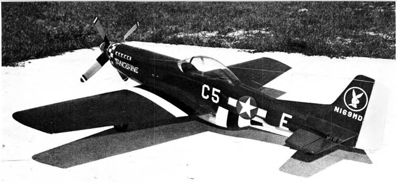
Soon-to-be-released stand-off scale R/C ship by Sig features the Kwik-Bilt style of construction; a 1/2 inch balsa profile/backbone is covered by two molded plastic half-shells. Foam wing cores and sheet tail surfaces back up the rapid completion theme of the kit. Of course, it's a P-51!
