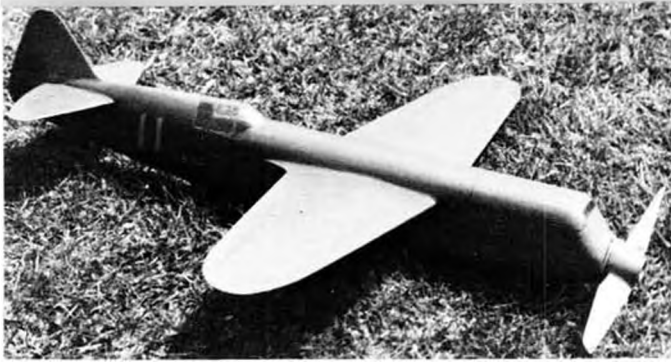
Mr. Smoothie, built by Granger Williams for the Scale Rubber Speed event. Fuselage carved and hollowed from a solid balsa block.
