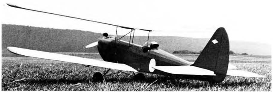
After some changes from initial "rollout," B.J. was fitted with a Fox .59; fuselage, fin, and rudder were painted with blue Hobbypoxy; and a Quadruplex radio on 6 meters was installed.
