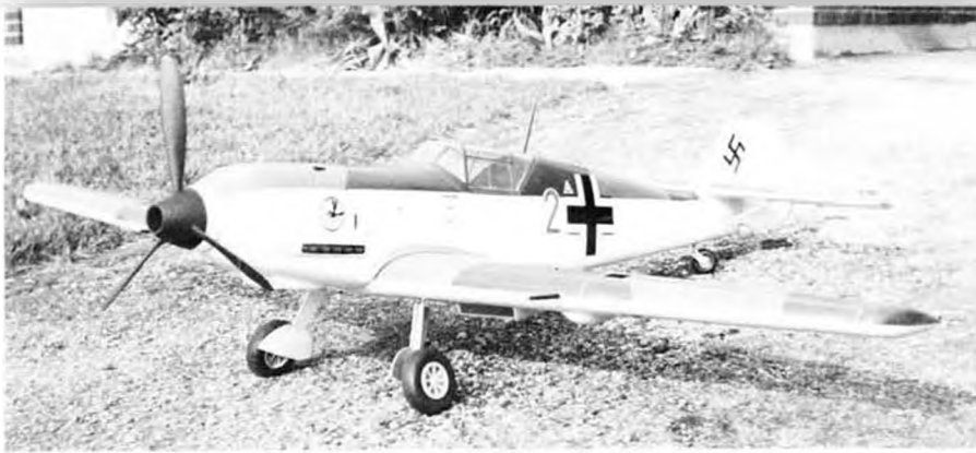
ME 109E built from Gas Model Products kit. Features molded fiberglass fuselage/fin. See text for further description.
