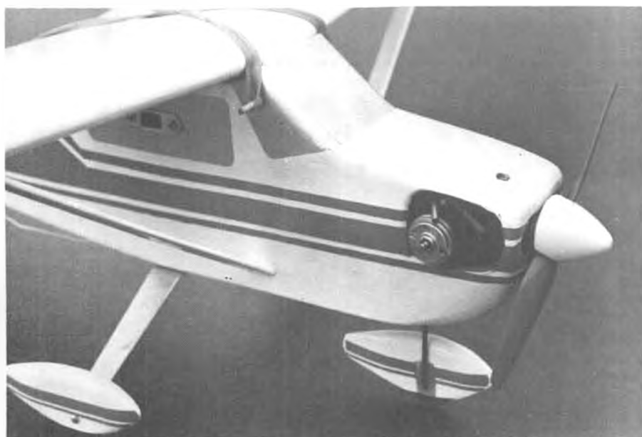
Business side of the model reveals the radio switch, engine cut-out, and the nosewheel strut fix. Separate fuel fill and vent were added for easy servicing. Spinner from Cox Sport Trainer.
