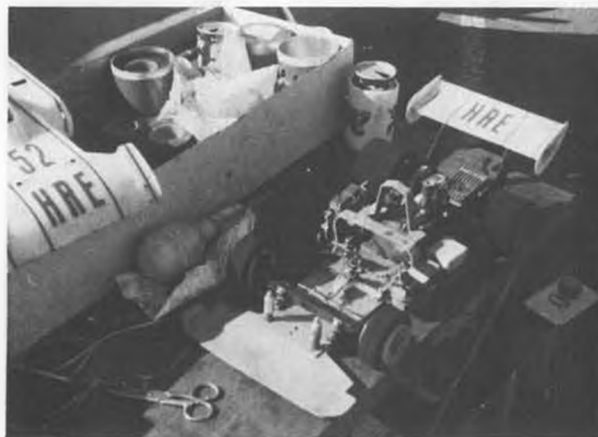
Weight biased to inside for left turns in columnist's Nats fast qualifier. Car won't handle without tip plates. Caster is noticeable.
