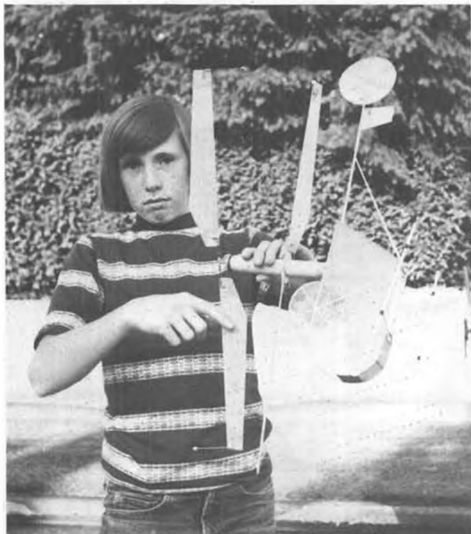
Roy's son Bob shows how to hold the 'copter for hand winding. It can also be winder wound from top end. Plug removable.
