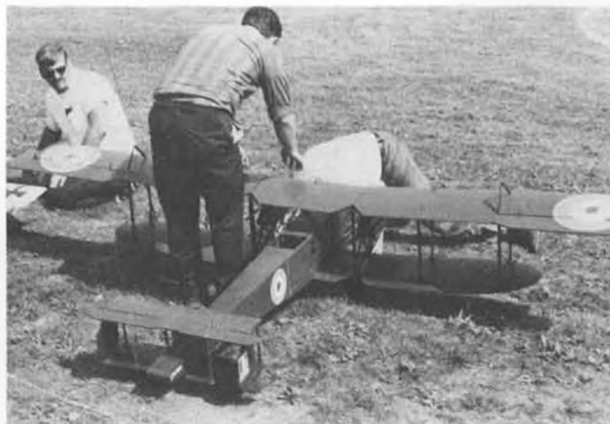
Magnificent Handley Page by John Goodrich, Burlington, Vt., spans 125" weighs 14 lbs.-10 oz, powered by 2 Max 60's, 1 1/4" scale. Flies!
