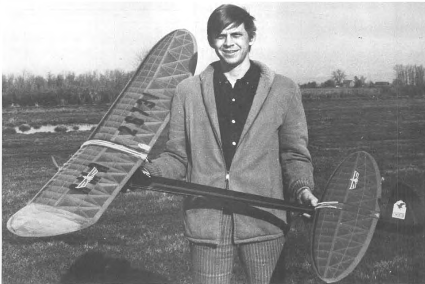
Co-designer Bob Stalick displays the clean lines of the "C-Quell". Geodetic wing and stab construction are essential in a ship this size, especially if a flexible covering material is to be used. Bob says NFFS decal is good for an additional 30 seconds on any model!
