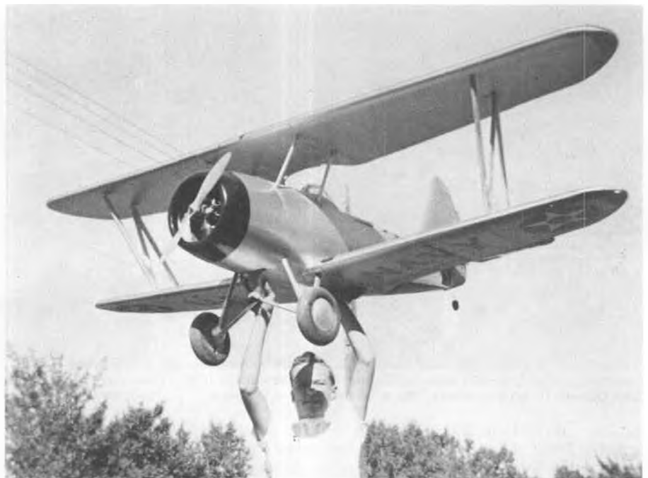
Remember the good old days in radio when we'd try anything? Bob Strand, Minniapolis, built this huge, 3'x1' Vought SBU-1. Forster 99, 19 1/2 lbs., 100" span, Bonner compound escapement(!) worked by ED receiver, 7 1/2" wheelbarrow innertube tires. Did it fly?
