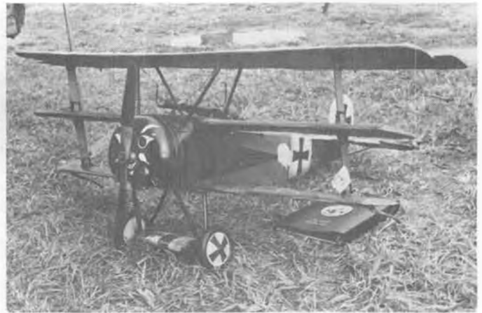
Tom Dietrick's veteran replica of Cole Palen's Fokker DR 1 at 2½" scale. Merco .61 engine and Skyleader (English) radio.
