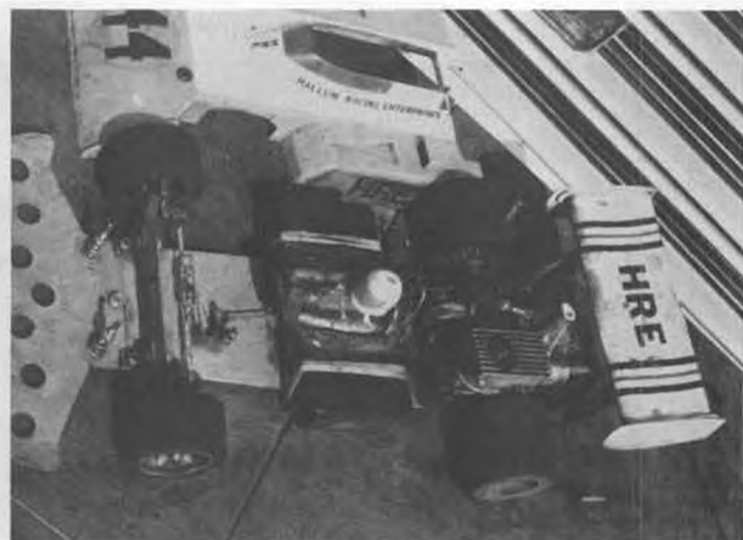
Chuck Engle's Amateur So Cal Formula Series warm-up winner. Uses exhaust pressure fuel system.
