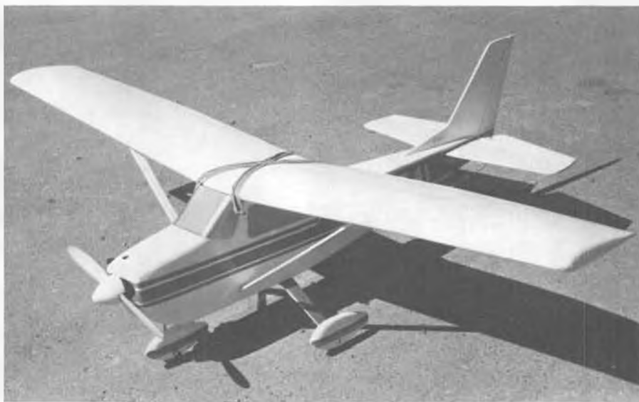
A simple modification of the Ace foam wing gives it the typical Cessna look. Ship is a snappy performer, and perhaps just a little tricky for a beginner. Reduced surface movement could help.
