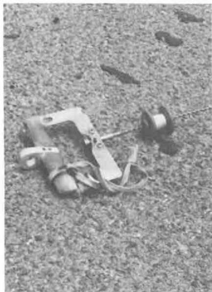
Special Monoline handle by Sam Snyder, to help young speed fliers to stay in the fork.
