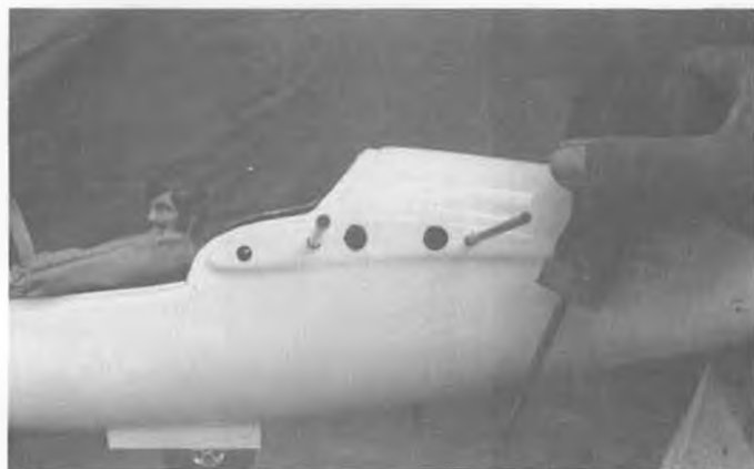
Filling the water ballast tank (balloon) in Jim Duda's Kestrel glider. Spoiler servo releases water when spoilers are deployed.
