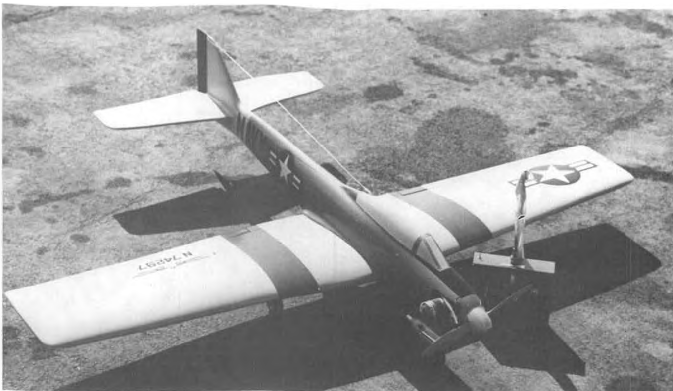
Charles Larkey's completed "Nutcracker" is brightly decked out in Navy blue and yellow. This was Jim Kirkland's last and finest design. Power is a K & B .61, and radio is by S & O.
