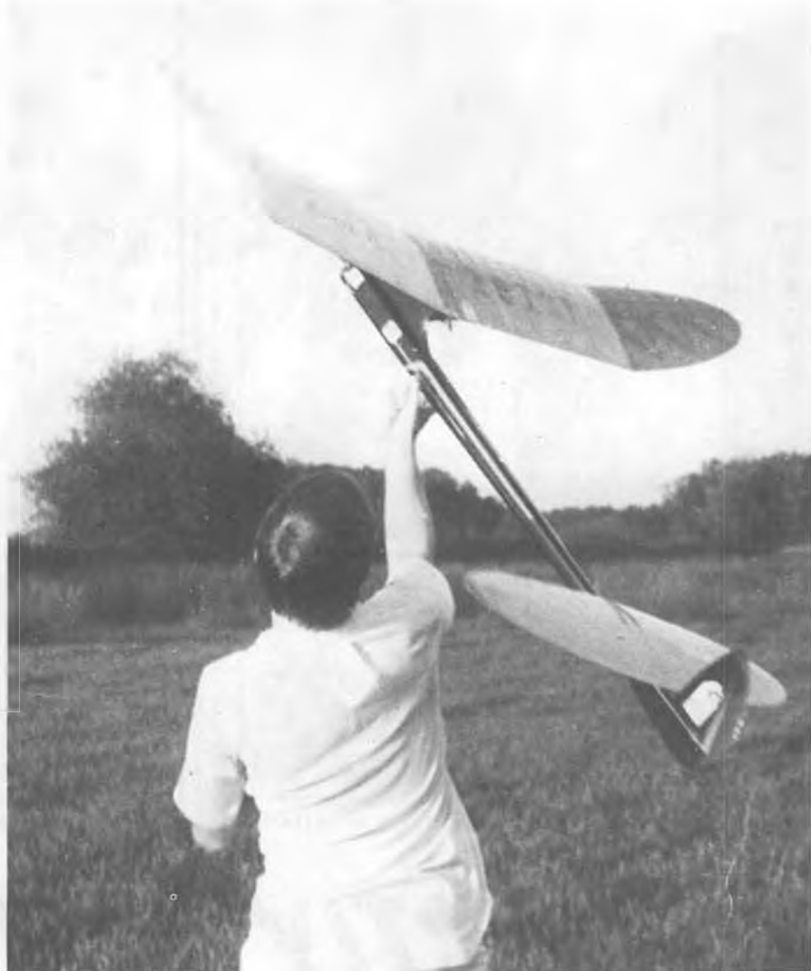
Bob "javelins" the "C-Quell" into the air. Climb is a tight right spiral, transitioning into a left glide circle with aid of stab tilt and a little left rudder tab.
