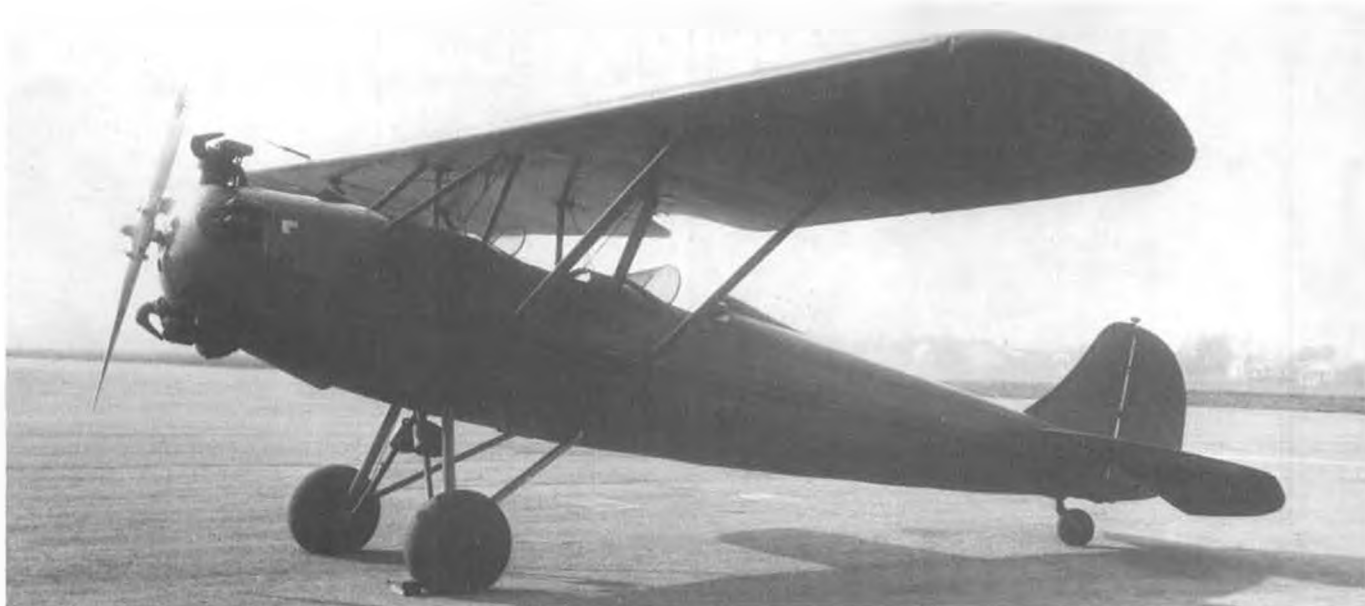
The sixth and last Meteor P-2-S, NC-12294. Five production models had Hamilton Standard props, and all six were powered by Kinner K-5 engines, 100 hp. What great lines for most any type of model; F/F gas-rubber-peanut-jumbo-CO 2 , or R/C. Photo by Pete Bowers.
