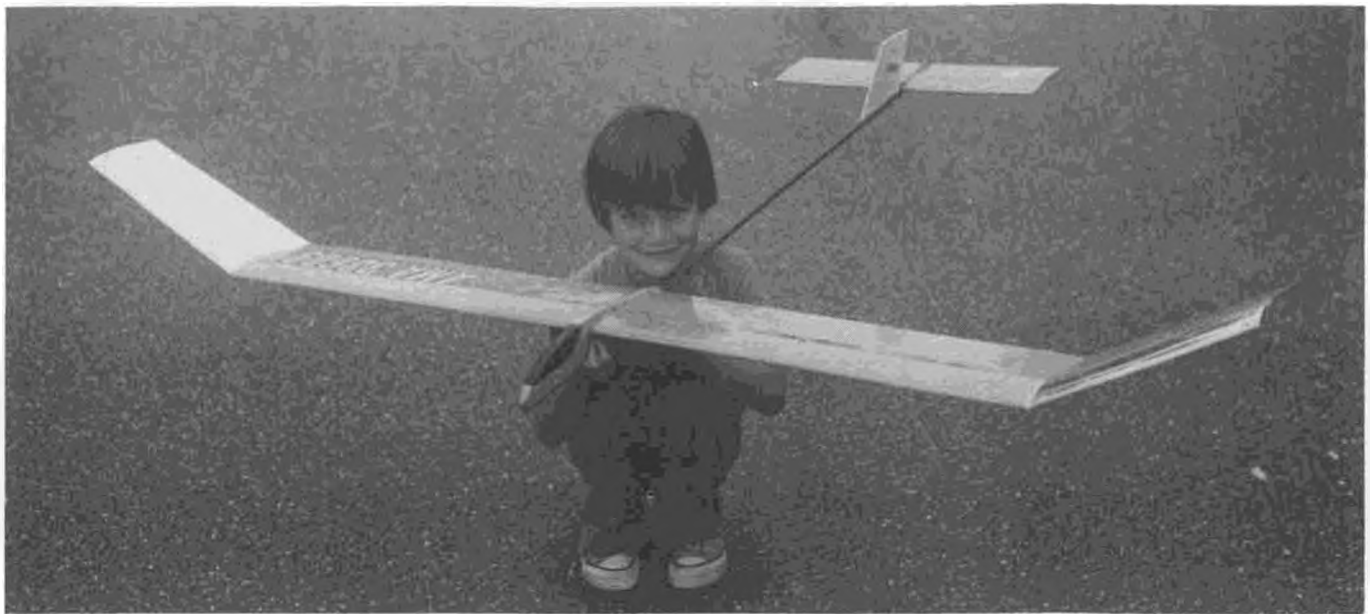
Carl Linstrum and his 72" span, all sheet balsa wing and stab A/2 Nordic. Placed 3rd in Junior class at '74 Nats. Called the "Big Bird," it was designed by . . . who else . . . Papa Dave. Construction is ultra-simple. Uses Bahrman fiberglass boom.
