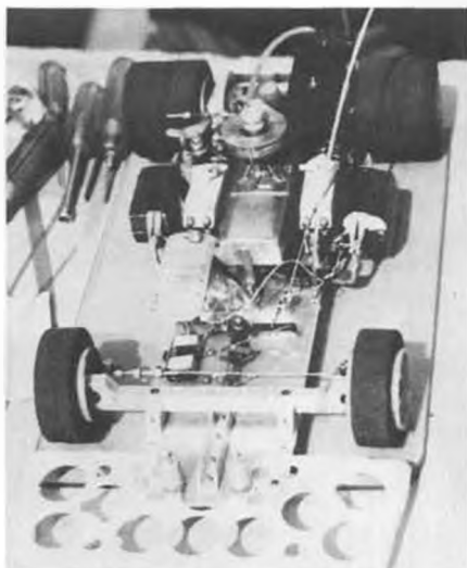
Mike Morrissey's top expert road qualifier. Typical, but tank raised to help fuel feed.
