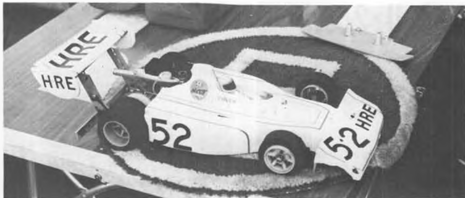
The author's Expert Oval Main winner. Layout had battery, fuel tank, and steering servo to left, same as in his 1974 car. Dig the fancy resting spot!
