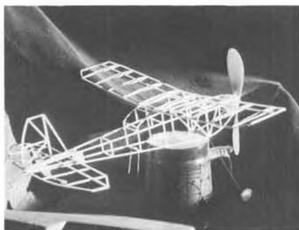
Framework of the TWIRP discloses the simplicity of the structure.
