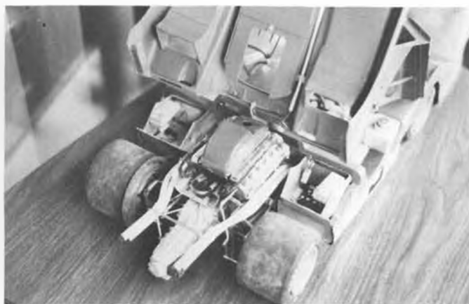
There's a Veco 19, exhausting through the manifold, under the scale V-12. Belt drive to left rear wheel barely noticeable.
