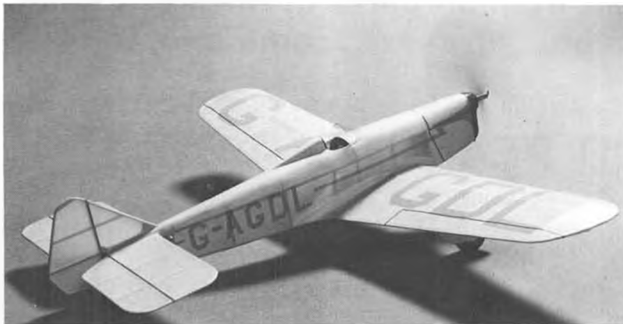
Beautiful Miles Sparrowhawk from Mooney/MB plans, weighs 1/3 of an ounce. Photo and model by Bob Clemens. Prop is free-wheeling. See the bent-over shaft?
