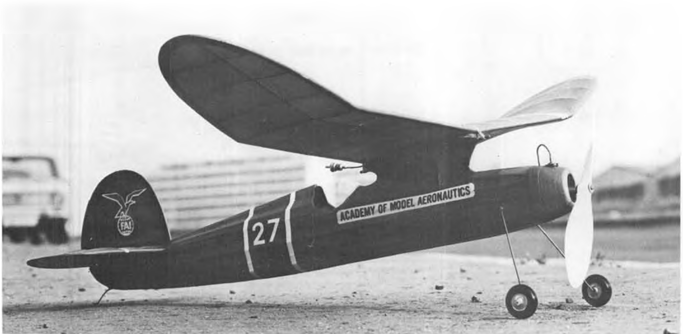
MB's modeling friend from Czechoslovakia, Milan Kacha, built this CO 2 powered New Ruler from printed sheetwood and plans by Ed Toner. The stretched nose is a little out of scale, but was necessary to make up for the extremely light Brown motor. Photo by Miroslav Kvapil.
