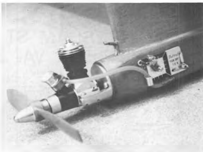
Fuel tank filler and vent tubes come out through the leading edge of the pylon. Fuel outlet located conveniently for Tatone timer.
