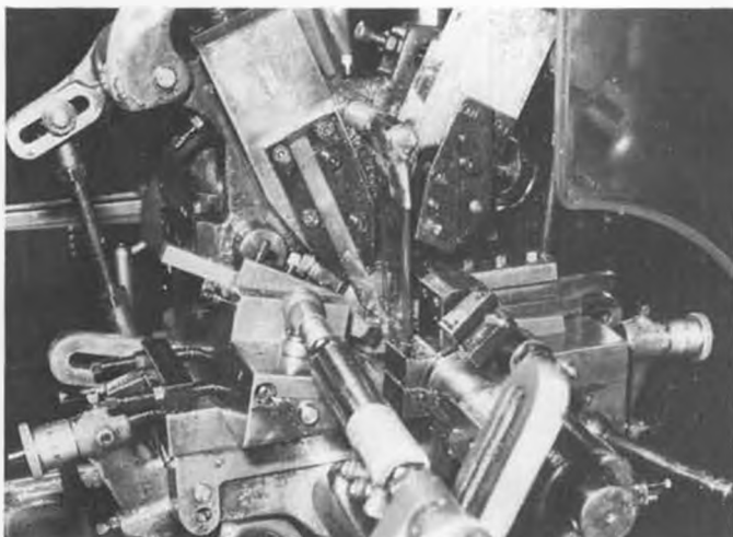
A Kavan automatic machine in action. About 5 separate operations taking place at once. Note solid oil stream in center of photo.
