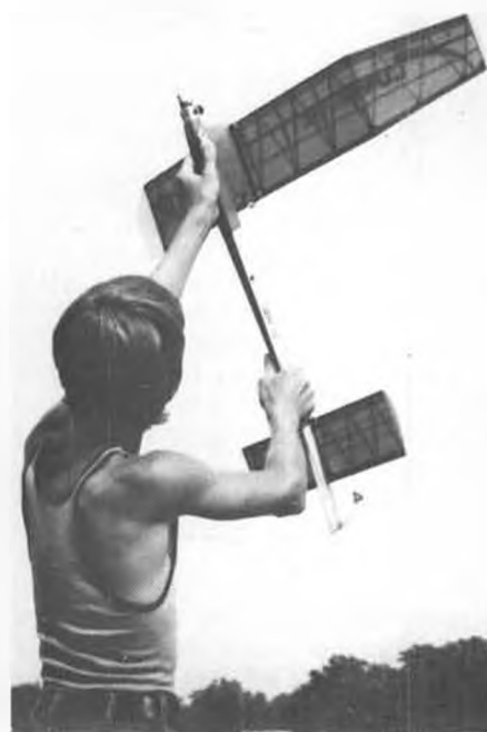
First flight launching technique, takes model immediately away from ground hazards.
