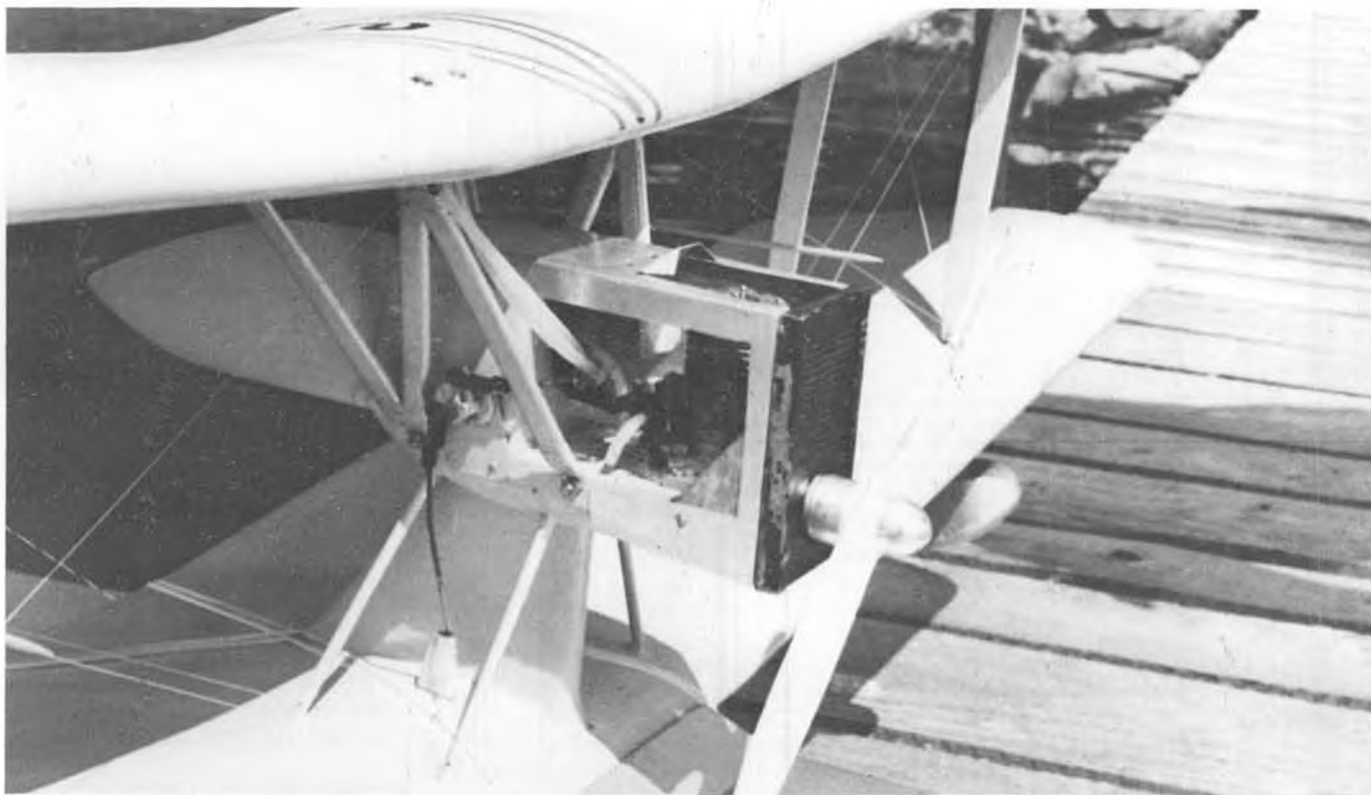
Close-up photo of engine mounting. Note waterproof shield around throttle linkage where it comes up through the lower wing. "Rustic" cowling is very typical of early 20's era . . . certainly no problem with cooling. Note fuel lines from tank to upper surface of top wing.
