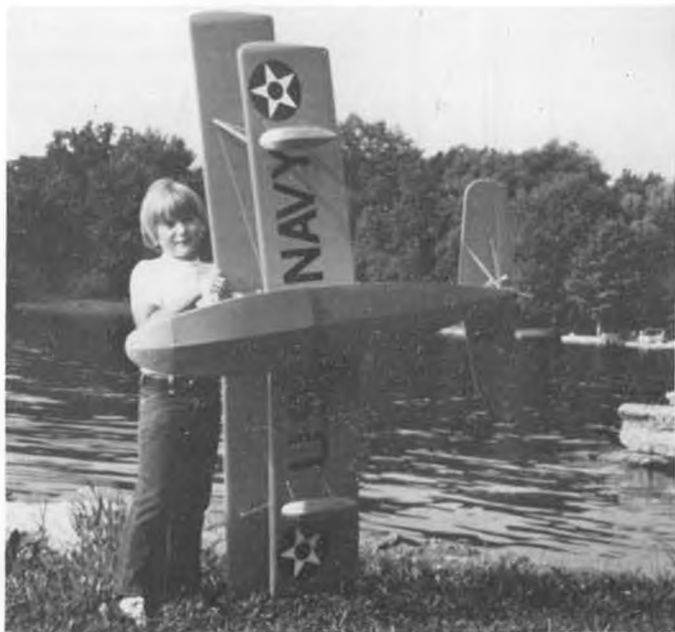
Our cover star, Jeff, gives us an underside view of the flying boat. Ship is a slow and realistic flier with the .40 rear rotor Supertigre.
