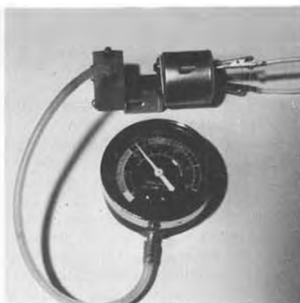
Pump unit pulling almost 12 inches of mercury on automotive vacuum gauge. It will lift fuel better than 10 feet above the container.
