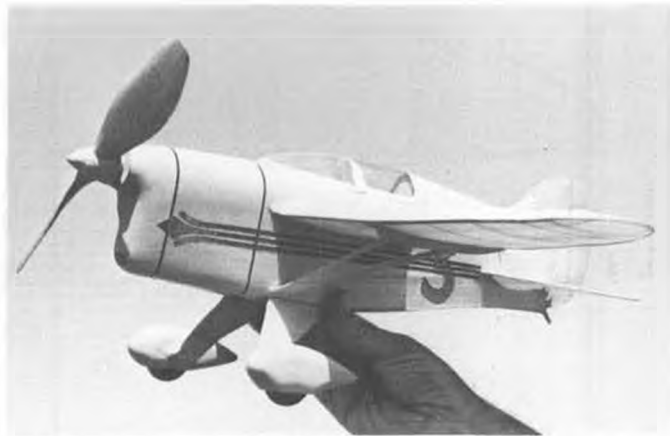
Art Chester "Jeep" by Tom Laurie, uses the R.A.F. 34 airfoil described in the text, also has trick stab incidence adjuster.
