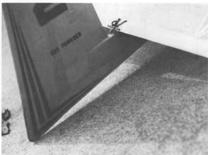
Detail of the stab hold-down, which goes through 1/16 I.D. aluminum tubing into the fuselage. Yep, that is "de tail!"
