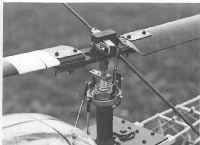
Close-up of the rotor head on the Kavan Alouette.
