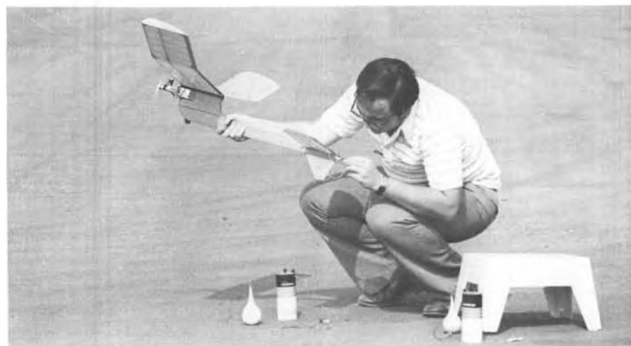
Eddy Flock, converted R/Cer, lights fuse on his Starduster. It flew "right off the board." Stock Tee Dee .049 on Cox Tankmount.
