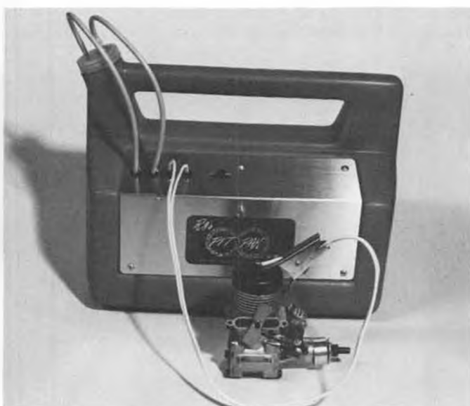
Glow plug clip line has connecting pins installed. Jug holds 1.3 gallons of fuel. Bottle comes in three colors. A very compact unit.
