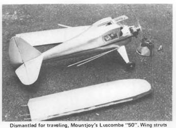
are functional. Fuselage is 1/16 sheet over bulkheads and stringers.
