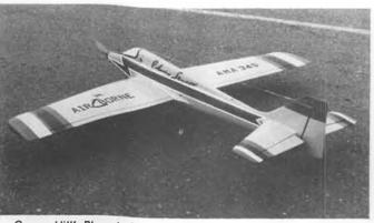
George Hill's Phoenix 7, his latest Airborne Associates production kit. Fiberglass fuselage, foam wing cores.
