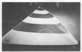
Hooked leach on a Newport 12-Meter main, caused by too tight leach tabling. Battens removed.
