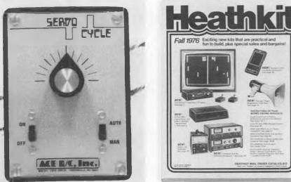
Ace R/C's Servo Cycle checks and breaks in servos.
