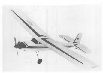
M.E.N. Trainer, for 3-channel radio and .15 to .25 engines.
