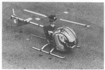
John Tucker's completed Super Heli-Baby, with Webra 40 engine. Only difference from regular model is collective pitch rotor head.
