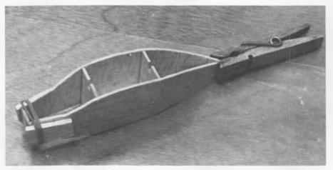
Pod is clamped together while glue dries, with clothespin at rear, and with rubber band at nose. Scrap balsa is used as padding at nose to protect sides from being crushed by rubber band.
