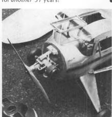
Another close-up of nose, showing radio, tank, and engine installation. Very neat work.
