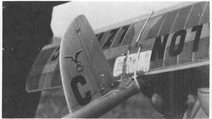
Tail assembly of winning Nordic displays some interesting mechanical goodies. Dial-a-trim on rudder!
