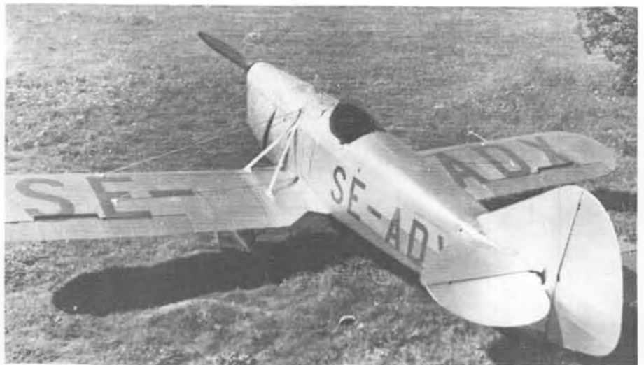
Original P-1 had civil registration, called S1. Note rounded wingtips, lozenge rudder, and no headrest. Note cooling air gill in cowling, similar to Tiger Moth.
