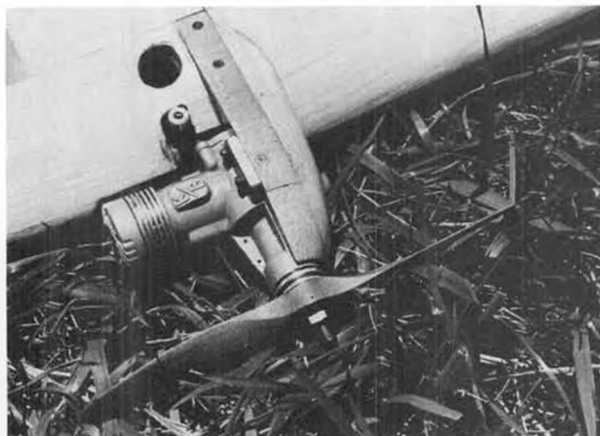
K&B .15 installation in US Combat Team member Chuck Rudner's FAI combat ship. Rear intake presents mounting problem.
