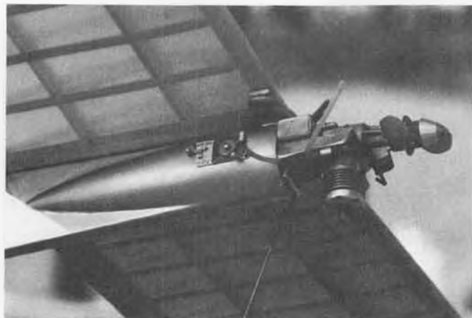
Front end of Virgil Coker's "Coker". Entry in A Gas had 650 sq. in. wing, and ST .19. Placed second.
