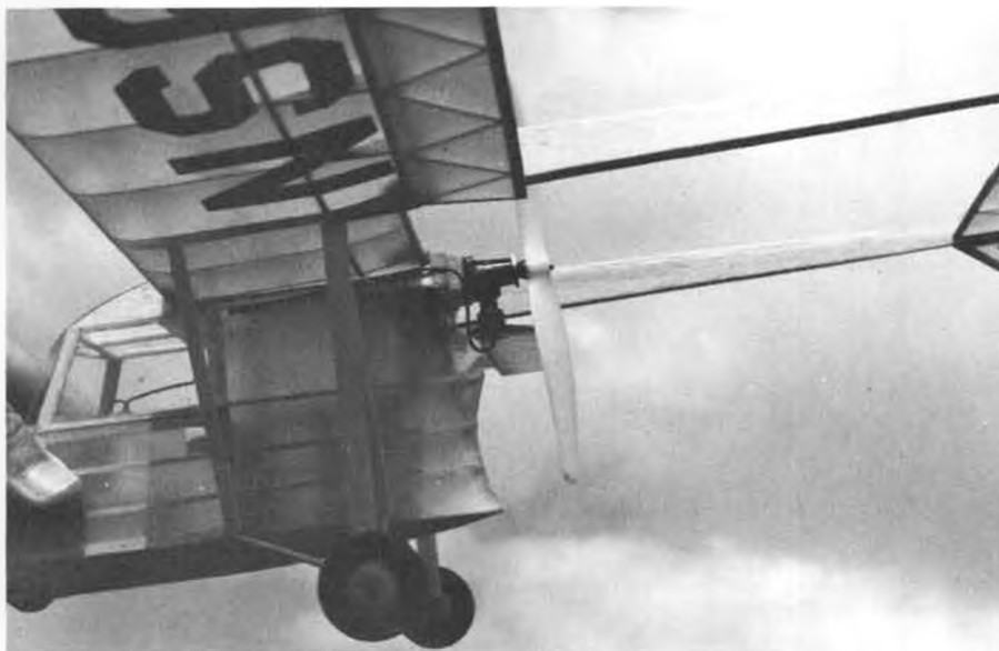
Cramped quarters for the prop are no concern with a CO 2 engine, as starting is extremely easy. One light flip should do it every time.
