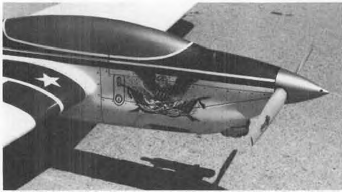
The business end of Citation stunt model, by Ted Fancher, San Francisco. Supertigre 40, Zinger 11 x 5 prop. Concours winner, also tied for 3rd in Open Stunt competition.
