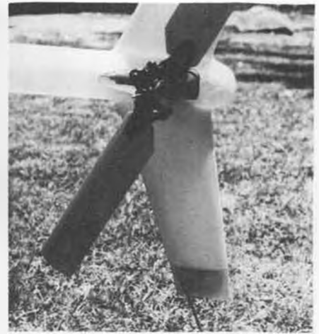
Tail skid is anchored in resin poured into hollow vertical fin. Good Kalt factory idea.
