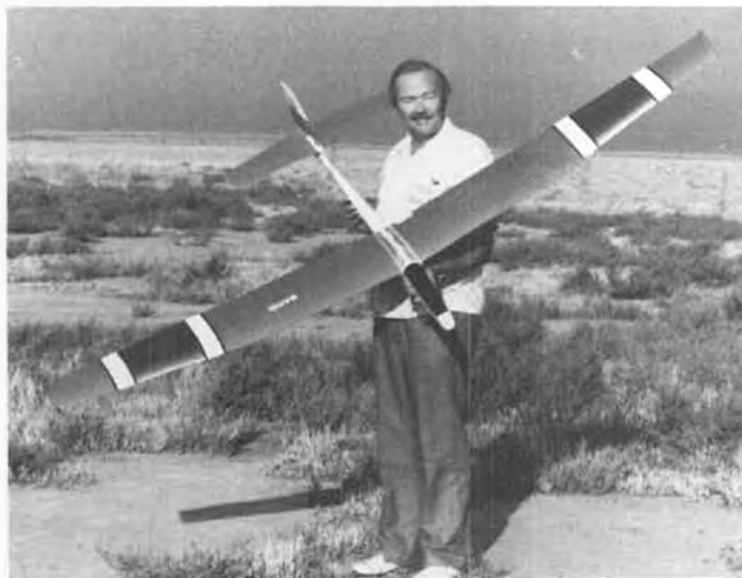
Bob Radcliffe, San Diego, and his Compromise. Olympic II airfoil, 888 squares, turbulators built in, flying stab, controls inboard.
