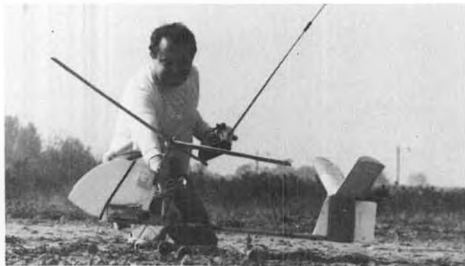
Georges Chaulet with his Gyro 76. This model has Enya .35 engine, throttle and rudder only, weighs 3 pounds. Profile cabin of styrene.
