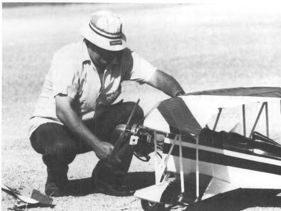
A 16 ounce fuel tank provides 15 to 20 minutes of flying time on Charlie's GLT, about 10 cents worth of gasoline. Compare that to glow fuel! Engine is easy to start, doesn't bother radio.
