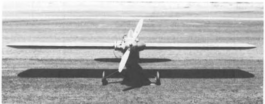
In his article, Austin Leftwich talks about the reduction of frontal area which was accomplished when designing this 3rd aircraft in his "Lil' Gem" series. Here you can see the results.
