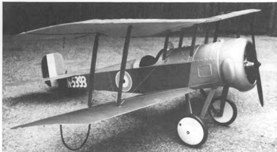
Quarter-scale Bristol Scout, built by Hank Iltzsch, Seekonk, Mass. Power, a bit marginal, is a Profi .76, turning a 16 x 4-1/2 prop at 9000. See text about big engine situation.
