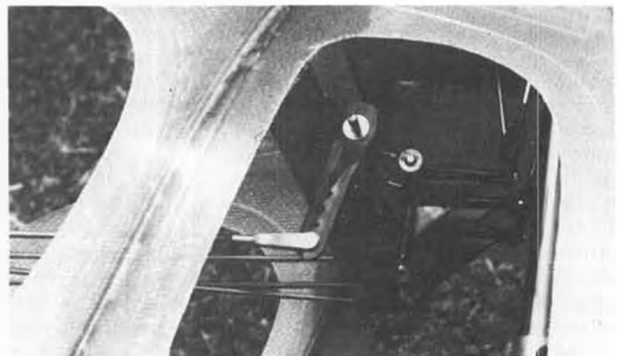
Side view of "walking crank" for lifting swash-plate. Schluter control arm provides leverage to lift the three ballcranks.
