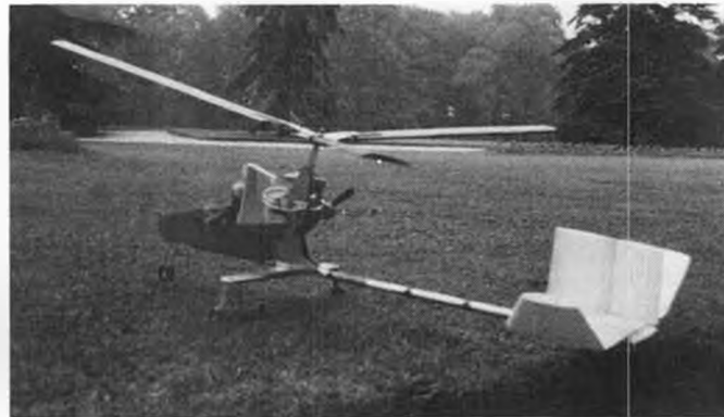
The 1977 Gyrotor from another angle. Note complete lack of wings. Foam tail surfaces. We'll have an article by Georges in near future.
