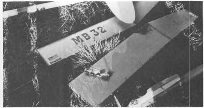
Russian power models had .03 dural wing skin. Mozyrsky's landed on high-tension lines, burned holes through skin.
