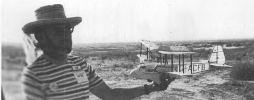
Bill Warner and his Airspeed AS 4, powered by no less than three electric motors. Electric power sure gets you away from that old multi-engine starting and tuning problem.
