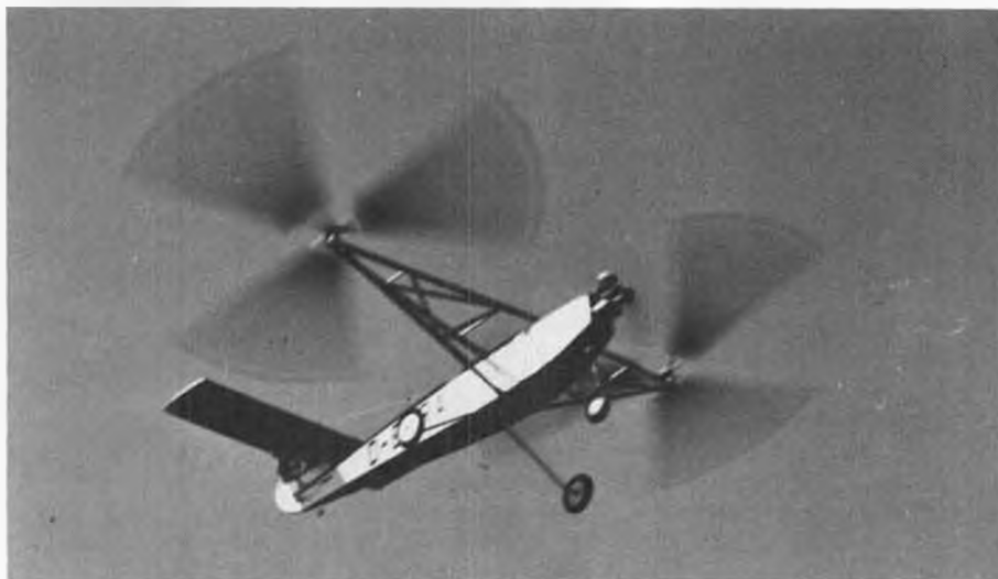
Skip Ruff's FA-61, in slow, stable flight, is an easy target for a photographer. Ship has all the characteristics desired of a trainer. A true autogyro, it has no wings, depends entirely on rotors.
