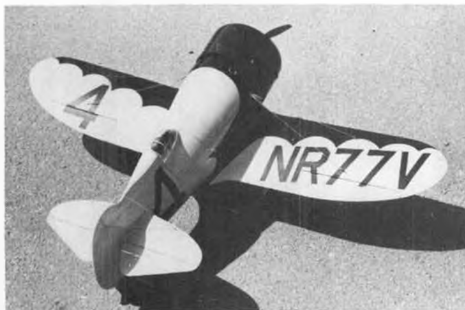
Granger Williams' Gee Bee "Z", powered by K&B 40, is stable R/C flier, but very tricky to get off the ground.
