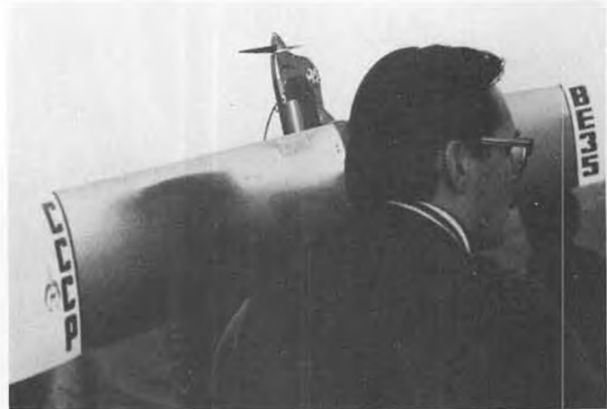
Igor Ziljberg, proxy flyer for Verbitsky, shows off the dural-skinned wing on Verbitsky's power model. Wonder if this will start a trend?
