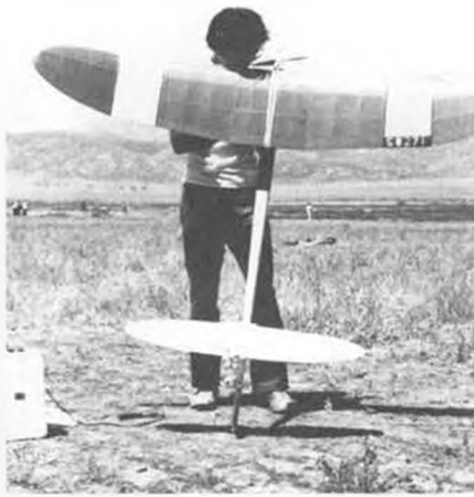
C Gas winner, Cliff Tanaka. His Satellite has extended fuselage, smaller stab, rear fin, OS .
