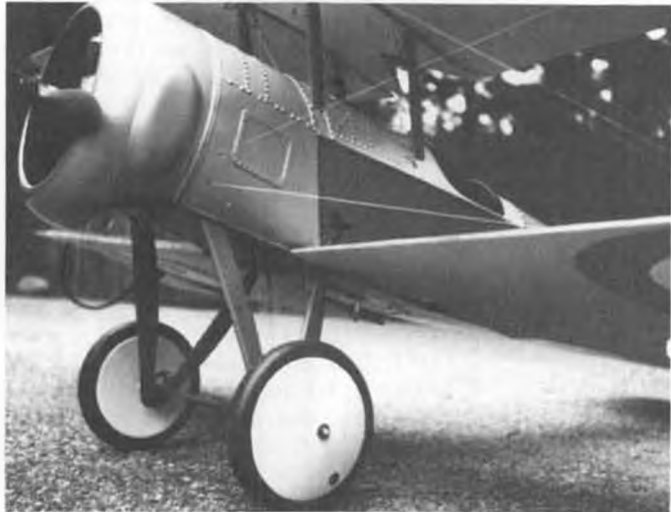
Close-up shot of Hank's Bristol shows off its AMA Scale detailing. AMA engine limit is 1.25 cu. in., but none this size are available.
