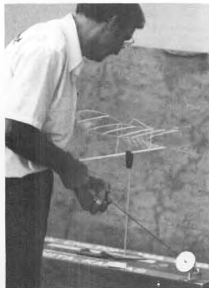
Stan Chilton watches torque meter, as he winds rubber for AMA stick entry.
