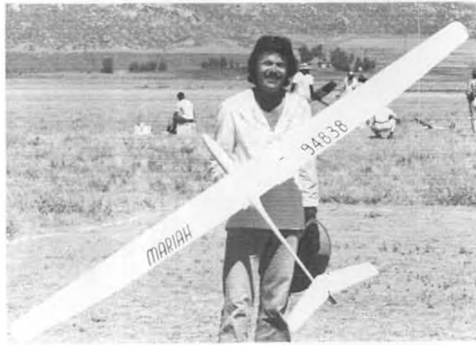
Noel Jones, Laguna, Calif., with Mariah. With 9-1/2 ounce loading, sleek ship gains efficiency through increased Reynolds Number.
