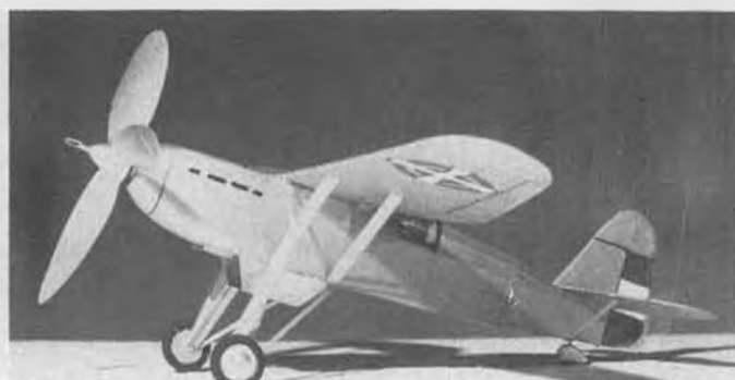
Long landing gear on this Yugoslavian design allows plenty of room for large flying prop, which is glued up from two Sleek Streak props and a rocket nose.
