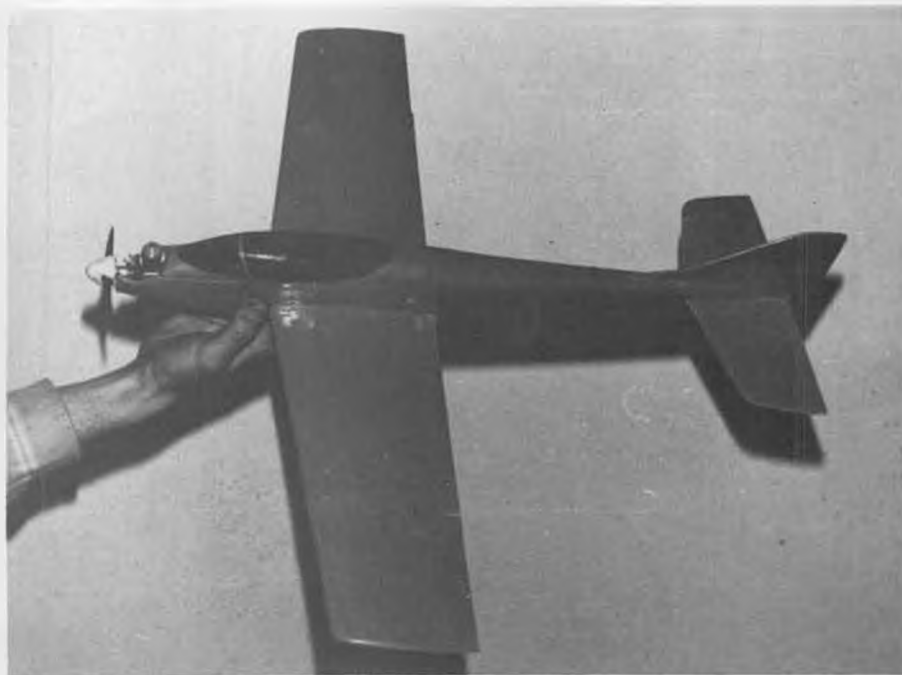
Another of Bob Parks' original designs is this Tee Dee .020-powered pattern model. Weighs only 8 ounces. Bob says it flies smoother than most .049 ships.
