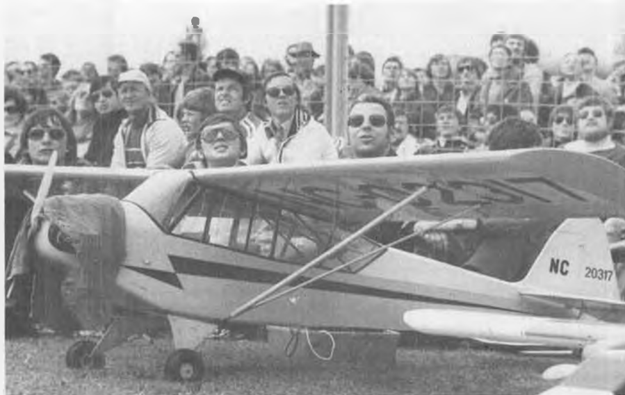
Hermann Sakbrook's J-3 Cub was one of several big models that showed up at Harsewinkel. Model spans 11 ft., 9 in., and is powered by a Quadra.
