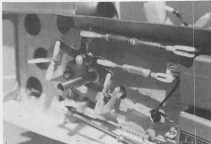
Don's Cheyenne uses the same positive/negative spring control concept as the full-size machine. Talk about authentic!
