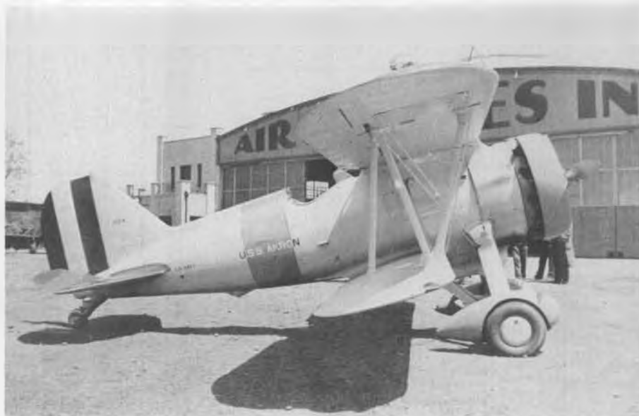
Assigned to the Akron, 9058 received blue recognition color; band on fuselage, chevron on wing, wheel fairings, cowl and anti-drag ring. Nine inches added to fin, blue portion.
