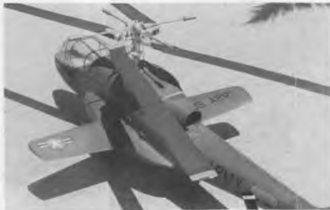
The rotor blades on Don's Cheyenne are foldable for transport and storage. Model is one of the first to use a rigid rotor.
