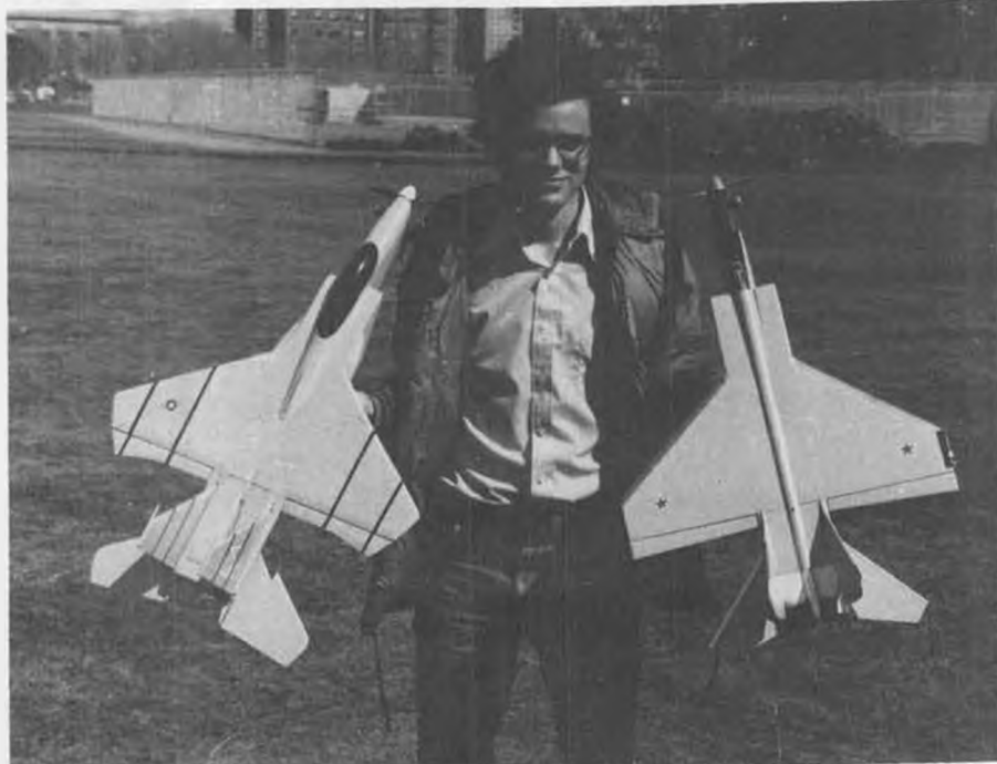
Dave Felsenthal with two of Bob Parks' 1/2A screamers, an F-15 (left) and MIG 25. Both use Tee Dee .049's with bladder tanks. Roll rate must be something else!
