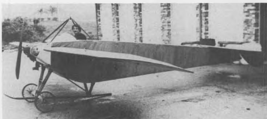
Reproduction Nieuport monoplane belonging to Cole Palen, Old Rhinebeck Aerodrome, N.Y., has Aeronca two-cylinder opposed engine. See text.
