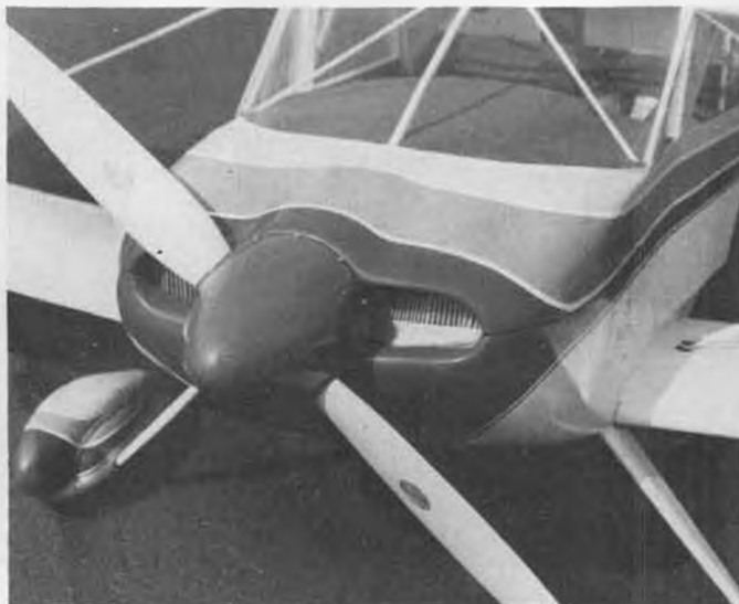
Close-ups of the cabin and nose on the Hiperbipe. The wild cloth pattern on the door panels was reproduced photographically. Hopefully, Bob will never break the prop; if he does, all he has to do to get the spinner off is remove ten 0-80 screws!
