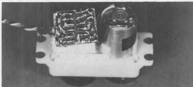
Servo guts. Note the uncluttered amplifier and the safe spacing between it and the motor.
