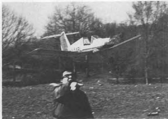
The heave. On low turns (125 this flight), launch it straight and level. On high turns, aim it about 15 degrees upwards and throw harder.
