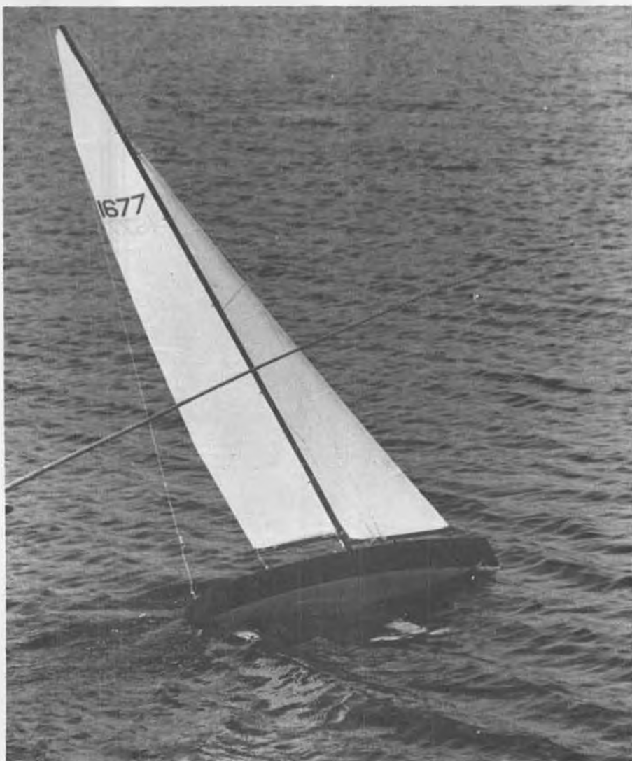
Featured in this month's article, the "Magic Dragon", pressed to weather, resists pitching forward, lee bow wave helps pointing ability by pressing on port bow.
