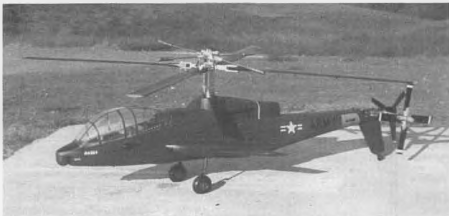
Don's Cheyenne has separate channels for cyclic pitch, cyclic roll, and the tail rotor. The fourth channel controls the throttle and collective, landing gear and pusher prop are on the 5th.
