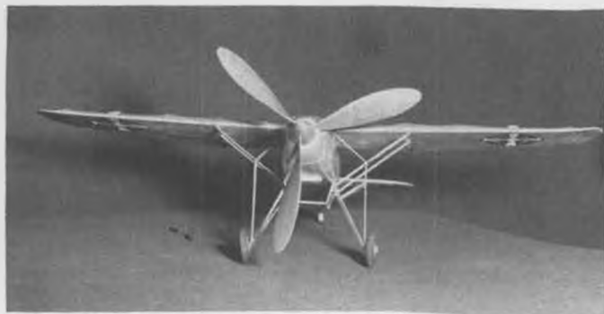
Long landing gear on this Yugoslavian design allows plenty of room for large flying prop, which is glued up from two Sleek Streak props and a rocket nose.
