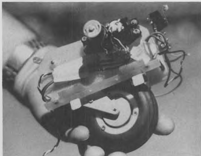
Handful of R/C retracting and braking mechanism built by Jack Alten, San Jose, for his Jantar.
