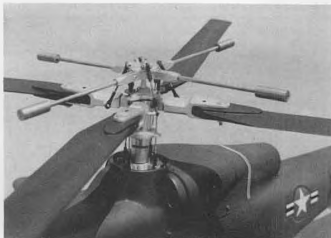
Close-up of the 4-bladed rigid rotor head. Outstanding design and workmanship is evident.
