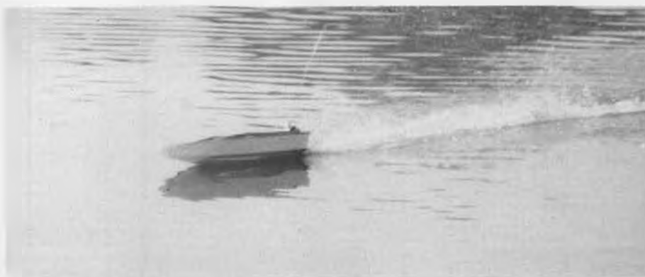
Test runs at Lombard, Illinois, showed a JG E-20 prop to be the best for this boat. At full throttle, very little of the hull is in the water.
