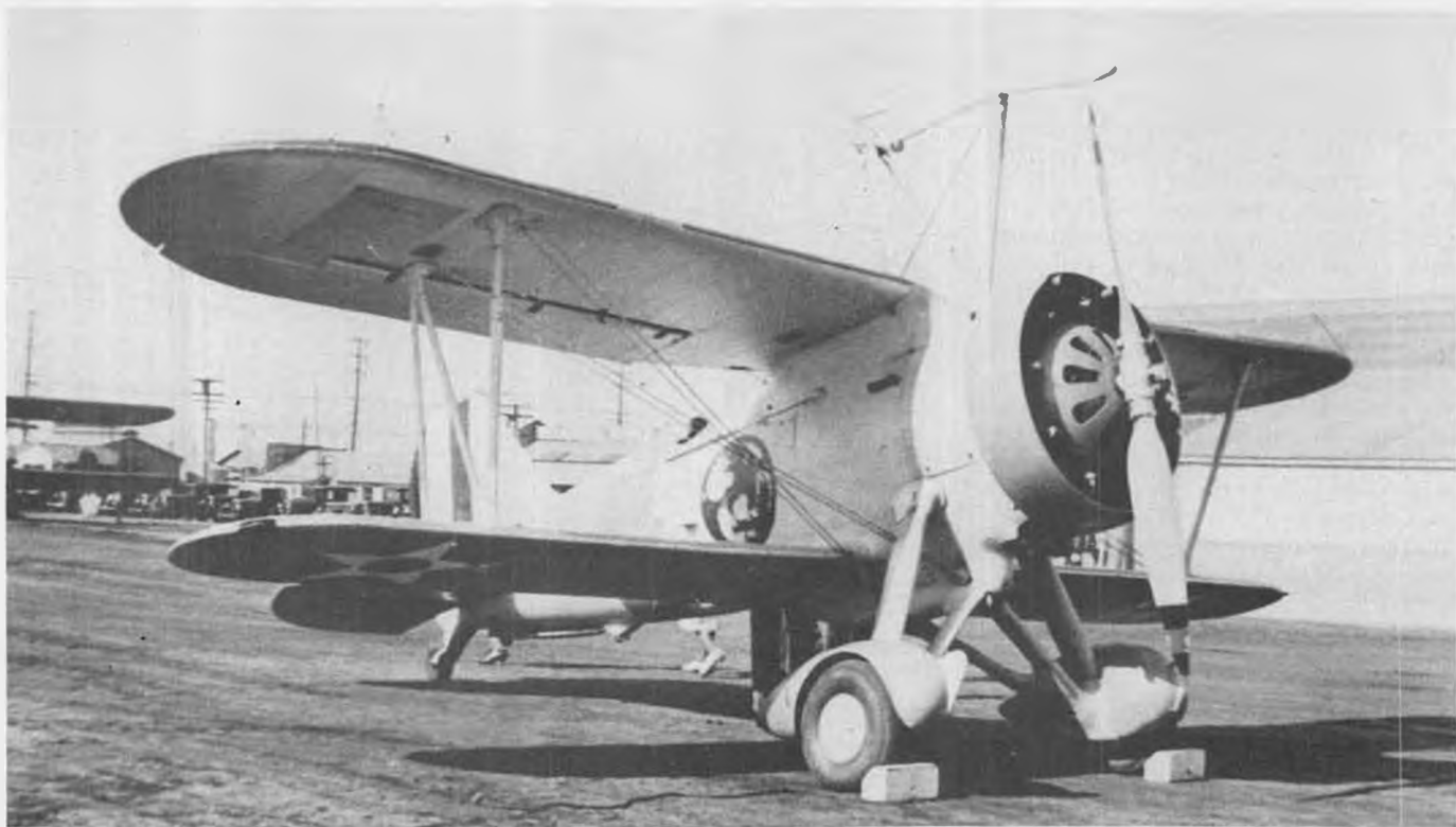
Fins on leading edge of wheel fairings were carrier deck arresting cable deflectors. Cable was normally 12 inches above deck, and 2 inches above axle on Sparrowhawk! Photo at Long Beach Naval Reserve Station, California.
