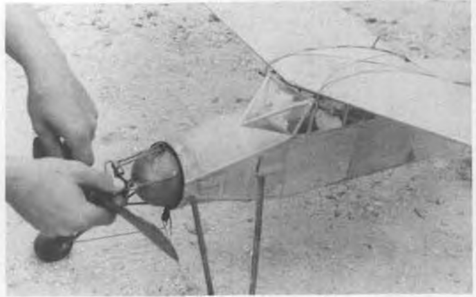
Close-up of Dodge's winner. Motor mounts on nose of air tank.
