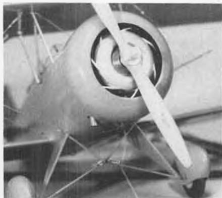
Even though cowl and exhaust collector ring completely cover the Webra .90, the aluminum shroud forces cooling air around cylinder.
