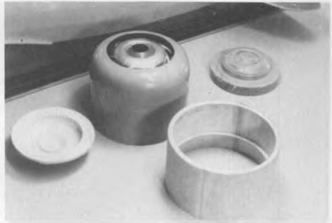
Finished and incomplete cowls . . . all-wood construction. Exhaust collector ring is molded fiberglass.
