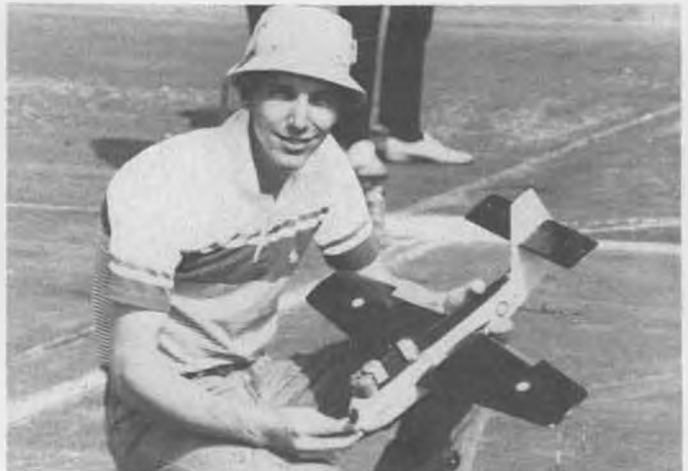
Former Navy Carrier Adv. Comm. Chmn., Dick Perry, with his 2nd Place (Class I) "Seamew". Bladder tank, ST G-40, 8 x 9 glass prop.
