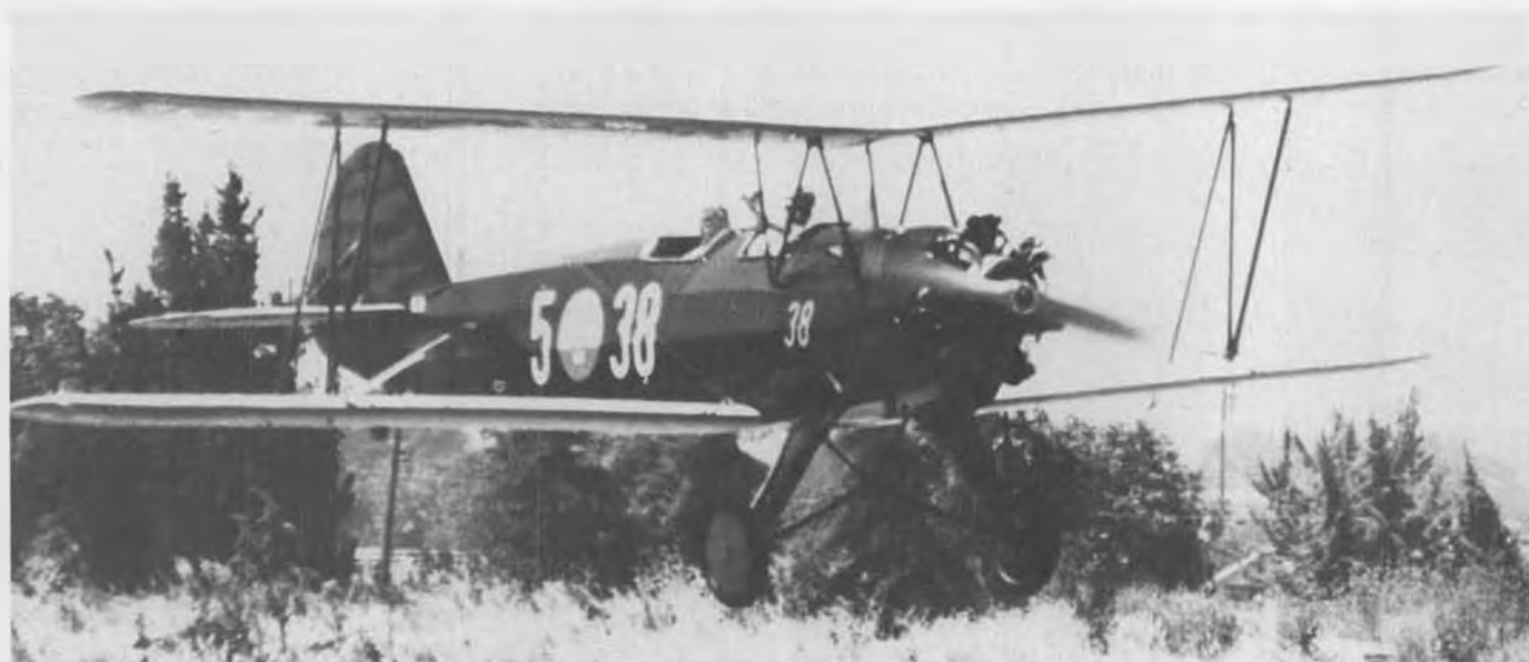
Monty Groves, Jr. makes a low pass in his Focke-Wulf "Stieglitz", featuring Swedish markings. Aircraft is powered by a 150 hp Siemens radial engine. Photo by Ken Hannan.
