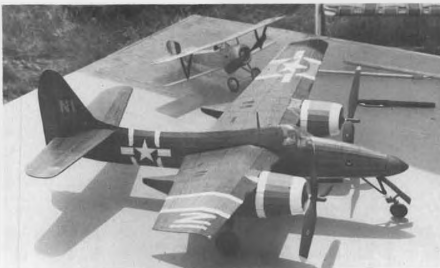
This Grumman F7F-1 Tigercat by Dennis Norman was one of two twin-engine models that showed up. Rubber motors are direct drive to the props.
