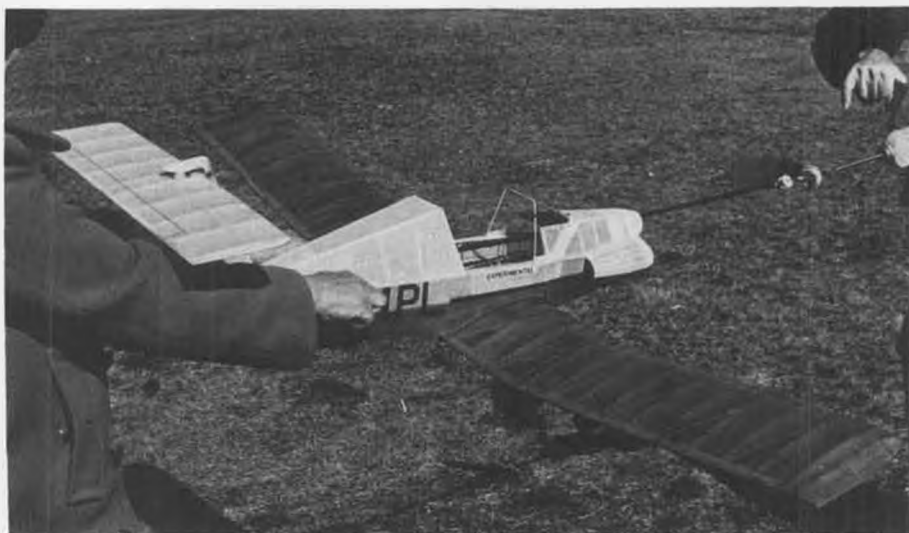
Living dangerously! Leon recommends using the winding tube if more than 150 turns are used. That long, high aspect ratio wing is no doubt one of the reasons for the excellent performance.
