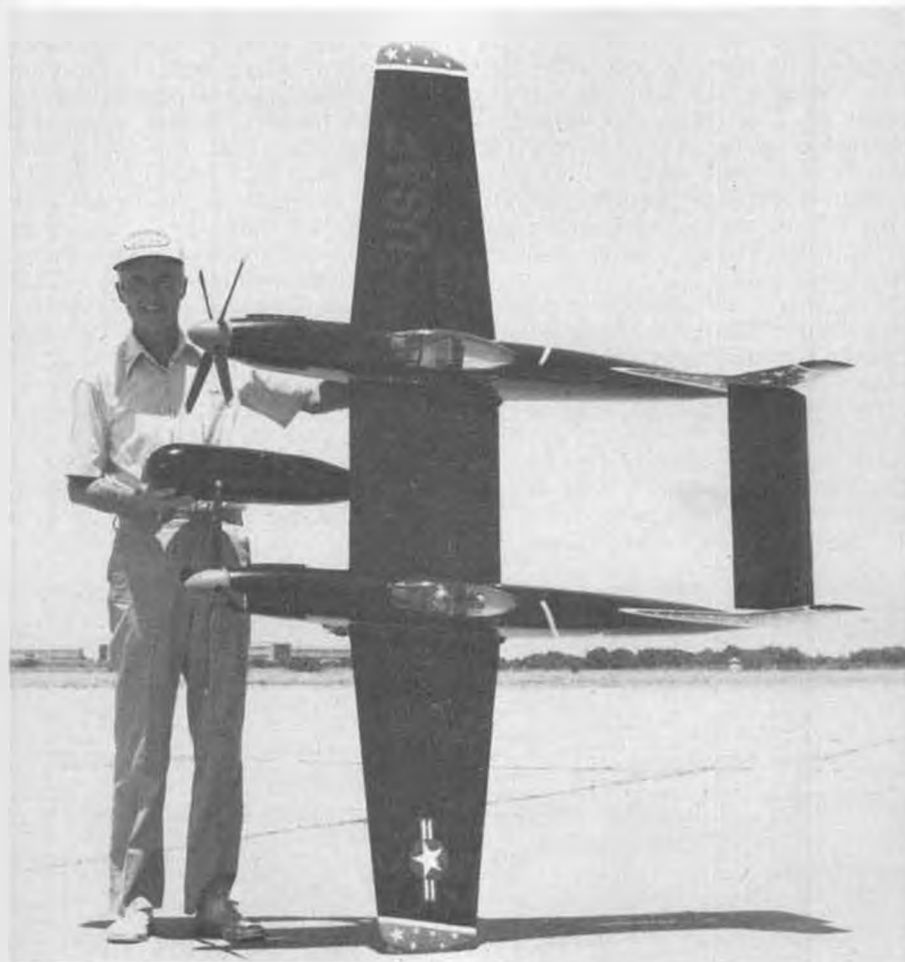
Another view of Col. Art Johnson's F-82-G (see inside cover, page 11) gives an idea of its size. No trim change for single engine flight. Plane just slows up.
