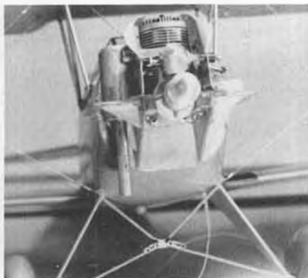
Even though cowl and exhaust collector ring completely cover the Webra .90, the aluminum shroud forces cooling air around cylinder.
