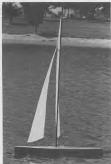
Bow slightly low on run, mast rotated 45° from slack rigging.
