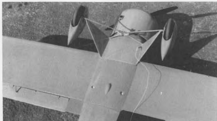
Underside shot shows nylon wing attachment bolts. Landing gear is 5/32 wire filled in with soft balsa.
