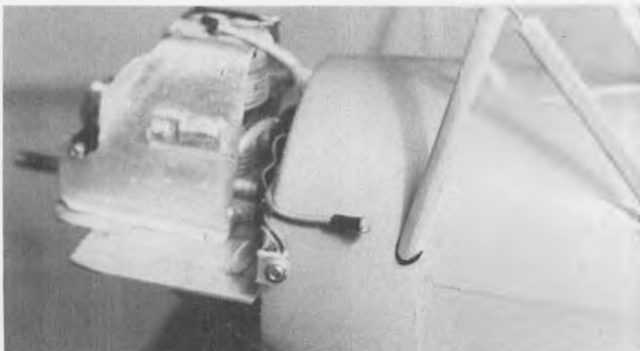
Glow plug leads come to battery jack which is accessible through cowl. Gas tank filler line just clears cowl.
