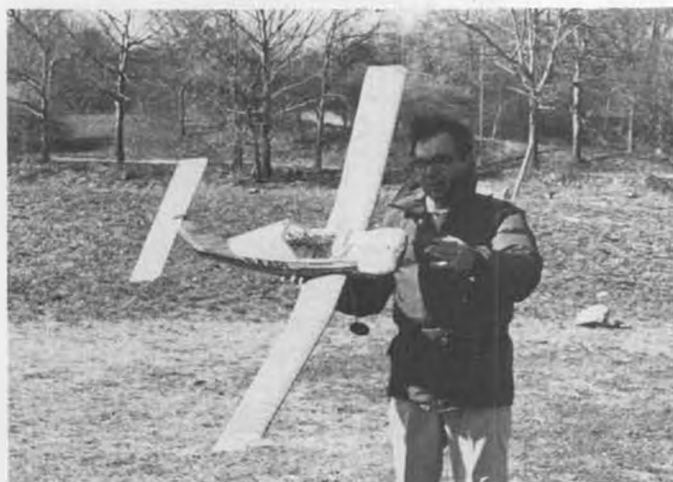
Checking trim before launch. Is noseblock seated? Tail incidence correct? Wing square? Car keys in your pocket?
