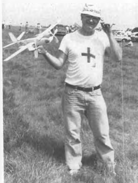
Neat A-26 by Ralph Kuenz had a best time of 32 seconds, uses geared rubber motors.
