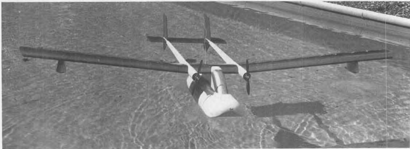
The first electric-powered seaplane to ROW was this twin Astro .15 design by Neil Whitman. The 7-lb. model had poor water handling and flight characteristics, led to the improved version shown at right.
