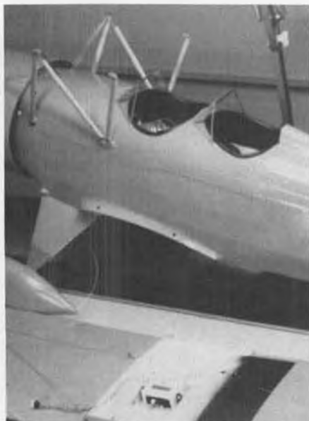
Neat fillet for bottom wing also houses flying wire terminals.
