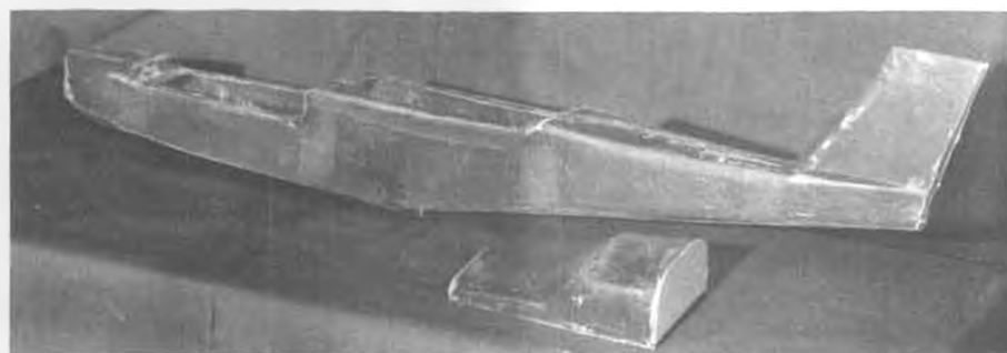
A fresh-out-of-the-mold fiberglass shell for the model shown directly above. Neil is a real craftsman with fiberglass.
