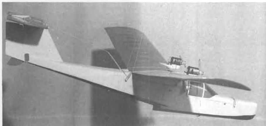
Another of Neil Whitman's designs is this twin Astro 020 flying boat. Again, no tip floats are used. Model flies well, ROW is marginal.
