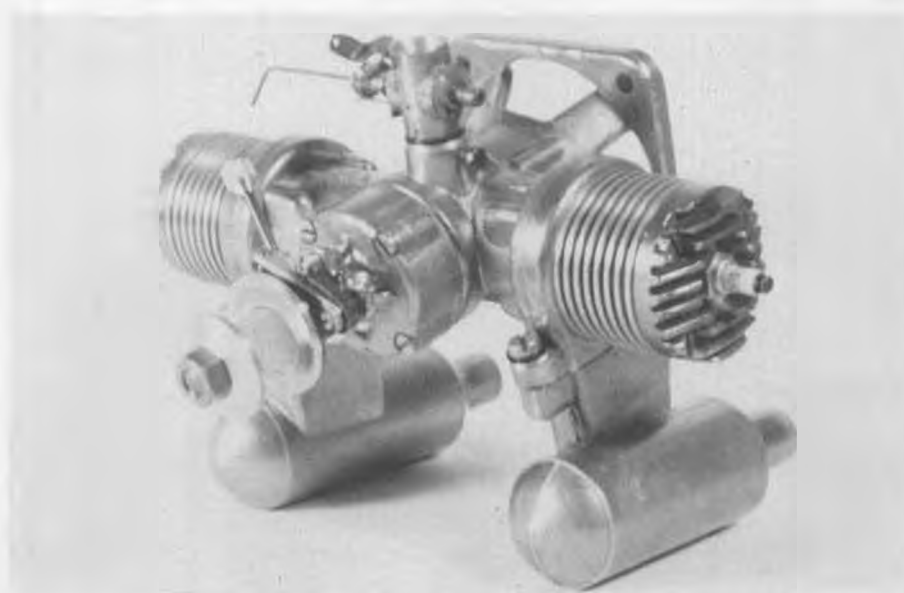
An FMO .61 twin, belonging to Ron Ford and converted to ignition by Otto Bernhardt. If you've got a photo of an unusual ignition engine, new or old, send it in!
