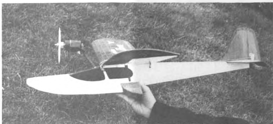
Mitch Poling's original design Astro 020-powered "Electric Tern" weighs 18 oz. with Cannon super-mini radio. Made newspaper headlines with rooftop landing . . . see text.
