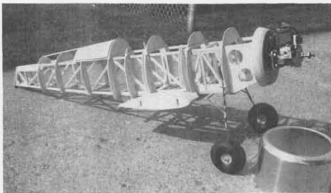
Les Hard, of Lansing, Mich., is currently building this 1/4-scale Stearman. Cowl for the 8-foot model is made from a 6-qt. kettle.
