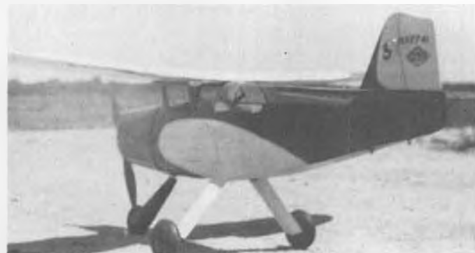
Pete's WF-4 was much racier-looking than his previous models. Tri-cycle gear is hardly ever seen on a free flight, even today.
