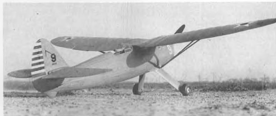
The WF-3 had a 65-inch span and was powered by a Baby Cyclone. Flew well despite a wing loading of 16 oz./sq. ft. This is the same model that lost a wing in flight . . . see text.
