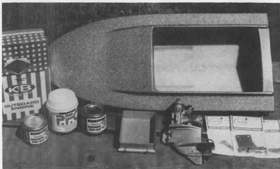
The ingredients of the E-Z Vee project: the E-Z Vee fiberglass hull, K&B outboard, Hobbypoxy Formula 3 glue and P.F.C. filler, and the Hughey Boats outboard engine mount.
