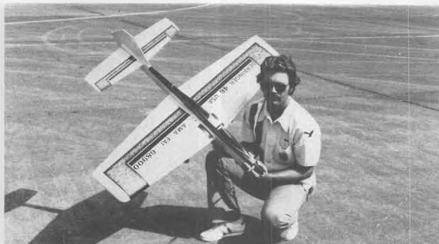
Bob Whitely, Fountain Valley, California, and his own-design "Derringer 46". S.T. 46 engine, 12 x 6 Zinger prop, J&K Products foam wing core. Built in 28 days!!
