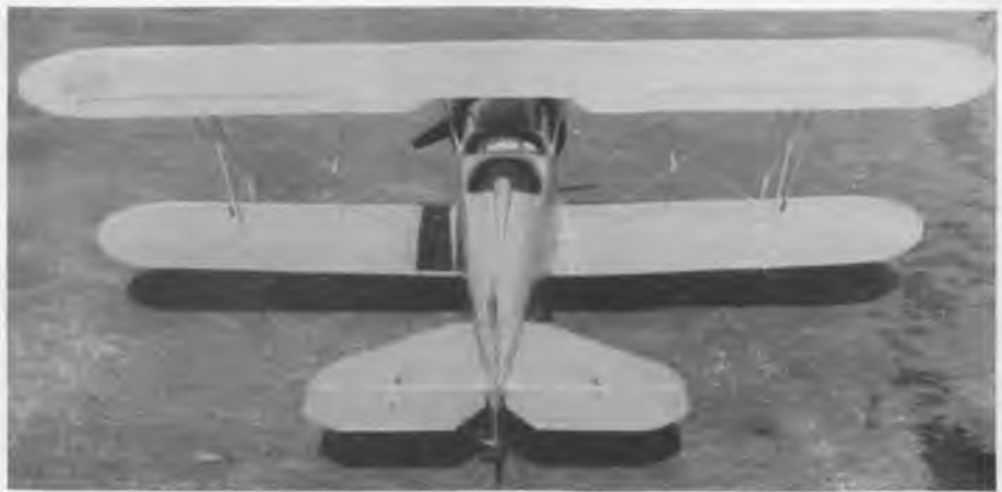
No Fokker-type "elephant ear" ailerons on this Speedwing version of the Travel Air. Remainder is almost exactly the same.
