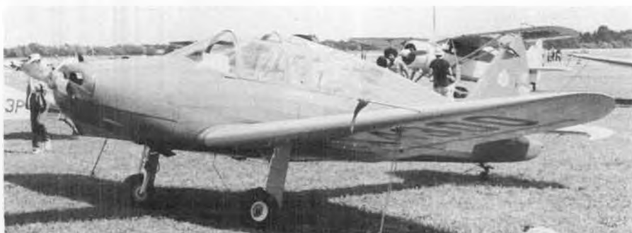
Piper Aircraft's first low-wing retractable gear airplane, the one and only prototype ever built. A very interesting plane, would make a good model. Blue fuse, yellow wings and stab.
