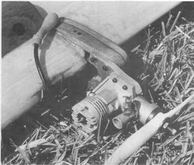
If you want to try FAI but only have AMA size models, try lashing a .15 on with an aluminum adaptor. Works great!
