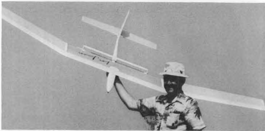
Woody Blanchard Jr. displays his original design "Les Joindres." Sailplane features a variable camber wing and a "flapler" over the center section of the wing.
