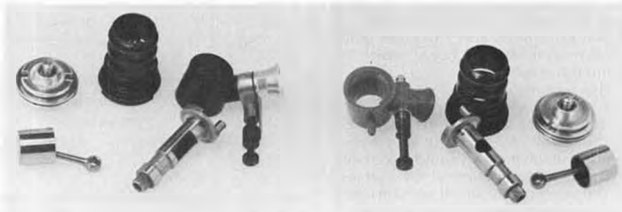
Innards of Tee Dee and Medallion .049's. Tee Dee on left has clear throat carb, big crankshaft port, twin ports in cylinder. Adds 3000 rpm, but drinks more fuel, too.
