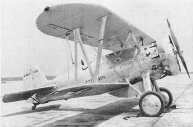
These nearly identical views clearly show the differences between the F4B-3 and F4B-4. Headrest and fin are obvious differences, but engine cowling and exhaust system are also different. Photo courtesy of Warren Shipp.
