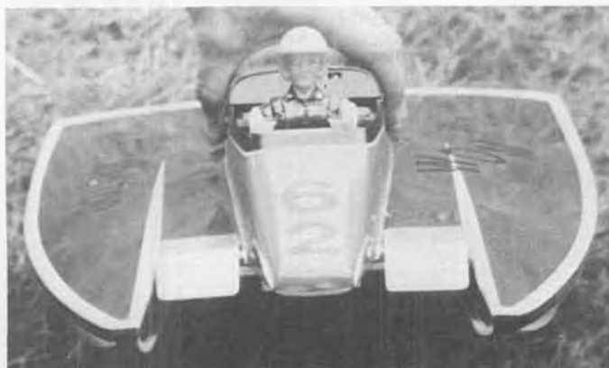
Front shot of Bill's Dumas Hotshot shows the use of air deflectors. Boat was timed at 1:52.3 for .9 mile oval.
