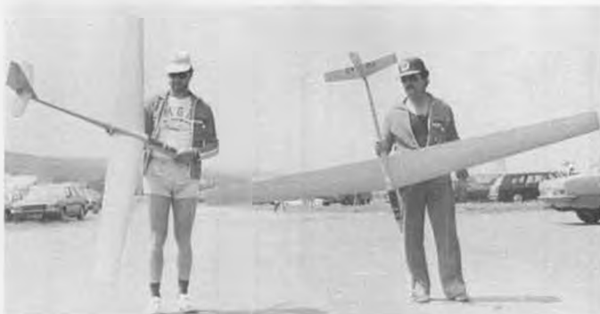
Fredi Schenk (left), Switzerland, and Rolf Girsberger, Team Manager. For roll control, each wing panel pivots at the root; there are no ailerons. Makes for an ultra-clean wing.
