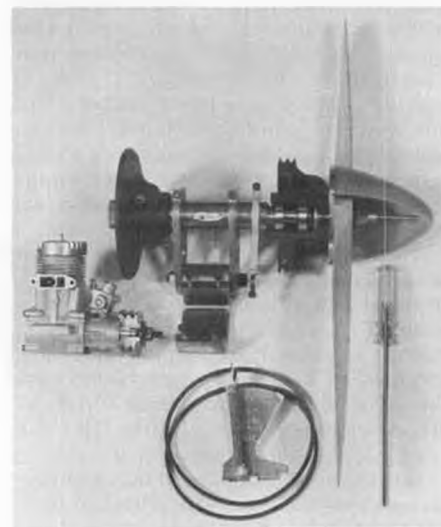
Factory photo of Byro Drive with O.S. .60 SR. Available to fit most popular engines.
