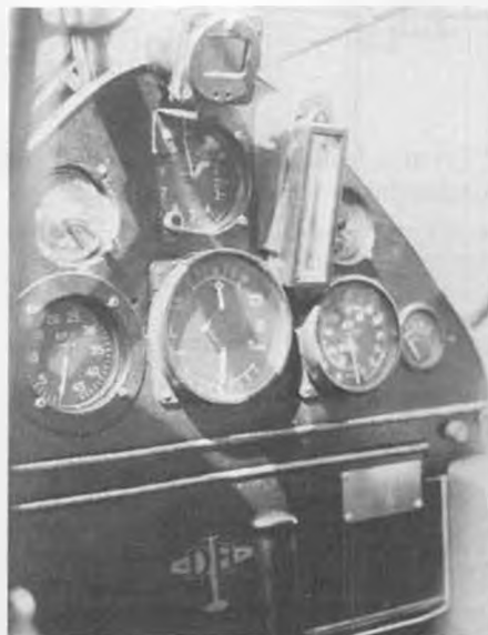
Puss Moth cockpit details. Note the unusual turn and slip indicator.
