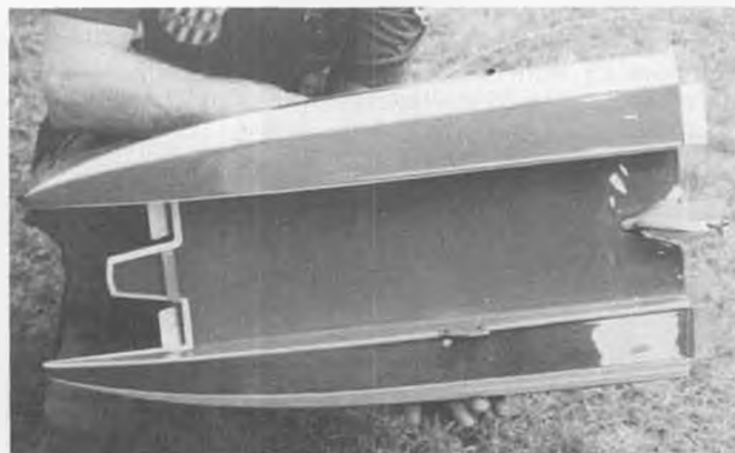
The bottom of Bill's Hotshot has been block sanded and ride strakes have been added.
