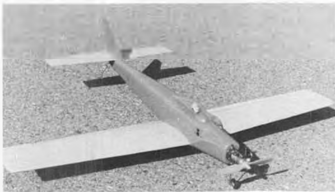
Darryl Stevens built this 2-channel hot rod with balsa sheeted foam wings. Pacifier tank and 5X3 prop make it very fast.
