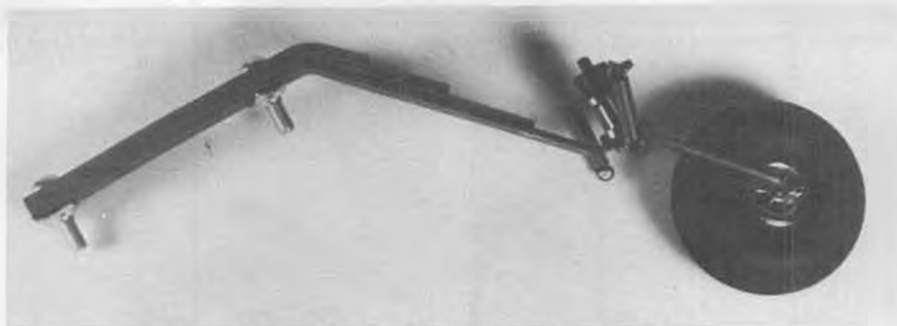
Also from C.B., a real workhorse of a tailwheel assembly for large models.
