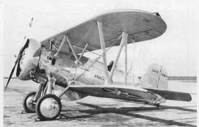
These nearly identical views clearly show the differences between the F4B-3 and F4B-4. Headrest and fin are obvious differences, but engine cowling and exhaust system are also different. Photo courtesy of Warren Shipp.
