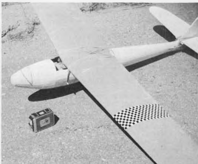
Old Timer enthusiasts should recognize this one. It's an old 1938 Berkeley Cavalier, converted to an R/C glider by Gordon Coddling. Span is 9 feet, and a Kodak Brownie movie camera can be fastened to the engine mounts for in-flight movies.
