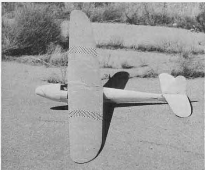
Old Timer enthusiasts should recognize this one. It's an old 1938 Berkeley Cavalier, converted to an R/C glider by Gordon Coddling. Span is 9 feet, and a Kodak Brownie movie camera can be fastened to the engine mounts for in-flight movies.
