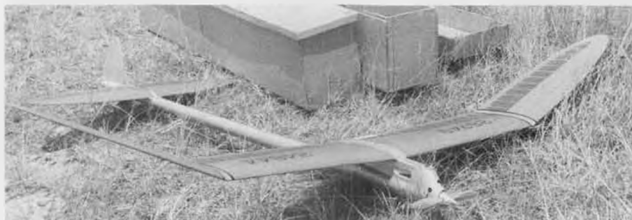
Mark Valerius and C.C. Johnson came up with this new design to handle power of new Schneurle engines (see Ralph Prey's comments in text). Resembles current FAI trends.
