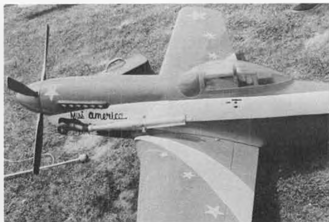
Powerplant details on the Byron P-51 flown by Dean Copeland. Uses a hot .60 mounted on a Byro Drive speed reducer.
