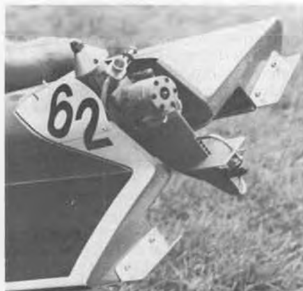
Rear view of Bill's Hotshot, showing the ride plates on the back of the sponsons.
