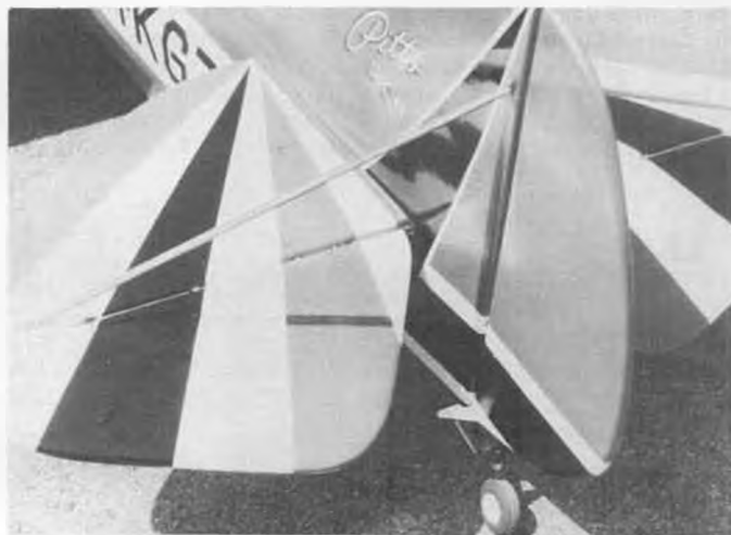
Tail assembly details. Stab brace is 1/4-inch aluminum tube. Finish is K&B Superpoxy.
