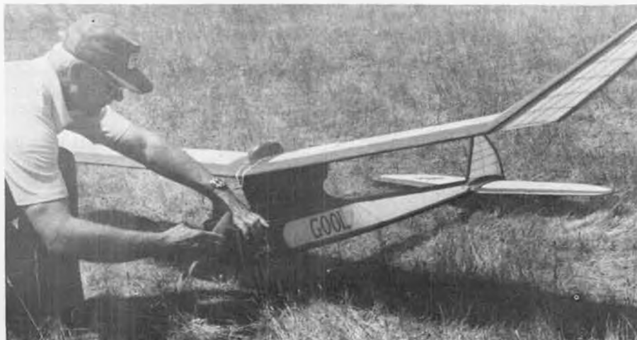
Larry Delaney used up 2 year's balsa rations building this "Gool." Hump on top of wing houses spoiler DT mechanism. Spoilers can be seen in half-up position.
