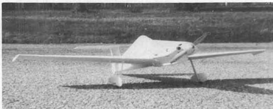
Another view of Dave Latsha's Rivets. Note the very clean frontal profile and the anti-vortex wing tips. Still very competitive even though it's an old design.
