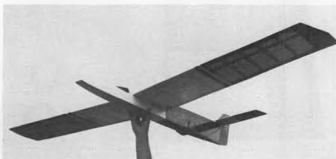
Two-meter wings have 819 sq. in. of area. Aluminum tube wing spar is typical of Legionair kits.
