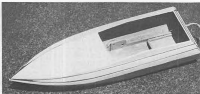
Top deck is masked off using Flex-Mask and regular masking tape.
