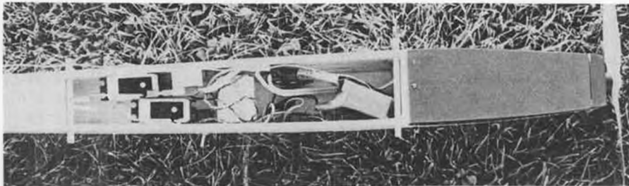
Radio installation in Oly 650 (l to r): elevator and rudder servos, motor push-push switch, airborne pack, receiver. Power batteries and motor in nose.
