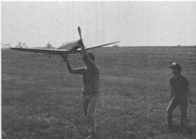
Leon Bennett launches his magnificent (90" span) DH Moth Minor. With 24 strands of 1/4-inch rubber, it weighs around 24 ounces. What a sight in the air!
