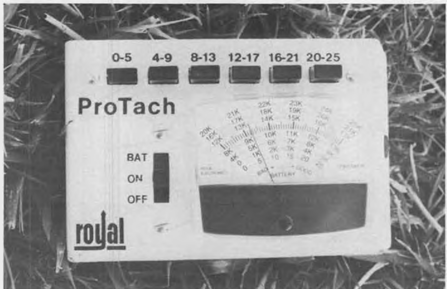
Pro Tach in use at the field. Main rotor being tached as quasi-governor is advanced from idle . . . 1,240 rpm indicated.
