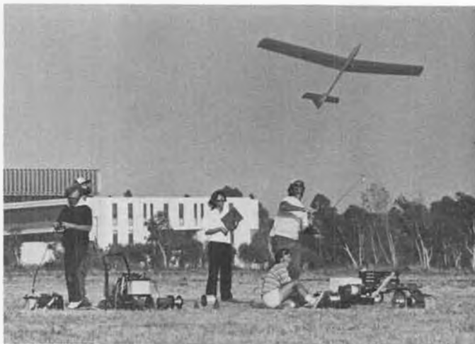
Trent McGee launches his Eismann "Camaro" during early round of semi's. Wortmann Fx 60/100 airfoil. Molded F/G skins . . . hollow.
