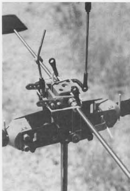
Complete head ready for balance check. Hiller rod and simulated collective rod left on head. Note high angle on collective yoke . . . 9-1/4° pitch needed for hover at 7,000 ft.! Low pitch set at 2-1/2°.
