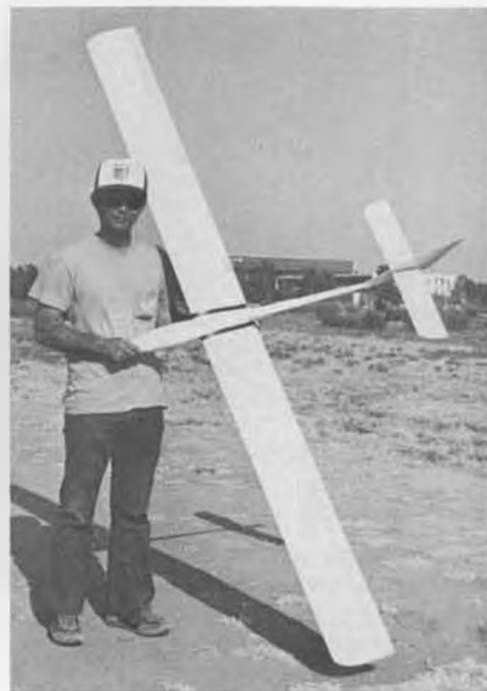
Steve Kaneshiro and his Eismann "Focus", which he modified by installing a wing joiner box around the joiner tube. E-387 airfoil.
