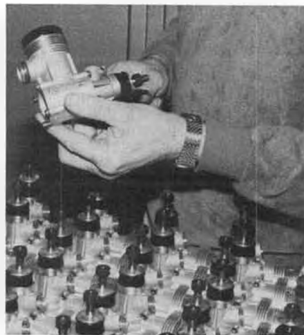
Ugo Rossi holds rear exhaust version of new .61. The .61's on table are side exhaust versions of this tuned pipe engine.
