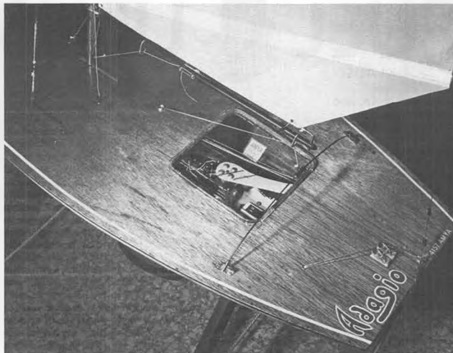
With hatch cover off, note winch, arm, and winch control servo. Note American Model Yachting Association hull registration inside hull.
