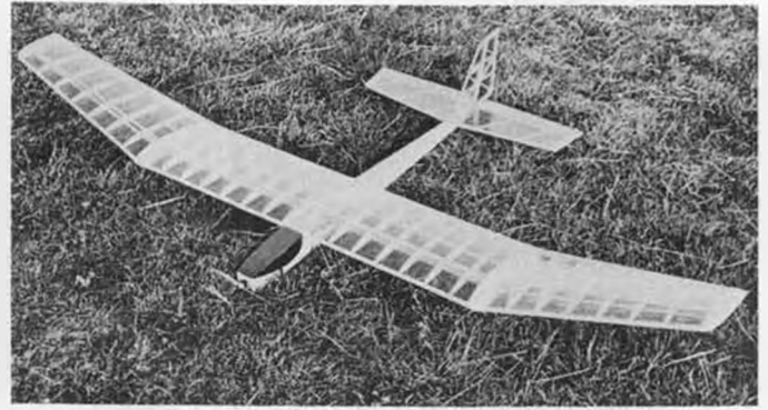
The Airtronics Olympic 650, as reviewed in this column. Parts fit extremely well and framework is strong. This one covered in transparent yellow Solarfilm. All up weight, with Astro 05 XL, is 46 ounces. Span is six feet.
