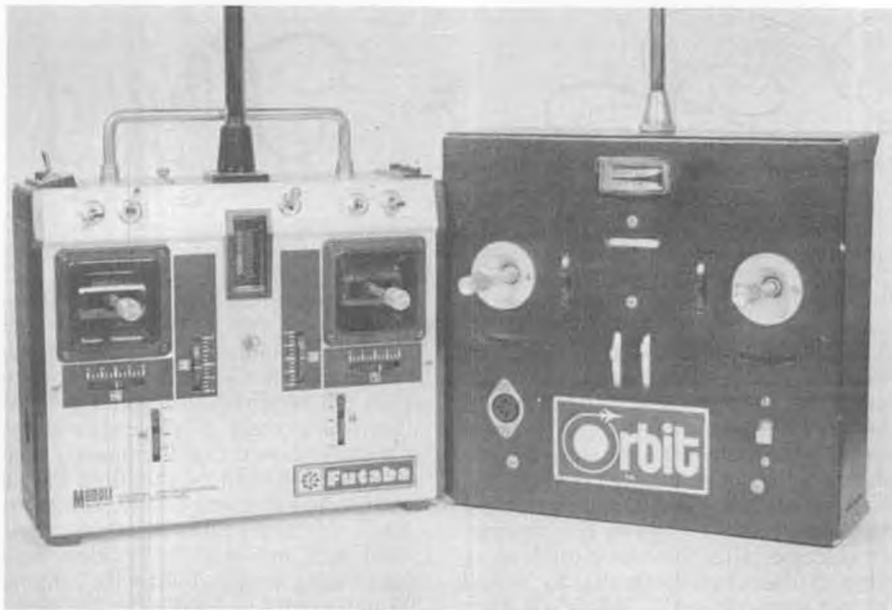
With just a few mods, older 27 MHz transmitters can become reliable 6-meter units, though lacking many of the modern bells and whistles. See text.
