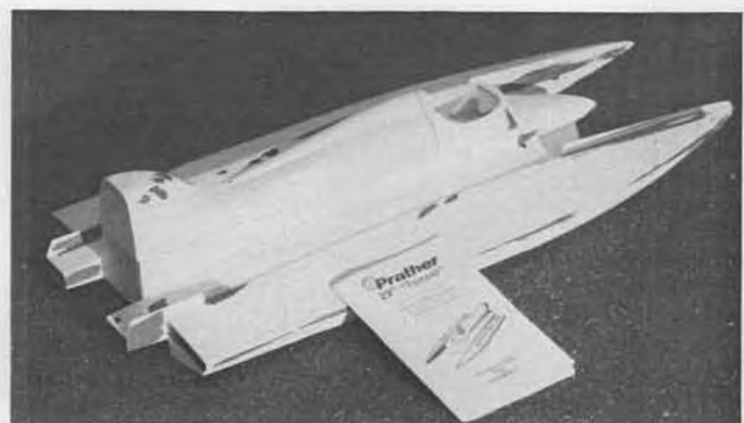
Automobile spot and glazing putty applied to Prather 3.5 Tunnel after the boat was primed.
