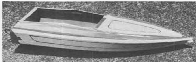
Masking tape is used to cover the areas that have already been painted.
