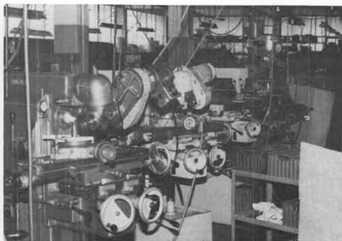
Several of the milling machines used to machine the ports in the sleeves of engines.
