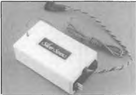
Five-Channel receiver shown — one to seven channel operation possible. Dean's connector version available with either End-Block or Pig-tail-type connectors.
