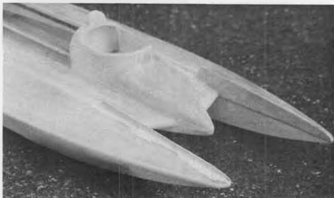
Automobile body putty used to fillet wooden air dams added to Prather 3.5 Tunnel.
