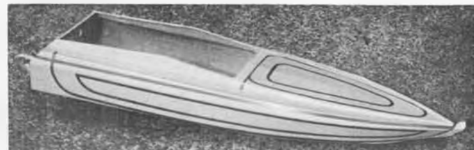
Flex-Mask is used to define color separations on this Offshore 33. Base coat is yellow, with color panels of orange and red.
