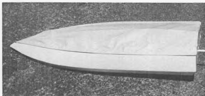
Plain paper is used to cover bottom of this Offshore 33 to protect it from overspray.
