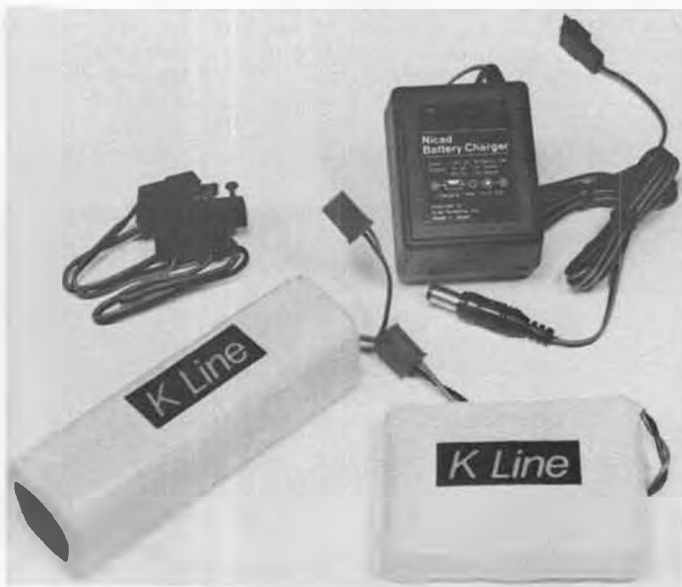
NiCd conversion pack for Kraft K-Line radio system. Receiver pack is five-cell unit . . . what the serious racers want.
