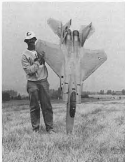
Phillip Avonds of Belgium deserves to smile about this F-15 Eagle; it placed sixth in the world scale champs, despite inconsistent engine runs. Model features twin K&B 7.5s in modified Turbax fan units.
