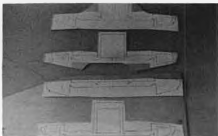
One way of transferring the plans to the plywood is to use a spray adhesive. The frames are cut out and the plans then peeled off.
