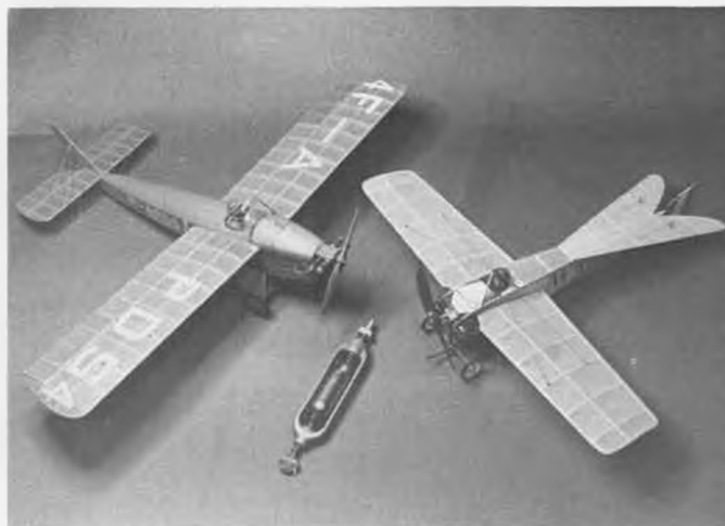
Two of the author's CO 2 models. On the left is the Brown Junior .005-powered Farman F.451, winner of the Open Free Flight Gas Scale at the 1977 Nationals. On the right, a Nieuport monoplane powered by a Brown Junior A-23 Peanut engine. Between the models is the only ground support equipment needed: a CO 2 capsule and charger.
