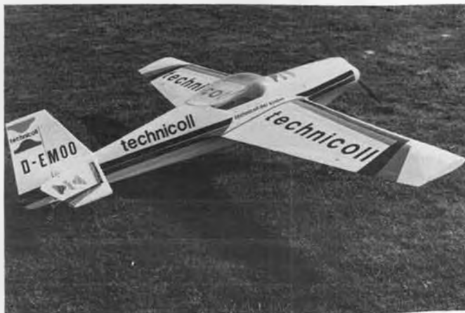
A 99-inch span Diabolo, powered by a 3.6 cubic inch AMT King. It weighs 18 lbs., and is suitable for aerobatics.
