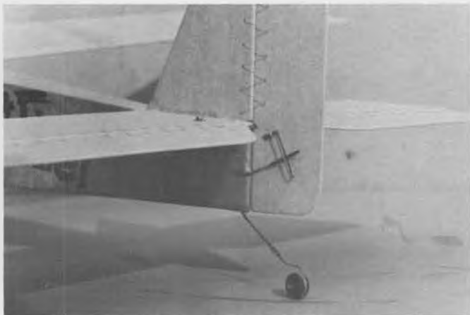
Rudder control on the Flier. Author used Ace Pulse Commander for control, on-board weight only 2-1/2 ounces. Keep it light!
