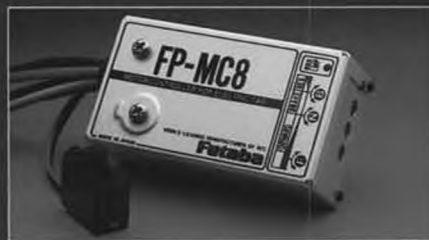
New FP-MC8 electronic speed control. Proportional forward and reverse, with adjustable braking. Capacity: 7.2v/20A (30A surge).
