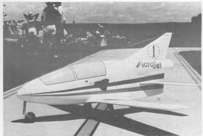
A huge 1/2-scale BD-5J, designed and built by Jim Werst and Kerry Sterner. The model is powered by a Byrofan/Rossi combo.
