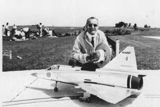
Col. Bob Thacker and his SAAB Viggen. This model is powered by a Byrofan/Rossi .81 propulsion unit. It represents a 10.5% scale model, and flies at 13 pounds.
