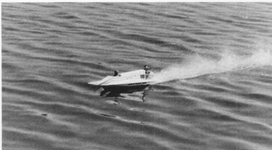
This 11cc tunnel boat was designed specifically for the K&B 11cc outboard motor. The tunnel boat has had considerable success, coming close to the 11cc oval record running time.
