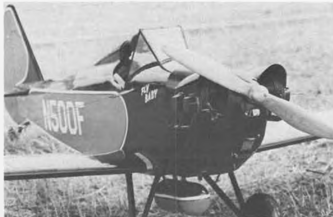
Take a look at how natural the Gemini Twin 1.20 looks in Austalian Lloyd Dipple’s Fly Baby. The model is 1/4 scale, and Lloyd made the extra cylinder head covers from a mold made from the originals.
