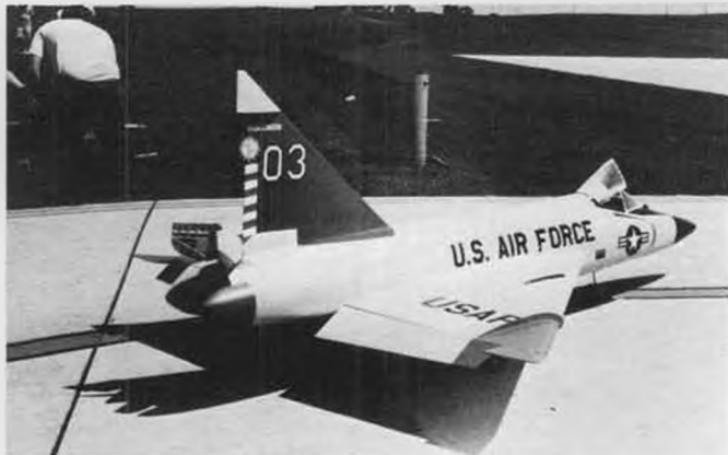
Ivan Munninghoff's latest design, an F-102A delta fighter patterned after the Convair aircraft. Model featured functional speed brakes, completely detailed cockpit with opening canopy.
