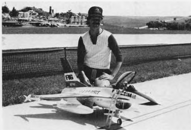
Scott Forster's highly detailed F-16A from the Byron kit. This model features functioning gear doors, full cockpit detail, and a boarding ladder for static display.
