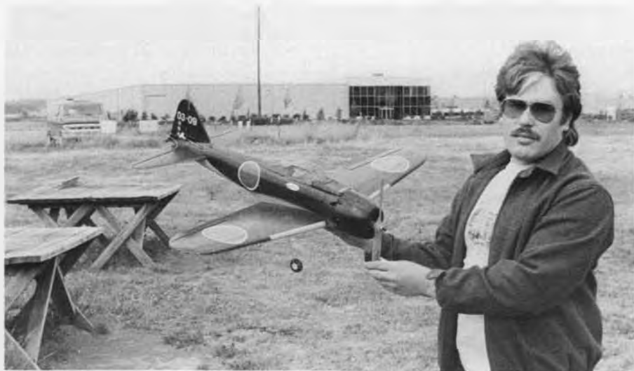
The unknown flier and his electric Zero. With an Astro cobalt 05 for power, it flies real fast—but sinks rapidly when slowed up. Flies like a gassy, fast and aerobic.
