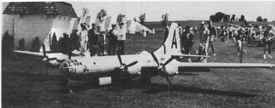
Look out... expected to be flying in August, the Byron Factory's B-29 will weigh around 450 pounds when completed, with power by four gas engines swinging four-bladed props. Yoww!!
