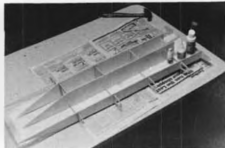
Cowling frame is added to the framework. Use of thick instant glues is recommended.
