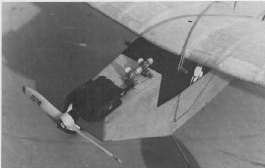
Motor is an Astro 020, connected to the circuit by a 10-amp fuse. This makes a simple on-off switch, and protects the motor armature as well. A simple and clever solution.
