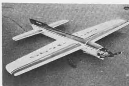
No. 2863 VOYAGER $5.00 C/L Aerobatic Stunt Champ for .40-.46-size engines. 64" span. By Piotr Zawada.
