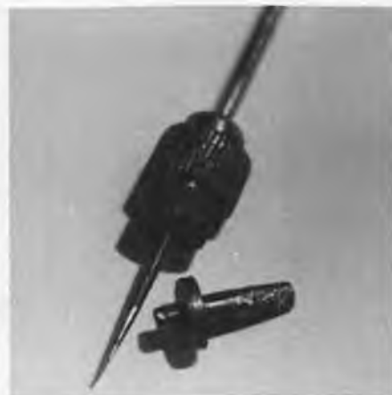
The MK-12B's needlevalve has a soon-to-be patented hook on its end to catch pieces of dirt from the fuel.
