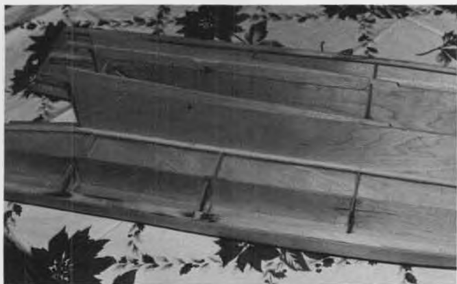
The rear sponson frames are attached to the rear cowl using 4-40 bolts and blind nuts. The top to the rear cowl is then glued in place.
