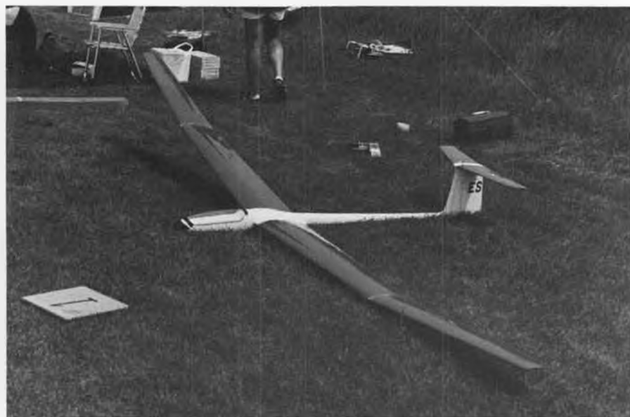
Stan Watson's Pegasus with modified NACA 4412-R412C. At 184-inch span it's one of the biggest; 22:1 AR; dry wing loading 16 oz/ft; no flaps or spoilers. Completed the Great Race 76 km course first time out during initial testing.
