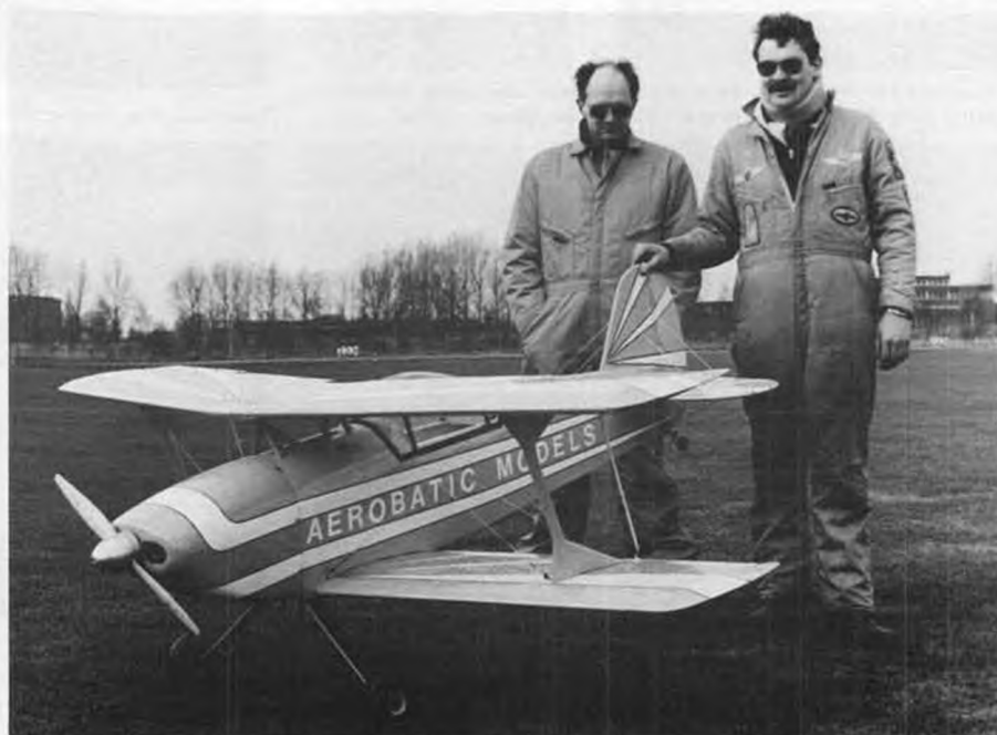
Menke Knol and Willem Wolterink, builders of the 92-inch Reed Falcon. Built from a 3-view from a German magazine, the ship weighs 26 lbs., is all wood, with foam ribs, and is powered by a 4.8 cubic inch engine. Colorful finish is Super MonoKote.
