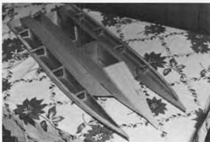
Front cowling of 1/2-inch balsa shown ready for shaping to final form.
