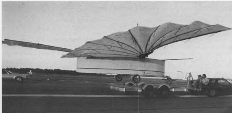
The Whitehead reproduction in tethered flight during pitch and roll stability tests at about 35 miles per hour, behind tow car. See text for details. Photo: O'Dwyer.
