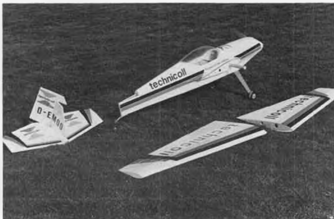
The Diabolo again, and no, it didn't crash! It disassembles easily for transport. All wood construction, except foam ribs, by Menke Knol.
