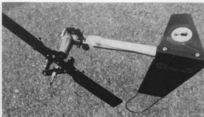
The most expensive component in the Cricket is the tail rotor gearbox, a well built, all metal unit. Tail fin is pre-shaped aluminum sheet.
