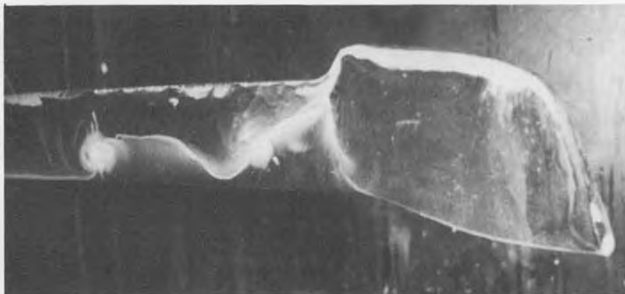
A model BERP blade in a wind tunnel oil flow visualization test, at a 12° angle of attack. Oil accumulation indicates where the air flow has separated from the blade.
