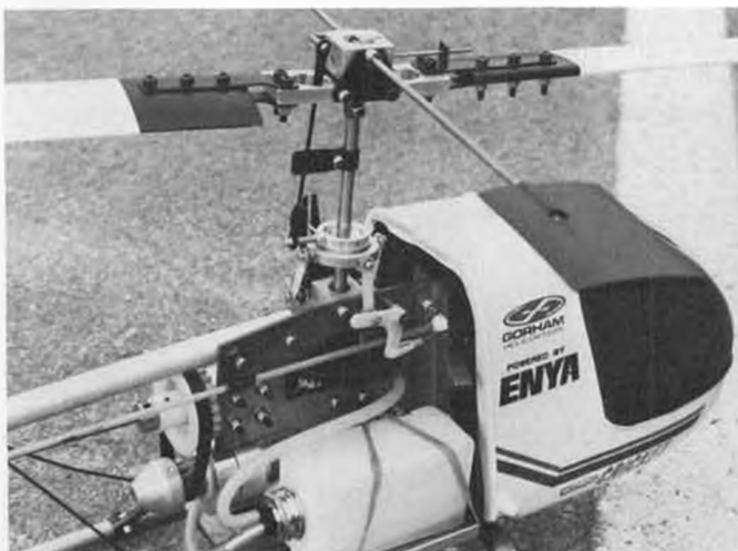
Fuel level is easily visible in side mounted tank. The Cricket uses a teetering main rotor head design; the teetering spring on the right side of the rotor head provides flap stiffness for improved control response.
