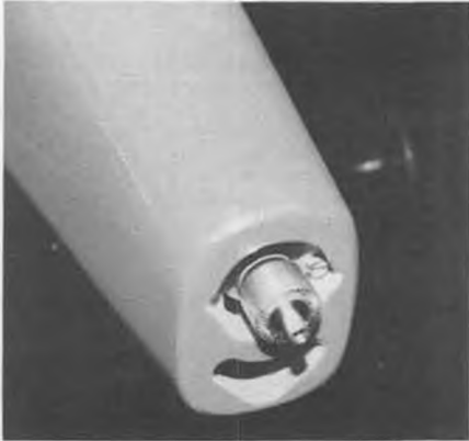
Front view with the prop and spinner removed shows the aluminum prop adapter mounted on the "Goldfire" electric motor, which is included as part of the Electro Streak kit. The bottom hole is an inlet for battery cooling air.
