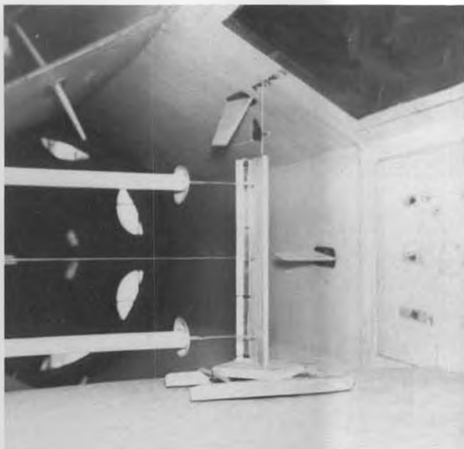
A wind tunnel model of CL Max undergoing tests at the University of Washington. Multiple trailing edge flaps showed best results.
