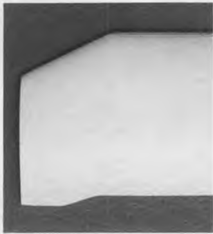
British hell filer Len Mount uses a small tab on the trailing edge of his blades and claims they are noticeably quieter.
