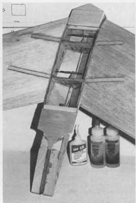
The fuselage skeleton, ready for sheeting with plywood and the installation of balsa nose and tail blocks. As our reviewer learned the hard way, this is a sturdy structure that can stand up to abuse.
