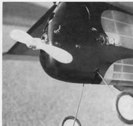
The well known stubby Pacer nose. The engine is one of Otto's early ignition conversions, a hot K&B .35 with points on the rear. ●
