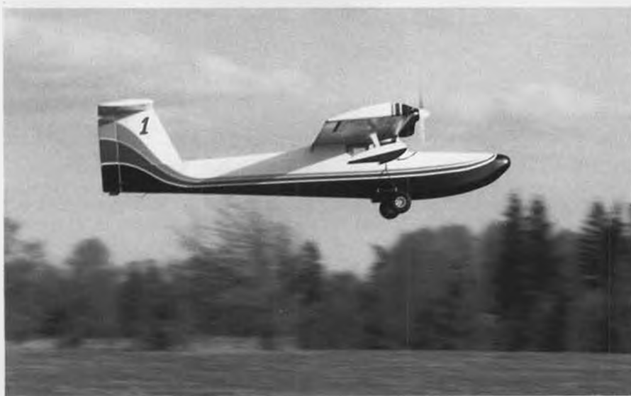
The prototype Seasport II is fitted with a removable landing gear for dry-land flying. This is detailed on the plan, but dyed-in-the-wool seaplane fliers may want to leave the gear off altogether.
