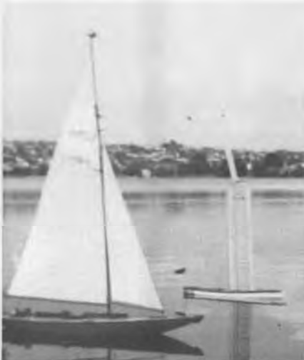
CL Max competing (make that "drifting") with the then National Champion conventional sailboat. The wing sail area was limited by the yachting rules to only a fraction of that allowed for cloth sails.
