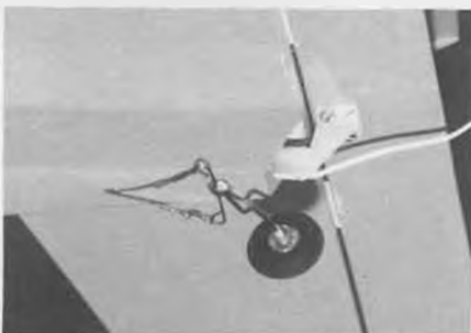
Our reviewer also chose to install a steerable tail wheel, controlled by cables from the rudder servo. Light, clean installation.
