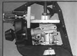
Motor is angle mounted for easy starting and transfer of power to the rotor blades.
