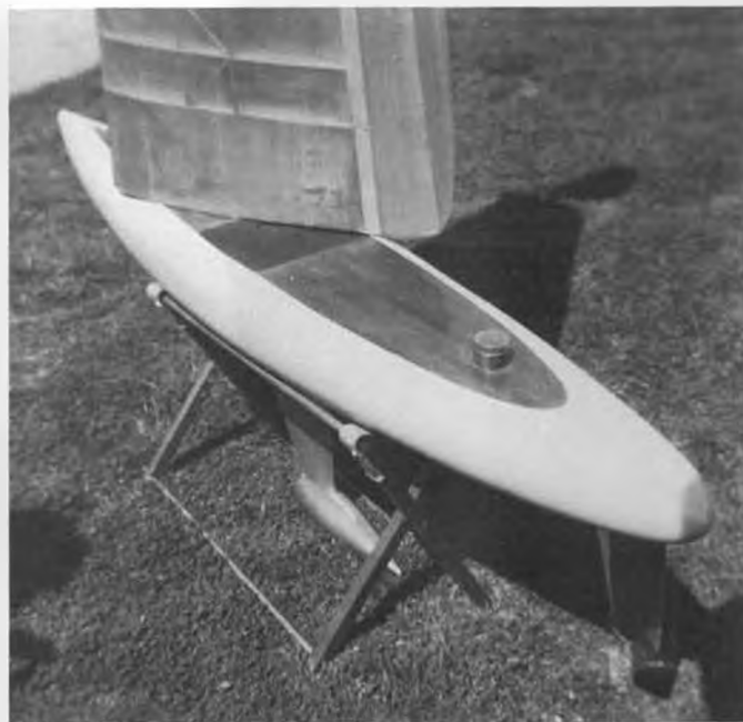
The "boom" or bottom of the wing sail seals against the deck to prevent air passage and subsequent loss of lift.
