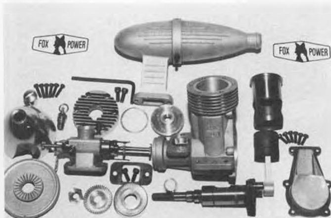
All the parts laid out for inspection. Cylinder's bore is .800 inch rather than .835 like other Fox .40s. Stroke is longer and the engine is comfortable turning 11x6 and 11x7-1/2 .60 size props.
