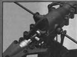
The enclosed construction and smooth surface of the rotor head allow a freely rotating head to be stopped safely.
