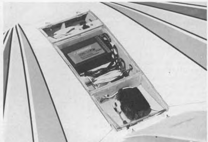
A view of the radio compartment. Receiver battery goes under the receiver, flap servo is at the back. Aileron servos are in the wings.
