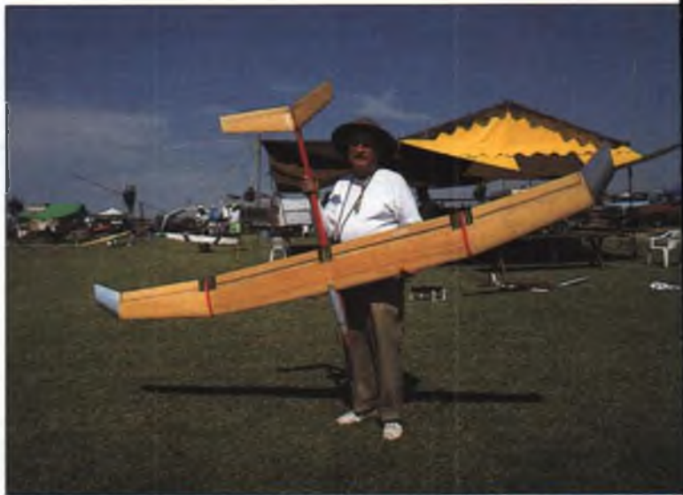
Al Doig (former RCM soaring columnist) and his original design "Slippery Hollow" V-tail, "The best flying sailplane I've ever owned. It is a gentle handling model that thermals beautifully." Ship weighs 85 ounces, SD7037 airfoil, 1026 squares, NASA sweep at tips, lots of carbon tow, C/F tailboom, V-tail mixing and electronic flap/elevator coupling.
