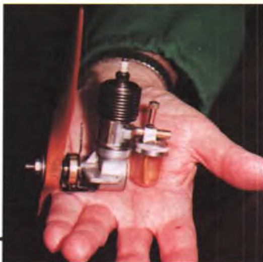
Photo No. 3. Nice example of a Junior Brown Junior, the featured Engine of the Month, as turned out by Bill Hofstetter from one of Roger Schroeder's casting kits.
