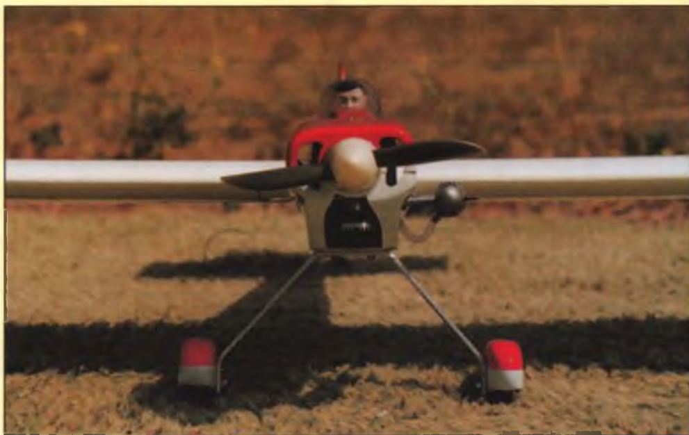
Wide-track landing gear makes for excellent ground handling. Engine is fitted with a 1-1/2 inch Goldberg plastic spinner (later changed to a Cermark aluminum splener to add nose weight) and an APC 7x4 prop. Also, an extension was needed to get the muffler to clear the cowl. Art recommends mounting the engine on its side so as to put the muffler on the bottom, which should do away with the need for an extension.
