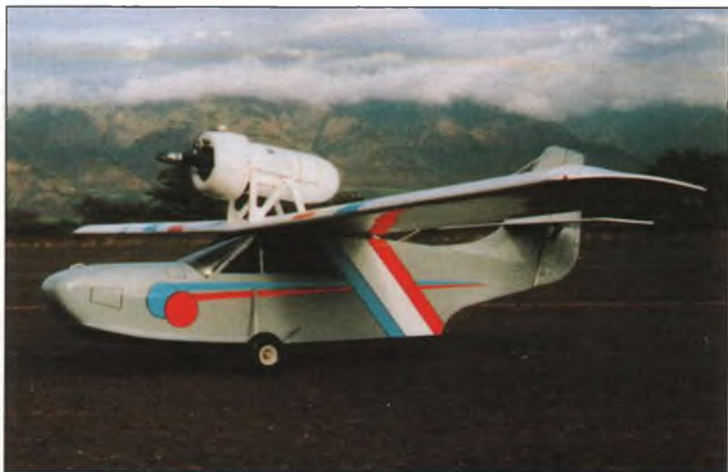
■ TOP: Engine nacelle is made mostly of plywood and hardwood; cowl and rear fairing are from soda pop bottles. Nacelle holds the engine (in this case, an O.S. .35 FP), fuel tank and throttle servo. ■ ABOVE: For land operations, the author recommends removing the tip floats (each is held on with two screws). Landing gear can be retracted manually for water flying; the front strut leg pivots in a tube, and the rear drag link fits into one of two holes in each side—the lower hole for gear down, the upper hole for gear up. Tail wheel also gets replaced with a water rudder for water flying.
