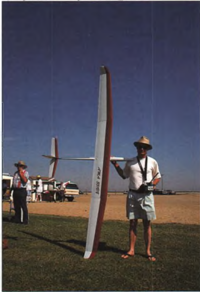
The prototype DCU Windstorm thermal competition sailplane as flown by Jim Parsons. Model will soon be commercially available. Triple-taper wing is 116 inches long, molded hollow core with Rohacell/fiberglass sandwich skins, SD7037 airfoil, slotted flap linkages to prevent ballooning, and vacuum-bagged stabs.
