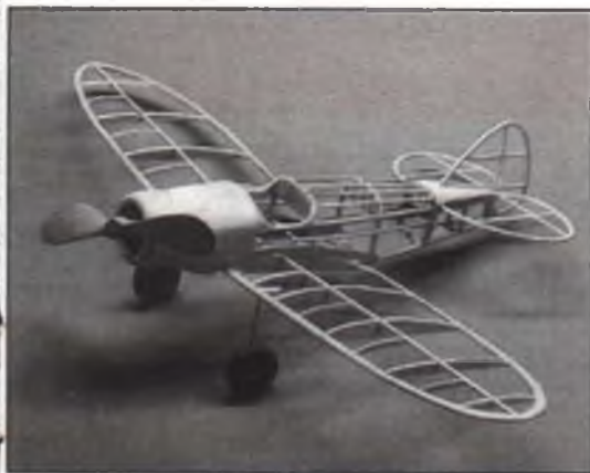
The author's Monoprop "in the bones." The landing gear is scale length and wheel diameter, there being no hope of making a presentable extension for R.O.G. takeoffs with a flying propeller. This model used cut sheet balsa wingtips and bent basswood laminated tail surface outlines.
