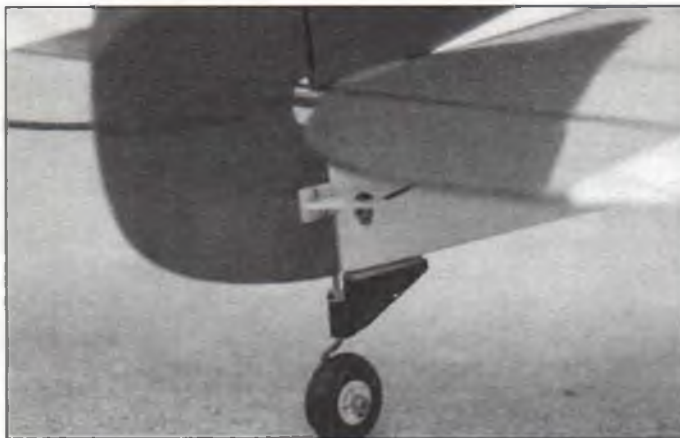
The tail wheel wire with hinge bearing supplied in the kit was replaced with a Du-Bro tail wheel assembly so that the load is carried by the fuselage, instead of the rudder hinges.
