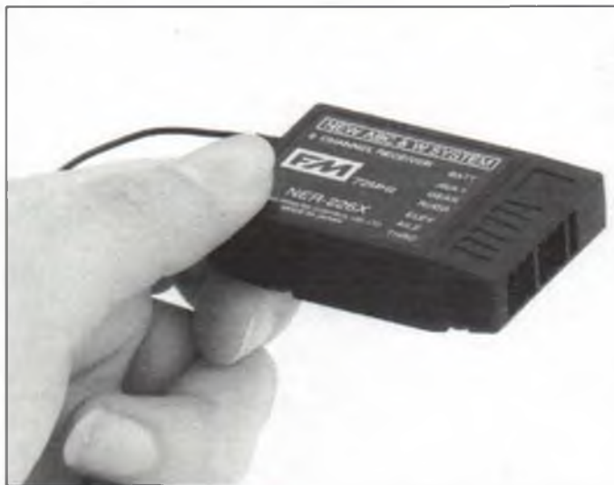
Things they are a-shrinking! Seen here is one of the new JR "Credit Card" receivers. Considerably smaller than previous JR receivers, which are comparable in size and weight to many other available brands, these little nine-channel marvels are available in PCM and FM versions.
