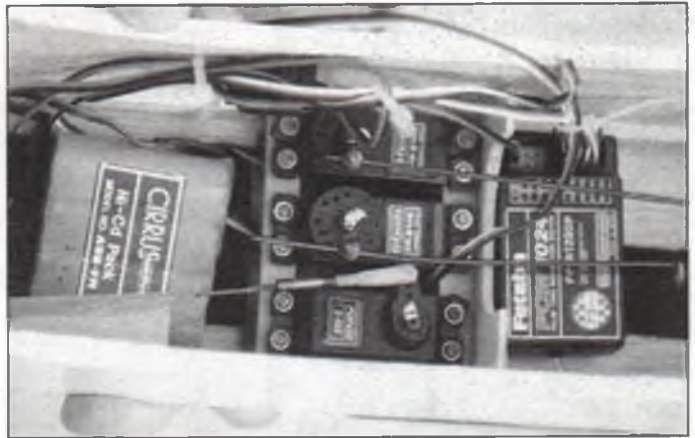
Fuselage is wide enough to take three standard servos abreast with room to spare. Radio used is a Futaba 7UAPS PCM. Aileron servo is mounted on hardwood rails in the wing center section.
