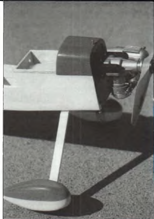
The Stinger 10's fuselage is a simple all-sheet-balsa box with molded ABS plastic turtledecks fore and aft. Wheel pants and cowl are also ABS plastic.
