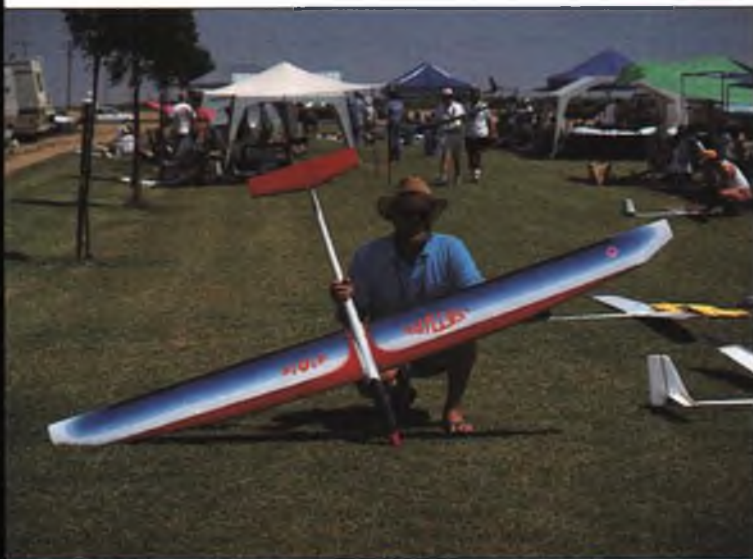
Brad Clasen (11th North, 24th overall) absolutely loves his new Layno/Urwyler Saturn 2.9T. He says he likes everything about it—great launch height, thermals well, Quabeck 2.8/9-2.8/8 airfoils, won't tip stall, no bad habits. Quite an accolade from a very accomplished contest flier!
