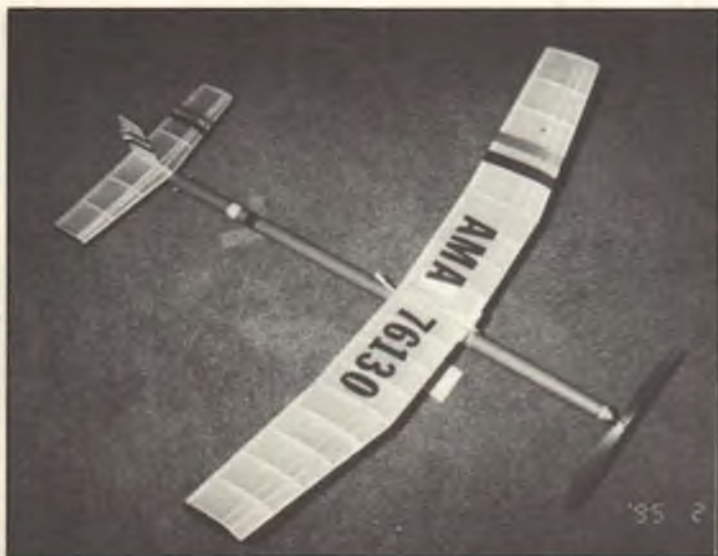
One of John Kamia's P-30 models, a Len Sherman design that features a 1/32 rolled balsa tube fuselage. John flies it on four strands of 1/8-inch FAI Tan II and gets 1,600 turns into the motor. Like Dave Linstrum, John finds the wing-mounted DT to be a very positive way to bring the model down from those boomer thermals.
