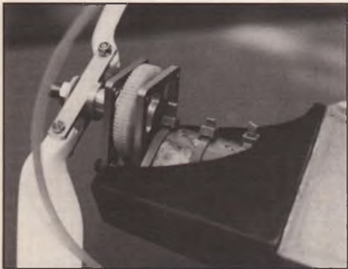
Close-up of the business end of Jerry's Lanzo Bomber showing the 17-turn Trinity car motor and a 7:1 Superbox from Model Electronics. Jerry reports needing very little throttle to get this bird in the air and he has extra power available if needed.
