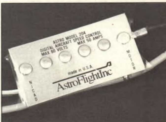
Astro Flight's Model 204 electronic speed control is one of that company's new series of digital ESCs; it's good for up to 36 cells and 50 amps. A companion unit, the 205D, is identical in size and performance but incorporates a propeller brake for electric sailplane fliers.
