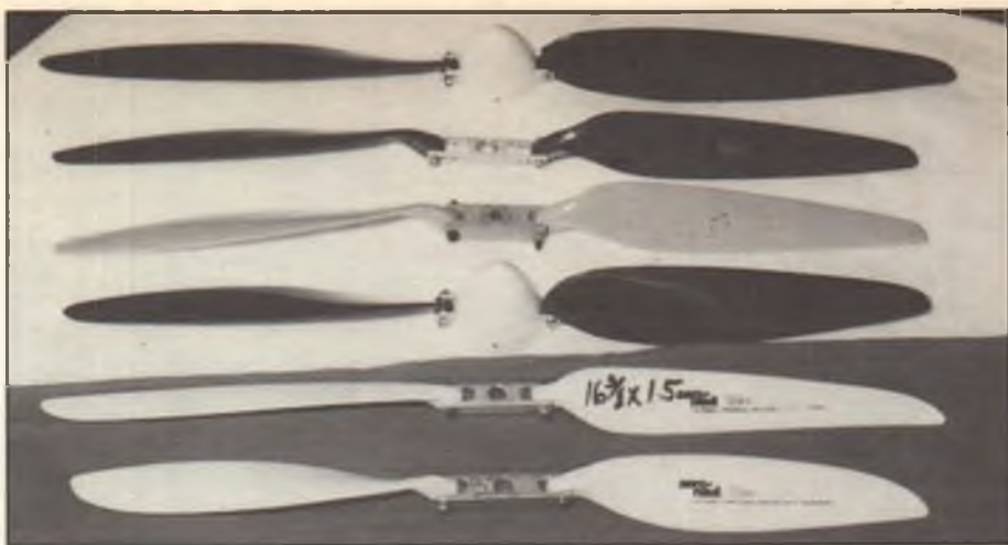
Jerry's propeller assortment, from top: a 18x18 Schöberl (German), 17x12 RASA (British), 17x10 RASA, 16x16 Schöberl, 16-3/8x15 Aeroant (German), and a 15x9-1/2 Aeroant.
