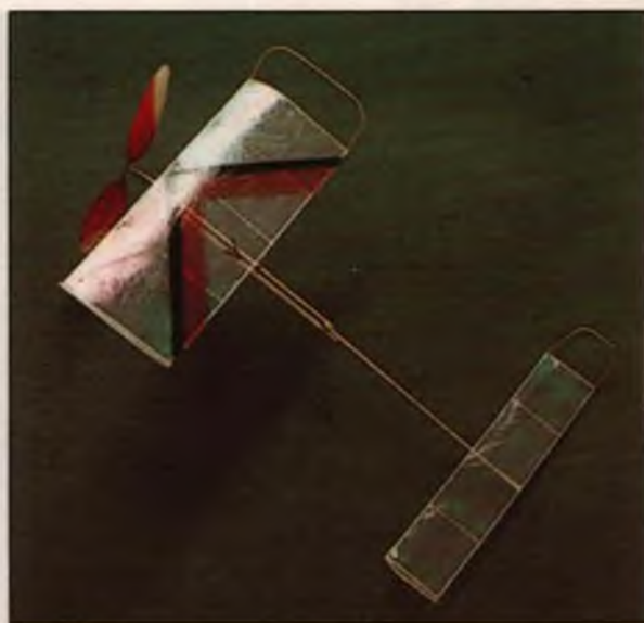
■ LEFT: What looks like microfilm covering is actually a super-lightweight type of Mylar called Polymicro; text tells where to get it. Rules limit Mini-Sticks to wood props and plastic/paper coverings only. ■ ABOVE: Another version of the Libelulae. This view emphasizes the long tail moment and 7-inch span stab (same as the wing). Maximum allowable stab area is 50 percent of the wing area. The smooth covering is Polymicro that has been crinkled and then ironed smooth; the author says it's easier to handle and is stiffer.
