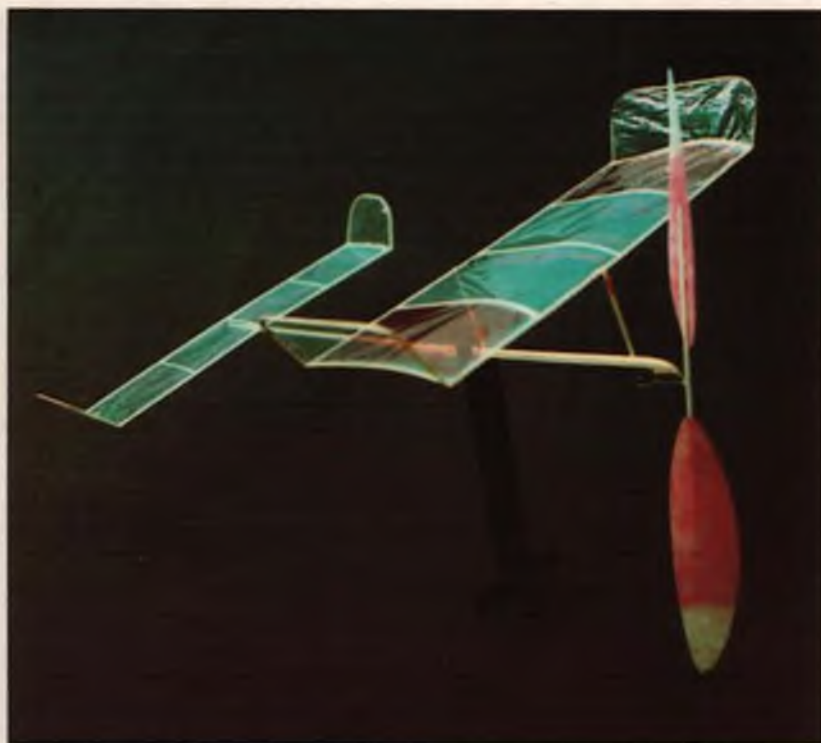
■ LEFT: What looks like microfilm covering is actually a super-lightweight type of Mylar called Polymicro; text tells where to get it. Rules limit Mini-Sticks to wood props and plastic/paper coverings only. ■ ABOVE: Another version of the Libelulae. This view emphasizes the long tail moment and 7-inch span stab (same as the wing). Maximum allowable stab area is 50 percent of the wing area. The smooth covering is Polymicro that has been crinkled and then ironed smooth; the author says it's easier to handle and is stiffer.
