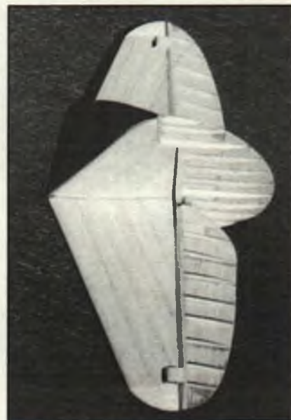
Fixed portions of the tail surfaces are fully sheathed; the elevators and rudder (and ailerons too) have a sheet balsa core with ribs on both sides, to simulate the fabric-covered control surfaces on the full-size aircraft.
