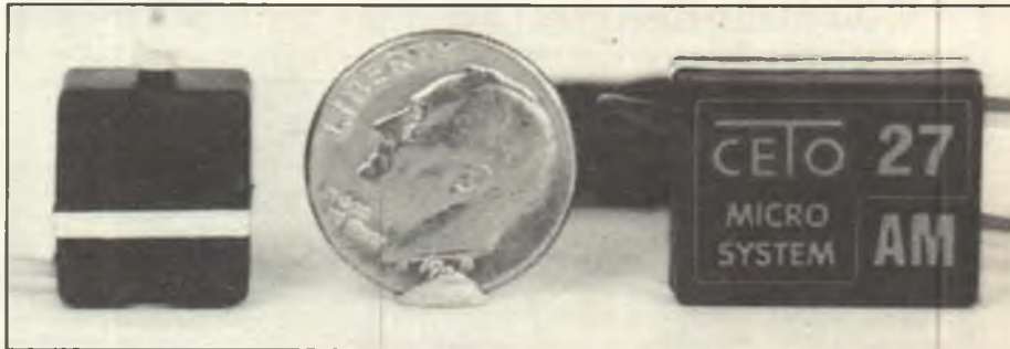
Probably the world's smallest receiver and servo, seen here with a dime for size comparison. Actual dimensions and weights are given in text, along with battery requirements.
