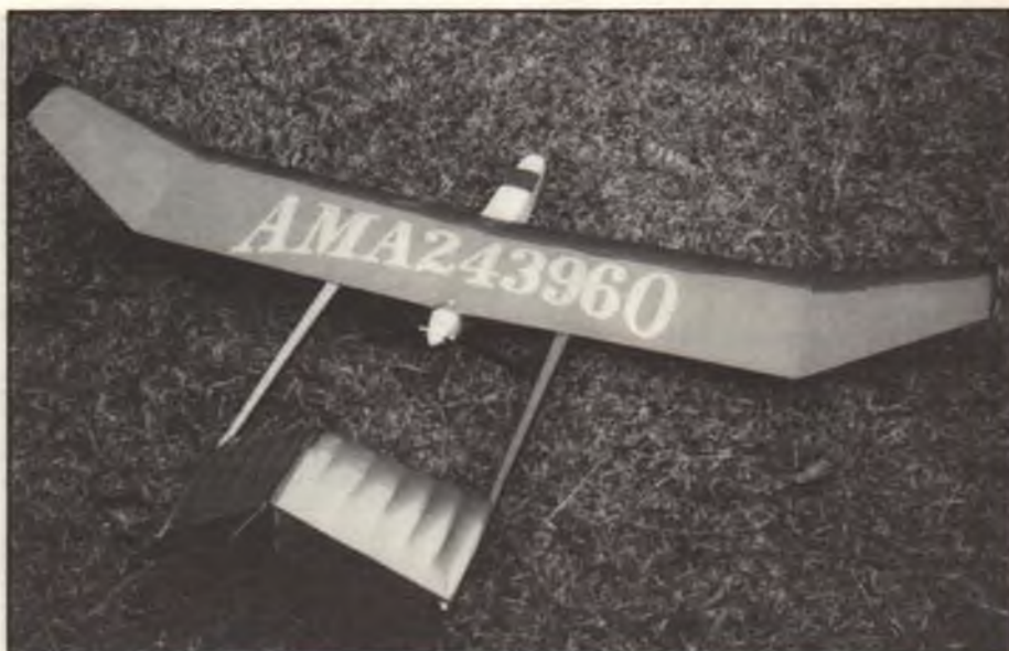
Novel inverted V-tail pusher duration aircraft by Mike Finnan of Covington, Louisiana. Wingspan is 72 inches, wing area is 800 square inches, airfoil is an Eppler 362. The V-tail angle is the normal 110 degrees. Ready-to-fly weight is 4 pounds. Motor is a Graupner Speed 600 00 12V with a Leisure 3.8:1 long shaft gearbox. The battery pack consists of 12 1700-mAh SCRC cells wired in two six-cell packs. A servo operates a series-parallel switch and an on/off switch for throttle control. Propeller is a 15-inch Master Aircrew.
