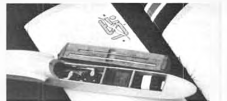
Wing joiner pins may be stored under canopy block. Snug fit for large R/C gear. Note LSF!
