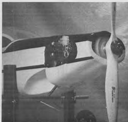
Once cowled in, the starter doesn't show. Black tube is crankcase vent.
