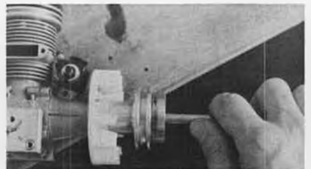
... then adjustments can be made by slipping a brass tube over the shaft and applying hand pressure to bend in desired direction.
