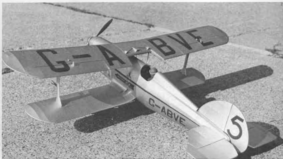
One of the author's favorite models is this Arrow Active biplane powered by an .06 Taifun German diesel. Model weighs 17 oz, has pendulum control, painted with silver Floquil.
