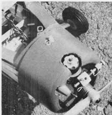
Cowl in place, wing and windshield removed. Throttle servo in fuselage's right side, receiver minus plastic case on left side.
