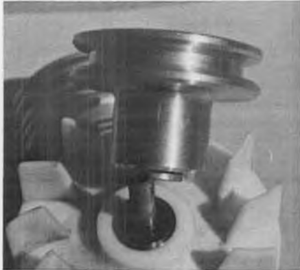
Cone start system fixes to eliminate vibration. Note how bottom of aluminum spacer is machined to fit fan recess. Centers automatically.
