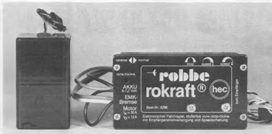
The Robbe Rokraft (Model No. 8298) is one of Robbe Modelsport's many variable speed controls. This device proportionally controls electric motor speed according to throttle position.
