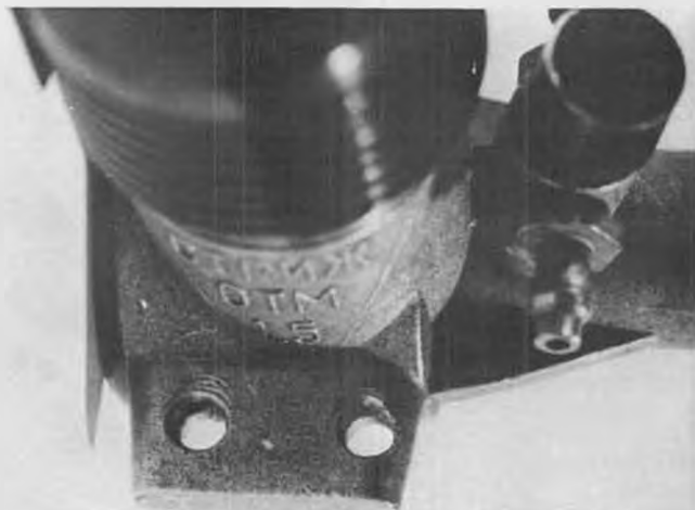
Notice the slightly off center mounting holes. This shows an apparent lack of manufacturing tooling and jiggling. The author only gives this month's engine a "2" in manufacturing excellence.
