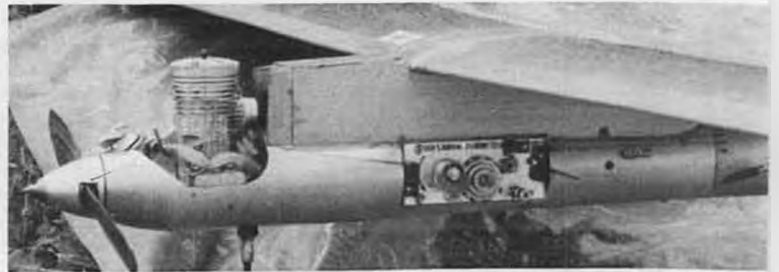
Here's another Chinese F1C plane with a Chinese made engine. Note Seelig Timer for engine cut-off, autoruder, and DT.
