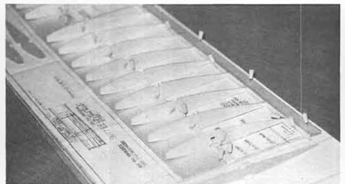
Wings are constructed rather conventionally. Airfoil is slightly curved on the bottom, so shims are needed at LE and TE for flat surface.
