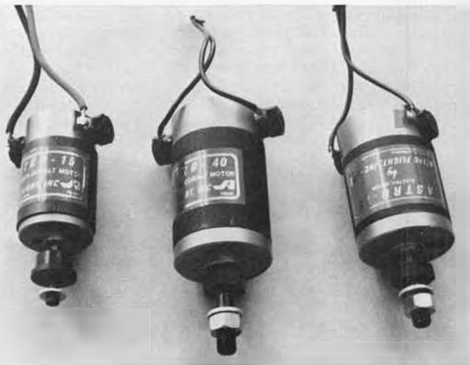
Astro motors. The author reports on static performance of the cobalt 15 (left) and Super Ferrite 15 (right). Cobalt 40 shown for size comp.
