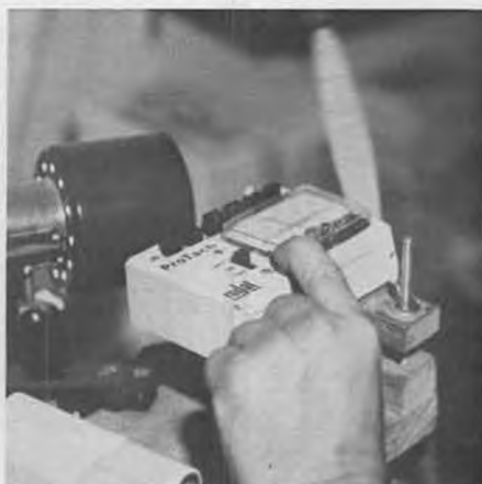
Camera almost stops prop as tach is used to test various prop and motor combinations.
