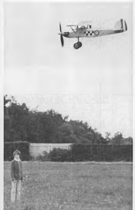
John Blagg's two-inch-to-the-foot scale Isaacs Fury Mk II is captured in flight over the Old Warden Aerodrome, England. Model is powered by 16 strands of 1/4" flat rubber. Model is still underpowered.
