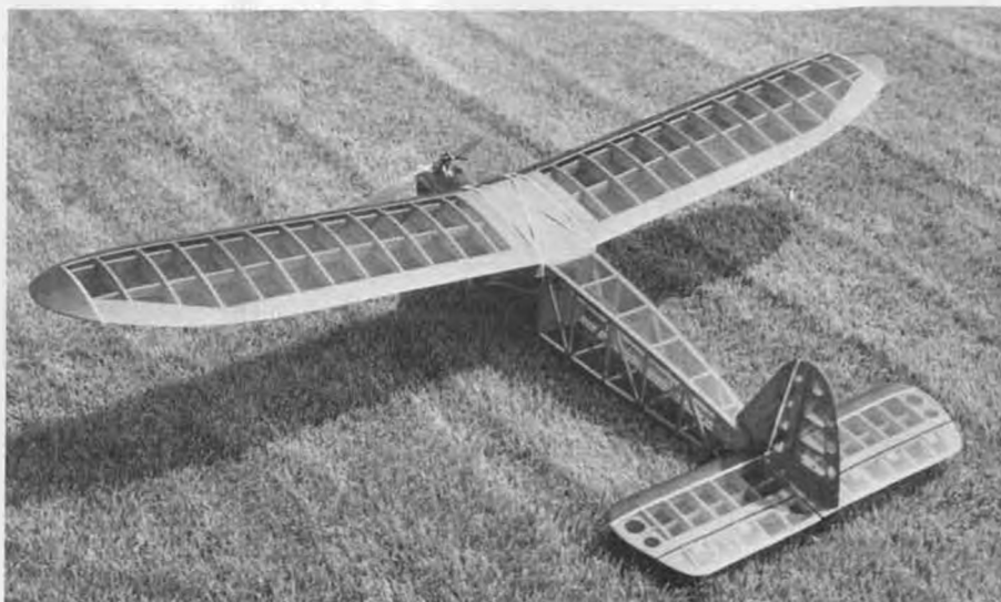
Wing and fuselage structure is clearly seen through the transparent red Monokote. Metallic green trim and silver striping tape really set this model apart from the "crowd" beautifully.
