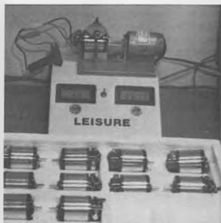
Dynamometer reveals current drain and rpm (3.89 amps and 15,190 rpm showing).
