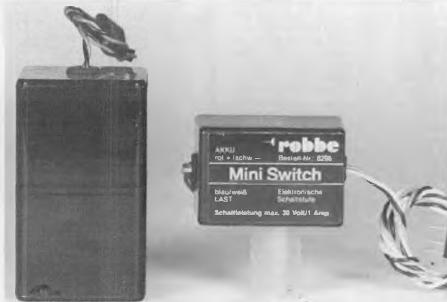
The Robbe Rokraft (Model No. 8298) is one of Robbe Modelsport's many variable speed controls. This device proportionally controls electric motor speed according to throttle position.
