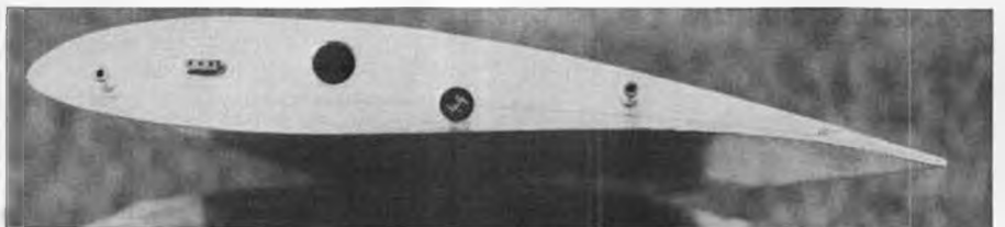
The Merlin sports a Wortmann airfoil (probably the FX 60-126 from the looks of it) which gives it a wide speed range for thermal hunting and climbing. Note aileron servo connector.
