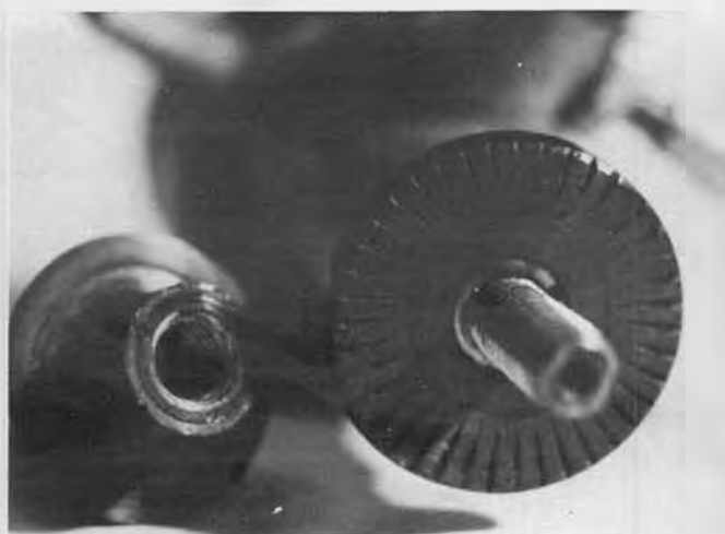
Another tell-tale sign of hand tooling ... was this done with a three-cornered file? This surface needs a lot more "grip" on the prop. The spinner nut requires the prop to be reamed out to 1/2-inch!
