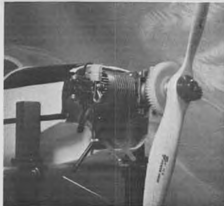
Enya .40 installation: clip provides glow power; white gear has free-wheel clutch allowing disengagement of starter and running engine.
