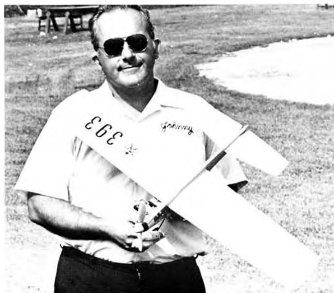
Sleeve bearing ST .35 powers Sport Racer by Johnny Tulach. Clocks between 90 and 95 mph.
