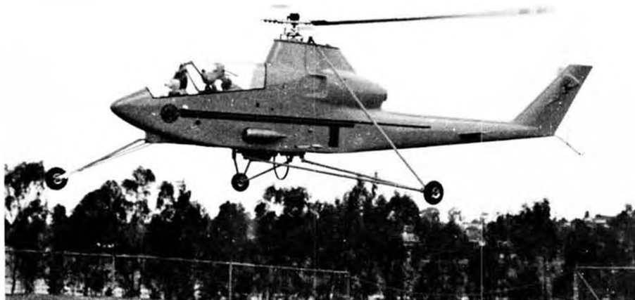
"Chopper Chatter" editor's Bell Huey Cobra, built from scratch. Model Helicopter's fiberglass fuselage, Schluter mechanics, O.S. Max .80, Orbit radio. Ship weighs 15 pounds!
