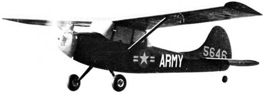
Fliteglas Models' new Cessna O-1E Bird-Dog is a combination stand-off scale and trainer. Has fiberglass fuse in olive-drab gel coat and foam wings precovered with 1/16 balsa. $49.95.
