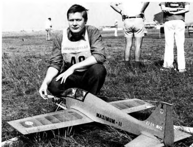
Norway's Poju (Pie-oh) Stephansen flew this ship in Doylestown and Gorizia. High fuselage profile nice for knife-edge maneuvers.
