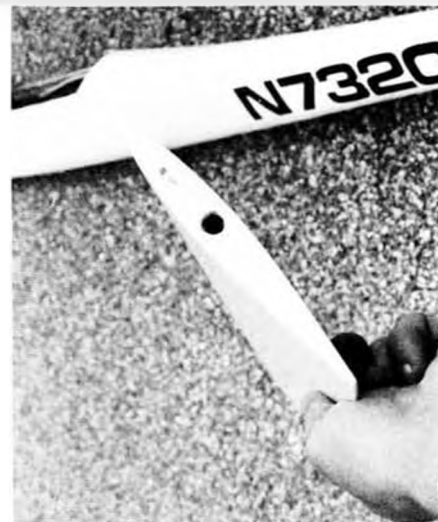
All-moving ruddervators plug into sturdy, 5/32 pivot rods. No slop a necessity!
