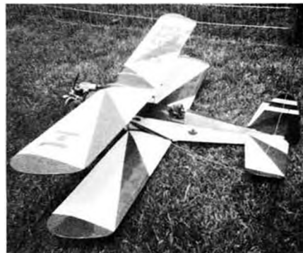
M. X. Carey's Galloping John, one of MB editor's many biplane designs. This one has OS .15 engine and OR 3 Ch. radio.
