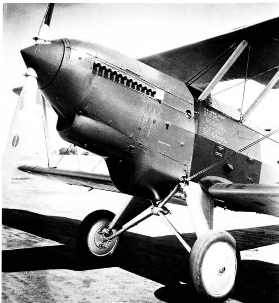
The clean nose, with oil coolers and Prestone radiator underneath, and the high thrust line, make the O-25C an ideal subject for modeling . . . rubber or gas. And, it's a biplane, folks!
