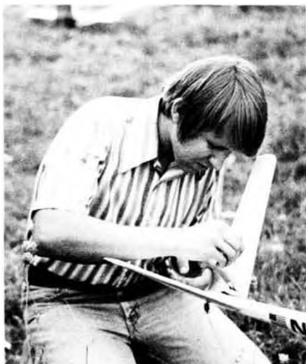
Author/designer/cover boy Niel Liptak hooks up the Quasoar's flying V-tail. Uses Todi link.
