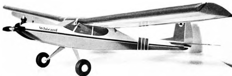
New 40-3/4 inch span "Whizzard" by Ace Radio Control. Foam wing with reinforced trailing edge. Tee Dee .049 power is plenty for one or two channel operation.
