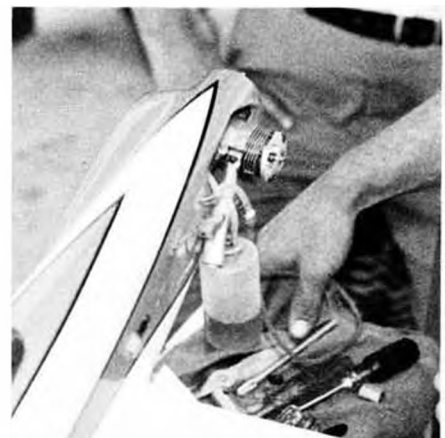
Terry Prather's ST X-40. Leverage of long exhaust pipe causes vibration problems.
