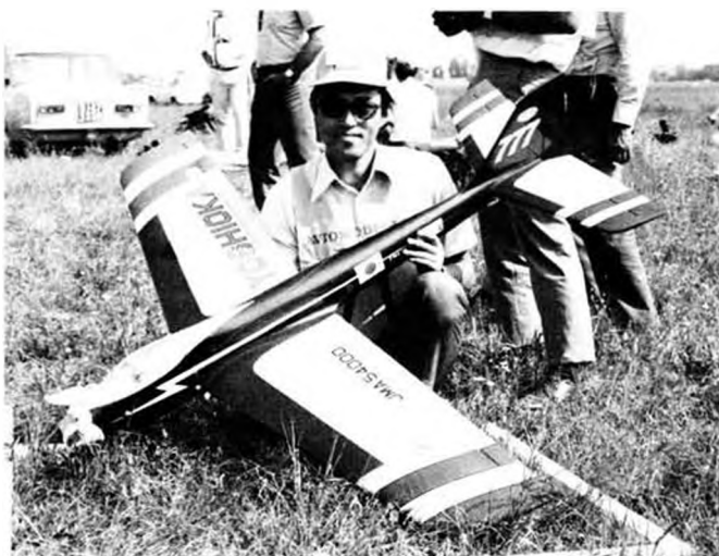
Champ Yoshioka with his Saber Liner. Japanese Digicon 6 radio. Enya 60 III had bored out, pressure regulated carb, used 45% nitro.
