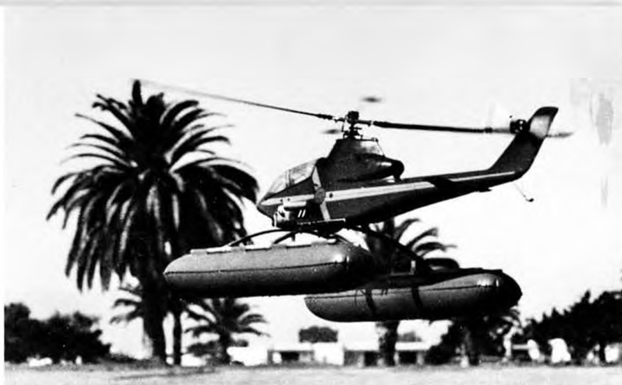
The Kalt Cobra, imported by Aristocraft, is powered by an ST .51, though a .45 is sufficient. Water test flights were made at the Model Yacht Basin, Mission Bay, San Diego, California.
