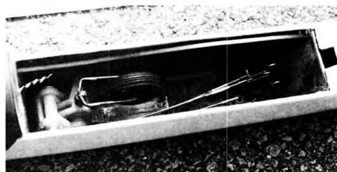
Goldberg nose gear retract unit is adapted for single wheel operation. For spot landing events, retract gear, put on double-stick tape skid!
