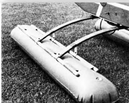
Close-up of float installation, showing adaptor brackets. Floats are vinyl.
