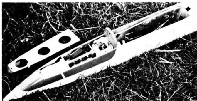
How's this for accessibility? Servos are mounted on a slide. Todd "Mixer" is in rear compartment. Hartman Fiberglass fuselage.
