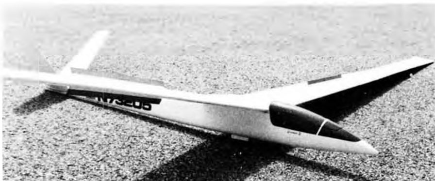
Spoilers and air brakes extended. Very useful control, once you get on to the knack of using it. They're made of stock K & S brass strips, direct from the hobby shop. Note retract wheel.
