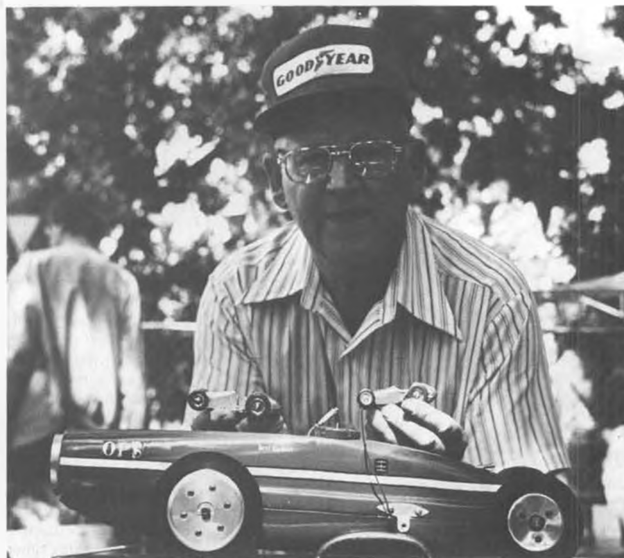
Bert Kuebler, Indiana, holds two table-top tethered cars that he built. They have .008 engines, and run 25mph! His OPS Class II car turned 168.54.
