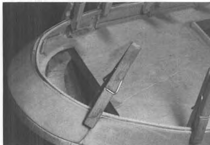
Bulwark has been added, now a strip of balsa or spruce is clamped in place to build up top for railing.
