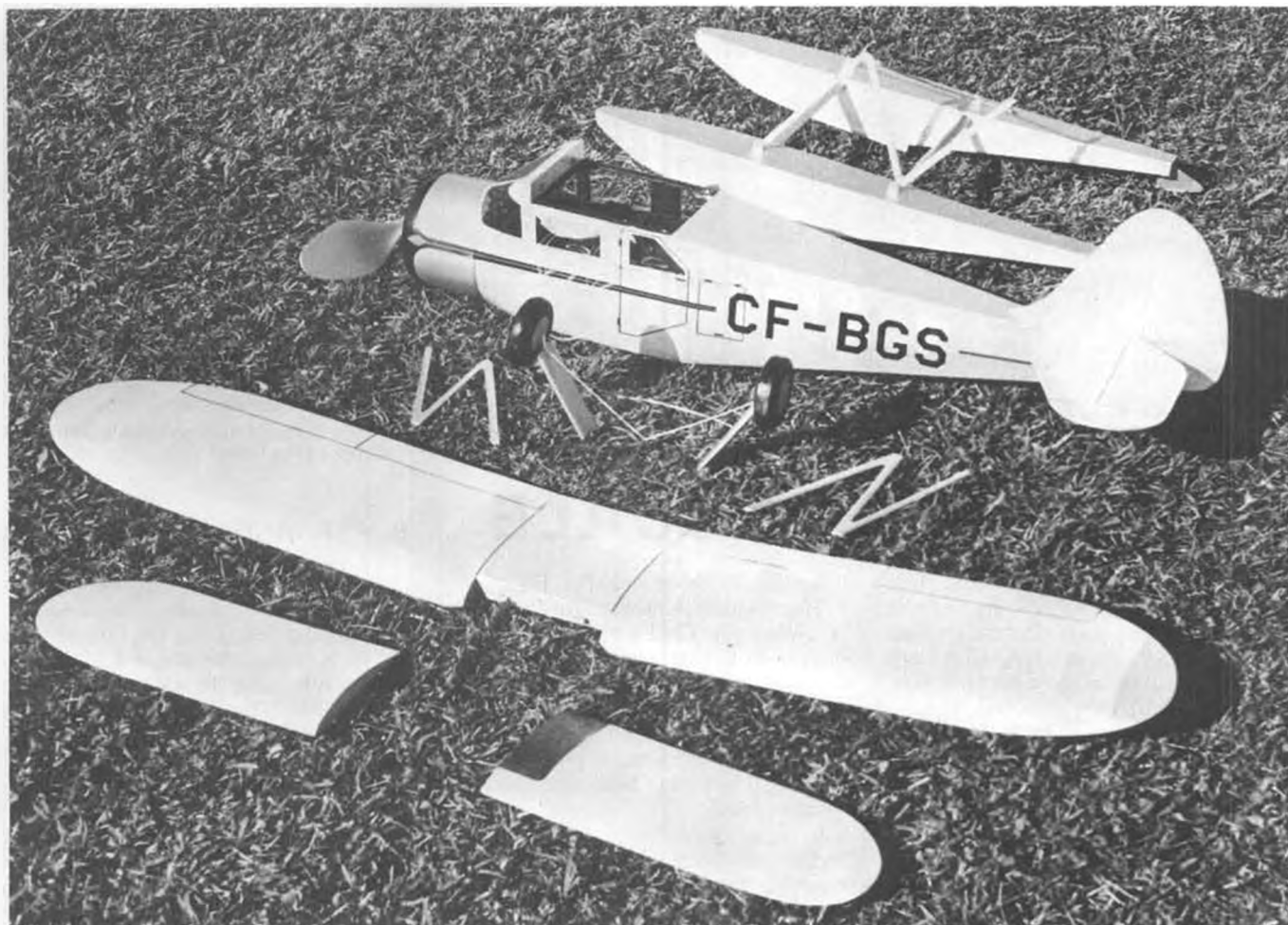
The Waco parts before "getting it all together." Building a model for disassembly makes repair work a lot easier, though initial construction may take a little longer. Author suggests replacing all aluminum landing gear tubes with brass.
