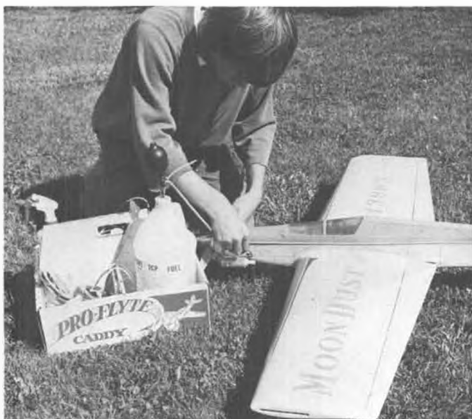
Mike Sheeks fuels up "Moon Dust" for a flight. Wing can be made with a foam core or with built up frame. It's sheeted either way.
