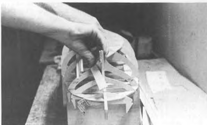
Planks are glued to frames only, NOT to each other, using 5-minute epoxy.
