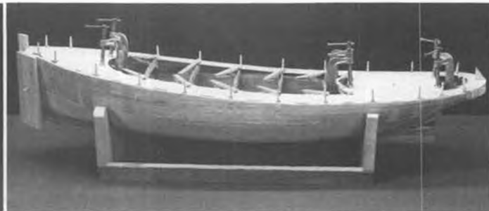
Clamps and masking tape hold main deck in place while epoxy cures. On this model, Epoxilite coating was added after main deck.
