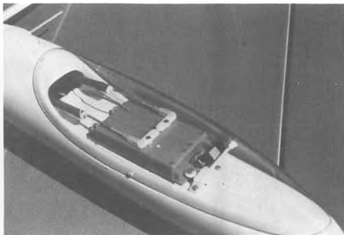
EK brick is an easy fit in the Hobbie Hawk cockpit. Complete radio installation took less than an hour . . . including two Martinis!
