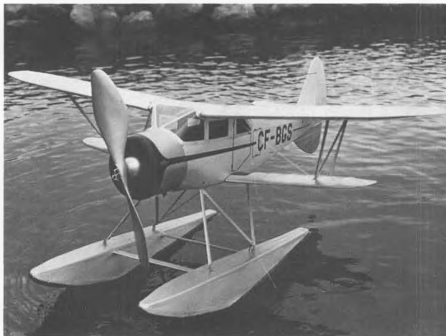
Land and sea versions of the Waco are shown on this page. Model is covered with satin-aluminum Monokote, which provides a very realistic finish. Floats from Oct. '73 issue, by Hal Cover.
