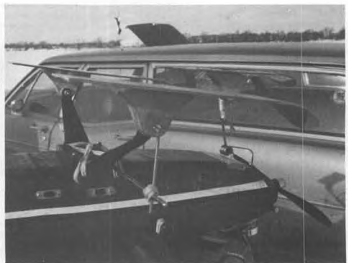
Trike gear installation on Senior Falcon. Main skis are 12" long, and the nose ski is 8. Note springing linkage.
