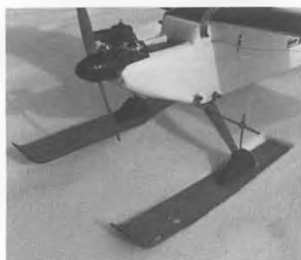
Veco 35 powered DeBoit Champion uses 18" skis. Note springing set-up.
