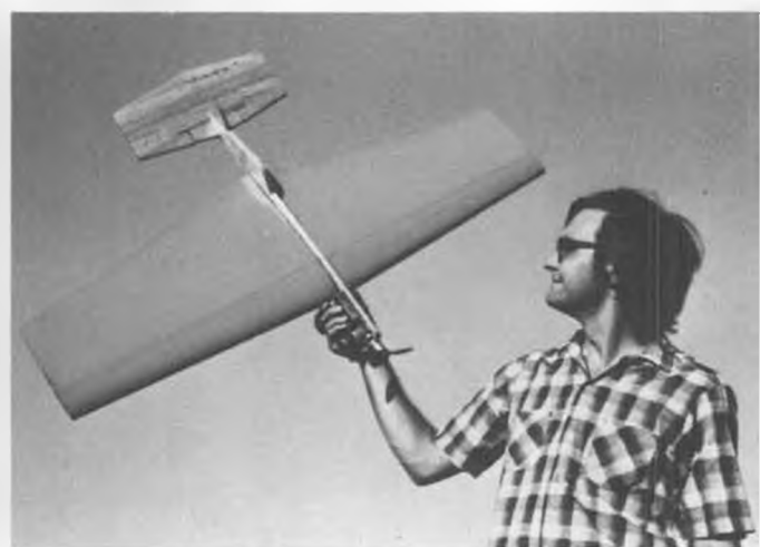
Phil Cartier, Fridley, Minn. and his Slow Combat ship, "Big Pig." It's mostly made of cardboard.
