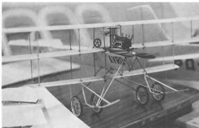
Chuck West's glow-powered Avro triplane flies well in spite of the absolutely zero dihedral. Had takeoff problems, however.
