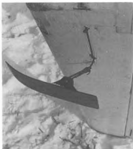
Photo shows mounting of 12 inch main ski on Lanier "Rubber Ducky."
