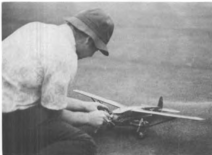
Glutton for punishment, Bill Stroman, with Stinson Trimotor. Three Cox .010's and pendulum ailerons.
