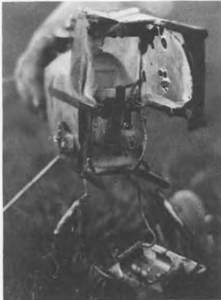
What happens when nitrate dope and hot solder get together. Jack Knapp's old timer Brigadier after the resulting fire.
