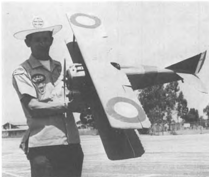
Gene Lamber and his scratch-built Spad. Ship is 1-1/2" scale, weighs 11 lbs., and is powered by muffled Veco .61. Dale Kirn photo.
