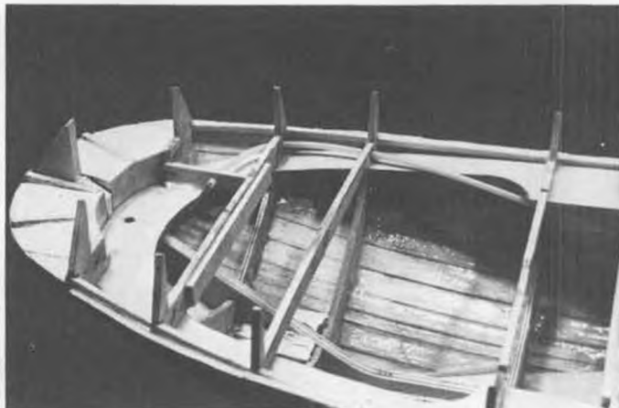
Flex-cable lead to rudder tiller is added before main deck is installed. Bulwark will be epoxied to extension of bulkheads.
