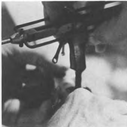
Ernie Huber installed several layers of electricians plastic tape on rotor shaft of Nate's Jet Ranger, which improved hovering capability, but limited maneuverability.
