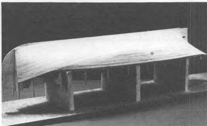
Since planking will not show, it is unnecessary to tediously taper each plank before gluing in place.
