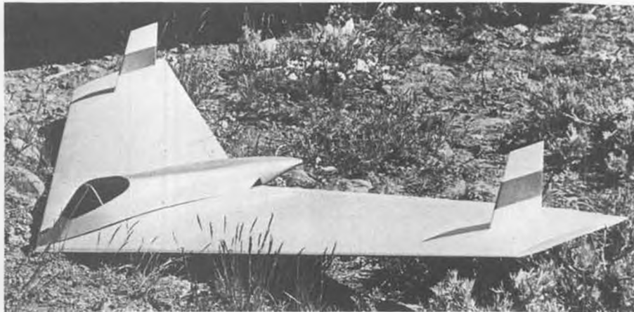
Original flying wing design by Ken Sthur, seen at Wenatchee Soar-In. Cab covers radio gear which is mounted in center section of wing. Note thin tip section.
