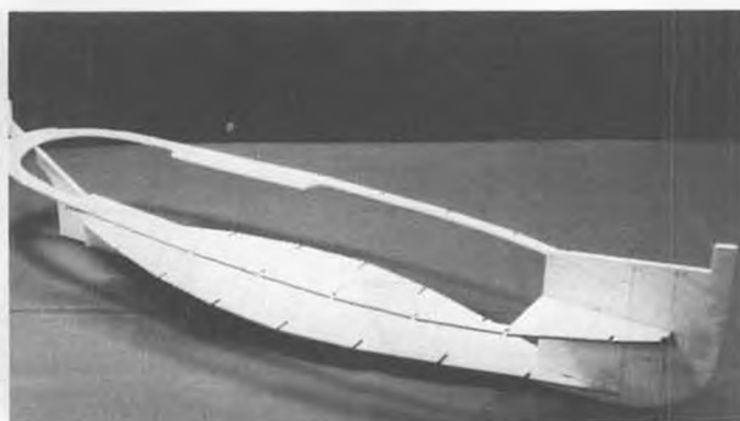
Extra-long notches at bow permit slipping upper deck in place without spring parts. Half-bulkheads can now be added.
