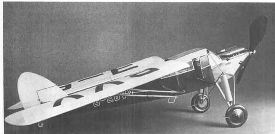
Upon removal of inverted U-shaped wire retainer at front spar, wing may be folded as on full-size aircraft. Rear retainer can also be pulled, for complete removal of wing panels.
