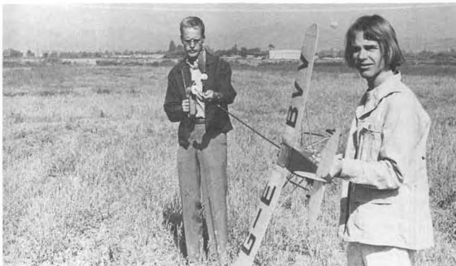
The author's son, David, holds model while Bill winds the 10-strand 3/16 rubber motor the easy way, with a converted Black & Decker battery-powered drill, complete with counter!!
