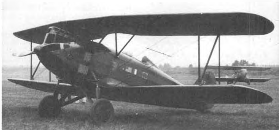
Stock GLT flown by Tex Rankin from Vancouver, Canada, non-stop 1350 miles to Agua Caliente, Mexico. Trip used 75 gallons of gas and took 13 hours, 17 minutes. Galloway photo.
