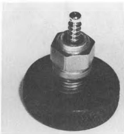
The "Size'r", by Hobby Products, cleans and sizes glow plug threads.
