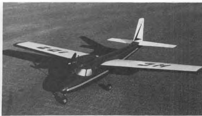
"Hobby Commander" sport trainer from Model Merchant. Features ARF construction of plastic and foam.
