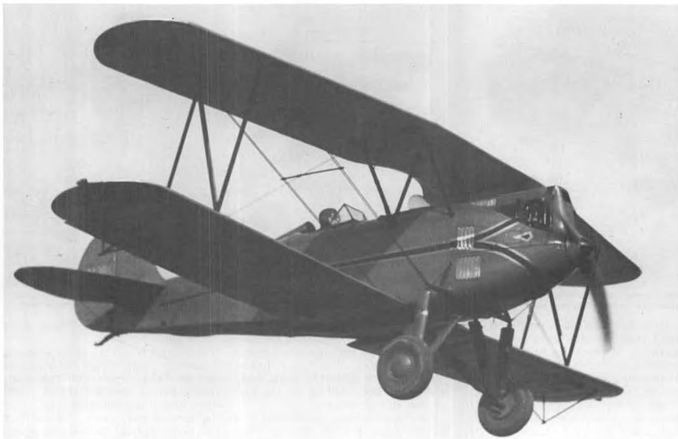
A Great Lakes Trainer 2T-1A coming in for a landing. School airplanes were often fitted with skids at the wingtips. Photo from John Underwood collection.
