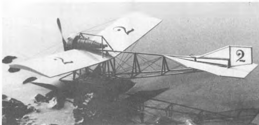
Tiny Train Monoplane . . . Bill Hannan's answer to the Japanese tissue shortage! Brown CO 2 gets it off the water and wins contests. Tail hook indicates it might also be rubber powered.
