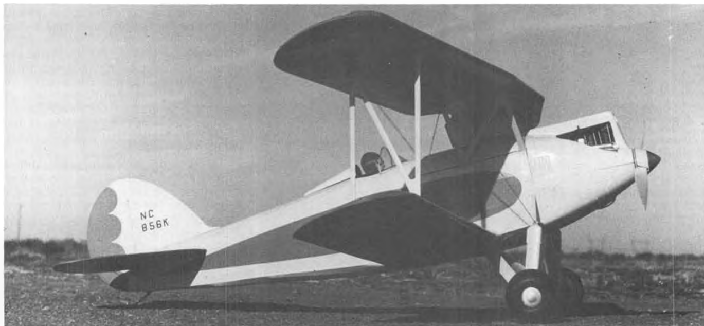
Ced Galloway (C.G. Enterprises) built this 1/10 scale electric powered free flight model of the GLT he used to own. He used Westburg's plans. Power is a VL-101 electric motor. Model came out a little heavy for this unit.
