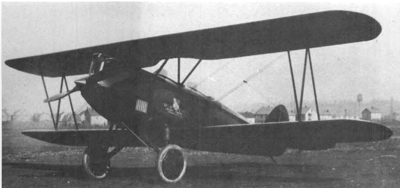
The first Trainer off the production line had a straight wing. Though shown at the Detroit Air Show in March 1929, and heavily advertised, it was found to be tail heavy and went back to the shop for redesign. Upper wing panels were then swept back 9.2 degrees, lining center of lift with CG.
