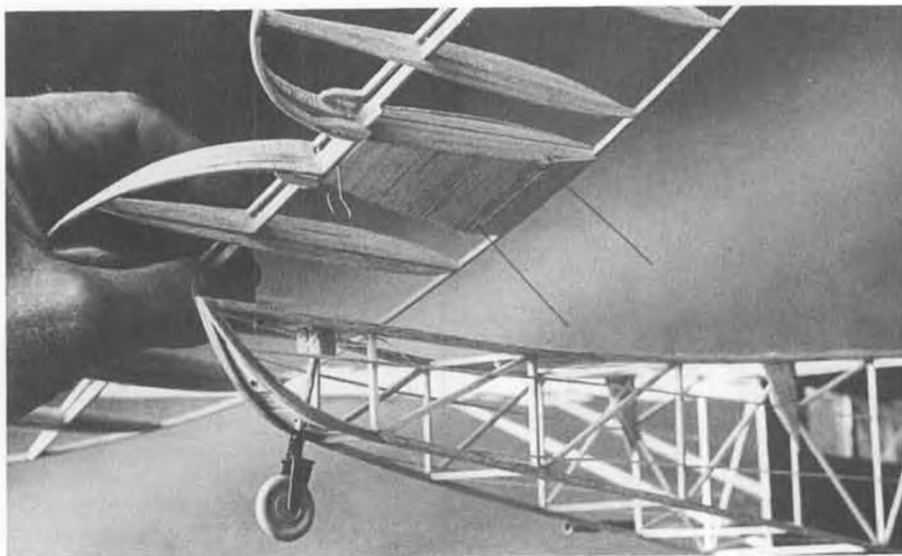
Stab is hinged for easy incidence adjustment during trim flights.
