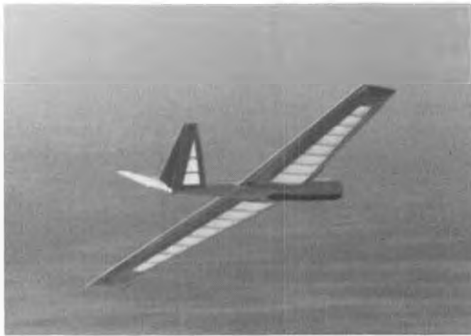
Dan Kreigh, Riverside, Calif., built this from left-over Gryphon wings. V-tail is for pitch only, ailerons handle the turns.
