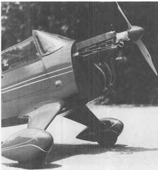
The Rearwin Speedster on the cover, with cowl removed to show the tandem twin K&B 40 (80) installation. Turns 16 x 6 at 7,500 rpm.
