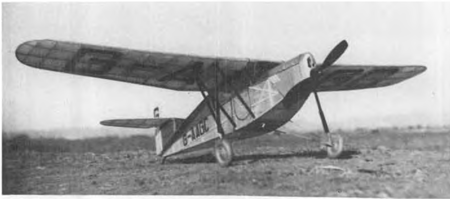
The author's Desoutter monoplane is powered by a VL HyTork planetary-gear electric motor. Span is 3 ft., weight 4-1/2 oz., has won 3 contests so far. Built from plans by E. Fillon, France.
