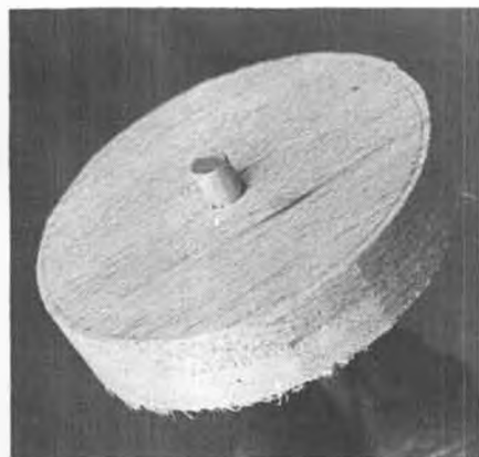
Rough-cut wheel blank, ready to be chucked in lathe or mounted hand-drill for shaping.
