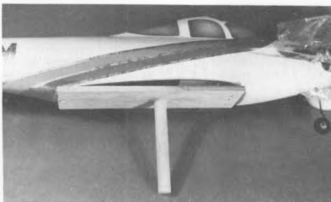
Fuselage painting jig provides a means of painting entire piece without having to touch the surface.
