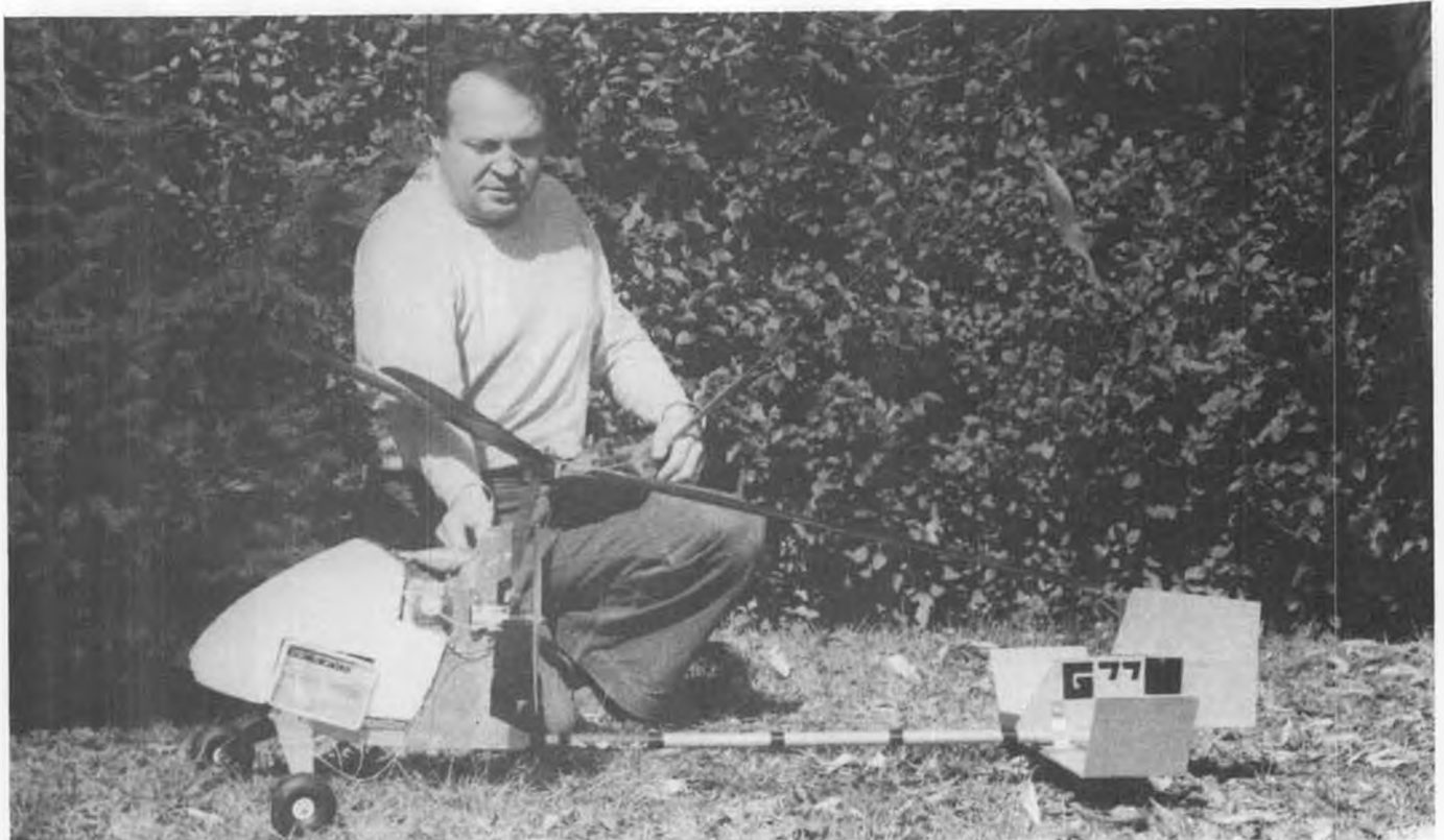
The author with his model G-77. Georges says it's not meant to be a beauty prize winner, but has proven invaluable as a research and development aircraft. Note pushrod tubing taped to aluminum tube tail boom.
