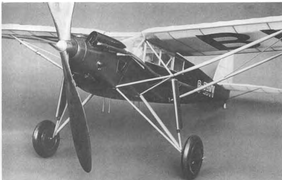
Close-up of front of model. Soda straws used for wing struts. Landing gear slightly lengthened to accommodate large flying prop.
