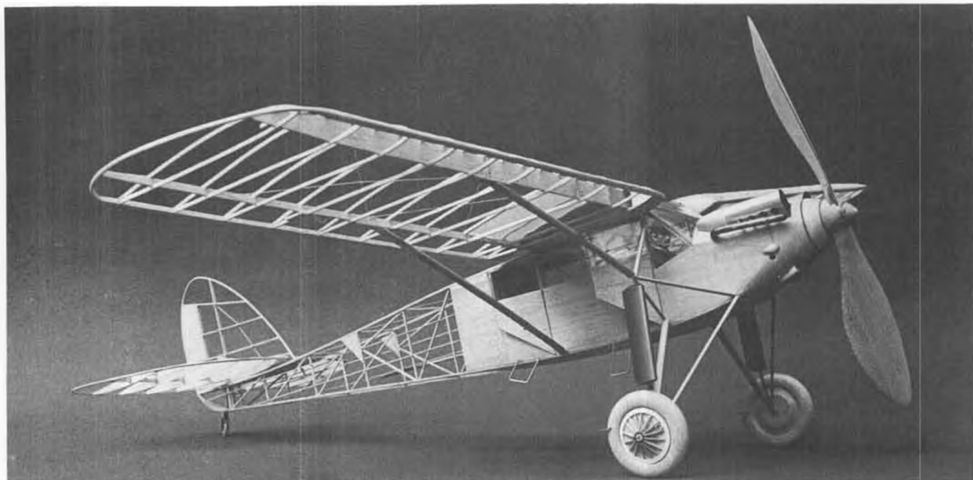
Wing ribs are individual laminated strips, for light, durable construction. Stab, slightly enlarged, and also with a thicker-than-scale airfoil, is the only deviation from scale dimensions. The model is completely stable. Prop is built up of ply and balsa laminations.
