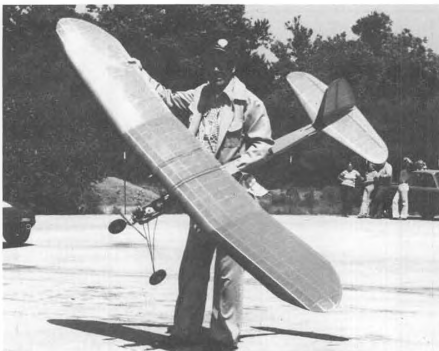
Our own John "Daddy Warbucks" Pond, with his much-flown Lanzo R/C Stick. Power is a Merco 60 converted to ignition.
