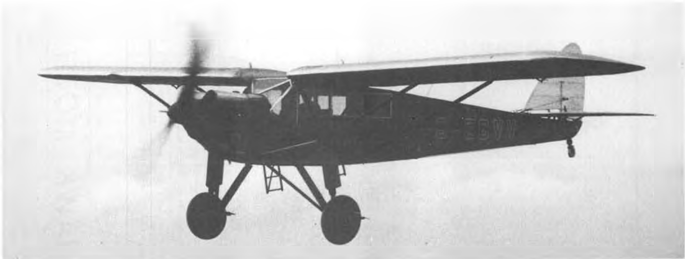
The one and only deHavilland Model 75 "Hawk Moth" in flight, 1929. Photo comes from Flight International Picture Library, London, England. Wingspan was 44 feet (Curtiss Robin was 41 feet), and landing gear had a generous 10 foot tread.
