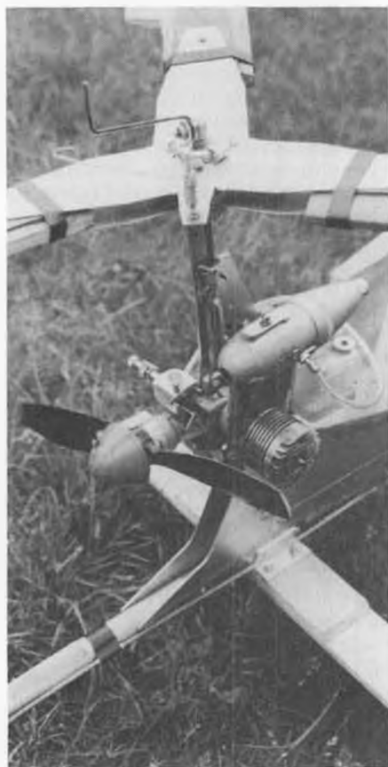
Close-up of GYROTOR head. Note rubber-driven prerotor. Useful for takeoffs.
