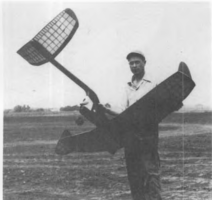
Bob Knutson, Austin, Minn., stretched Sailplane main wing, clipped Zipper front wing, retract gear, parachute DT, flew great in 1942.
