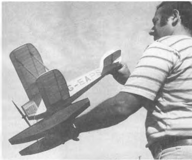
Fernando Ramos with his Sopwith Baby on floats. Merlin .049 diesel couldn't overcome suction of flat-bottom floats. Flew hand launched.
