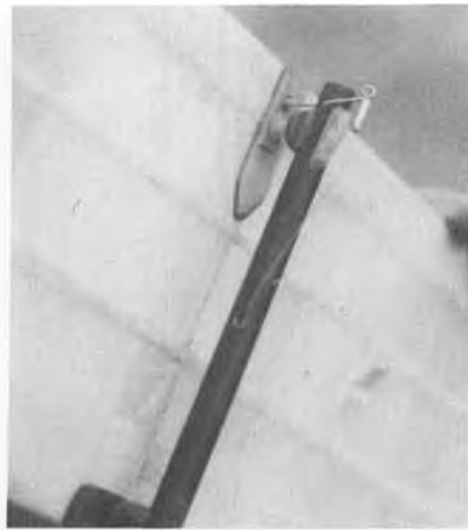
Auto-stab kicker used on Wayne Drake's A/2. Releases after line disconnects for glide trim.
