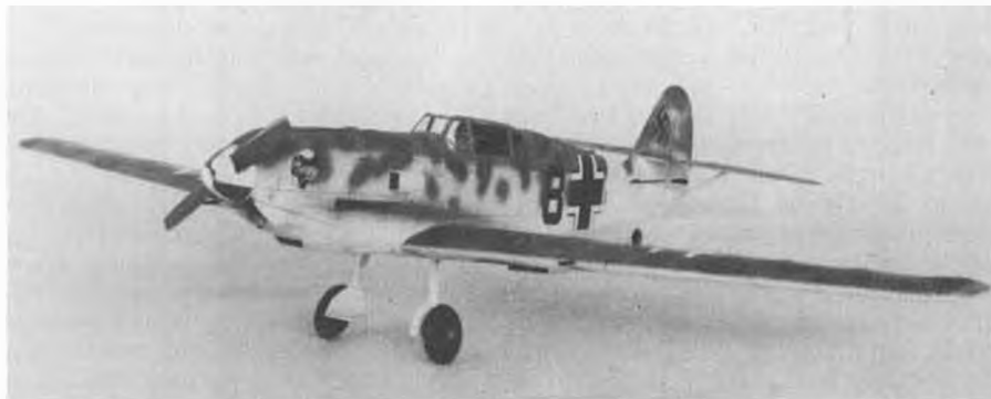
House of Balsa's ME-109 for 2-channel radio, is a real smooth flyer. Needs a strong engine, so figure on a large tank, high nitro (40%), and a drilled venturi with pressure fuel supply.
