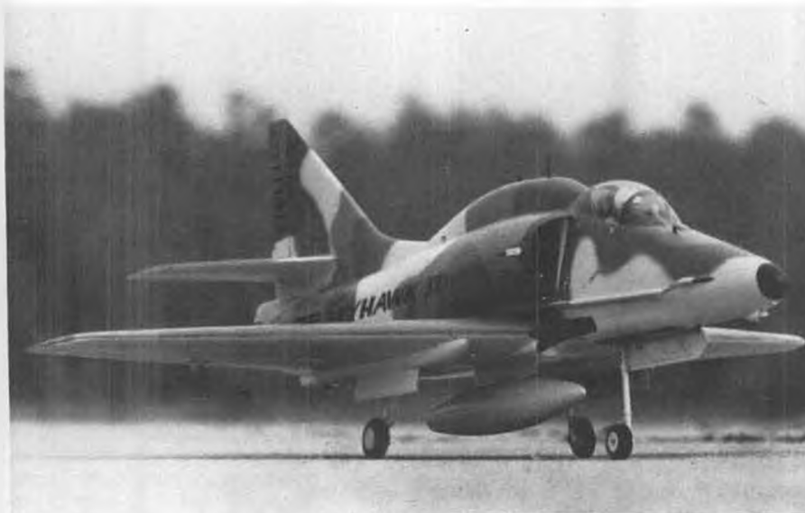
Latest version of Bob Violet's Skyhawk is this A-4N, with avionics dorsal pack and long-range fuel tank. Kit is fully described in text. Ship placed 2nd in Nats Sport Scale.
