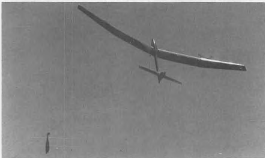
Chet Tuttle's original design "Dreamer" on winch tow at the Nats. Thirteen-foot model has tip spoilers for turn control, reported to be very effective.
