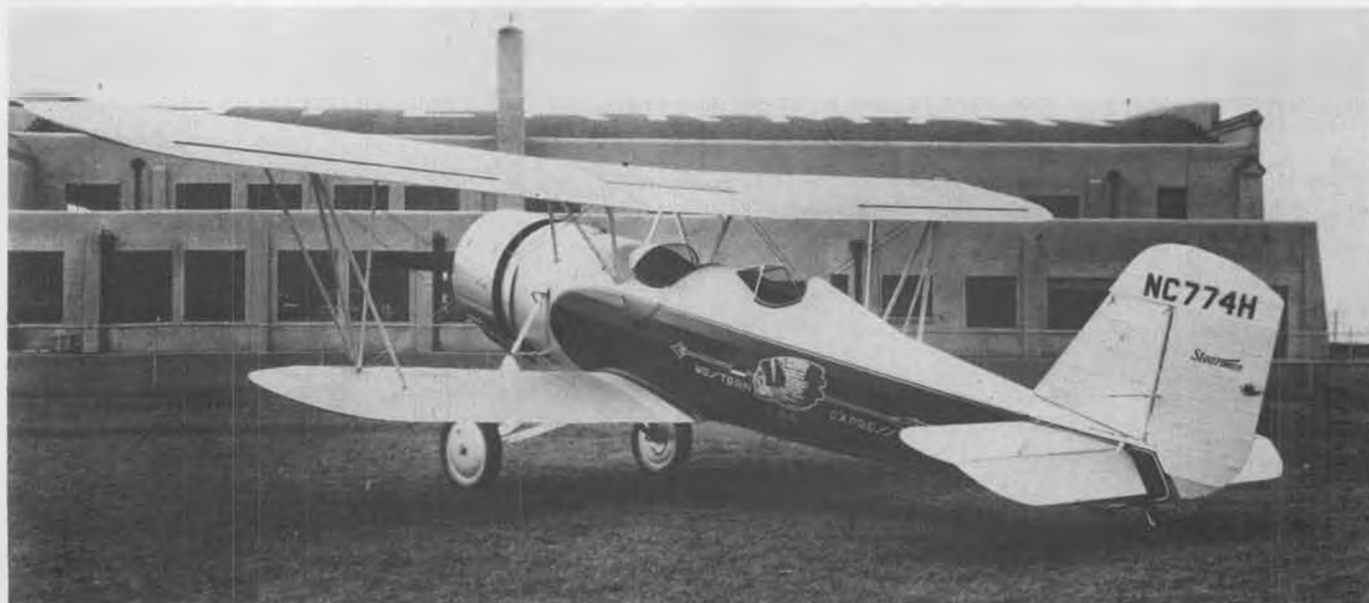
Stearman s/n 4011, shown above, was originally a 4D powered by a 300 hp P&W Wasp Jr., as shown here. The aircraft was later converted to a 4DM by covering the front cockpit; it was used to haul express and mail. Stearman plant is in the background.
