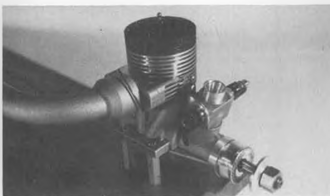
RADIO CONTROL PATTERN, ENGINES: Rossi .60, one of the engines most used in this class of competition, with airplanes such as the Bridi UFO. Tuned pipe available for added power. $166.90.
