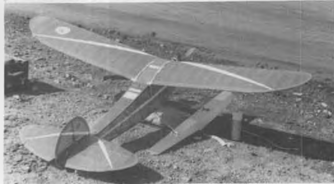
Bob Von Kinsky's Anderson Spitfire-powered Powerhouse used a simplified version of the Berkeley Gondolier 40 floats.
