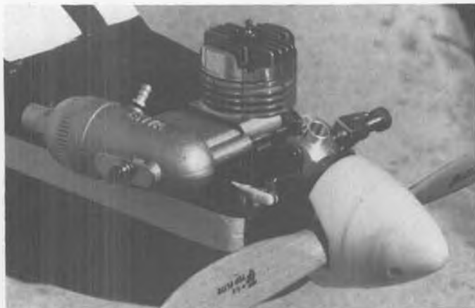
Everything in this photo is furnished . . . Enya .15, muffler, glow plug, spinner, and Top Flite 8 x 6 prop.
