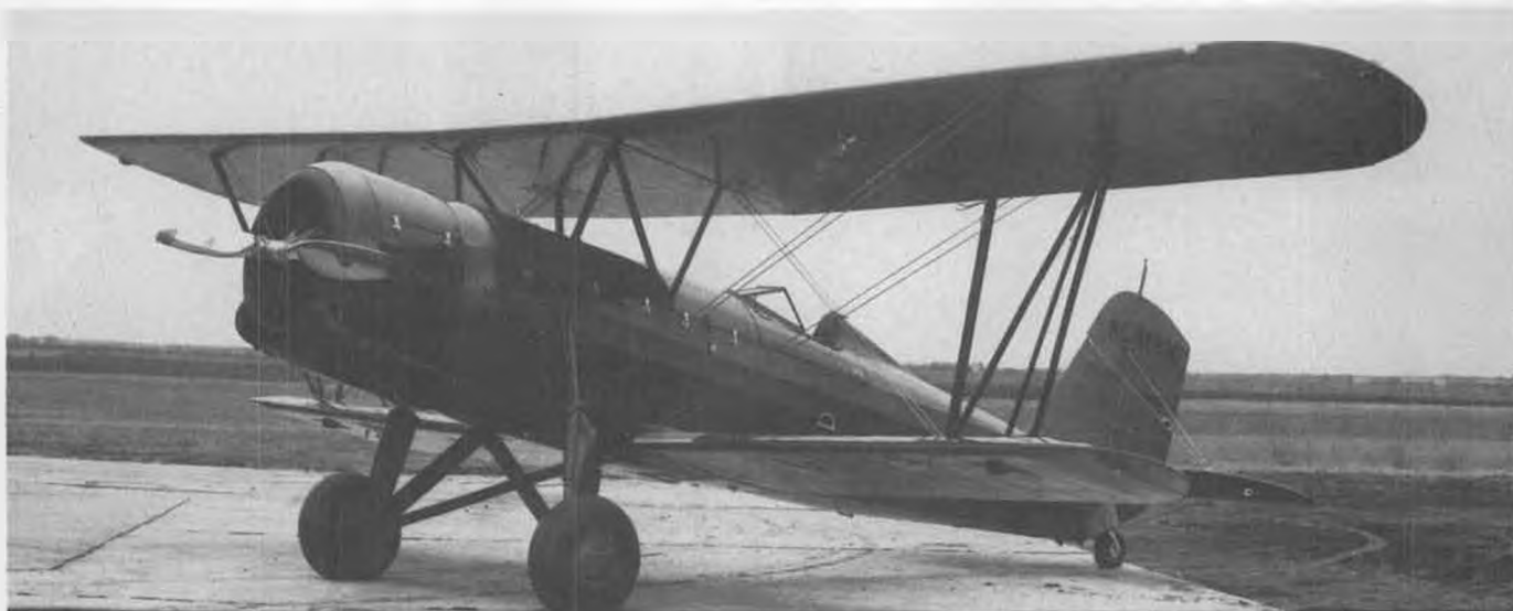
This Stearman 4CM was the first of 12 sold to American Airways, forerunner of American Airlines. The planes were used to shuttle mail on American's routes. Note that the exhaust collector ring forms the leading edge of the NACA cowl, a distinguishing feature of 4C models.
