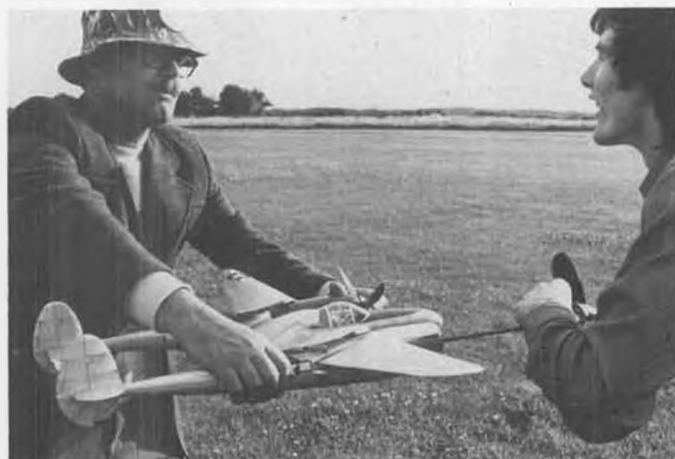
A real scale challenge is this rubber-powered P-38 by R. Falconer, of England. Model features well-detailed cockpit and counter-rotating props. Must require special launching technique!
