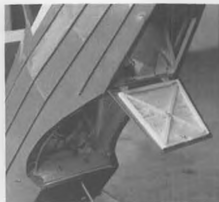
Radio hatch, spray tank and shut-off valve. Tube connects to spray booms.
