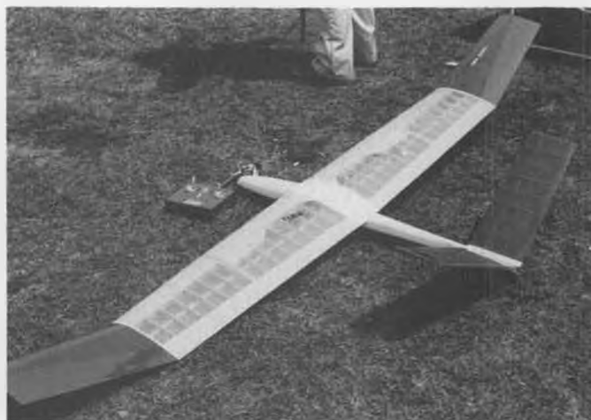
"TUES" (Truitt's Ultimate Evolution for Soaring), by Jim Truitt, features a low aspect ratio, all-flying V-tail, and tiny spoilers.
