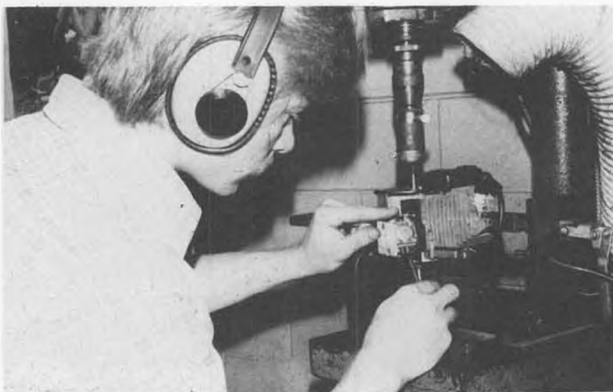
Initial running and test station. All Quadra engines are run at the factory. Here, a worker adjusts the high and low-speed needles.
