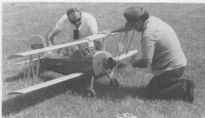
Designer Floyd Fitzgerald applies manual starter to O&R ignition engine. Radio is unaffected by ignition interference.
