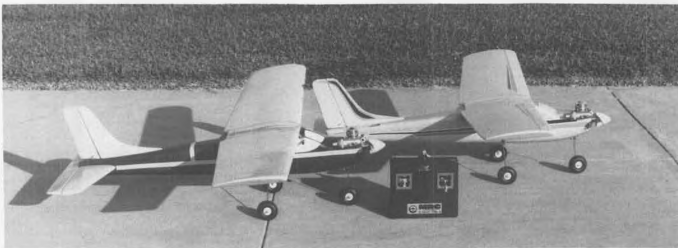
A pair of Hawks, with MRC 775 transmitter. Model on the right is stock; one on the left is customized as per the text. Customized version looks more individualized and also makes the model last a little longer.
