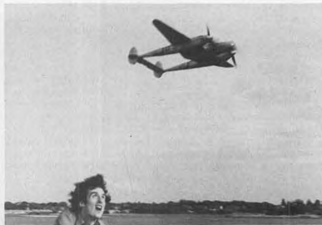
A real scale challenge is this rubber-powered P-38 by R. Falconer, of England. Model features well-detailed cockpit and counter-rotating props. Must require special launching technique!
