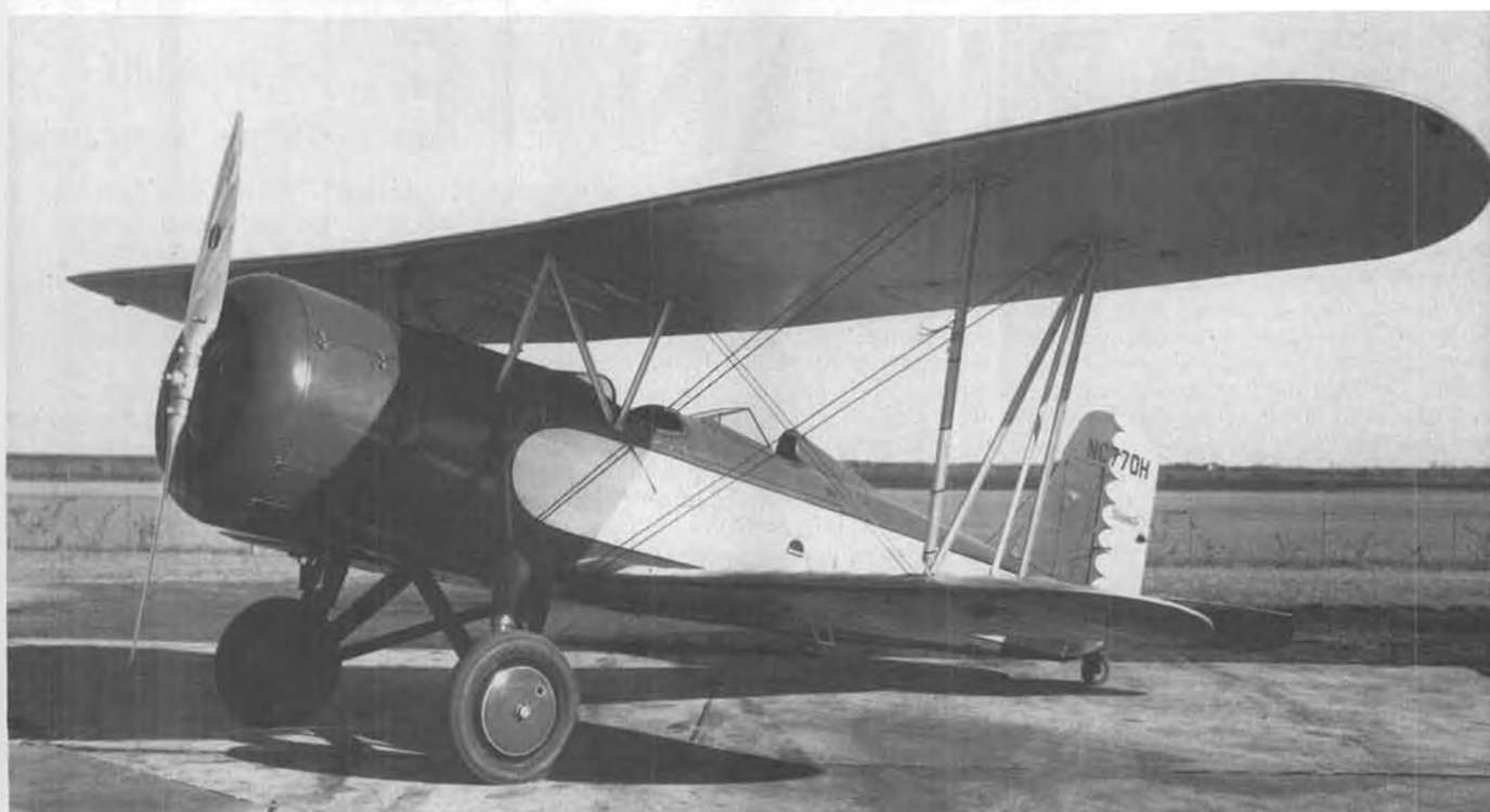
The caption on this Boeing photo states that the airplane is a 4E, but the engine is a P&W Wasp Jr., making it a 4D. The airplane was originally a Stearman test article before being sold to Canadian Airways, where it was converted to a 4EM.
