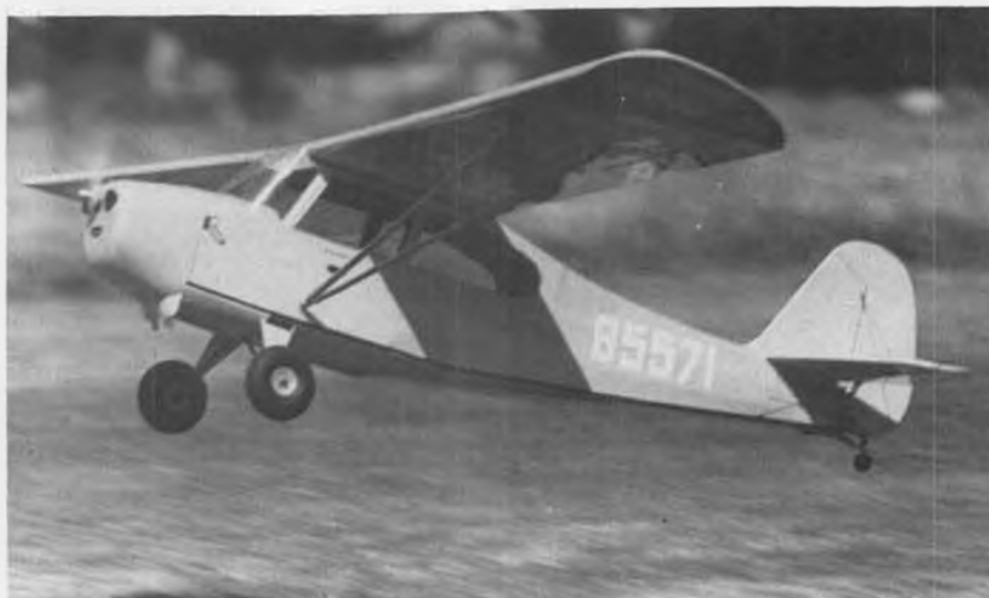
Jim Love's Aeronca Sedan is his first 1/4-scaler. Short prop arc leads us to suspect he's using a .60-size engine with no speed reducer. Hey, Jim, where's the driver?
