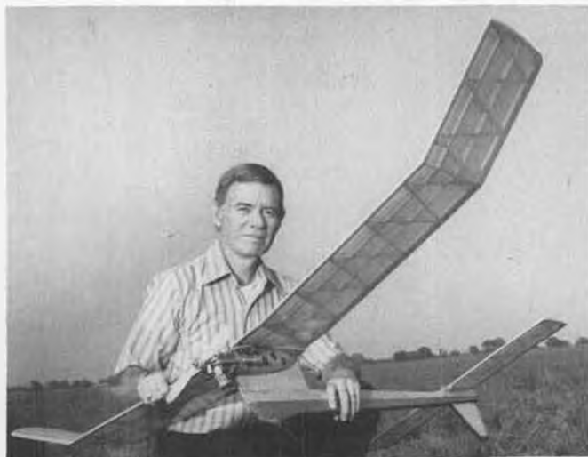
FREE FLIGHT, AIRPLANES: A-B-C Scrambler, Sig Mfg. Co. Designed by Jim Clem. For all engines from .15 to .35, $14.95. Kit includes die-cut Sig balsa, covering materials, full-size plans.
