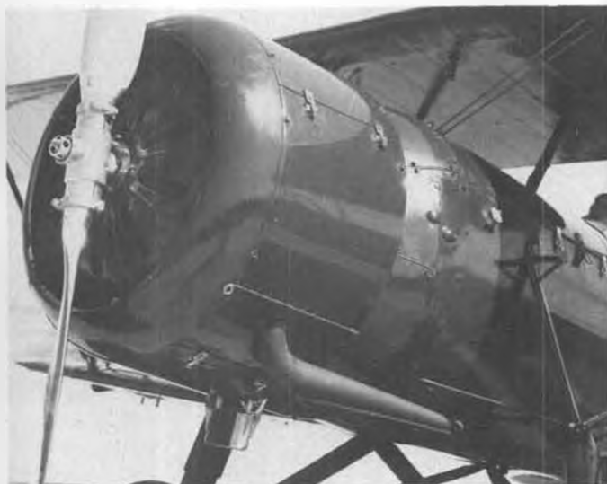
Excellent detail is visible in this close-up of the nose of the Stearman 4DM, powered by 300 hp P&W Wasp Jr.
