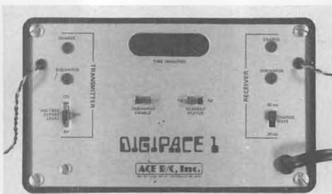
MISCELLANEOUS: Digi-Pace, from Ace R/C. The latest in radio system battery testers. Tells the exact amount of current, thus the exact amount of flying time possible. Detects bad cells. $95.
