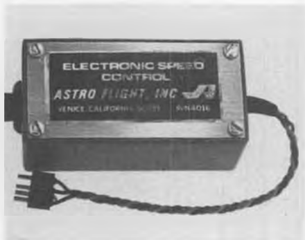
Receiver-operated ON-OFF electric motor switch, from Astro Flight.
