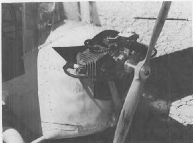
Which Quadra is a dummy? No, it's not a Quadra twin. Cylinder on Aeronca's right is bolted on for appearance... also helped balance.
