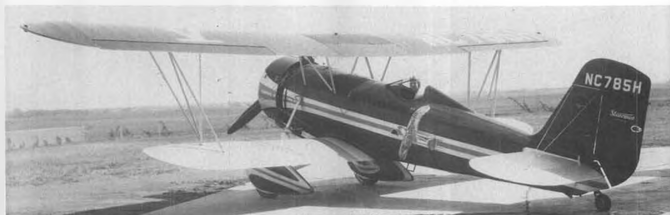
The third of three 4E's delivered to Standard Oil of California has had the forward cockpit converted to a mail pit, making it a 4EM. The words "Junior Speedmail" are painted on the rudder; however, when converted to a mail plane, the planes were called "Senior Speedmails".
