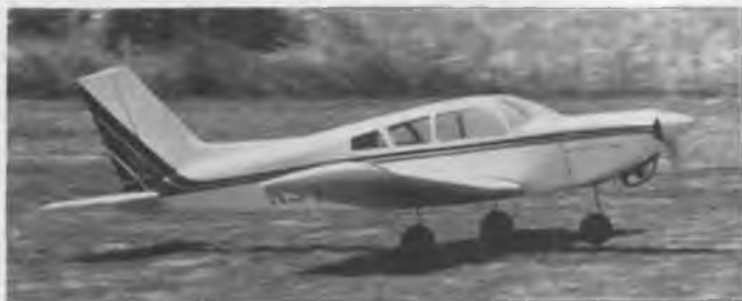
Bert Baker's scratch-built Piper Cherokee 235 uses a plywood frame with balsa covering. Model is very easy to fly.
