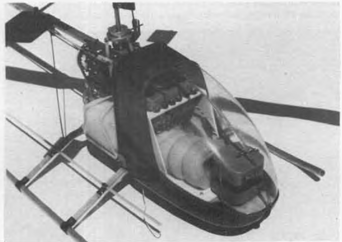
Nyrod tube clipped to landing gear is for the radio antenna, keeps it up off the ground (and out of the rotor blades!).
