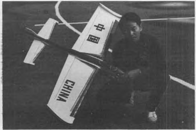
China's Wu Dazhong with his 16th place F2B stunter. "Lifting" tip plates are intended to help maintain line tension during overhead maneuvers, seems to work. China was 5th in team standings.
