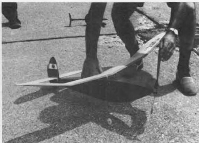
Photo No. 18. Neat flying Nelder Moffett by Ken Groves. Model must be launched in 3-point attitude, otherwise the prop hits the ground.
