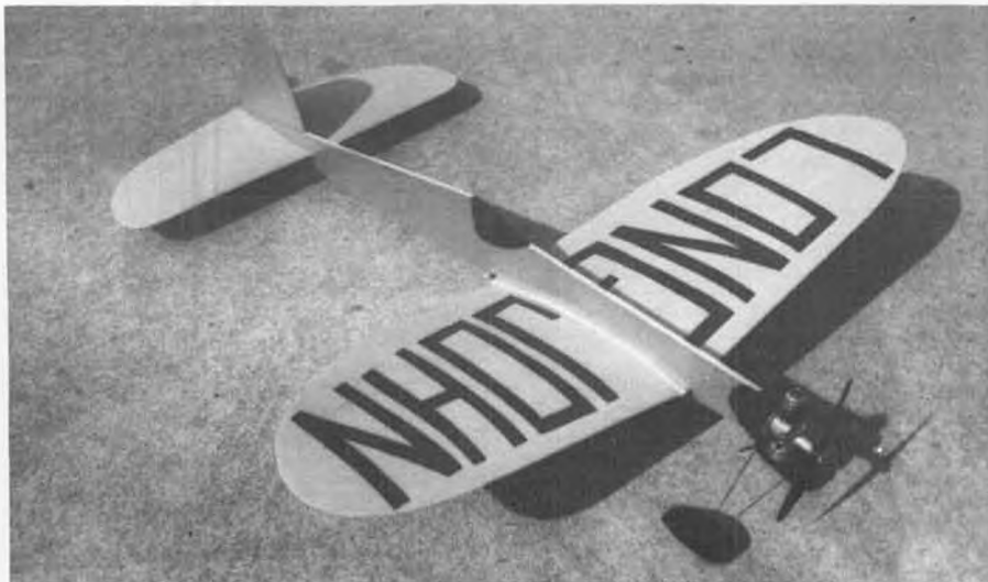
Long John, the author's favorite sport free flight. Uses 1/4-inch balsa fuselage, 1/16 sheet surfaces, and an ancient K&B Infant .020. One evening to build, another to cover and trim.
