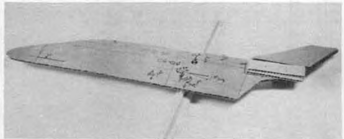
For would-be canard designers, these photos demonstrate how to find the center of lift of a wing (left) and center of lateral area of a fuselage (right). Profiles of a half-wing and fuse are cut from cardboard and balanced over the edge of a ruler. Fully explained in text.
