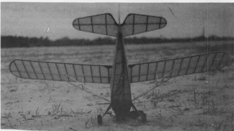
Text calls for two strands of 1/8 rubber, but this shot reveals at least four. Light, simple construction make it especially good for beginners to Rubber Scale.
