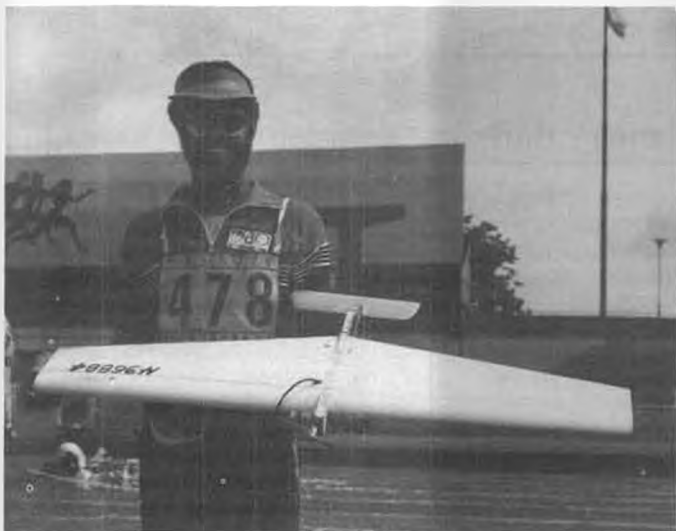
Phil Granderson was the USA's best in Combat at the World Champs, wound up in 3rd place overall. All-foam model is powered by a Super Tigre X15, weighs about 18 oz.
