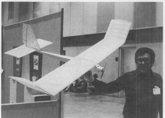
Bob Boucher holds the Naccaratos' first indoor electric, very similar to the one used to set the 1980 duration record of 1-1/2 hours. This one used a direct drive Astro 020, flew surprisingly fast.
