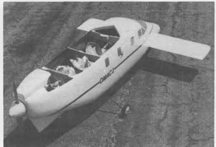
Not much radio mounting room in the fuselage, eh? Wadded-up newspapers keep resonance to a minimum.
