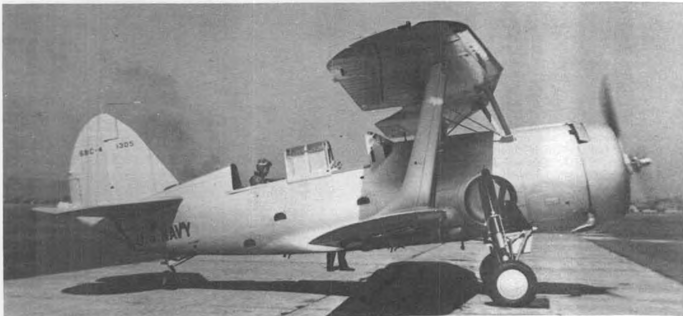
This unmarked SBC-4 was finished in aluminum over fabric and metal. Steps on right side had black painted flaps. Streamlined fairings cover the catapult hooks at the lower wing leading edge on this shore-based airplane.
