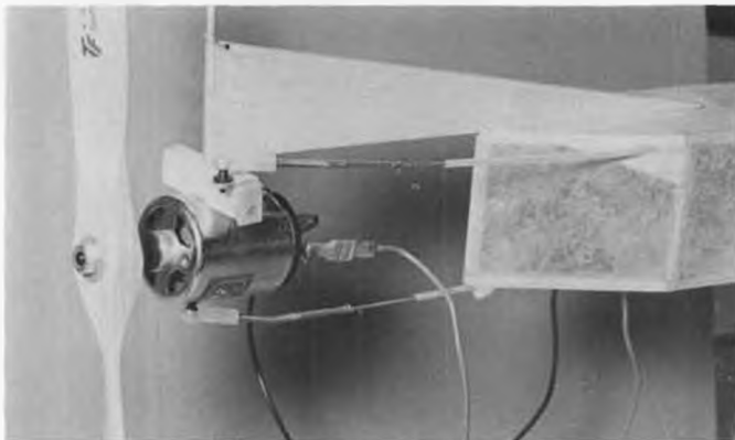
Motor pivots left/right, and up/down. Long loops of wire from motor are needed to prevent metal fatigue and provide clearance around the pushrods. Upper ball link was offset to compensate for movement.
