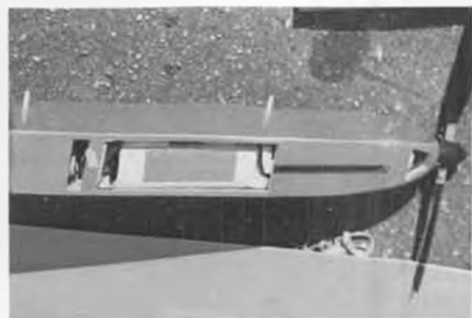
Neat trap door idea with vent for cool air to exit just behind.
