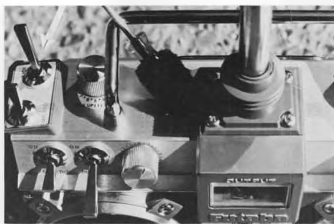
Idle Up-2 switch is easy to find for aerobatics. Note tiny screwdriver that attaches to velcro strip.
