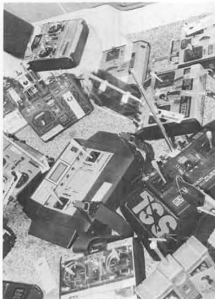
Glider transmitters show Australian variety. 90% fly on Mode 1, right stick forward as Stu flies.
