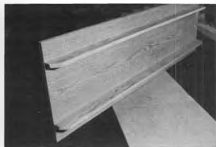
The two runners keep the base true and also lock the 24 station carriage bolts in place.
