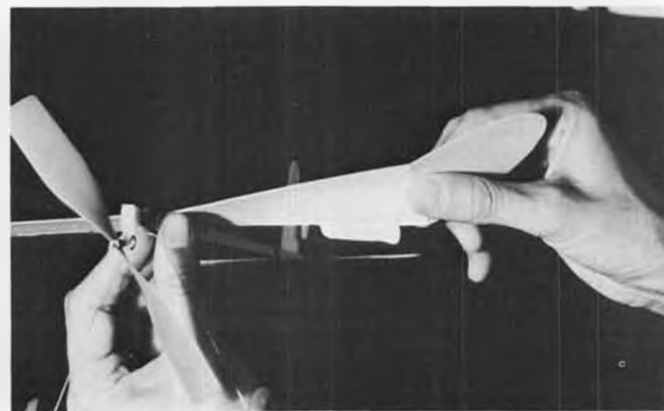
A wing twisted like this is said to have 'wash-in.' In flight, airflow will push this wing up and roll the plane, in this case to the right.
