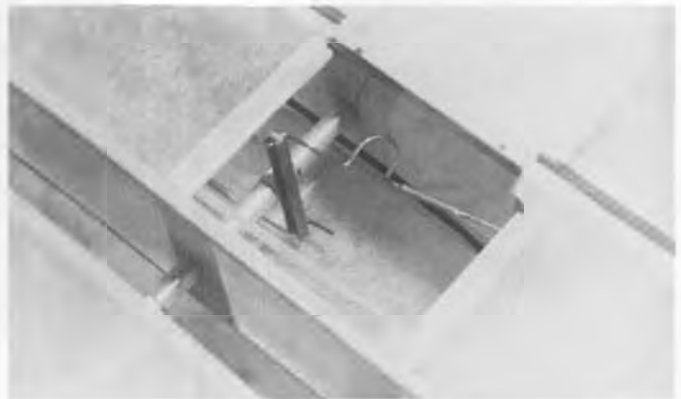
Forward elevator pivot point, showing pushrod loop. Make it from plastic, as control arm needs a backing as shown on plans to strengthen joint in case you hit something in flight.
