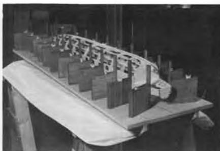
Overall view of the fuselage jig. Base must be solid and straight. See text for details.
