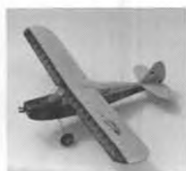
Baby-Pacer $59.50 Versatile small size. Wing Span 50 inch; Weight 2.5-3.5 lbs; Wing load 19-25 oz; Engine 15-40 FS or 19-25 TS or ELECTRIC.
