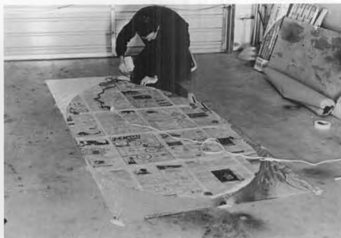
Work completely around pattern, making sure to overlap each individual seal with the next. Process takes about an hour to do.
