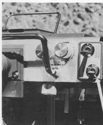
Throttle Hold switch (arrow) and invert switch can be located without fumbling.
