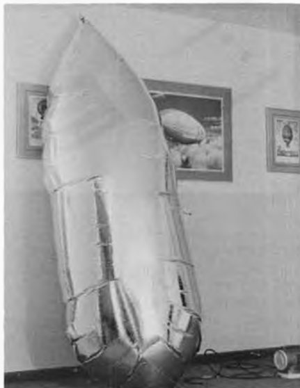
Once bag has been inflated, stand it up and watch for slow, steady deflation. If it is leaking significantly, nose will start to flatten in just a few minutes. Patch leaks with Scotch tape.
