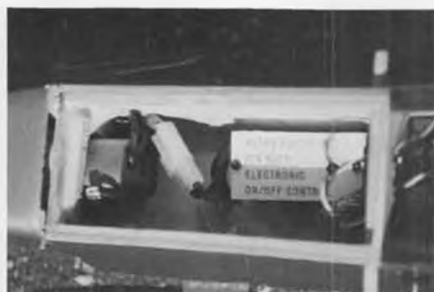
Paul Smith's modified Goldberg Electra, Paul's Thing, uses Astro Flight on/off control
