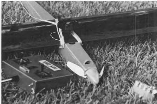
Al's glider with a 9-cell 800mah pack to haul it up with a 3.8:1 Leisure gearbox and an RX540 Technituned motor. Prop is Al's own.
