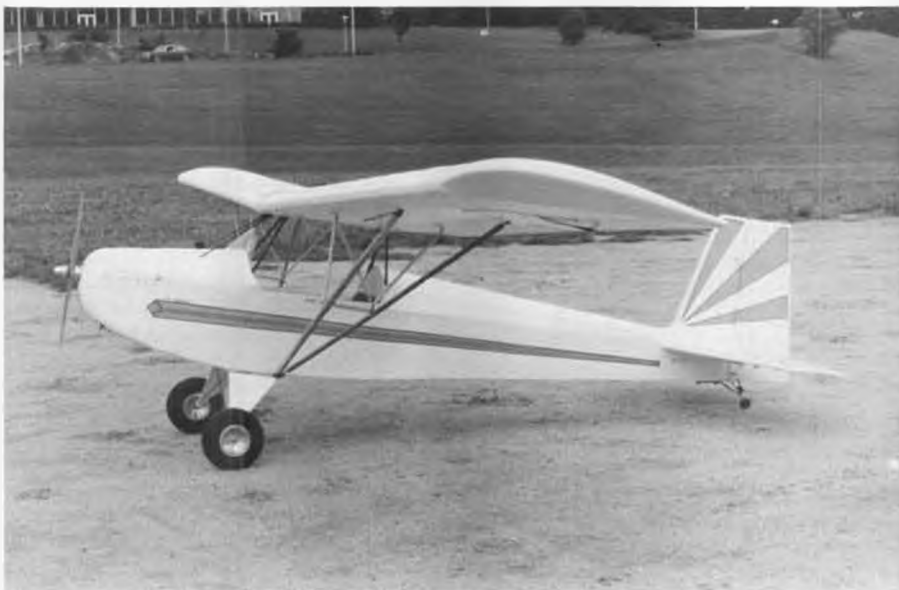
Dry Ridge Models' 1/3-scale J-3 Kitten weighs only 13-1/2 pounds, even though she spans 10 feet. An O.S. SF .61, swinging a 14x4 prop, is ample power for this model.
