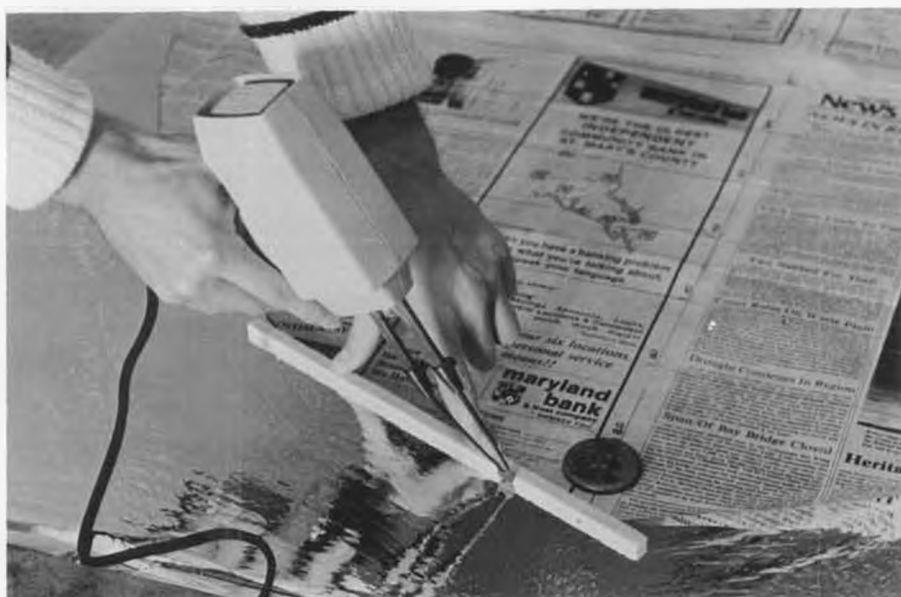
Sealing the plastic bag is done with a soldering gun, using the plastic cutting tip. The wooden stick will scorch and burn a little as you work, but don't let that bother you.
