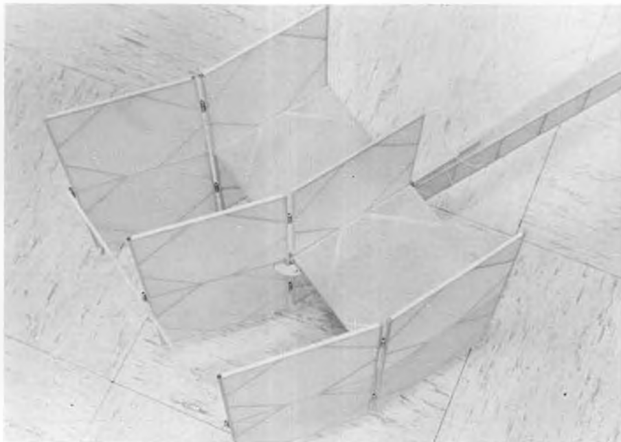
The triple tail. The outer two rudders are slaved to the center by the rudder stick on the trailing edge.
