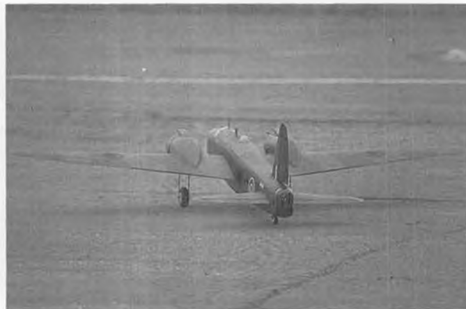
Chris Gauntly flew this Vickers Wellington Bomber to a fourth place in FAI scale, with two Enya .46 four-strokes for power.
