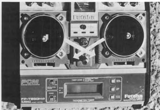
Cross trims for elevator and throttle are unique PCM 8 feature.
