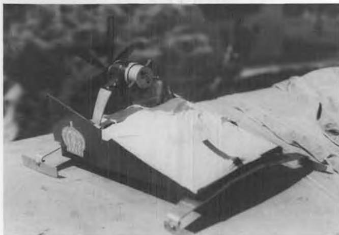
The final design, with lowered CG. Note six-bladed prop; it was later discarded in favor of Cox Grey 7x3.5.
