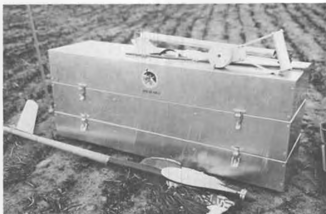
Chuck Dorsett's torque-actuated winding stoooge. He's doing a much better winding job now that he uses Bob Wilder's stoooge.
