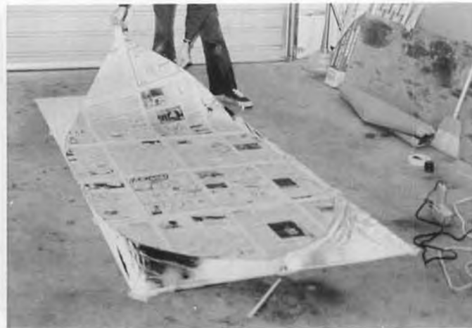
After sealing, lift plastic and pattern off floor, then separate. Tape filler and deflation tubes in place, then inflate.
