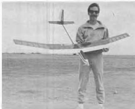
Dennis Brandt holds his slimmed down, high aspect ratio Electricus with E374 wing and five-turn cobalt. Placed 8th.
