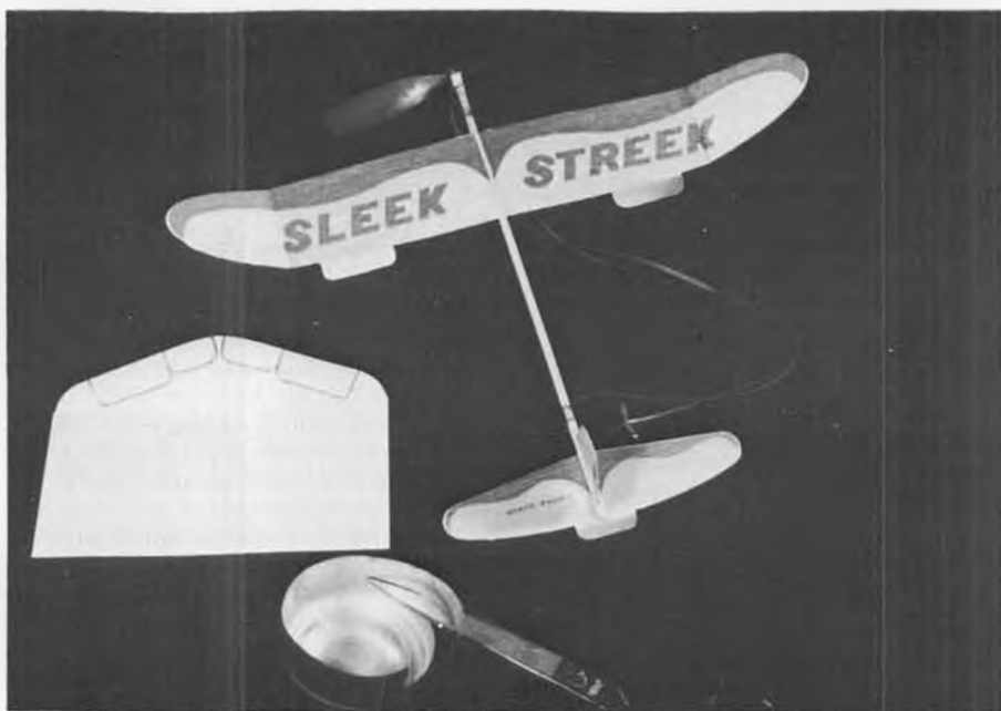
Adjustment tabs can make the model easier to get flying. They are not necessary if you don't want to try them. Envelope-flap tabs will work. Aluminum soda cans keep adjustments put.
