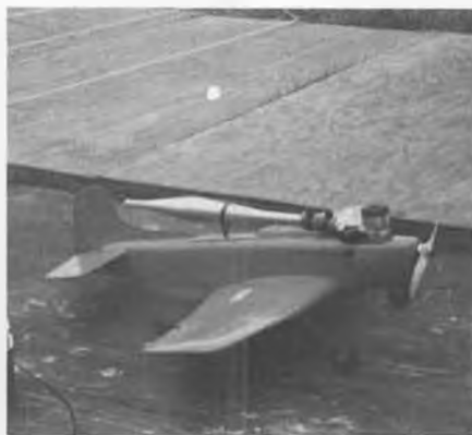
Glen Simpson's AM-1 Martin Mauler sports an OPS 65 with tuned pipe. It'll turn 107mph. Not AMA legal, but for local 'Quiet Carrier' event.
