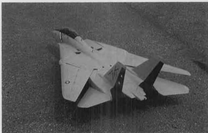
Dr. Jack Tse's 1/10-scale F-14 Tomcat with wings swept in full aft position.
