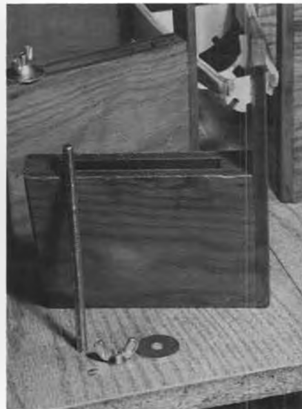
Closeup of station clamp. Note reference line and that base is high-density particle board.
