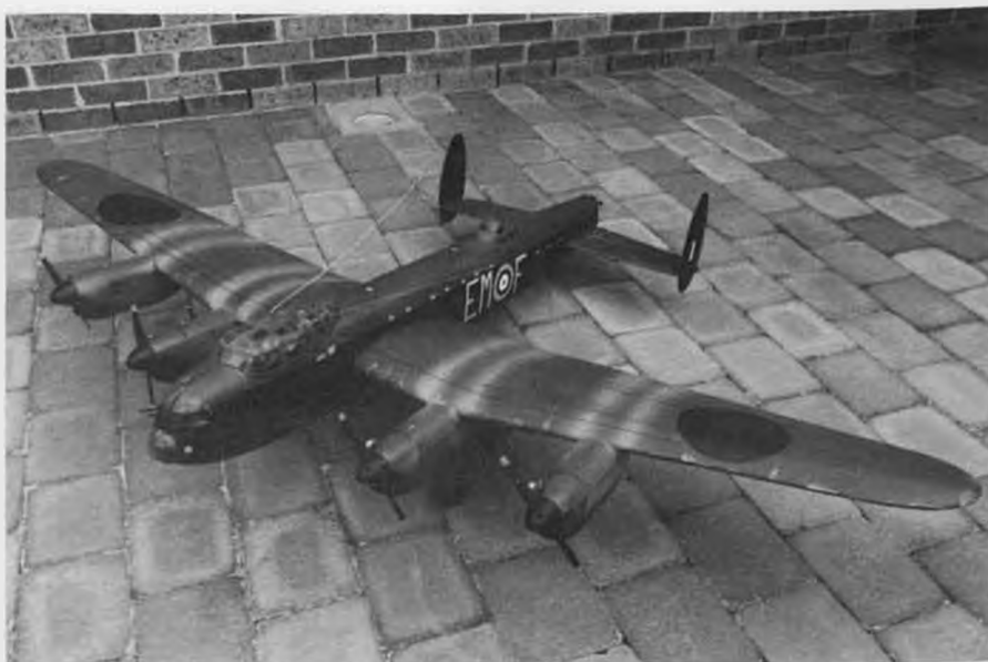
Avro Lancaster built by John Considine, of Bossley Park, NSW, Australia. Span is 88 inches, weight 8-1/2 pounds, powered by four O.S. 10 FSR engines, Rhomair retracts, and controlled by a 6-channel Futaba radio system.
