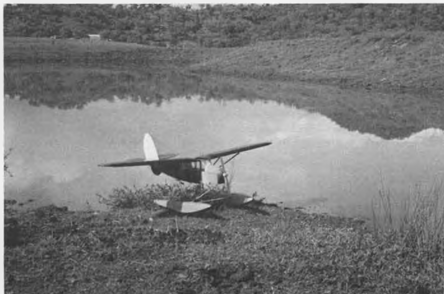
Combining the old and the new, Allan Wall, Kootingal, NSW, Australia, built this Lanzo Puss Moth, installed a geared Astro cobalt 035, driven by five or six Sanyo 900 cells, Jomar SC-5 throttle, and Sermos connectors. Weight is 2-1/4 lbs. and it takes off water in 30 feet turning a 10x5 prop. Flies in calm or rough, gusty weather, about 15 minutes per charge.
