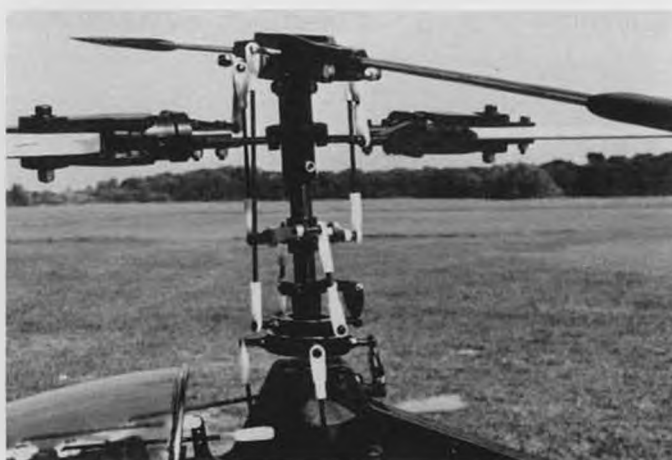
High quality, all-metal rotor head, mixer and swashplate, all factory assembled.
