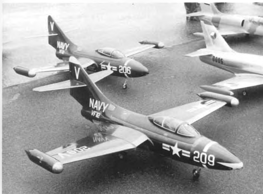
Panthers are Peter Nyes' latest creations, with O.S. 77/Dynamax systems for power. Fuselages are glass and foam, with carbon fiber-reinforced wings.
