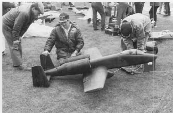
John Menhennet's huge A-10 Warthog, scratchbuilt by John, is an excellent flyer. Power is two Picco 45s, and Thorjet fans.
