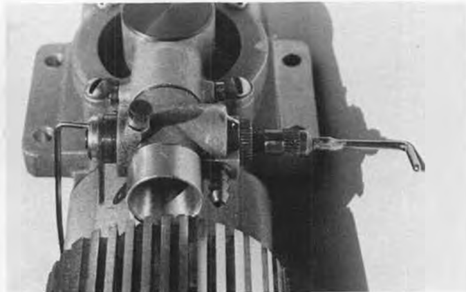
The throttle barrel has a transfer wire that fits onto the engine's exhaust baffle. As the throttle closes, so does the baffle close to maintain combustion heat at low speeds.
