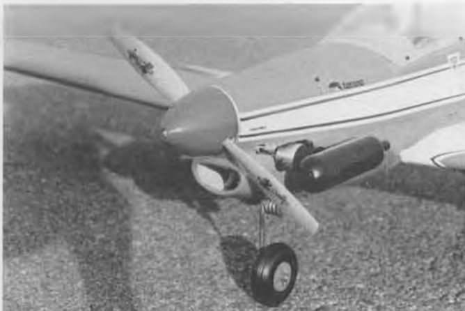
A Picco .45 was used in the test model, which required a few easy-to-make changes in the nose section. It has more power and scale-like speeds with the Picco.
