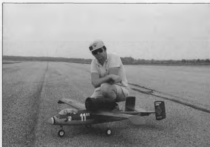
Scale jet models don't get any simpler than this. Ken Rawlins' scratch-built Heinkel He-162 flies very well with a Turbax 1/Supertigre X-40 fan setup, thanks to its relatively light wing loading.
