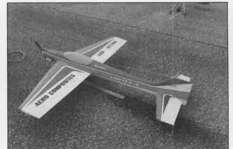
Dean Koger's Vortex II, 7th in FAI. Dean uses a two-stroke engine belt-driving a huge 15-inch prop for almost helicopter-like performance.
