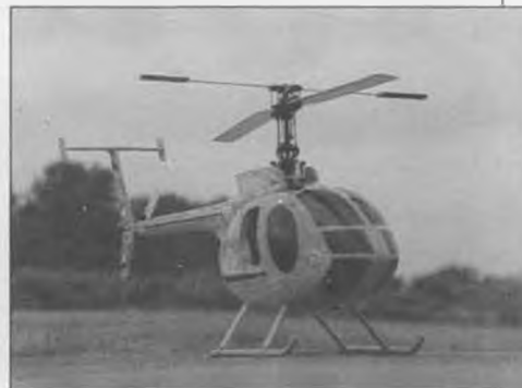
Author's old Shuttle XX is now fitted with a E&G scale Hughes 500 plastic fuselage and Concept 30 DX aluminum paddles for more relaxed flying. The ZX has taken over the role of pint size rocket ship!
