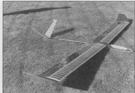
Erich Topfer obviously put a lot of thought and work into his Solarmax. Unlike most other solar models we've read about, the Solarmax's motor is run directly by the solar cells, with no buffer NiCds used.
