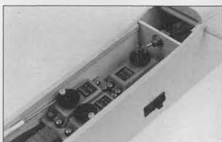
There's ample room in the Eclipse fuselage for small to medium size servos. The one in front actuates the motor on-off switch (supplied in the Deluxe kit). Simple and effective!
