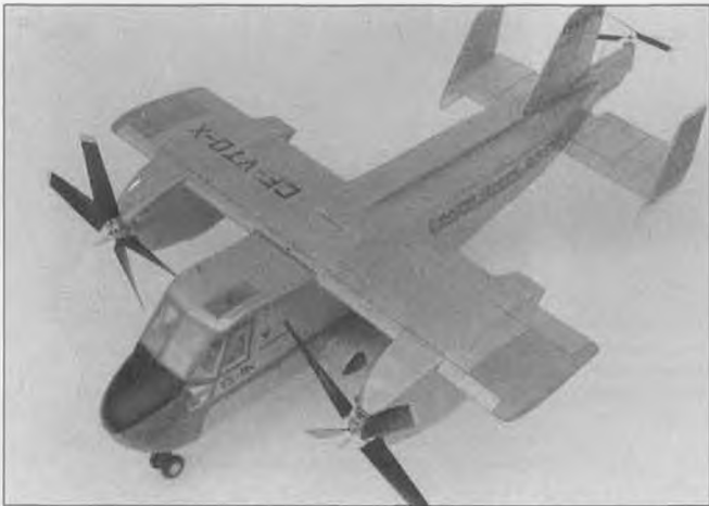
Now here's a model we'd give our right arm to see perform. It's a Canadair CL-84 Dynavert STOL as replicated by Tonda Alfery, of Czechoslovakia. The rubber-powered model is capable of 50-second flights, but what's really amazing is that it employs a timer to (get This): actuate wing tilt, retract the landing gear, and eject cargo during flight! Wow!
