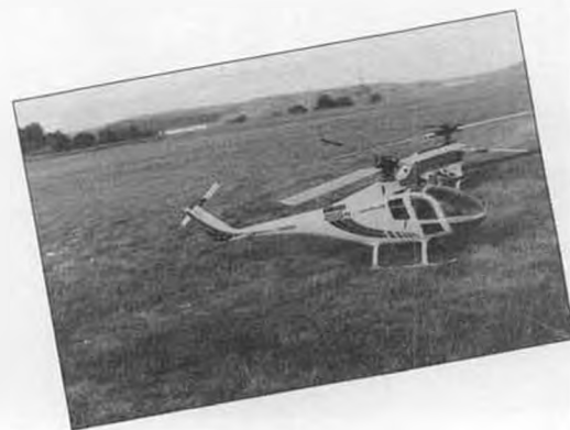
(Left) The non-scale electric chopper built and flown by K. Reutes is a 60-size ship powered by a Plettenberg cobalt motor on 24 cells, and weighing in at 9.7 pounds. With the big motors and high cell count, the airframes on these aircraft have to be built as light as possible to get good performance. (Right) Sleek Lockheed 286h is the work of W. Wiedesheld. Uses a Plettenberg motor, 30 cells, Heim mechanics, and weighs just over 11 pounds. It's capable of six-minute flights and mild aerobatics.
