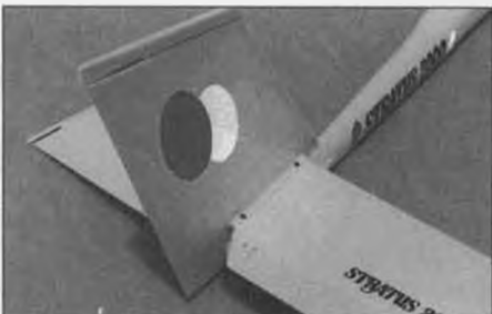
Clean and simple mounting of tail surfaces. Note built-up balsa frame visible through plastic film covering, also tip caps. See text about these.
