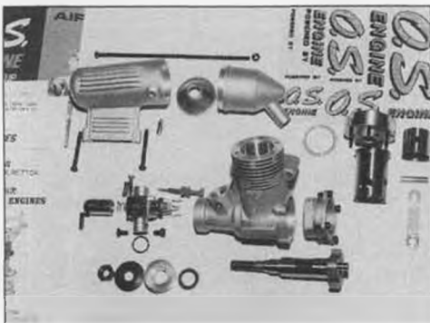
(Left) With few exceptions, the O.S. 25SF is of pretty much standard design. Stu suspects the engine is made in O.S.'s new robotic factory purported to be operating in Japan. (Middle) The crankshaft's disc is extra thick to aid balancing. (Right) Even a close-up shot reveals faultless workmanship. Lubrication for the front ball bearing is via the groove in the crankcase casting (11 o'clock position).
