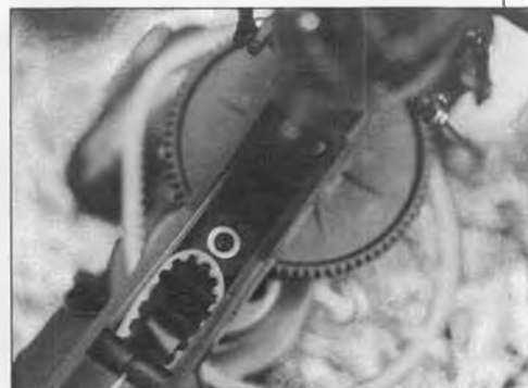
This shows the tail rotor drive belt. After the drive belt is slipped into the small drive pulley, pull the tail boom back sufficiently to ensure the drive belt is fairly tight.
