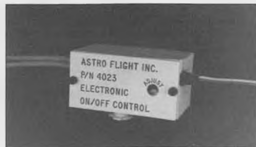
An alternate to the servo-operated motor on-off switch is the electronic on-off switch shown here, also made by Astro Flight. No moving parts, no mechanical actuators to hook up.
