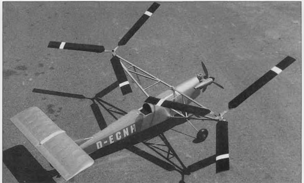
Second F-A 61 built and flown with great performance by Barry Killick, Novi, Michigan. Note taildragger landing gear, which Barry says improved takeoff characteristics. Powered by ASP-40.
