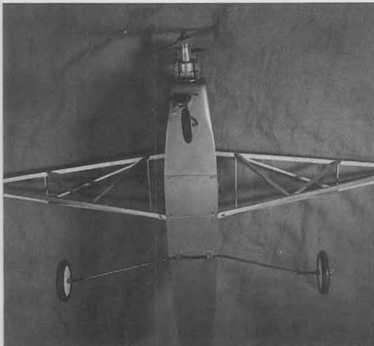
Bottom view shows outrigger bracket and radio access hatches. All of the construction is extremely simple.
