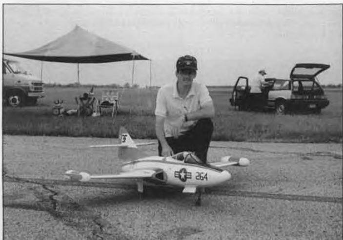
Gorgeous F9F Panther is another of Jean-Guy Rechafort's scratch-built efforts. Features a Byron/Rossi .81 fan, wooden fuselage, foam wing, and removable wing tanks.
