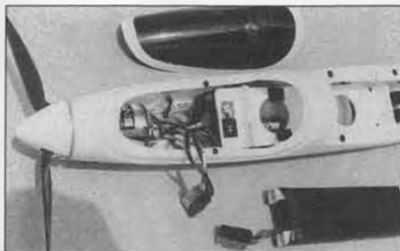
Everything stuffed in but the power pack. Folding prop and spinner, included with kit, installs quickly. Sermos connectors used to cut down power loss.
