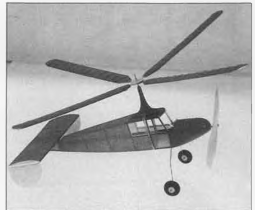
John Walker's variation of Louis Garami's wingless autogyro is unusual in that it is a stable, dependable flying model—most F/F gyros are not!
