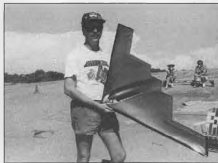
Hey! Who took the pinking shears to my trailing edge?! Randy Warner took my vote for most interesting scale subject at the TPG meet. Stealth bomber, B-2, made out of conventional balsa, ply, and spruce. Flew well, too.
