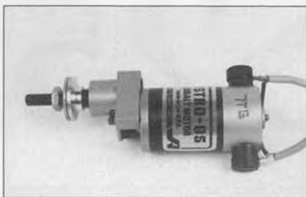
For those looking for a faster climb than can be realized with the Mabuchi motor supplied with the Eclipse Deluxe kit, try substituting an Astro Flight geared 05 Cobalt motor . . . and prepare yourself for a major boost in performance!
