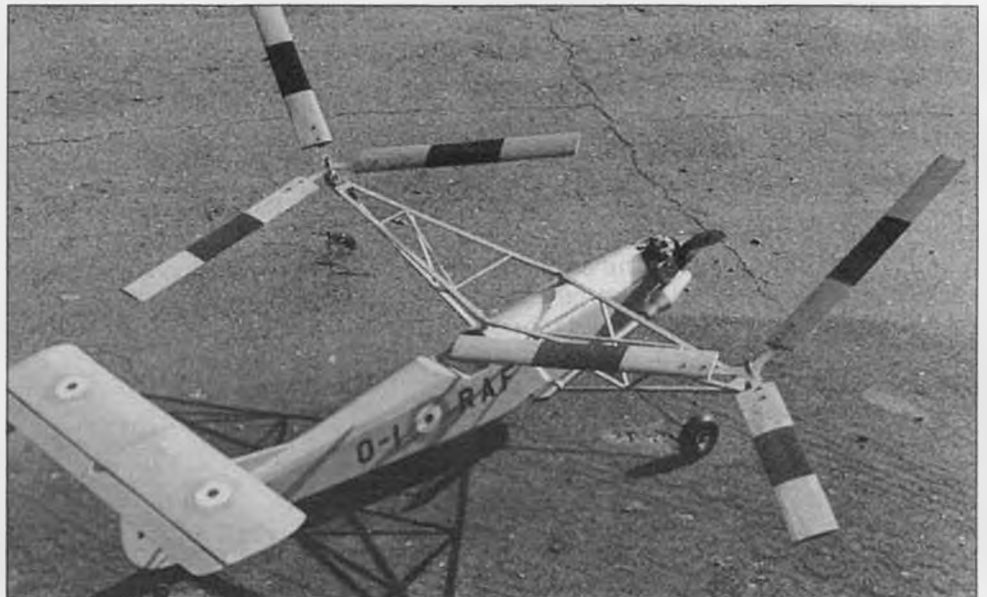
Skip's latest has taildragger gear, constant 2-inch chord rotor blades, and is powered by a muffled K&B 40.
