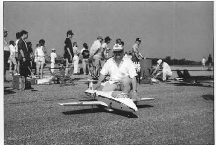
Pretty CT-114 Tutor in Canadian Snowbirds colors is the handiwork of Martin Lefebvre. Fiberglass fuselage and foam core wings, Byron/Rossi .81 fan combo . . . a possible future kit. Of special interest is that, because the scale air intakes are so small, the two forward sections of the painted windscreens are hinged to blow inward in flight to provide additional air to the fan—a clever idea!
