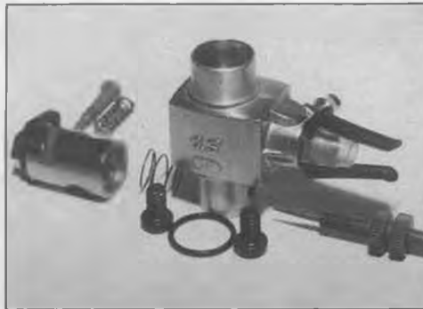
The O.S. 2F carb comes with a piece of silicone tubing installed to prevent air leakage through the needle valve threads—a good idea. Carb barrel is easily removed for cleaning.
