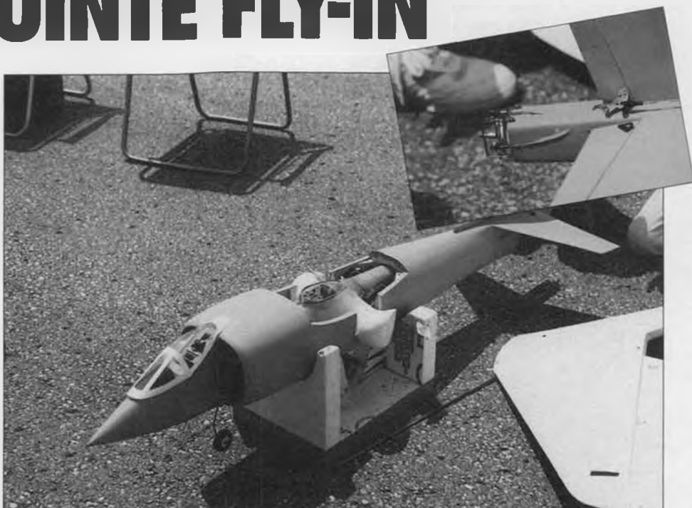
One of the biggest crowd pleasers at Quinte was the sport scale Hawker Sea Harrier being developed by Canadian modeler Eric Dainty. The wing was removed for this photo to show the internal fiberglass ductwork. Eric has the Harrier to the point where it's almost, but not quite, capable of honest-to-gosh VTOL performance—just needs more power. As it is now, takeoff and landing rolls are a scant 20 feet or less. (Inset) Close-up of the thrust vectoring mechanism at the tail of Eric Dainty's Sea Harrier. Control is via cables connected to the rudder and elevator horns. (Below) Jean-Guy Rechfort's scratch-built F-104 Starfighter in pretty W. German livery. She weighs in at 11 pounds and even with a span of only 3-1/2 feet, performed very well with Rossi .81 power.
