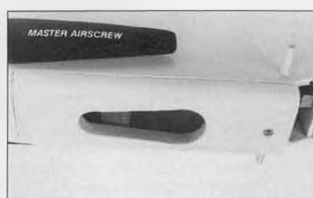
The ventilation opening in the motor/battery access hatch is a slight modification of the one detailed in the kit instructions; this one's a bit easier to make and works just as well.
