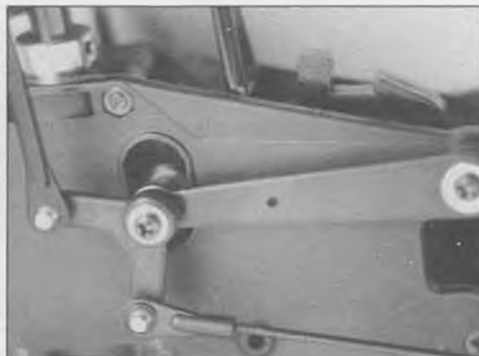
On the ZX, the slot on the side frame is enlarged to permit the collective pitch control swing arm to swing a greater arc for plus to minus 10 degrees of collective pitch travel. This is more than sufficient for any type of right-side-up or inverted aerobatics.
