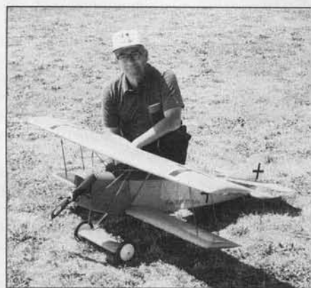
Fred Seiler powers his Fokker D-7 with an S.T. 2000. Radio is Airtronics. Plane weighs 16 pounds.
