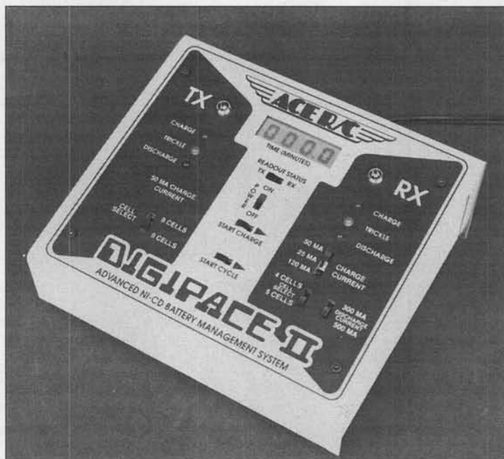
The Ace RC Digipace II, successor to the popular Digipace I, is used to accurately measure the ampere-hour capacity of all common RC equipment batteries, and even to calculate the available flying time for a given battery in a given airplane. The latest Digipace has some worthwhile improvements - read all about it!
