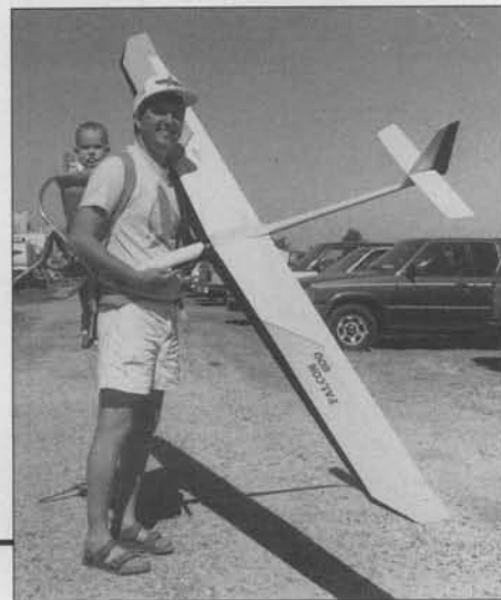
Bob McGowan and his baby daughter pose with the Falcon 800 Standard Class design which swept one-two-three at the '91 Nats in Class C (Std.). Bob prefers the quick handling of the 100-inch Falcon 800 over the 112-inch 880 for better landing scores.
