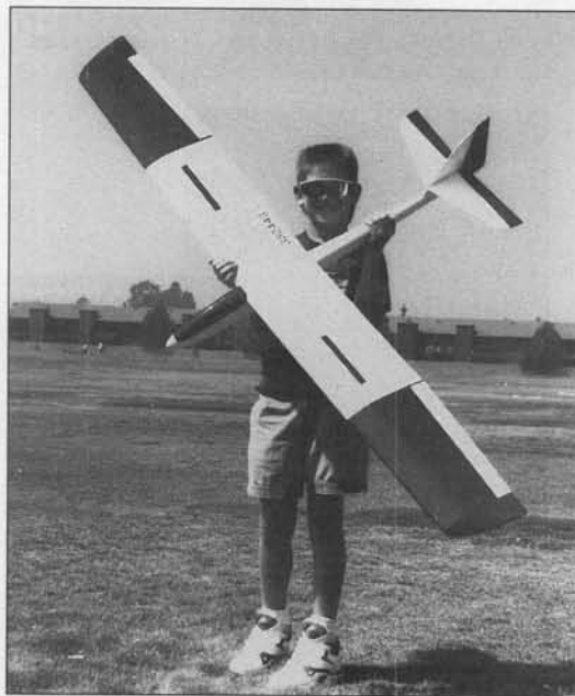
Junior flier Kevin Bauder (age 12) of Riverside, CA, flattened the wings of a 2-meter Gnome (Midway Model's kit), gave it ailerons and coupled rudder, spoilers, and a raised (1") horizontal stab. Only the sixth plane he's ever owned, he's so good that Dave Wilkins (fellow ISS'er) said of him, "I hope he discovers girls real soon 'cause he keeps beating us adults!"
