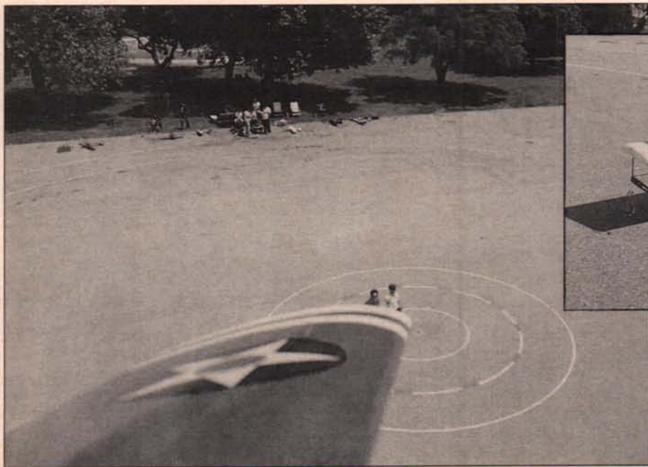
Above: Fred Cronenwett and Grant Heistand, both SoCal CL fliers, have been experimenting with in-flight photography from a CL model, with interesting results. The camera ship pictured here spans 71 inches, is powered by an O.S. .60FP and uses through-the-lines electronic controls for the 35mm camera, which can be turned 360 degrees as well as upward and downward. Left: One of the in-flight photos taken by the Cronenwett/Heistand camera plane. Site is Whittier Narrows, a popular RC/CL spot just east of Los Angeles.
