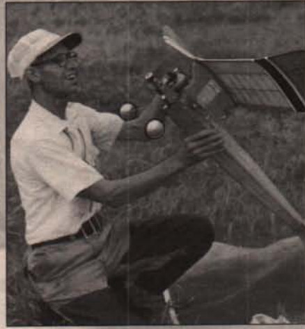
Warren Weisenbach, of Cleveland, Ohio, seen with a Forster .29-powered LaTorre "Alert." Note the lightweight wheels, made from the bottoms of aluminum beverage cans.
