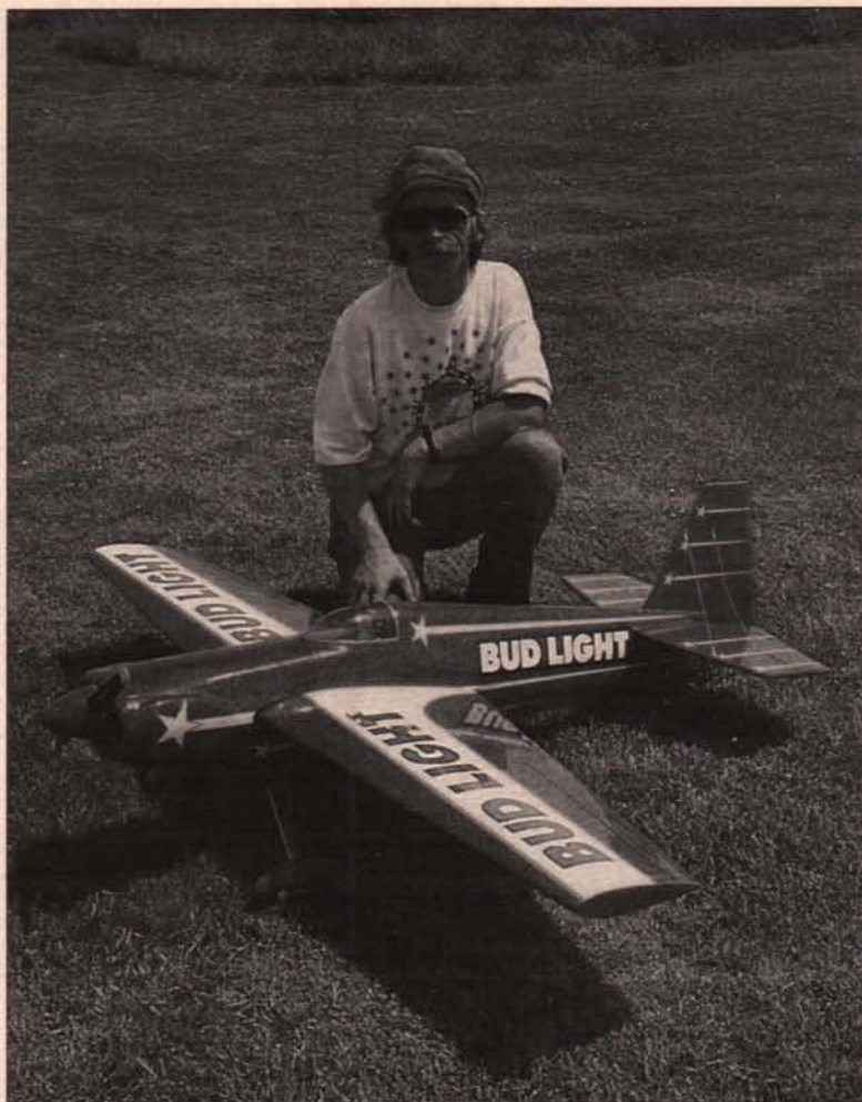
Andy McIndoe did a nice job of flying this Molly Models Laser 200. Power is an S.T. 2000. It weighs 14.5 pounds, wingspan is 74 inches.
