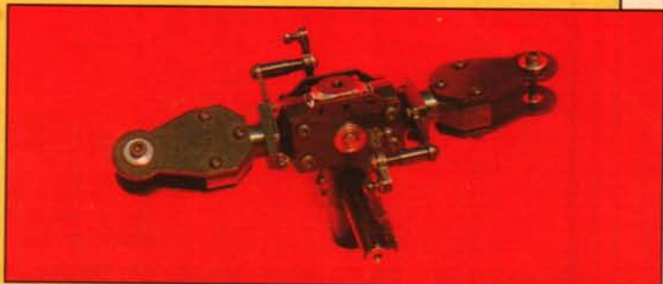
You're looking at the most solid 30-size model rotor head available. Of all-metal construction, it's almost bulletproof. The Bell-Hiller mixing arm on the blade pitch control arm is located out of line with the blade flapping axis, which gives some Delta-3 effect.
