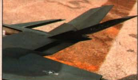
The F-117's control system is quite complex and requires some unusual mixing. Seen here, for example, is full up elevator command; note how both halves of the V-tail—and the ailerons as well—are deflected to produce a nose-up effect. Nothing is simple on this model!
