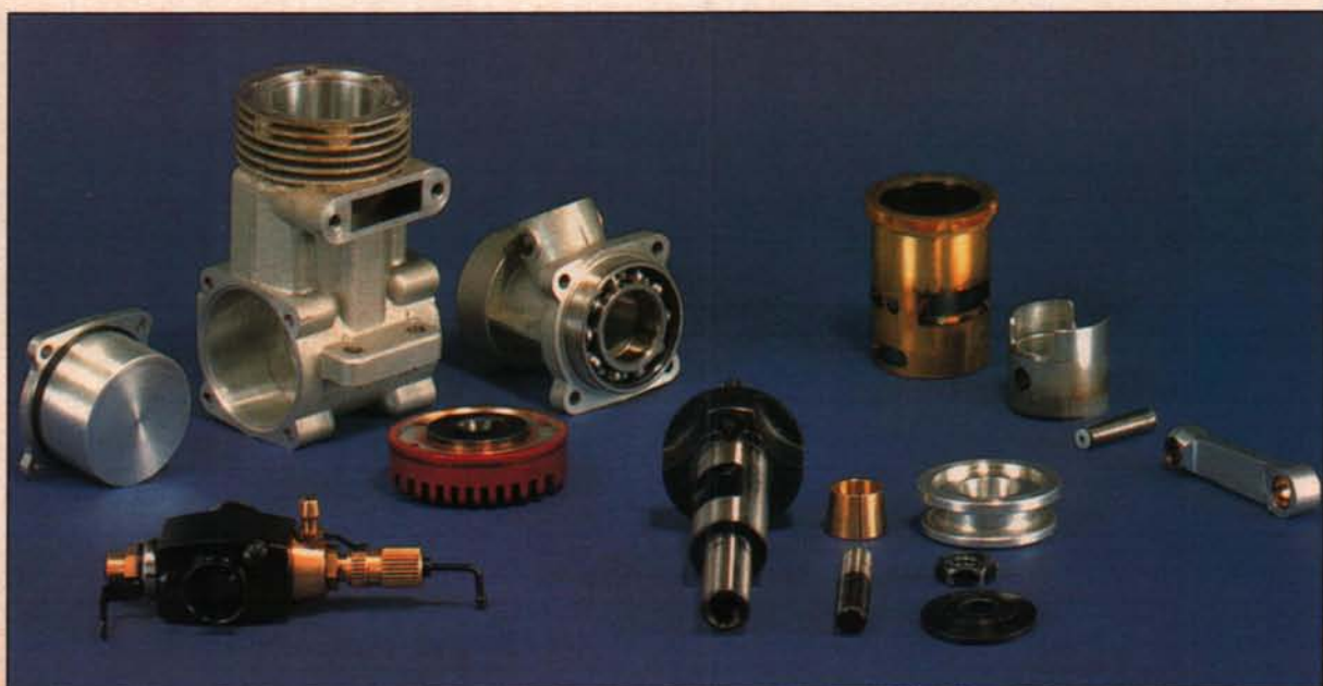
Parts breakdown reveals the stout construction typical of all Irvine engines. Crankshaft is the same as used in the Irvine 46, while the ABC piston/cylinder is from the Irvine 40 Diesel. This photo was taken after extensive running tests were completed, which explains the discoloration on some of the parts.
