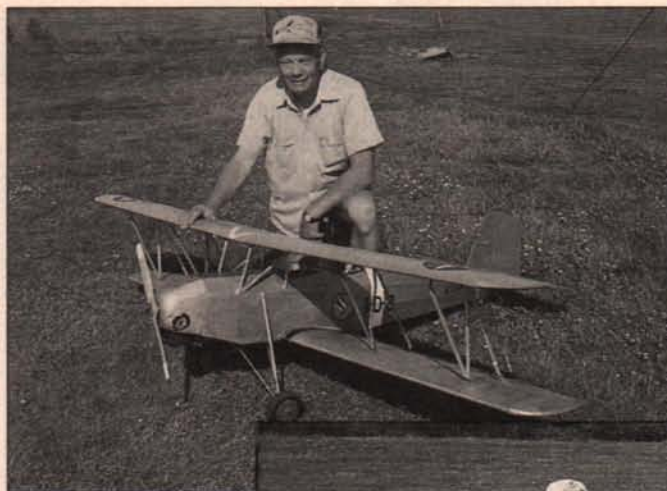
Tom Hammond enjoys flying his Curtiss Fledgling at the RCFCBC's Fry's Corner flying facility. It weighs 21 pounds and has an 8-foot wingspan. Power is a Quadra 35.
