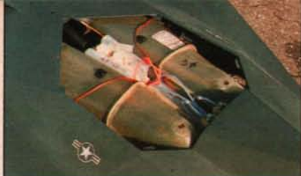
Removing the rear top hatch reveals the fiberglass ducting for the twin O.S. .91s, along with some of the fuel system plumbing. Fans are Dynamax units.
