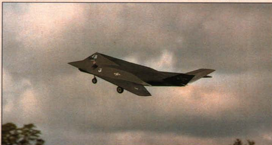
At an all-up weight of 23 pounds, the Yellow Aircraft F-117 delivers performance similar to that of a pattern ship. Needs about 250 feet to get off in no-wind conditions. See text for Bob Firenze's comments on how the airplane handles.
