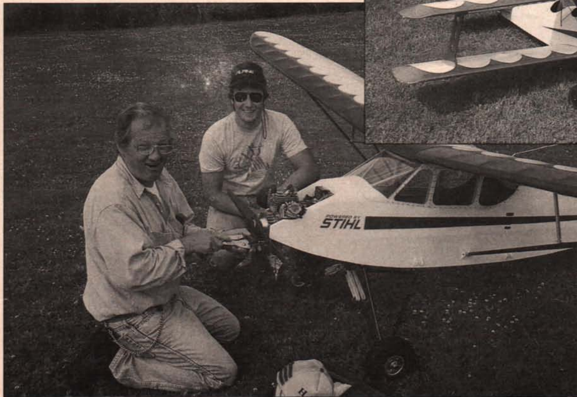
Bennie Phillips often opens Big Bird fly-ins by pulling the Stars and Stripes aloft. His Super Lazy Ace has a Quadra 52 for power and uses a Harris smoke system. The plane weighs 31 pounds and has a 96-inch wingspan.
