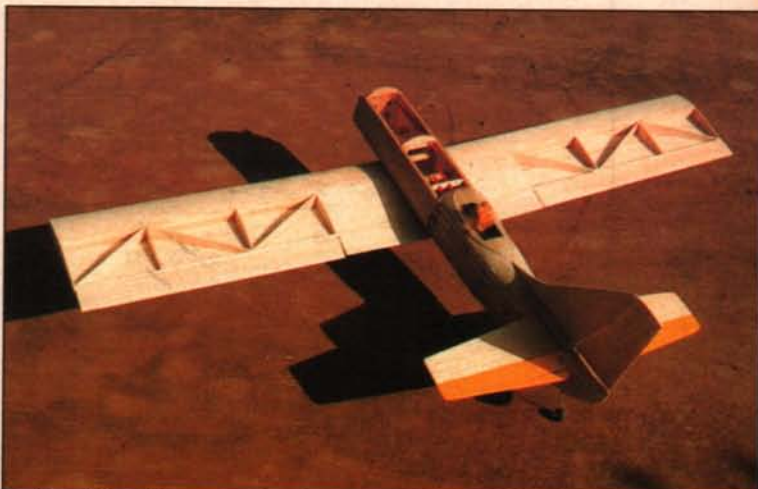
Uncovered framework reveals construction typical of AI's other EEE-Z-FLI efforts. Design can be easily modified with an open cockpit, slightly reshaped vertical tail and wingtips, etc., to create your own customized look. Be creative!
