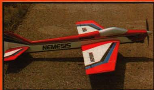
Mike Klein's Nemesis design. O.S. 1.20 SP power, 9-1/4 pounds, JR PCM-10 radio. This one carried Chip Hyde to the N-PAC title.
