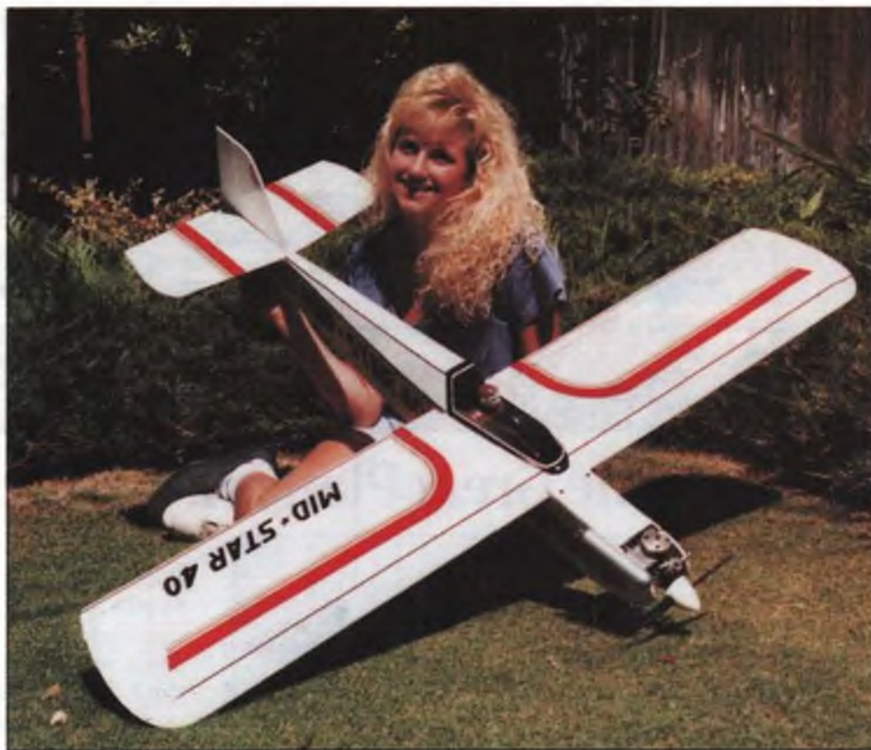
Kristine Adams poses prettily with hubby Kris's Mid-Star. Model is covered entirely with Sig's Supercoat iron-on film; colorful graphics—two full sheets of 'em—are supplied in the kit.
