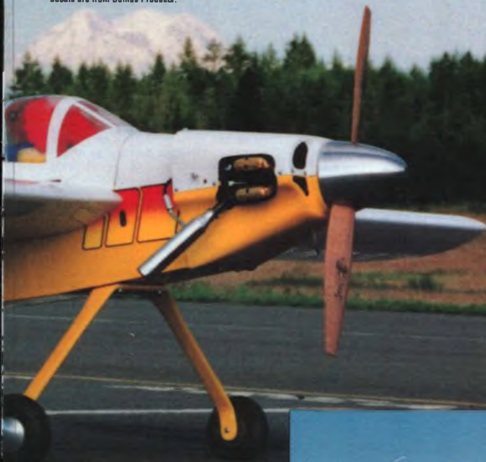
Rear view emphasizes the Stinger's large tail surfaces—no shortage of control authority back here! Tail braces ensure that the stab stays with the rest of the model during violent aerobatic maneuvers. The author's model is finished entirely with Coverite's 21st Century materials—palm on the turtledeck, cowl and landing gear, and film everywhere else. Wing decals are from Dumas Products.
