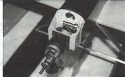
Removing the cowl reveals the Astro 25 installation on its built-up plywood mount. There's plenty of room up front for a geared Astro 40 and 18 cells, for those who really want to tear up the sky.
