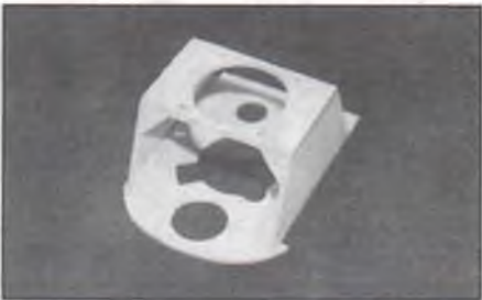
Motor mount is built of 1/8-inch plywood and gets epoxied to the firewall (F-1). Diagonal cutouts in the big hole in F-1 are to clear the Astro cobalt's brush holders.
