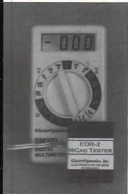
When plugged into the DM100, the Electro Dynamics EDR-2 NiCd Tester module provides a constant 220 milliamperes load to a cell or battery for true operational voltage readings.
