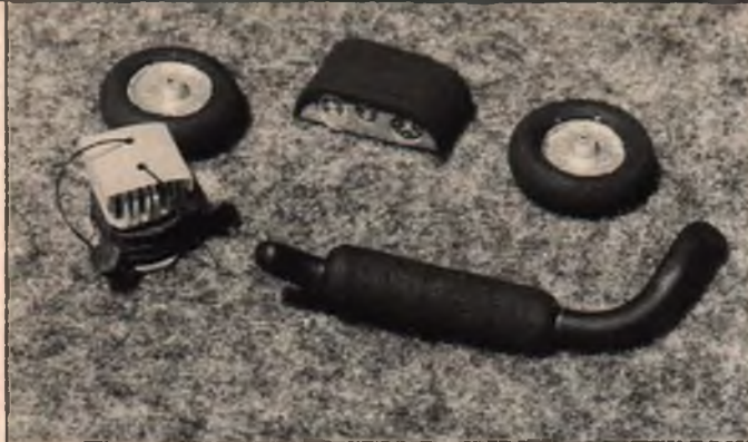
Scale details are made mostly from blue insulation foam and painted with water-based acrylic paint, which won't affect the foam. The finished motor and exhaust weigh only about 1/3 gram, which shows the benefits of using foam for non-structural parts.
