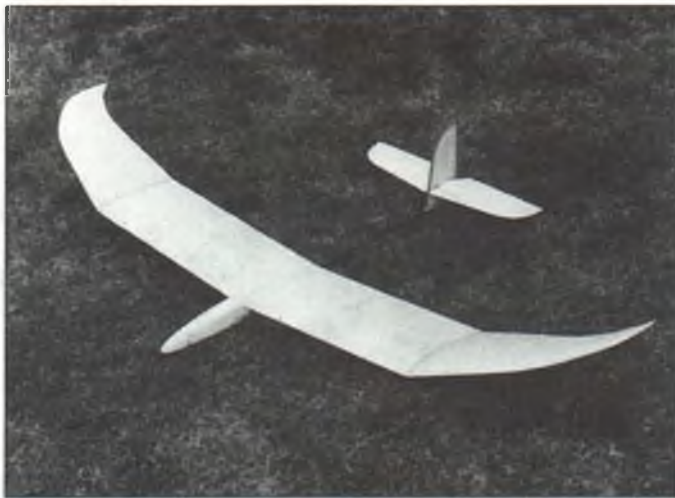
Recent correspondence from George Spitzer, editor of the F3B/USA F3F/USA newsletter. Included this photo of his modified Greco Technologies Javelin HLG. It features the SD7037 airfoil and foam-core wings V-bagged with multiple layers of 3/4-ounce glass cloth. Building a new plane was made necessary by a car burglary while George was on his way to a contest in Arizona.
