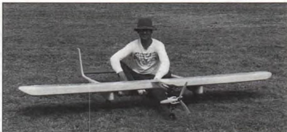
Dave Halley poses with his custom glider tug, dubbed "Andante." The 25-pound plane features homemade retract flaps and a full-flying horizontal stabilizer. It's powered by an Enya 1.20 four-stroke and does a good job of aerotowing large scale RC model sailplanes.
