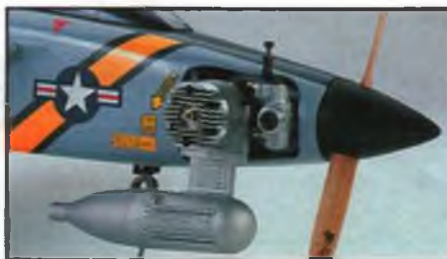
A front-mounted engine and prop provide familiar sport plane construction.
