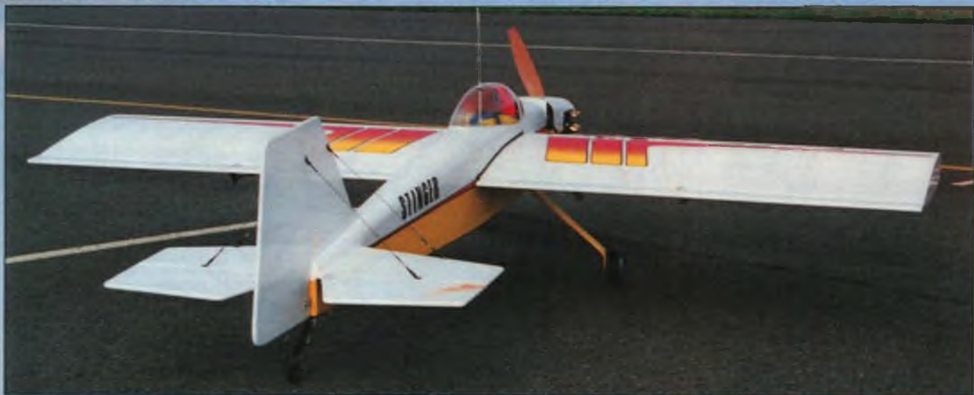
Rear view emphasizes the Stinger's large tail surfaces—no shortage of control authority back here! Tail braces ensure that the stab stays with the rest of the model during violent aerobatic maneuvers. The author's model is finished entirely with Coverite's 21st Century materials—palm on the turtledeck, cowl and landing gear, and film everywhere else. Wing decals are from Dumas Products.
