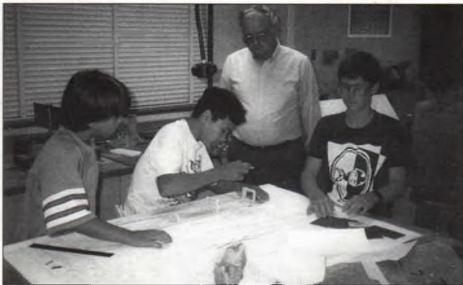
Once the bulkheads were constructed and square, they were applied to the fuselage. Emphasis was placed on gluing them at exactly 90 degrees to the fuselage sides and getting tight glue joints. Pictured from left: Robert Martinelli, Randy Padrique, Pat Payne (industrial arts teacher) and Ryan McCollum.
