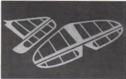
Tail surfaces are simple built-up structures of 1/4-inch balsa.
