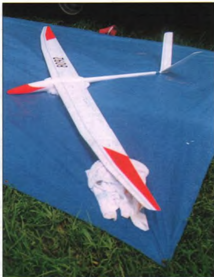
At the 1993 LSF Mats, Dr. Alan Schwerin photographed this beautiful example of the 130-inch span Magic Mk. II as produced by Weston Aerodesign (410-974-0968). Weighing in at around 70 ounces, Herk Stokely's ship has a wing loading of around 9.35 ounces per square foot. With its long tail moment, light wing loading and full-span turbulators, the Magic appeared docile on tow and reacted more graphically to lift than other models with lower aspect ratios.
