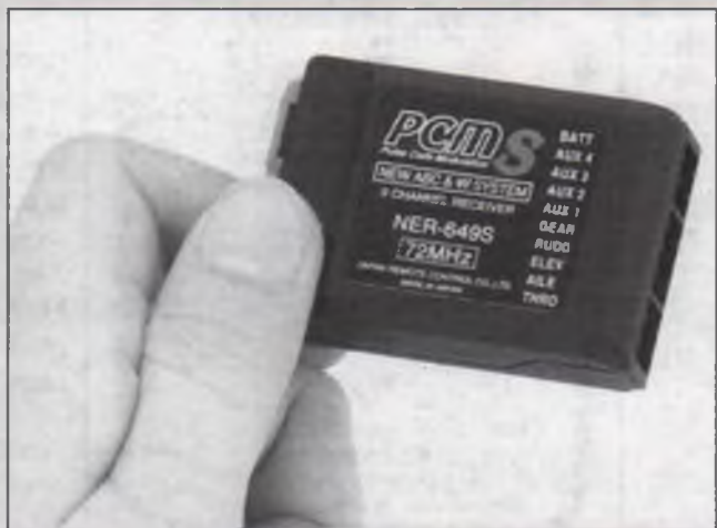
The X-388S heli system is available with four different servo/receiver packages. You can choose between a nine-channel NER-529 FM receiver or this latest nine-channel NER-649S SPCM unit. All four packages include five servos, from the 507 standards to the ball bearing, coreless 4131s.
