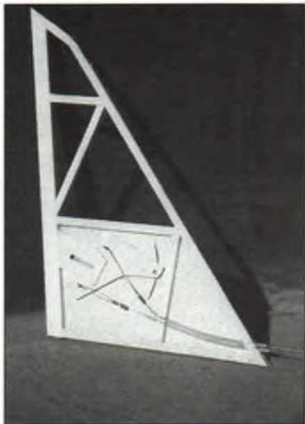
The Alcyone 2M has a full-flying stab, actuated by a pull-pull cable system, using Sullivan 1/32-inch stranded cables. Base of the fin is sheeted with 1/64 plywood.
