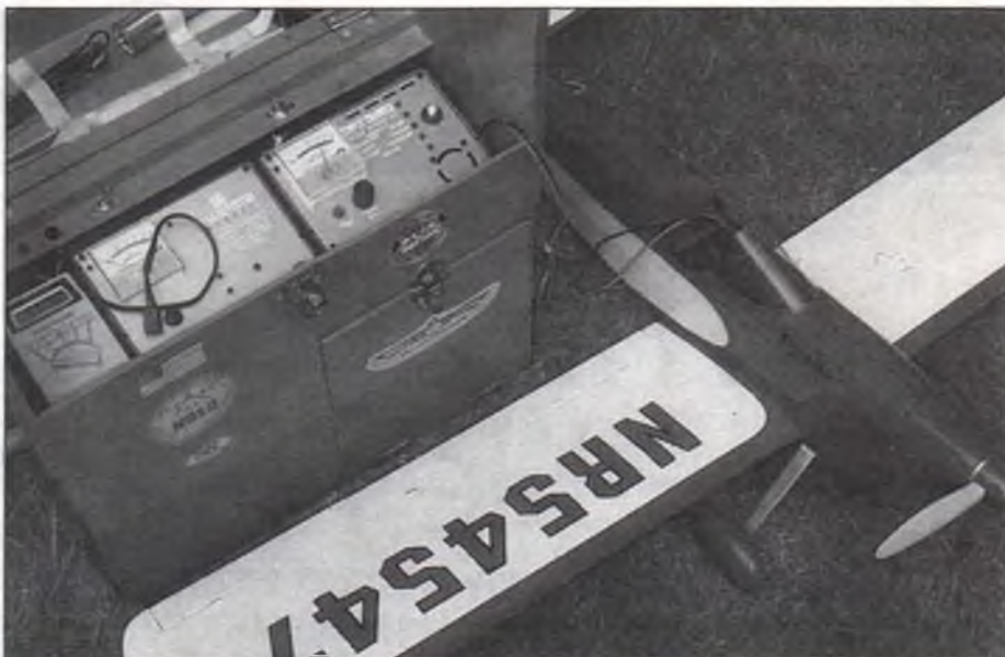
Bob installed his new Model 112PK in his field box alongside an old reliable Model 110. The toggle switch just above each charger's meter is used to turn on the input power. Here the 112PK is being used to charge the 14-cell system in one of the Tigerkitten prototypes.
