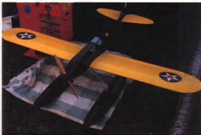
The Schneider Sport Electric is a versatile design that can be changed from wheels to floats or vice versa in a couple of minutes. Design is based on the Schneider Sport "wet power" models kidded by Stream, Inc., but with a completely redesigned structure. Floats, cowling, landing gear, etc. are all stock Stream units.
