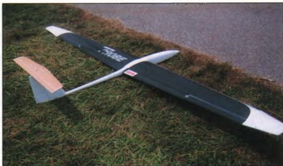
Terry Luckenbach attended the LSF Mats with his unlimited class Probe and also had a couple of two-meter versions. Design uses the thick, moderately cambered Eppler 214 airfoil, which seems to carry the weight very well. Photo by Alan Schwerin.
