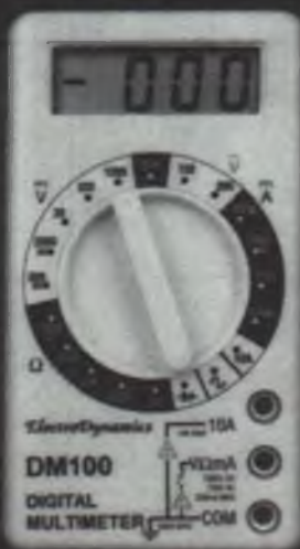
The Electro Dynamics DM100 Digital Multimeter, a small toolbox-size instrument useful for measuring all common circuit values. Looks good, too! A deep rich yellow! More in text.
