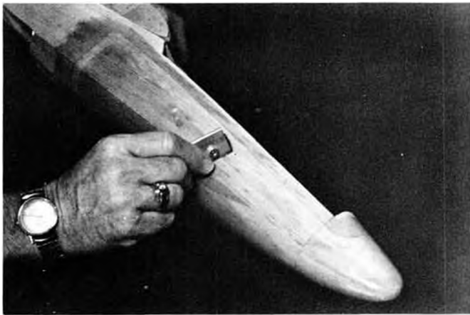
9. Final step is to scrape the resin surface with a razor until all shiny areas are removed. This is particularly important for Monokoting.
