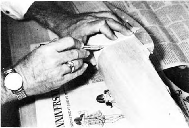
5. With a cutting guide such as a piece of file card, the excess cloth is trimmed, leaving a clean, straight edge. You're now ready to pour!
