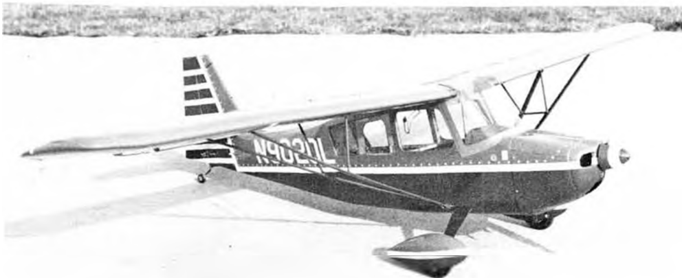
One of Sig Mfg. Co.'s new line of kits for 1972, the Maxey Hester designed "Komet." Wing span is 67", and the foam cored wings are available with balsa or plywood skins. Molded fuselage top.
