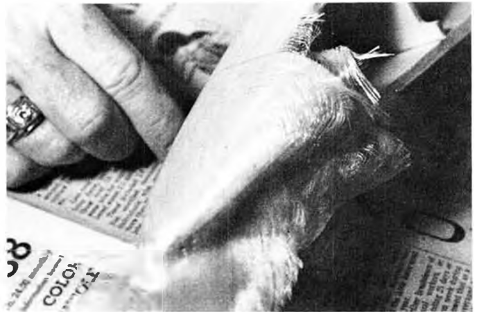
4. The cloth will follow the nose contours . . . with a little care. "V" shaped gores may have to be cut out to avoid overlaps and creases.
