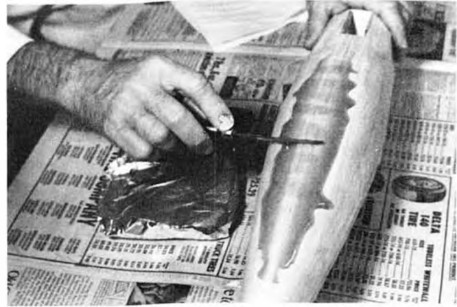
6. "If the phone's for me, I'm not at home." Does it ever fail? Note the disposable epoxy mixing dish . . . a piece of aluminum foil.
