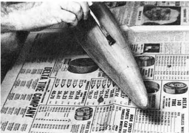
7. After spreading with the spatula, brush out the epoxy with a stiff bristled disposable brush. The better the job, the less sanding later.
