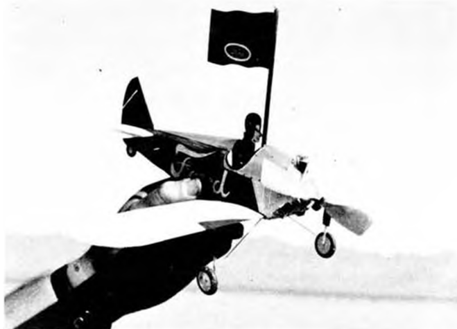
How's that for a wide tread? Now Ford can claim they had it before Pontiac! Little flivver is all sheet balsa for fast yet light construction.
