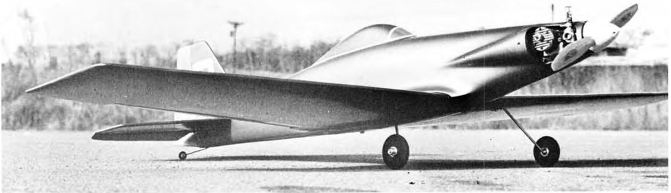
Ray Bingham's "Ballerina," built from K & K kit. Fiberglass fuselage, foam wing cores. Max .15 power, light blue acrylic finish. Roy Stephens pic.
