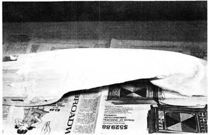
2. A single piece of fiberglass cloth covers all. Masking tape holds it in place as you get started. Two ounce cloth seems best for the job.
