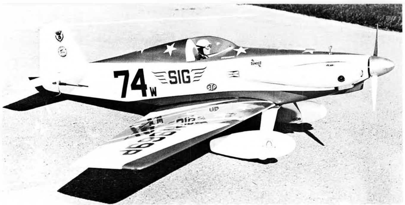
The "Mustang 450" is latest Formula I kit, a new release from Sig Mfg. Co.. Features foam cored wings, molded fuselage top and cheeks. $29.95.
