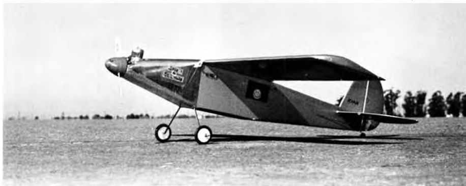
Seeing is believing! The winner at Mile Square was Carl Weyl's "Spirit of St. Louis" with Fox .15 power. Plane had Kraft KPS-9's, big pack, six channel receiver. Still weighed only 2.55 pounds.
