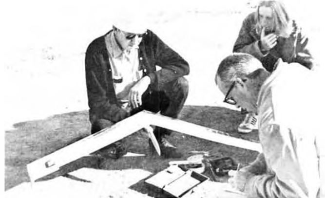
A/1 Class original by Bob Provart, Newbury Park, Ca. "Counterfeit" design has 25 degree sweep, 270 sq. in., body falls away for D/T.
