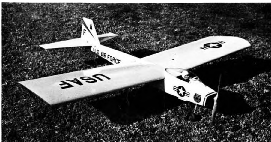
Latest Jack Stafford kit, available in late January, is the Weekender. It has completely finished, balsa-on-foam wing panels, 1/4 inch sheet fuselage, 3/8 inch tail surfaces, weighs 6 pounds, uses 45 to 60 engines. Thick 800 sq. in. wing makes plane an excellent sport-pattern-trainer. $39.95
