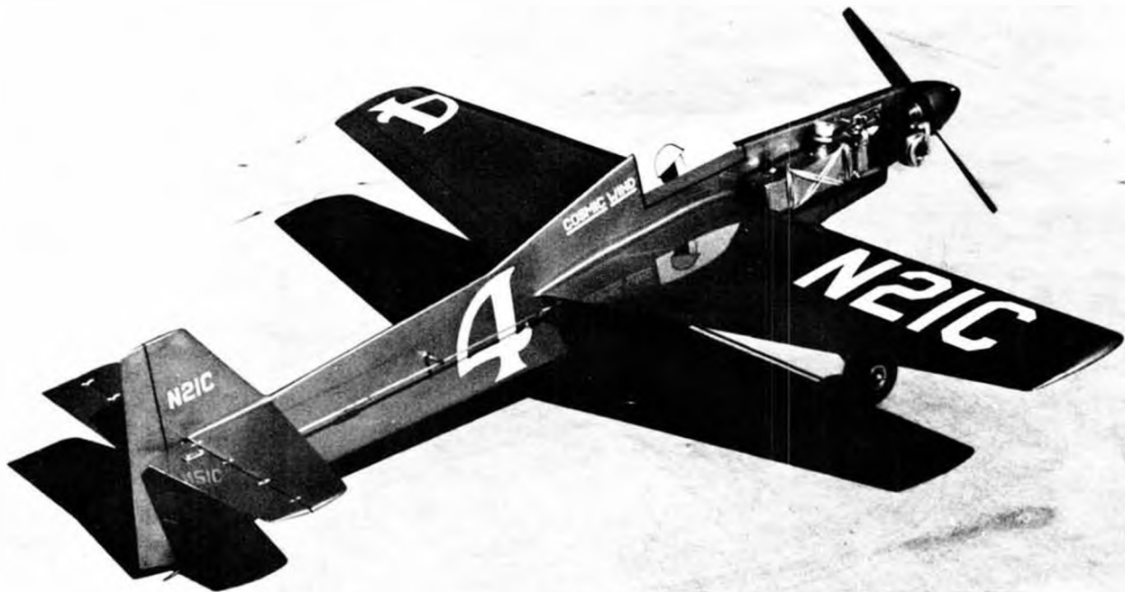
Profile AMA Goodyear Scale racer by John Penhallow. Ship is Cox .15 powered and has cut-off to predetermine landing spot.
