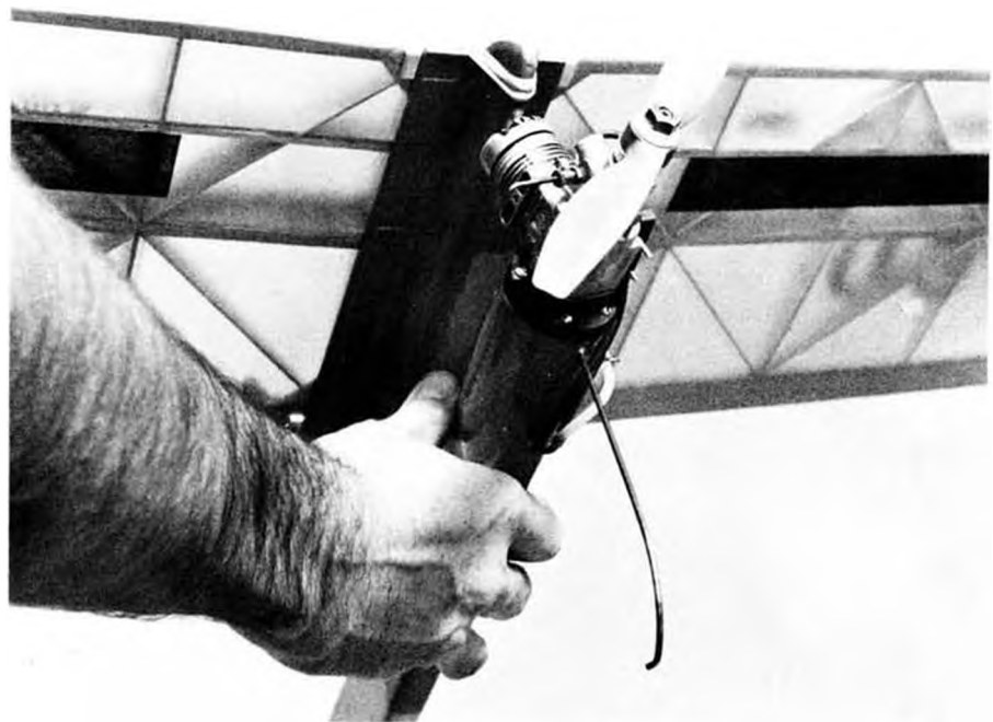
Geodetic wing structure prevents high speed wing flutter. Fuselage fairs neatly into Kraft-Hayes glass filled fiberglass molded engine mount. ST G/20 .23 is tilted for access to plug.
