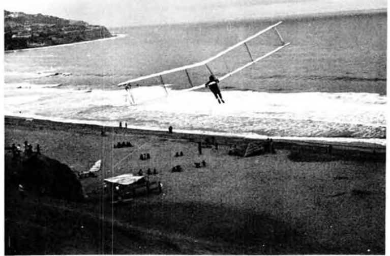
This swept-wing biplane has outboard rudders, giving excellent directional control. Well designed glider made some of best flights of day. Scene was hang-glider gathering at Torrance Beach, California.
