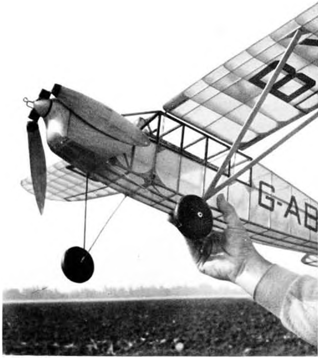
Jumbo Scale rules required a free wheeler prop, but the original plane used a folder like this one. Hal finds trim changes needed for each.
