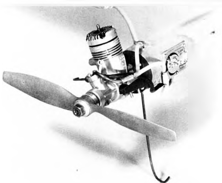
The business end of "Shocer" showing the plumbing hook up for the Tatone "Flood-Off" timer. Copper tube directs fuel to venturi, giving instant shut-off. Wire skid protects prop and engine on D/T landing.
