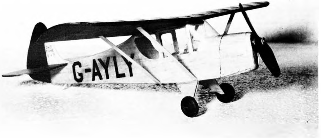
This little peanut is a natural flier on CO-2 or rubber. A little small for a dethermalizer, so have your track shoes handy just in case!
