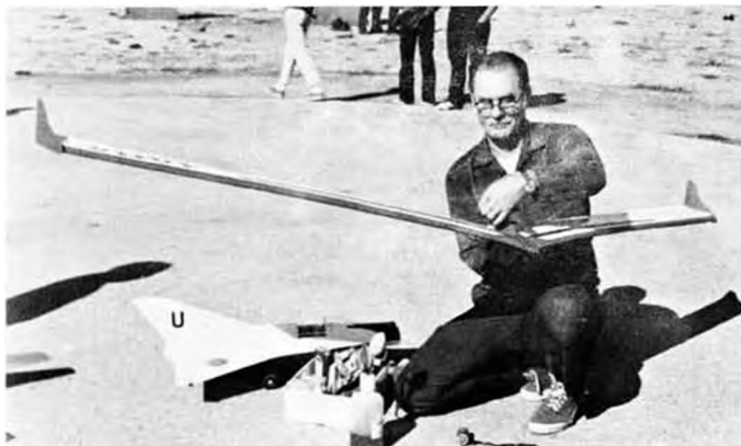
Wayne Schindler assembled 6 Ace Mini-foam wings to make this 8 foot model. Cox .049 power with pusher prop and Tatone cut-off.
