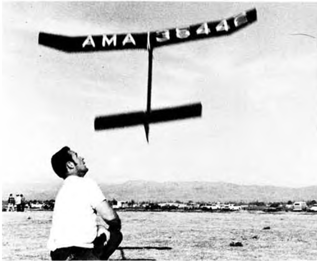
Don Zink's "Shocer" accelerating from VTO takeoff. Flight times exceed 4 minutes for 8 second power run in dead air.
