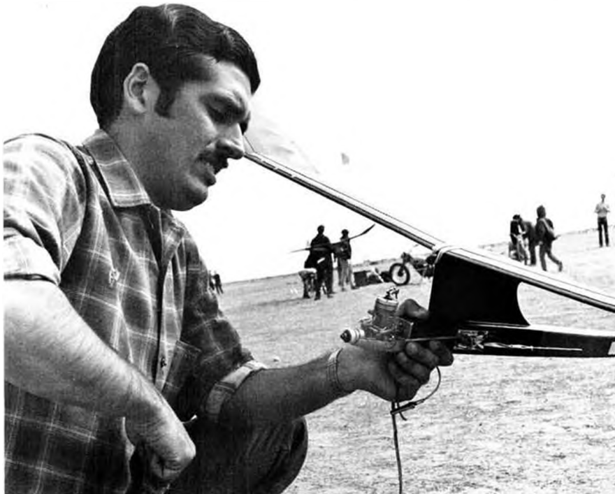
Walt Ghio starts up his FAI power ship. Note turbulators applied over sheeted leading edge. Are you smiling, Le Gray? Timer is a Selig four-operation unit. G20/15 Supertiger.
