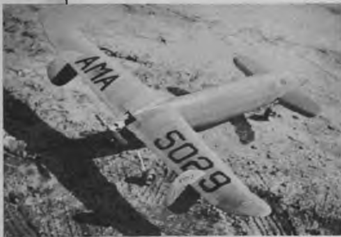
This canard design weighs 30 ounces, seemingly heavy for a B motor. But "tail" carries nine ounces of the weight, wing 21 ounces.
