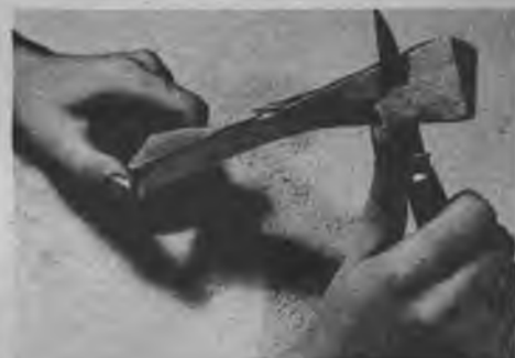
Drill the prop-shaft hole, carve out the blank, and then rough out the two inside faces as shown above.
