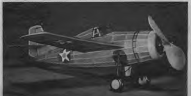
Under view and tuck-up wheels for a Jap view of the Wildcat. Note the well-proportioned prop with free-wheeling, for astounding performance.
