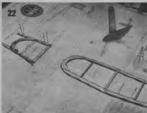
22 The finished stabilizer with rudder "in the works." Note, for structural reasons, never place pins in wood.
