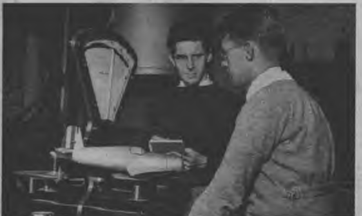
Bob Crawford, facing camera, and Frank Wolak weigh in a navy Vought-Sikorsky XF4U-1 model for free-spin tunnel. This model has both rudder and elevator controls.
