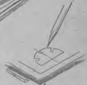
Carbon paper is handy for tracing full size plans -
