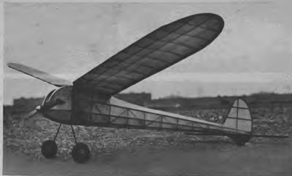
Try this job on your Class B motor and see for yourself the advantages of hardwood construction. Note neat built-up cowl.
