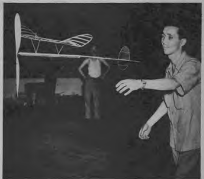
Here's how to launch the featherweights. The wings on this stick model are braced with tungsten wire for rigidity. Propeller turns at about 75 r. p. m.
