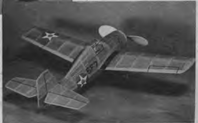
Can you tell it from the big brother? The Wildcat includes large tail area, ample dihedral, which are necessary for all successful flying scale models.
