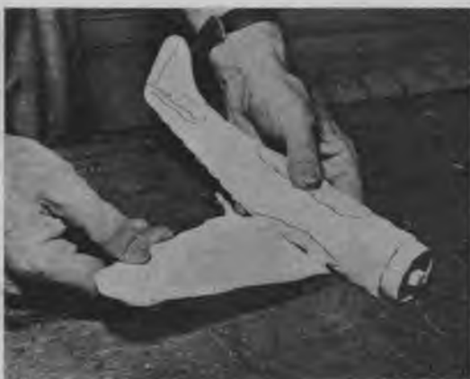
Wings fit smoothly into finished fuselage. Rigby has developed different types of wing fittings to simplify assembly.
