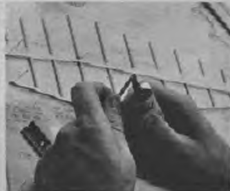
5 Cement crosspieces in position. Use plenty of glue and be careful to see that they are properly spaced.
