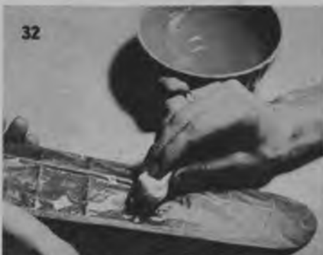
Tissue tightened by using water applied with cotton. Wet thoroughly, allow to dry, then dope one coat.
