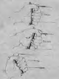
Primary flying position control for level flight, diving and climbing.
