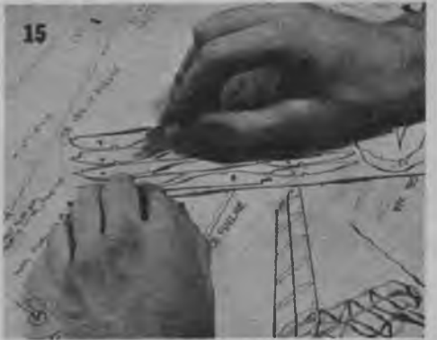
15 Cut all ribs and other printed parts in one step to save time. Use a sharp razor blade for this operation.
