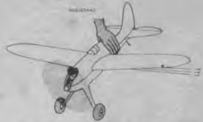
Assistant holds plane for take-off. Lines must be taut at all times for good control.
