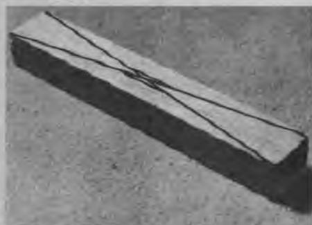
First step after selecting the correct size block is to draw in the diagonal lines on top and bottom.
