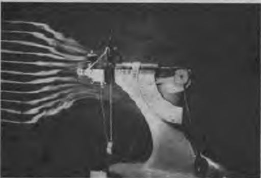
Another example of clean propeller design showing a smooth airflow along the blade with little disturbance near the hub.
