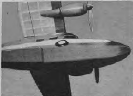
Under view of hull shows details of engine-nacelle assembly.
