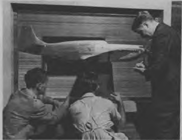
Takes a master model maker for this job. Many laminations of mahogany are used for accuracy. Tunnels heat up, require cooling.
