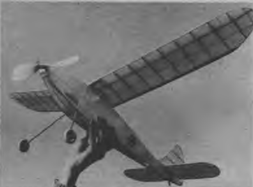
● A Wakefield type with a free-wheeling prop. Made of ersatz material, it flew well and met weight rules.
