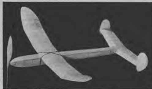
● This little stick job features dihedral in the stab and twin rudders.
