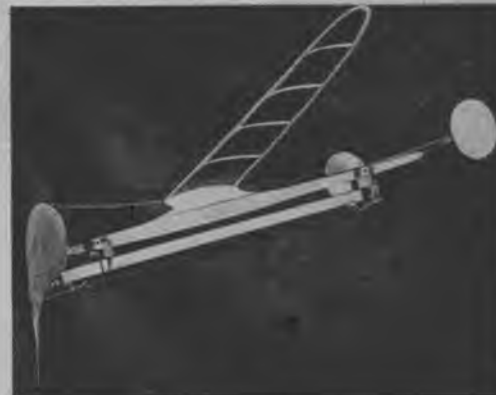
● The rubber motor and motor stick dropped off at end of power run.
