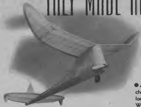
● The Zombie by Shulman. Another one-wheeler with tip skids on the stab. It has the usual Shulman features: low thrust and retracting gear.
