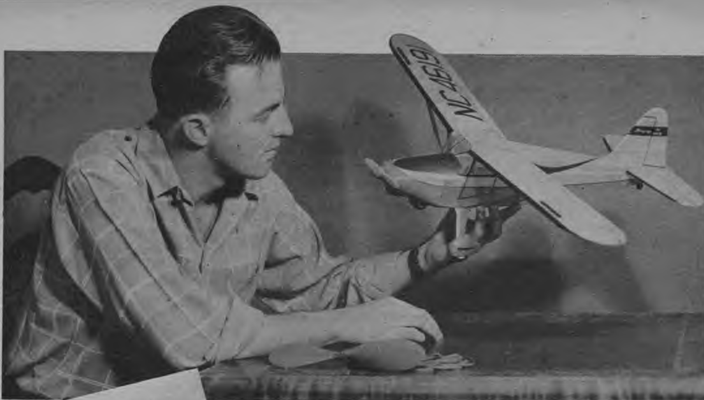
● The author displays his model. Note the flying and scale propellers, finish and scale details.
