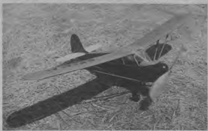
● Struck's Interstate Cadet set a new high in endurance at the '41 Nationals. Beautifully finished, it featured generous blade area and a free-wheeling unit.
