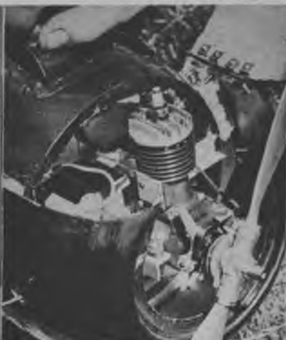
● A flying scale installation. Note scale prop and gas tank in the top of the fuselage cowl.
