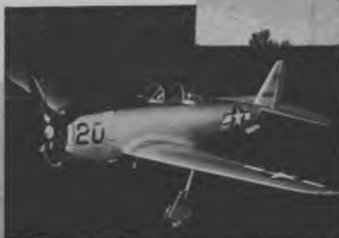
● P-47N with 4-bladed prop and sliding canopy.
