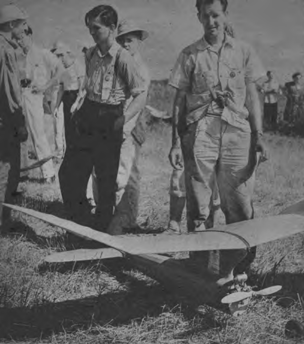
● Comet's Sailplane was the most consistent winner in the field of the large gas kits. Designed by Carl Goldberg, it featured a pylon wing mount, generous wing area, and retractable landing gear.
