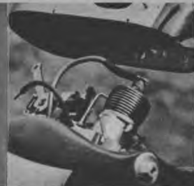
● A unique motor installation in which the entire motor and ignition system is removable.
