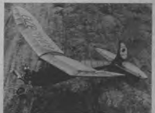
● This little Atom-powered cabin job featured a very fast climb and soaring glide with a low sinking speed.
