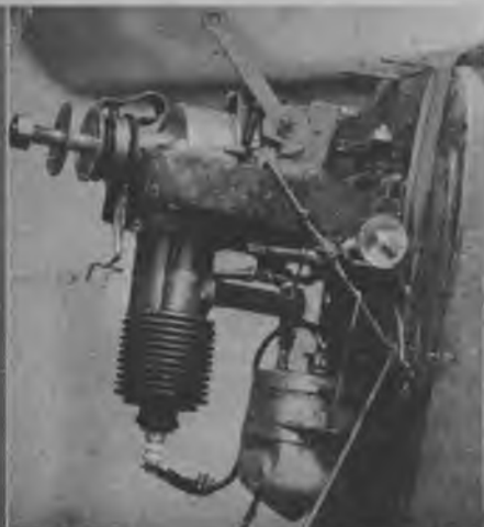
● In this mounting, the motor timer is mounted directly with the motor. Note needle valve.
