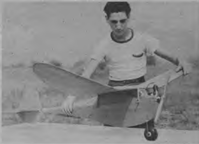
● Schoenbrun's Rocketeer was among the first single-wheelers. It featured a deep bellied fuselage, high thrust, and the innards deep down in the fuselage.
