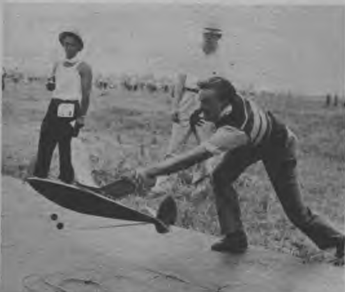
● Roy Nelder's 1938 and 1940 Moffet trophy winner. This model featured a rectangular fuselage with a high aspect ratio wing and a tremendous climb.
