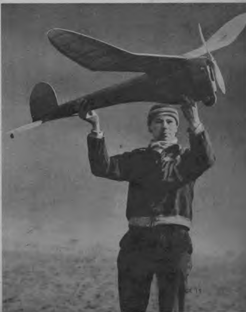
● Struck's Record Hound—the 1939 NAA record holder. This gassie featured cathedral in the stabilizer, inverted motor, and a single-wheel landing gear.
