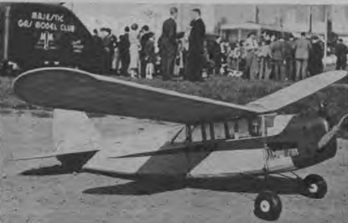
● Berkeley's Super Buccaneer is another famous kit model. It is a colossus among class "C" models. Here is Raspante's radio-controlled version.
