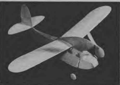
● Imagine rubber without Garami! This little duck of his featured a sheet balsa fuselage and a retracting gear.
