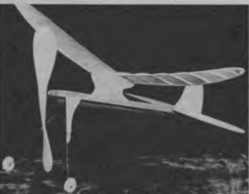
● A simple little ROG that performed very well indoors and outdoors. Note landing gear fairing and spar-less wing.
