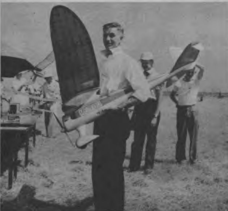
● A super-streamlined Sailplane. Note the revisions of the original design, the streamlined landing gear, the engine cowling with the air scoop on top and the side vent.
