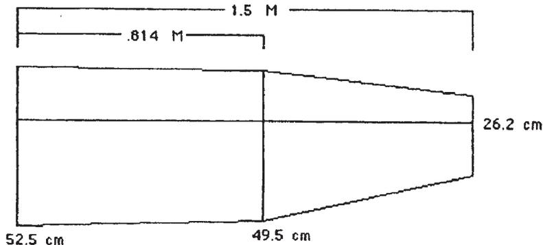
Washout 0 deg. Mass 4.050 Kg. Wing loading 3.00 Kg/sq.m.
