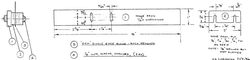
First, the construction. Material for the spacers can be plywood, fibre board, etc., but it should be exactly the thickness indicated (1/32", 1/16", 1/8"). All spacers measure 3/4" X 2". Cut two pieces from 1/32", one from 1/16" 10 and six from 1/8" material. The spacers can then be stacked
