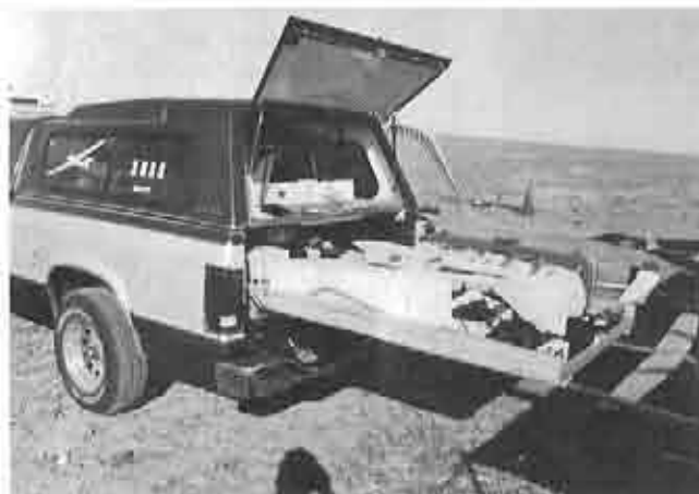
Tom Overton's method of transport. Each level easily rolls in and out and is designed and organized to hold wings and fuselages neatly in place. Photo by Lee Murray.
