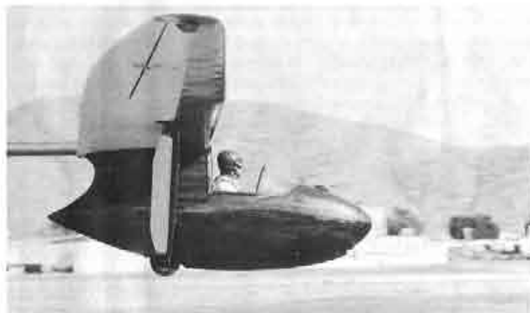
Bowlus Baby Albatross on tow. This glider had a mahogany plywood fuselage, with a finish like a grand piano.
