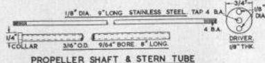
FIG. 23. PROPELLER SHAFT & STERN TUBE.—The shaft is a piece of brass tube of the size shown. This gives an easy fit for the \frac{1}{8} in. shaft, but a \frac{1}{4} in. brass blank should be turned to fit each end and the end of this accurately drilled \frac{1}{8} in. clearance. It is a good idea to fill the tube with hot vaseline before inserting the shaft.
