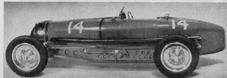
Nearside view, showing oil-cooler on the side-member. The unique "3.3" wheels are magnificently reproduced with full spoking.
