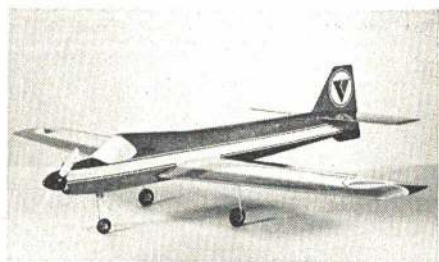
At rest on the gear, Viper has that look of ready action. Note the moveable sub-fin. This is most helpful in wingovers.
