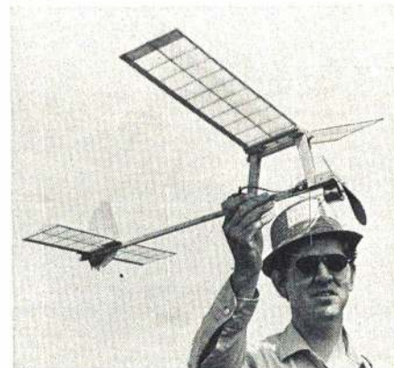
David and Carol Kruse, Minneapolis. Models are stick-and-tissue and foam. Free-flight duration model uses 50 cent Mabuchi RE56 motor from Radio Shack.
