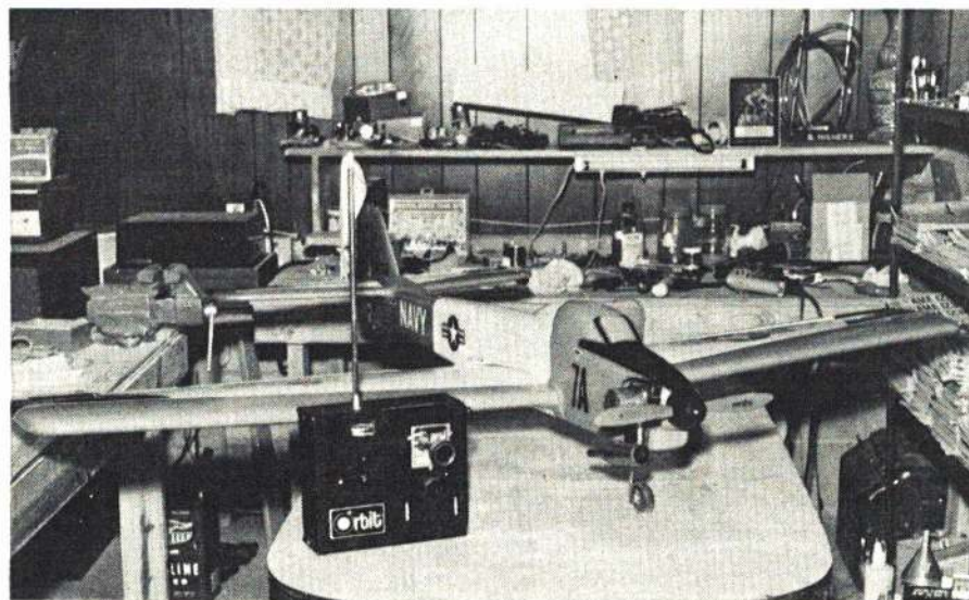
Top: In addition to the above parts, the Custom systems also include all servo trays, frequency flag, an excellent instruction manual, and plenty of servo output arms. Above: New Orbit single deck receiver. It now operates at full range between 4.8V down to 3.6V. A one-cell battery failure is not a guaranteed disaster as in the past. Left: New feature in the transmitter is the attached service record card. The technician who does the work also signs the card. This speeds service and assures quality work. Below: Workshop effort on the Intruder is finished—now for some flying.
