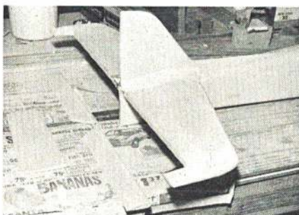
Top: The Intruder is typical of all SkyGlas kits. Finely-detailed and precision-joined fiberglass fuselage with foam wing and stab cores. Sides are actually joined while still in original molds and there's very little flash or gaps in the joints. Above left: Every builder has his pet materials. Van Highers strongly recommends Weldwood water-based contact cement for skinning wings and stab. The skinning job is about an evening's work. Above right: Spackling compound is great for filletting the joints of the tail surfaces with the fuselage. It sands easily, too. Left: The muscle up front is a Blue-head Supertigre 60 equipped with Perry carburetor and flow-through type muffler. Remember to balance the plane for the side-mounted engine. Below: Most fun part of all Blue Ribbon Reviews is flying. The Intruder is an excellent ship for a sport flier with a grass field. It even stunts nicely at half-throttle.
