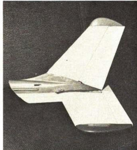
Here a plastic R/C job was repaired using inside doublers; then inside was foam filled.
