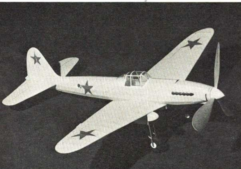
In modeling this unusual Russian aircraft, few modifications were needed. Long nose and long wing are perfect for rubber power. Painted all-white.
