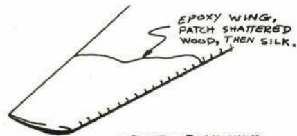
BROKEN FOAM WING
