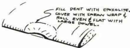
FOAM WING REPAIR
