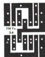
FIG. 2: Add-on board (above) accepts IC and timing capacitor. Terminal strip board (right) is for use with slider pot to get third channel—as seen in upper left corner of single stick Tx. Negatives of both boards are available through AAM Plans Service.
