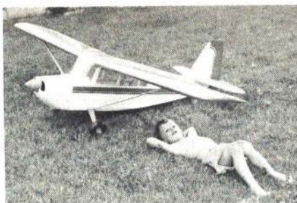
Sureflight/Citabria. Huge, eight-ft. span Stand-off Scale ship features all-balsa construction except for a vacuum-formed cowl. Plane has over 1500 sq. in. of area but, because of light wing loading, will fly on a good 60 to 80 engine. Should have a good scale effect. $125. Sureflight Products, 656 Nome Rd., Valparaiso, Ind. 46383.
