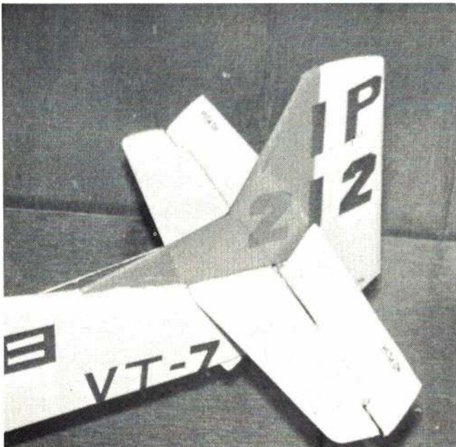
TOP: The T-28's bold outline fits even the most basic color schemes. Navy versions, usually the most popular, have easy straight lines to paint. Easy, smooth lines can be achieved with basic building skills. ABOVE: Large amount of elevator travel shown here is not necessary for good performance, but a free-moving linkage is!
