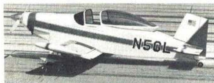
"Thorpe 18," an Experimental Aircraft by Ralph Burnstine, Danville, Ill., won the EAA Homebuilt Scale Special Award in CL at the '73 NATS. The Thorpe featured throttle control, sliding canopy, finely detailed instrument panel and cockpit, and electrically driven flaps.
