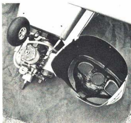
Nice and clean before the first run-up. The interior of the wood cowl has been shaped and finished. It entails much less work than fiberglass construction because of the simple curves.
