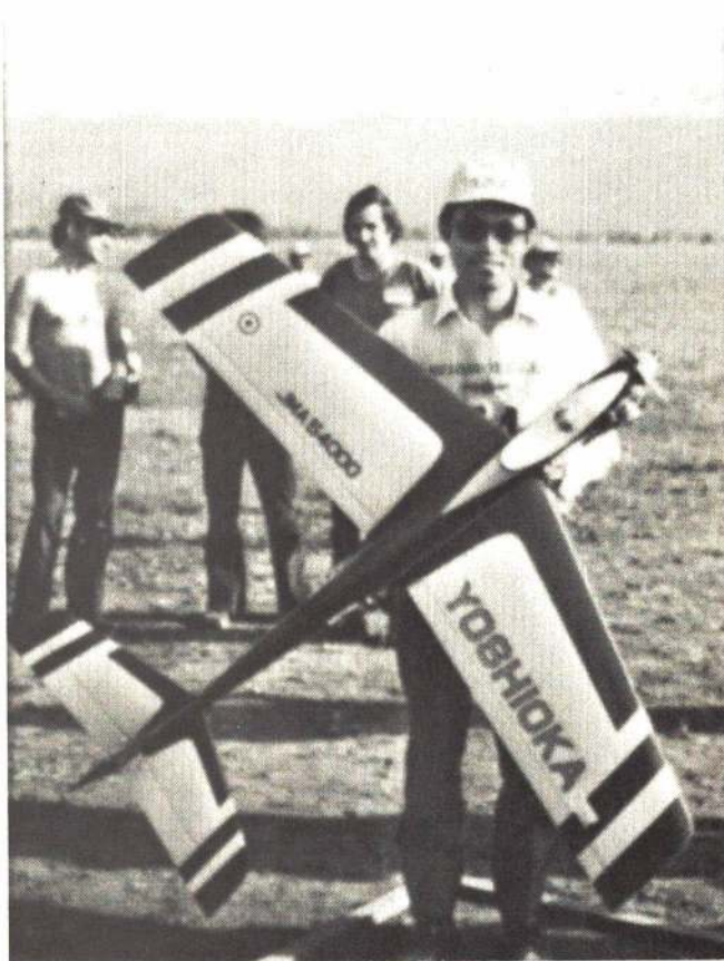
Yoshioka's winning model illustrates superb craftsmanship common to all Japan's entries. High degree of wing sweep by U.S. standards, yet an otherwise straightforward design. AAM will publish a full construction article on this design in the future.
