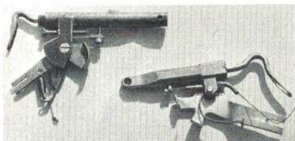
Lepp's (USSR) glider tow hook gear is made from brass. The mechanism is supported and pivoted through the hole at the end of the main pillar.
