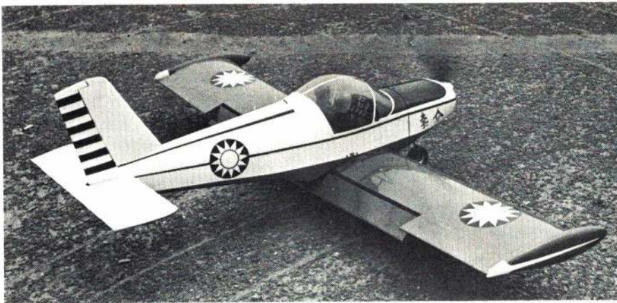
Taxiing back after the first flight. Author reports that the flaps slow the model easily; this makes up for the rather high wing loading and low power loading. Full flap movement for landing, but only small movement for takeoff.
