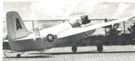
Rossi 60-powered Guardian by Gene Wielms of St. Louis. Note release for tailhook and rubber band to pull down hook.
