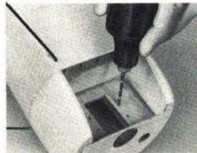
Drill engine and equipment mounting holes.
