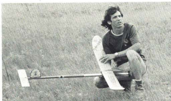
Nineteen-year-old Jon Davis of Albuquerque kept cool, waited for good air, made Wakefield team. Aluminum tube fuselage.
