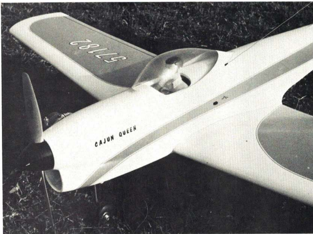
This is the retract equipped version of the Queen. That air scoop below the engine gives ample space for the nose gear unit and access to its mounting bolts.
