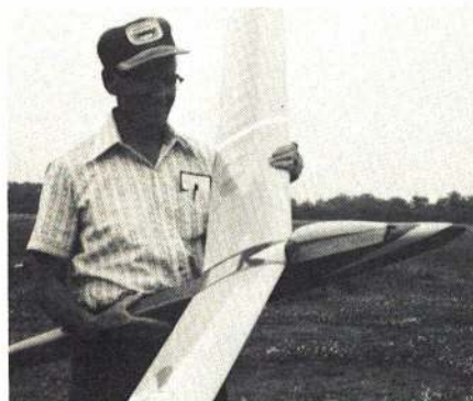
W. Zehr and his original design—Zehrgutt—in which he reversed a Du-Bro canopy to fit a glider.
