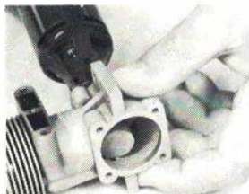
Polish intake ports. Lighten pistons and rods.
