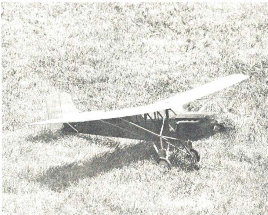
Being a slow flyer with a large wing, the model will take off from close-mown grass.
