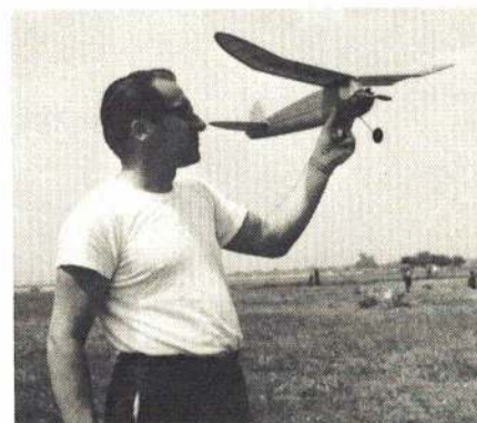
Bob Oslan's 020-powered Brooklyn Dodger weighs in at 4½ oz., flew right off the drawing board. Very docile—seeks out thermals as though it had radar. Now kitted.
