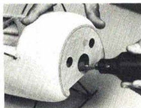
Sand and shape wood, fiberglass and foam parts.
