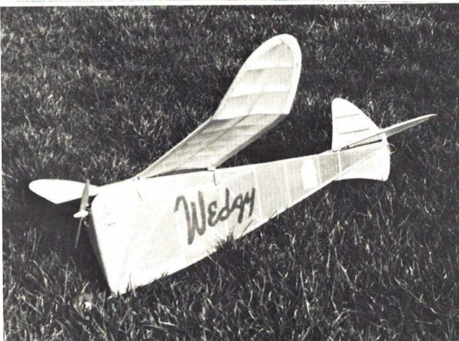
TOP: Wedgy shows the origin of its name. Bunches of side area don't detract from performance a bit. ABOVE: Power is a Cox 020 hidden inside the snout of Wedgy. Fuel shutoff is adjacent to engine to make everything accessible.
