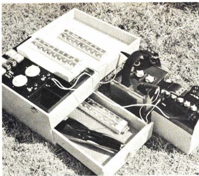
Charging modes are either elaborate, where the master charging unit at left can charge several battery trays simultaneously, or the simple portable charger which operates off the car cigarette lighter.
