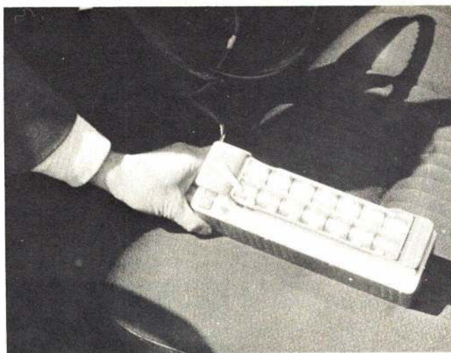
Charging modes are either elaborate, where the master charging unit at left can charge several battery trays simultaneously, or the simple portable charger which operates off the car cigarette lighter.
