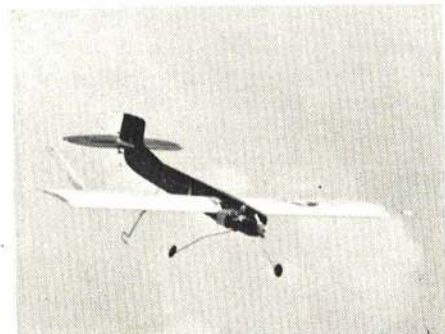
Joe Tracey's (Eliria, Ohio) Profile Carrier came apart during this flight. Note aileron is disengaging.
