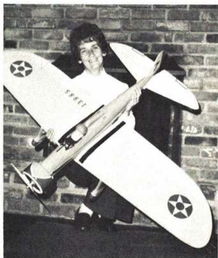
Donna Sheeks holds her husband Jack's original design, his P-26 Peashooter, a Semi-scale Stunter. Wingspan, 61 in., ST 46-powered. (Photo by Jack Sheeks)
