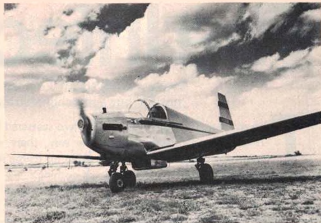
Very early production M-18 Mite displays super-clean lines. Radiator for its liquid-cooled Crosley Cobra engine rides beneath the fuselage. (Photo courtesy Smithsonian)
