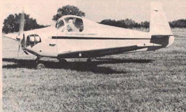
The author's beloved Mite, as depicted in the drawing on next page—all yellow with black trim, complete electrical system, starter and generator. Gross weight (including author) 850 lb.
