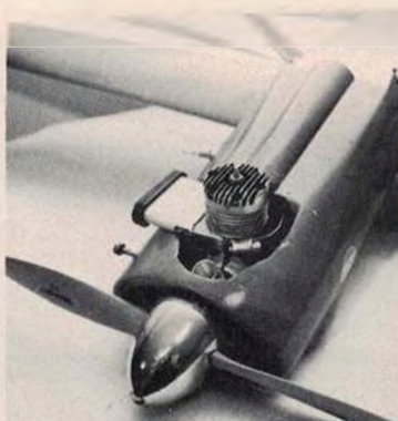
LEFT: All stunt fliers are wise to the advantages of a commercial foam core. They go together fast and don't warp. CENTER: The Max 40 and Du-Bro muffler got there mysteriously—note that there is no removable cowl. RIGHT: The rudder is manually adjustable. The ring on the tail wheel wire is for a stooge (see page 46 for details on how to build this helpful device).
