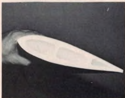
LEFT: All stunt fliers are wise to the advantages of a commercial foam core. They go together fast and don't warp. CENTER: The Max 40 and Du-Bro muffler got there mysteriously—note that there is no removable cowl. RIGHT: The rudder is manually adjustable. The ring on the tail wheel wire is for a stooge (see page 46 for details on how to build this helpful device).
