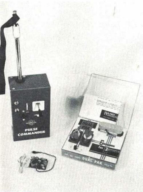
ACE Radio Control/Pulse Commander System. Transmitter and Dual Pak provide 2-channel pulse proportional control for planes up to 29 size. Full-house version of unit covered in Jan. Check List. Dual Pak includes two actuators, receiver, 1-amp 3.6v. Nicad. Price, $139. Charging gear extra. ACE Radio Control , Box 301, Higginsville, Mo. 64037.
