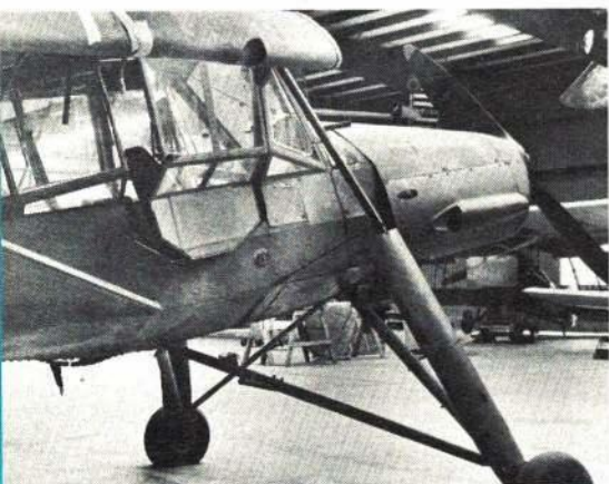
Projecting greenhouse cabin gave excellent downward vision. Picture top of page shows folded wing, full-span Handley-Page slots.
