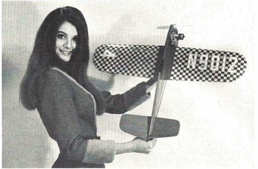
Some flyers like the circular bellcranks for smooth linear control. Regular cranks also are fine. Right, cheerful young modeler displays a Sweeppea powered by a Supertigre 35. Covering is checkerboard silk.
