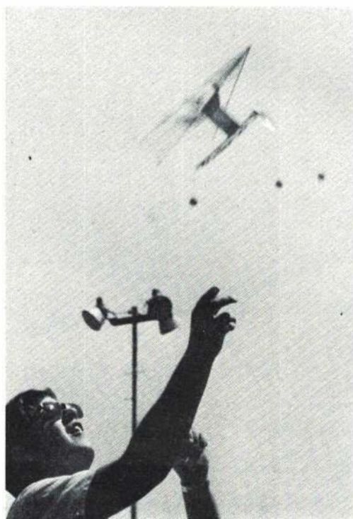
Above: Bill Watson holds his own flew-wing type model in right hand, author's Insect in left. Holes in pylon were punched two at a time until correct power turn obtained. Big pylon overcomes left turn due to prop torque. Left: Watson launches Insect No. 3 for powered climb on 5/32" Pirelli rubber.
