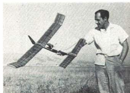
Earl Thompson's 1/2A canard is a really fine contest performer with straight climb and excellent glide. Thrust is right at the C.G.
