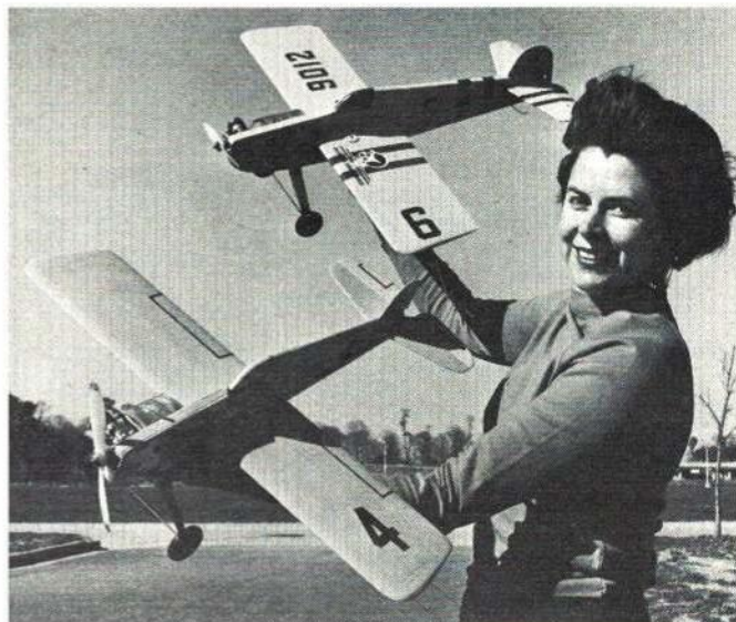
Although the models look like racers, they make fine trainers too. Just mount the prop backwards and fly at a slower speed. Solid wing and sandwich fuselage are extremely strong. Rugged gear too.
