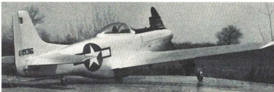
Myers' Mustang has big flaps and auto rudder. Uses Rossi 60 with homemade throttle.
