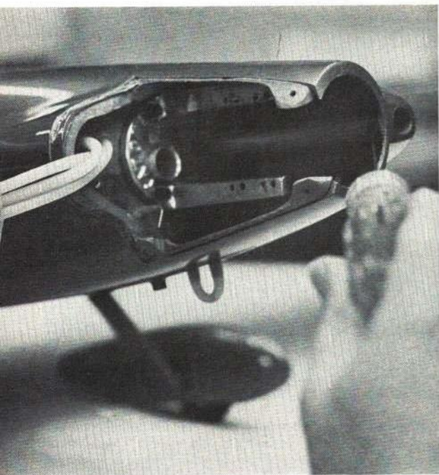
Tatone long-beam engine mount holds the engine firmly enough because the firewall is rigid and well anchored to the fiberglass fuselage sides. Tube from left cowl brings ram air to carburetor.
