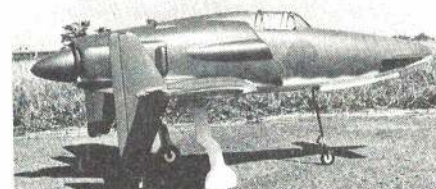
Rare Japanese WW-II pusher fighter design modeled by Tom Tjarda. Has Rossi 60 and retracts.
