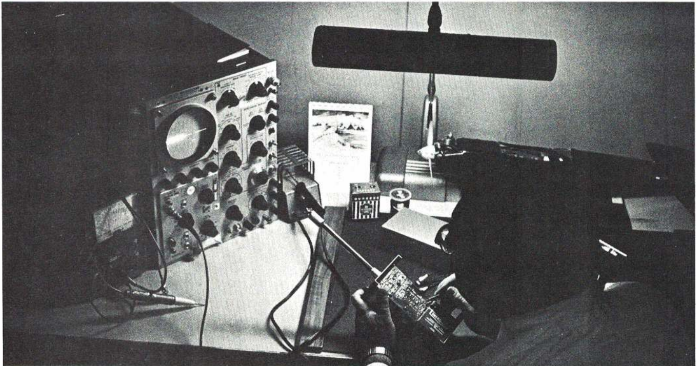
Using a Tektronix 435 scope, Fred Marks checks encoder pulses. Scope is also capable of showing modulation patterns at 27MHz.
