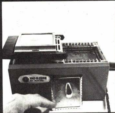
A Mattel Vac-U-Form is used to make the radome and the nose turret.
