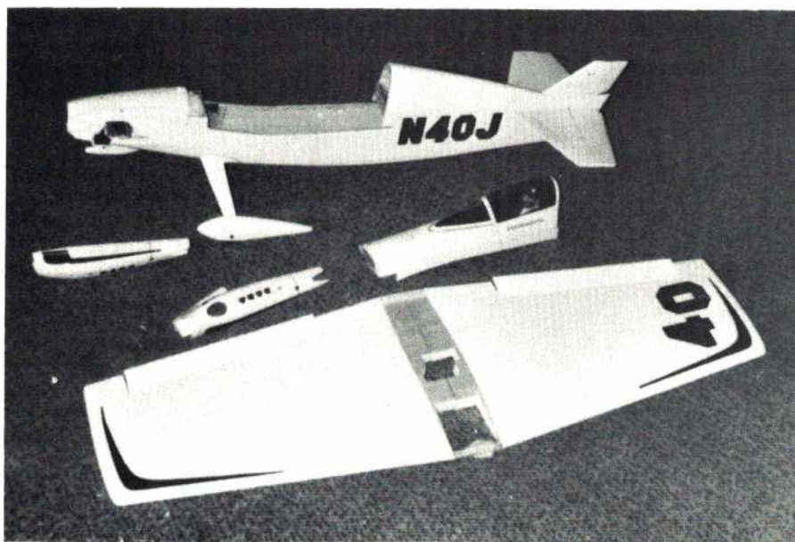
The wing is pre-MonoKoted, except for the gluing area. The canopy assembly will be permanently affixed later. It's nice to build in this modular fashion, since the components may be easily handled all the way through the finishing stages.
