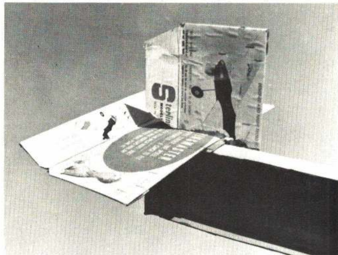
Subtle, isn't it! At first glance, one easily misses the staples (heavy-duty type), split corrugation hinging (a process which the U.S. Patent Office rejected), and the stressed skin control surfaces. Eat your heart out, EAA homebuilders; we modelers got all these methods first!
