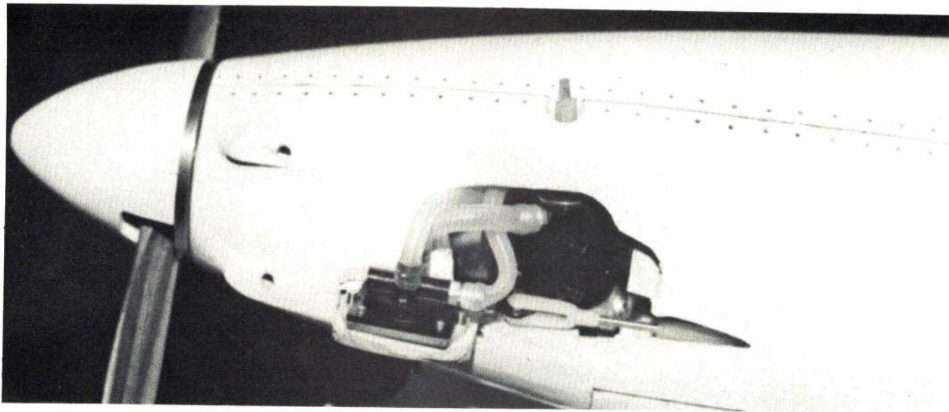
Jenesco fueling system hidden under the cowl keeps nitro uncontaminated.
