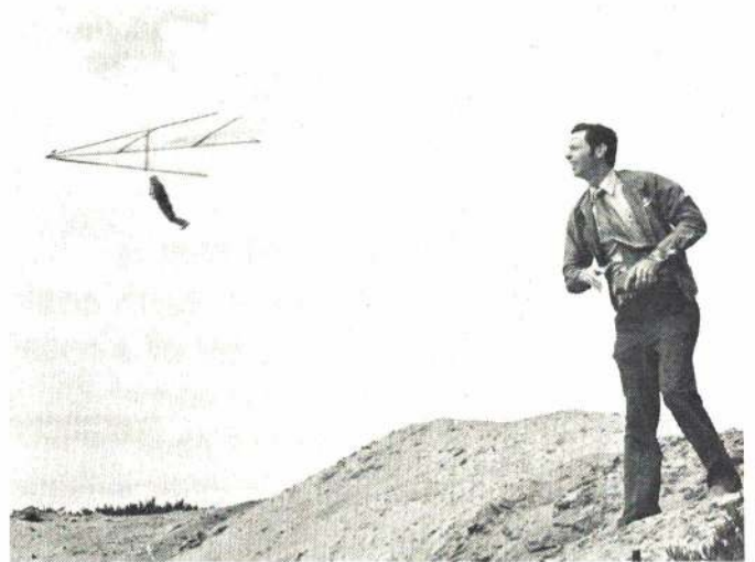
ABOVE: The doll in position on his hang bar, amid a maze of rigging. Tow hook release bridle is shown here. GI Joe is also available with a beard. BELOW: GI Joe takes a hop aboard his Flexi-Flier. Note that the author holds the transmitter at a 45° angle, a clever way to get elevon control. Watch that you don't detune the signal by accidentally grounding the antenna with your hand. (Photo by Jerry Trager)
