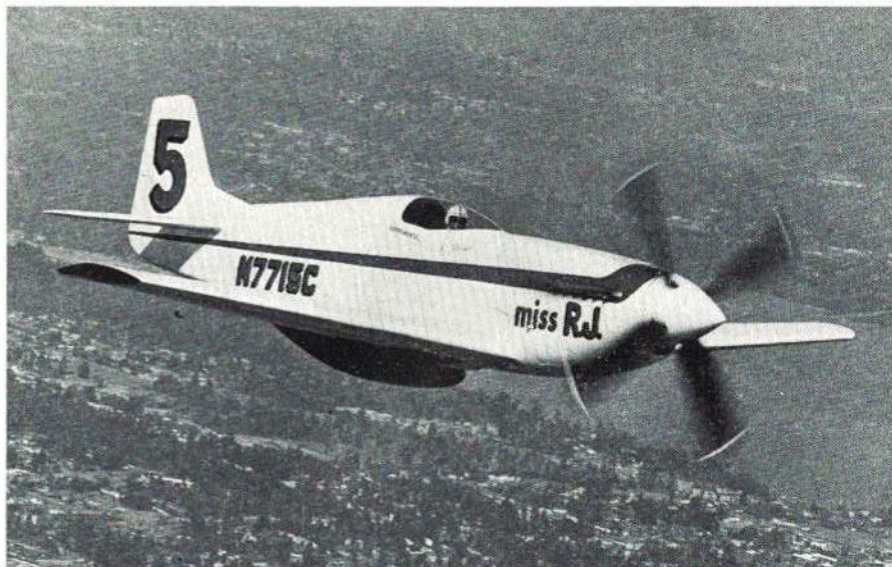
Clean, much modified P-51D flown by Chuck Hall placed second in pylon races at 377 mph. Drawing prepared by Hall's crew chief.
