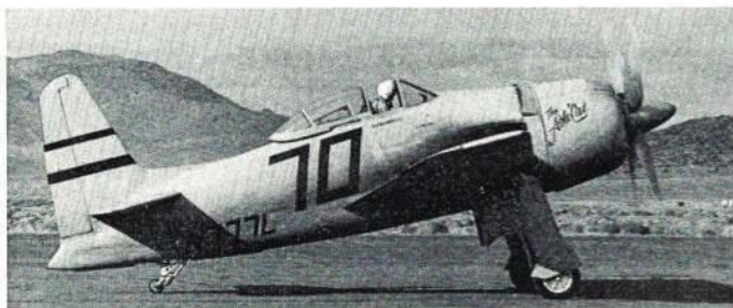
The distinguishing feature of Able Cat is not visible; under that normal cowl is huge Wright engine. Still testing, not even painted.
