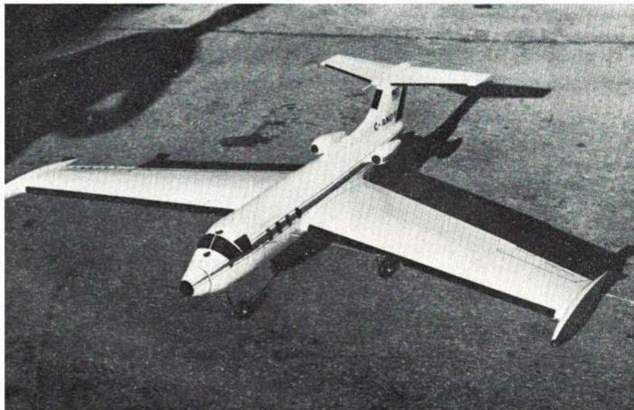
Semi-scale Hansa-Jet will fly a nice AMA pattern. Engine is neatly hidden in cockpit area. Fine-mesh window screen simulates the cockpit windshield. Designed/flown by Mike Scott.
