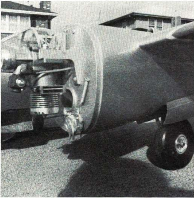
With practice, inverted engine installation is just as easy to start and operate as any other. It is not a factor in reliability. Glow heat improves any engine or installation.
