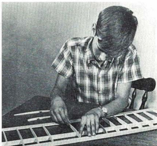
Assemble the wing on flat surface by pinning spars to tip ribs, then fit in all other ribs. Align structure, pin, and glue together.
