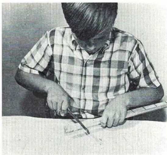
Leading and trailing edges are made by taping them together and then cutting the rib notches with a doubled hacksaw blade.
