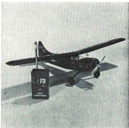
Test-flight plane is Sig's D. H. Beaver. Wing was painted with foam spray colors, fuel-proofed, with sprayed polyurethane.
