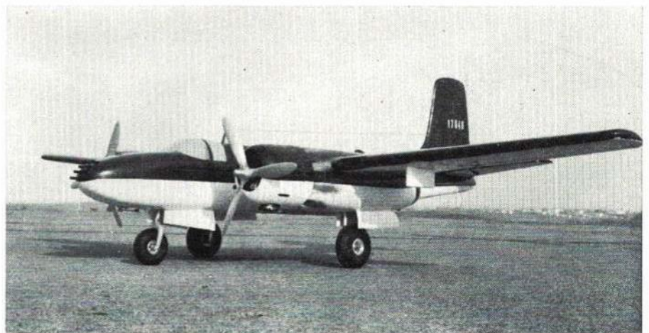
Author's other twin is B-26 Invader with two inverted 60's. Besides reliability, another benefit of glow heat is engines stay in synchronization through all throttle settings.
