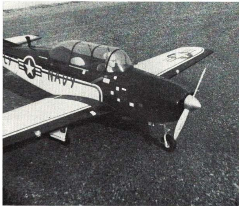
Bud Atkinson uses a D cell NiCad in his Mentor. He even uses it for starting—which looks mighty impressive to the judges at a contest. He still gets about ten flights per charge.
