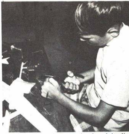
With pliers, bend the pushrod and landing gear wires to shape.
