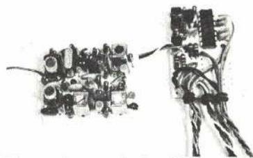
The receiver uses just well-proven techniques, double-tuned front end and three-stage IF. Note the decoder has space for another IC and associated components for more functions.
